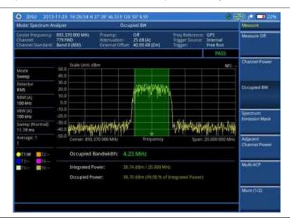
Figure 15 Occupied bandwidth measurement with spectrum analyzer
