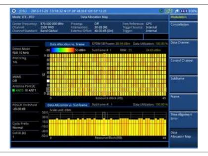
Figure 107 Data allocation map measurement with LTE - FDD signal analyzer (MBMS On)
