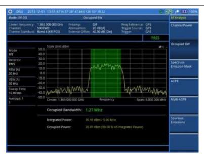
Figure 190 Occupied bandwidth measurement with EV-DO signal analyzer
