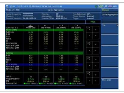
Figure 151 Carrier aggregation measurement with LTE - TDD signal analyzer (SA)
