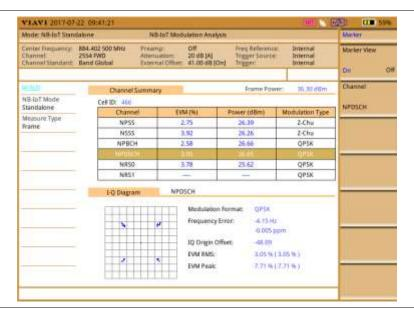
Figure 268 NB-IoT Standalone Modualtion Analysis measurement screen (Subframe 0- NPBCH)
