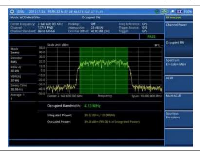
Figure 63 Occupied bandwidth measurement with WCDMA/HSPA+ signal analyzer
