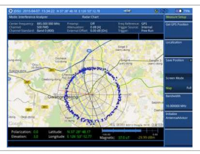
Figure 38 Localized RSSI data on the radar chart
