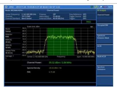
Figure 62 Channel power measurement with WCDMA/HSPA+ signal analyzer
