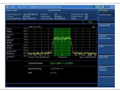
Figure 166 Channel power measurement with CDMA signal analyzer
