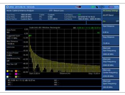
Figure 281 DTF measurement with the alternate DTF band on
