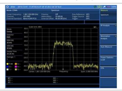
Figure 165 Spectrum measurement screen with CDMA signal analyzer
