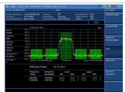
Figure 65 ACLR measurement with WCDMA/HSPA+ signal analyzer
