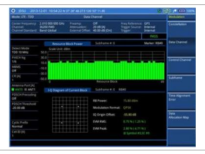
Figure 140 Data channel measurement with LTE - TDD signal analyzer (MBMS On)
