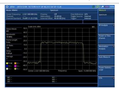
Figure 238 Spectrum measurement screen with Mobile WiMAX signal analyzer
