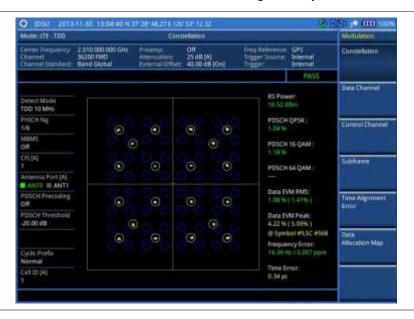
Figure 138 Constellation measurement with LTE - TDD signal analyzer (MBMS On)
