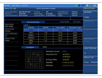
Figure 122 NB-IoT modulation measurement with LTE-FDD signal analyzer (Subframe 2)
