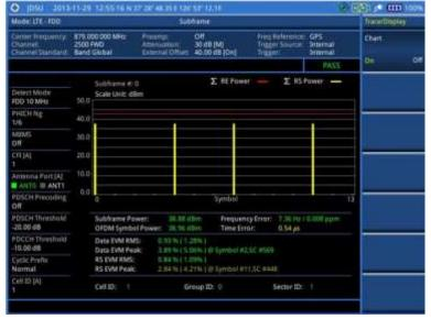
Figure 102 Subframe measurement with LTE - FDD signal analyzer (MBMS On)
