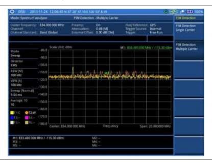
Figure 26 PIM detection for multiple carriers
