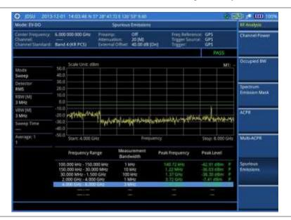
Figure 194 Spurious emissions measurement with EV-DO signal analyzer
