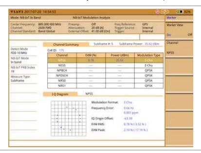
Figure 258 NB-IoT In Band Modualtion Analysis measurement screen (Subframe 5-NPSS)
