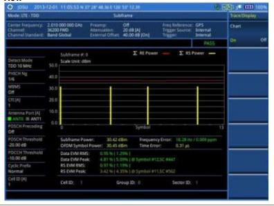
Figure 144 Subframe measurement with LTE - TDD signal analyzer (MBMS On)
