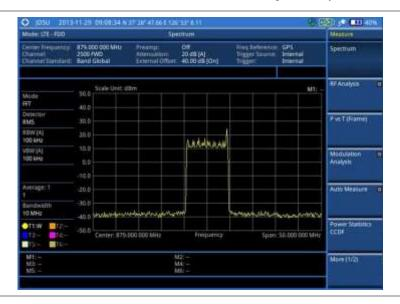
Figure 86 Spectrum measurement screen with LTE - FDD signal analyzer
