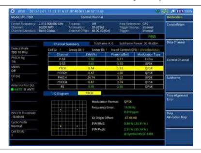
Figure 142 Control channel measurement with LTE - TDD signal analyzer (MBMS On)
