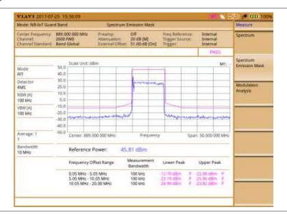
Figure 259 Spectrum Emission Mask measurement screen
