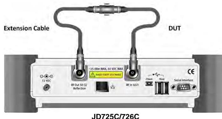
Figure 59 Connection diagram for 2-port phase measurements
