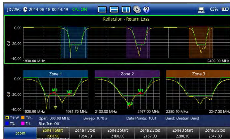
Figure 90 Reflection return loss measurement with zoom zones
