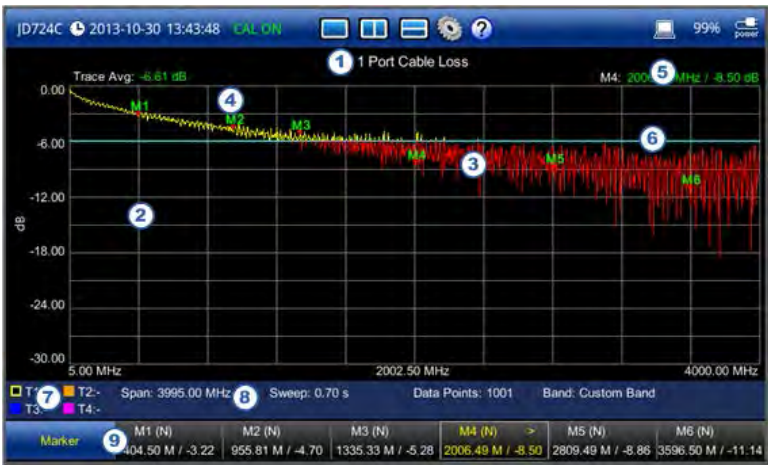
Figure 33 1 port cable loss measurement screen
