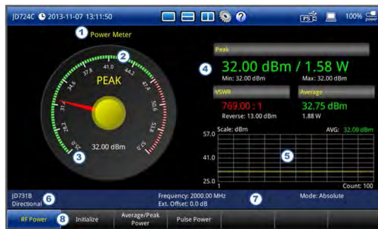
Figure 62 RF power measurement screen
