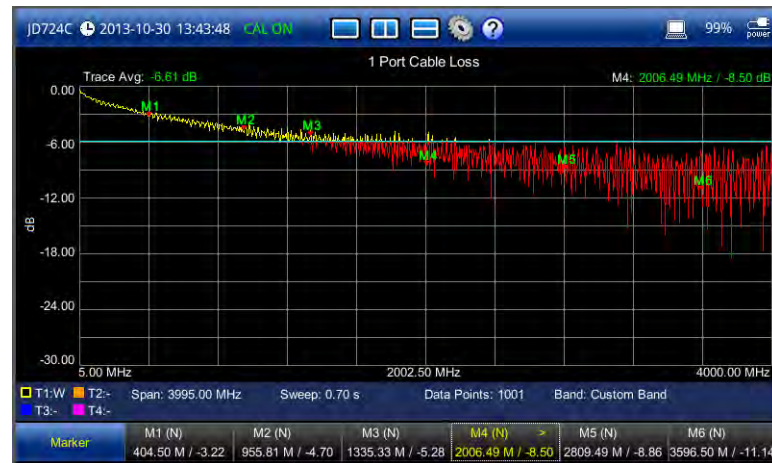
Figure 38 1 port cable loss measurement screen (zoom zones)
