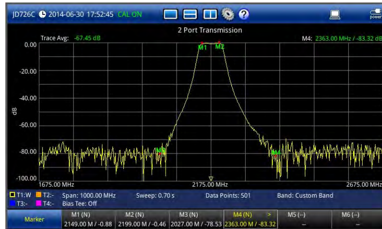
Figure 55 2 port transmission measurement screen (single layout)
