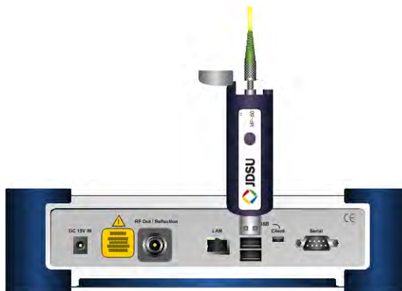
Figure 73 Cable connection diagram for optical power meter
