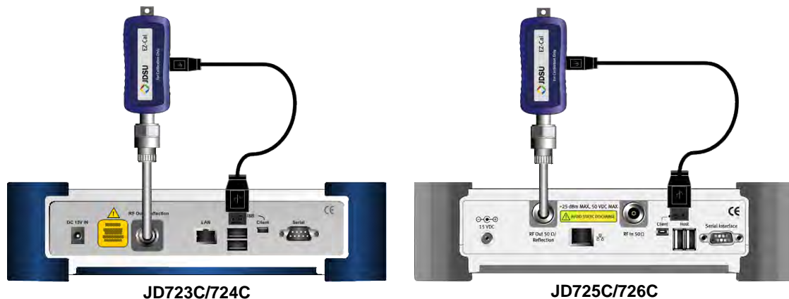
Figure 9 e-Calibration connection diagram with an extension cable
