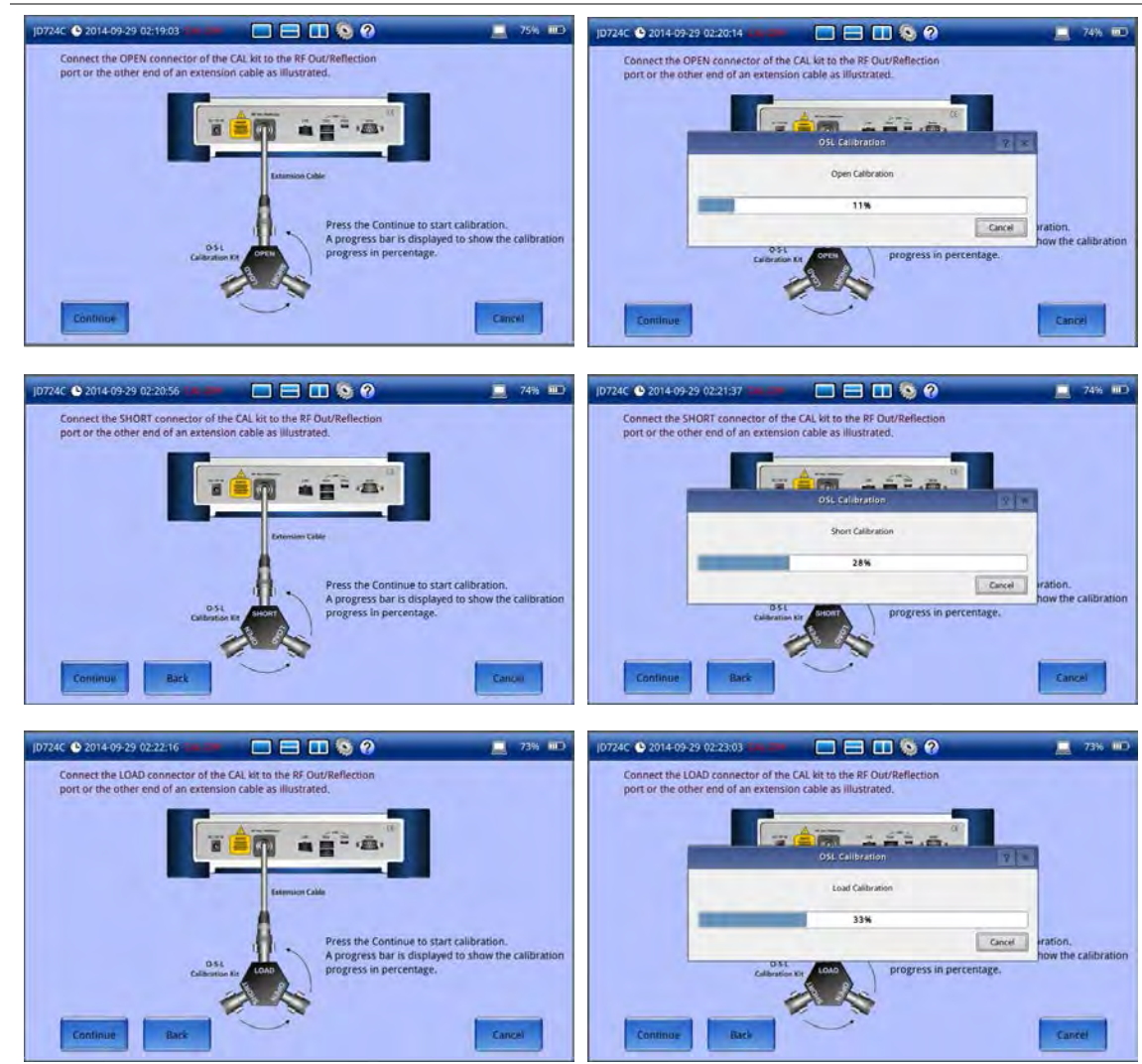
Figure 7 O-S-L calibration on JD724C using Y-Cal kit
