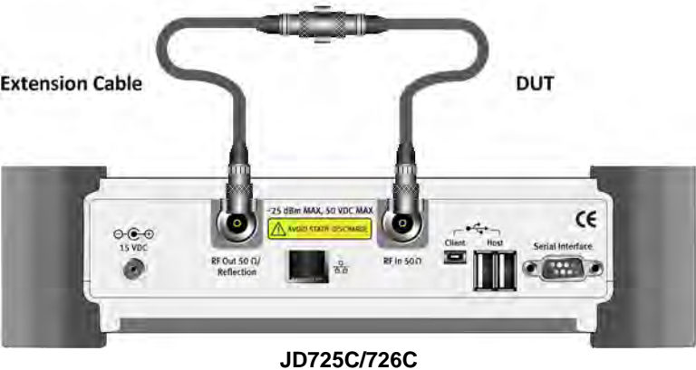
Figure 54 Connection diagram for 2-port transmission measurements
