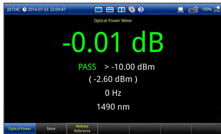
Figure 75 Relative optical power measurement vs. reference
