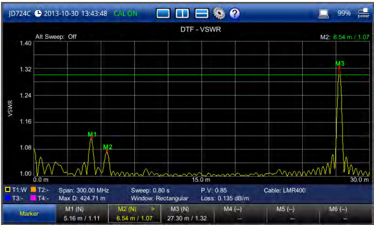
Figure 29 DTF return loss measurement screen (single layout)
