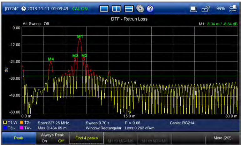
Figure 29 DTF return loss measurement screen (single layout)
