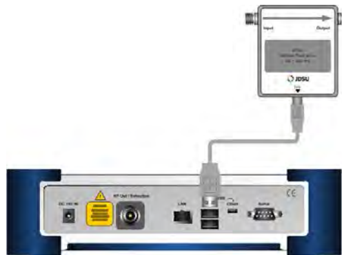
Figure 67 Cable connection diagram for directional power sensor
