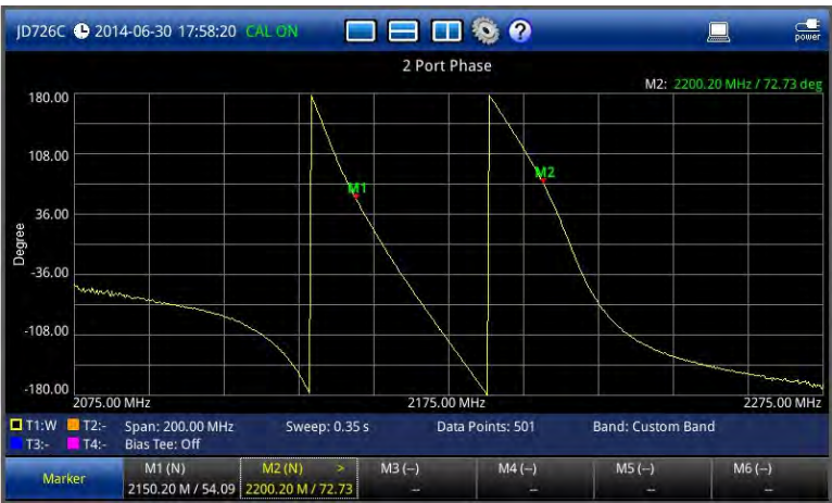
Figure 60 2 port phase measurement screen (single layout)
