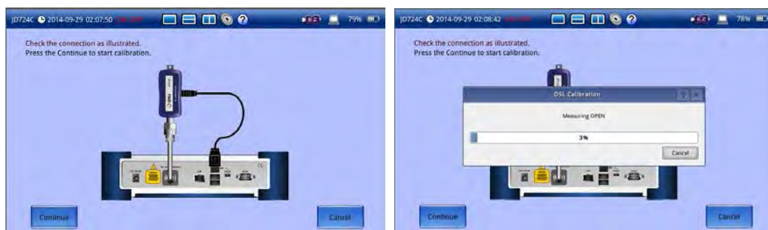
Figure 10 e-Calibration on JD724C using EZ-Cal kit
