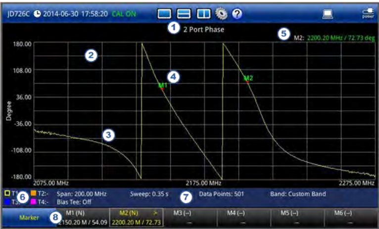
Figure 56 2 port phase measurement screen
