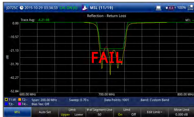
Figure 87 Task #11 “Limit Line - MSL” in Reflection – Return Loss
