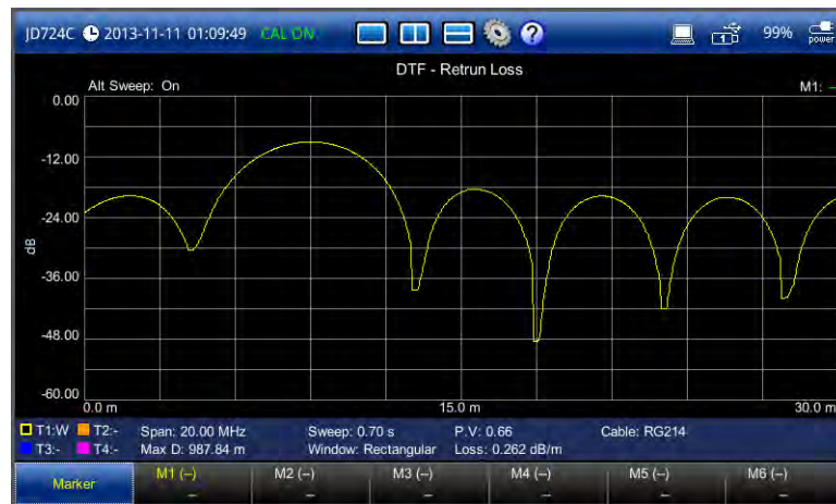
Figure 30 DTF return loss measurement screen (alternate sweep on)
