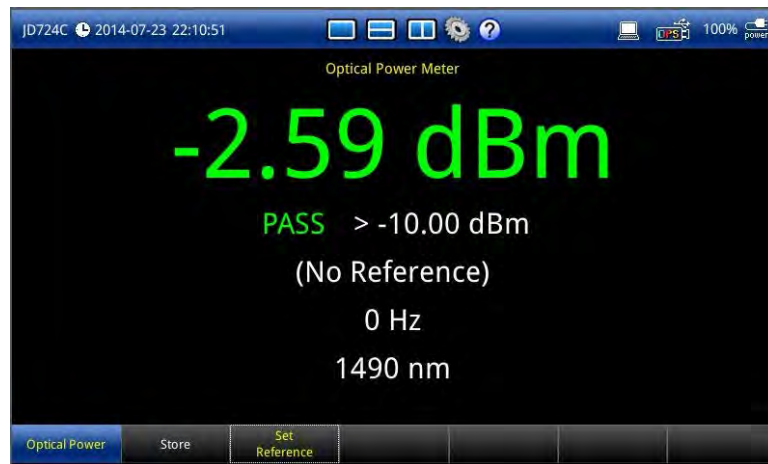
Figure 75 Relative optical power measurement vs. reference
