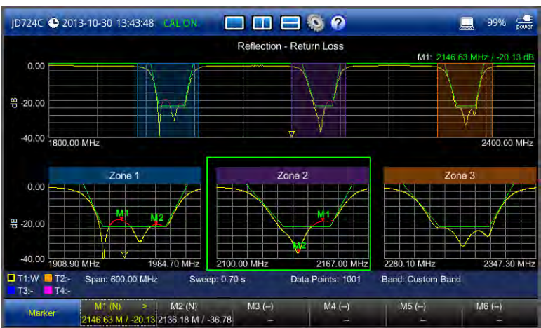
Figure 21 Reflection return loss measurement screen (zoom zones)
