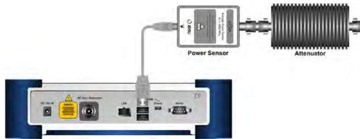
Figure 66 Cable connection diagram for terminating power sensor
