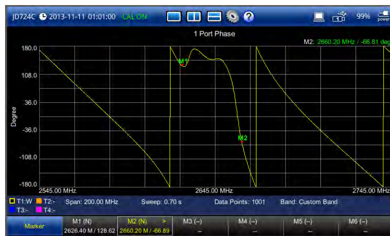
Figure 43 1 port phase measurement screen (single layout)
