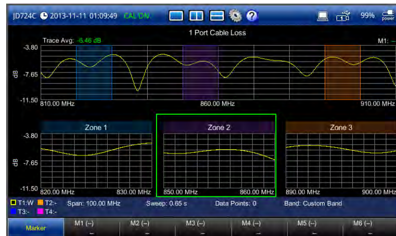
Figure 38 1 port cable loss measurement screen (zoom zones)
