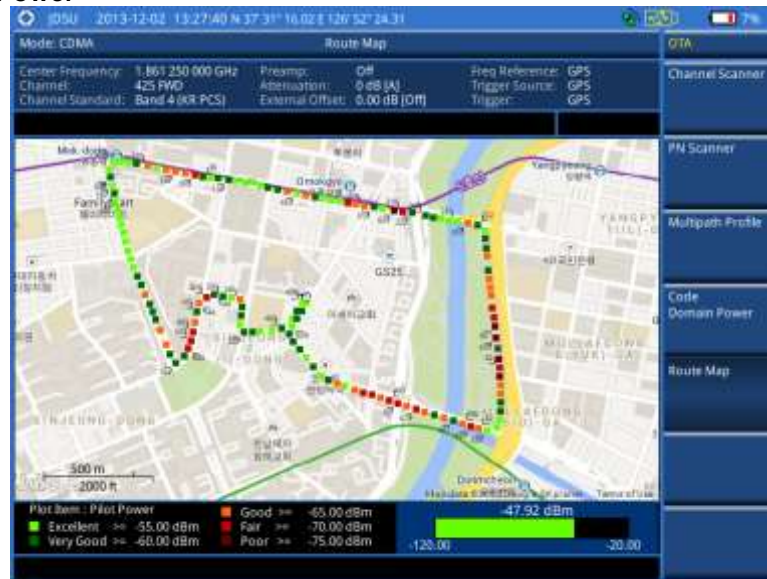
Figure 178 Route map measurement with CDMA OTA signal analyzer
