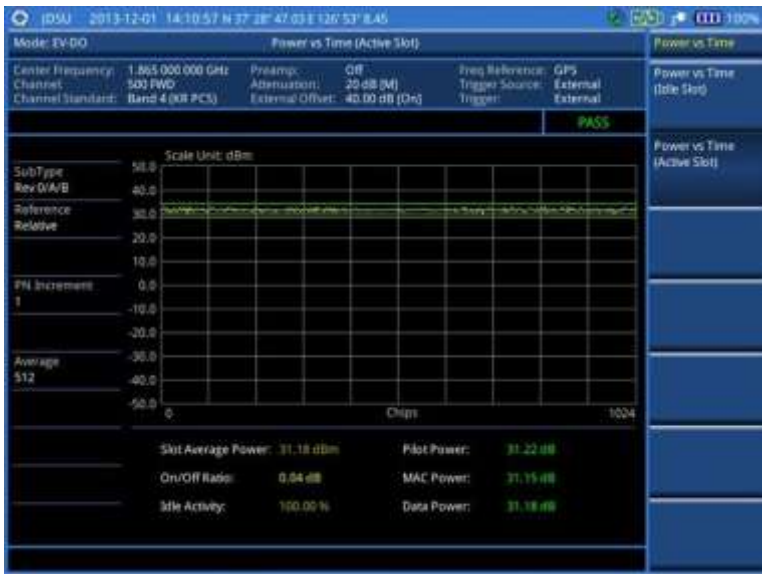
Figure 192 Power vs. time (active slot) measurement with EV-DO signal analyzer
