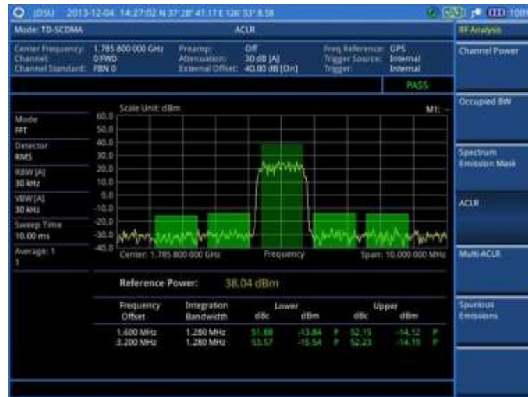
Figure 213 ACLR measurement with TD-SCDMA signal analyzer
