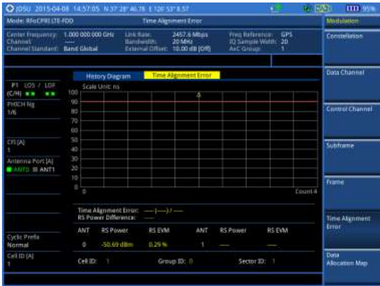
Figure 296 Time alignment error measurement with RFoCPRI LTE-FDD signal analyzer
