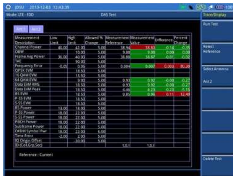
Figure 107 DAS measurement with LTE-FDD signal analyzer
