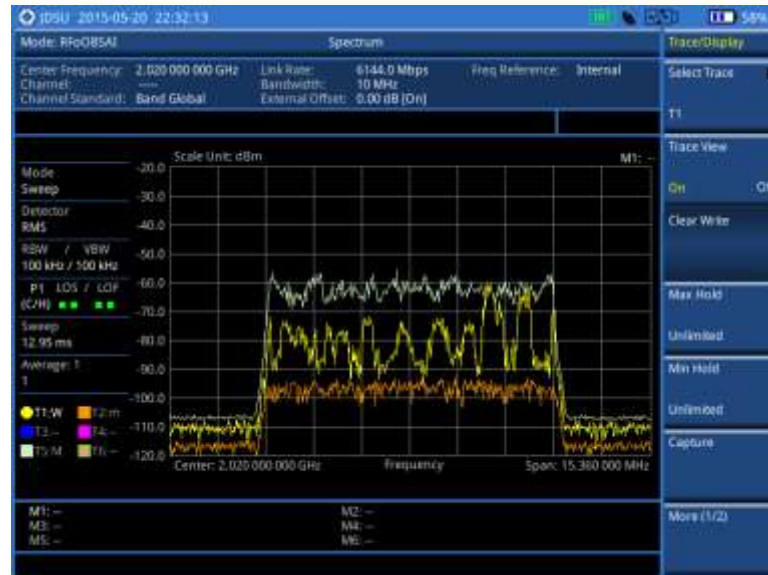
Figure 305 RFoBSAI spectrum measurement
