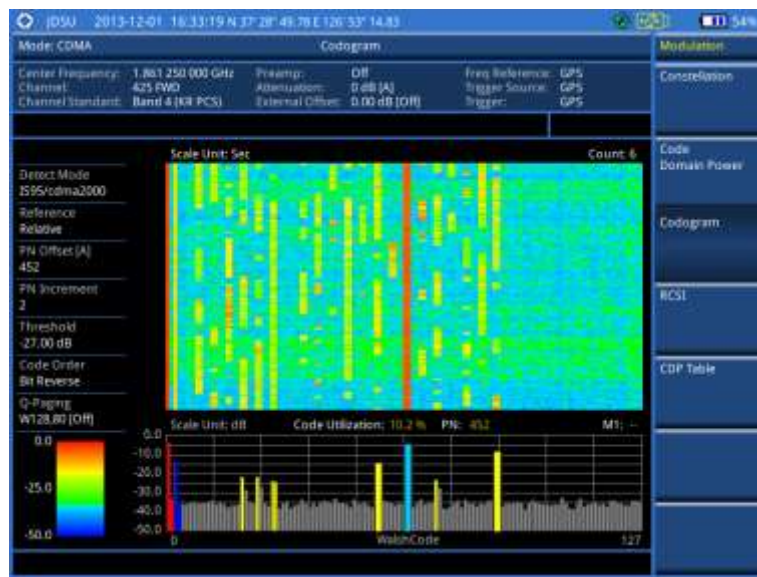
Figure 170 Codogram in full view with CDMA signal analyzer
