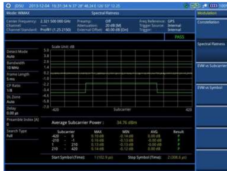
Figure 241 Spectral flatness measurement with Mobile WiMAX signal analyzer
