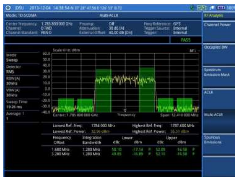
Figure 214 Multi-ACLR measurement with TD-SCDMA signal analyzer
