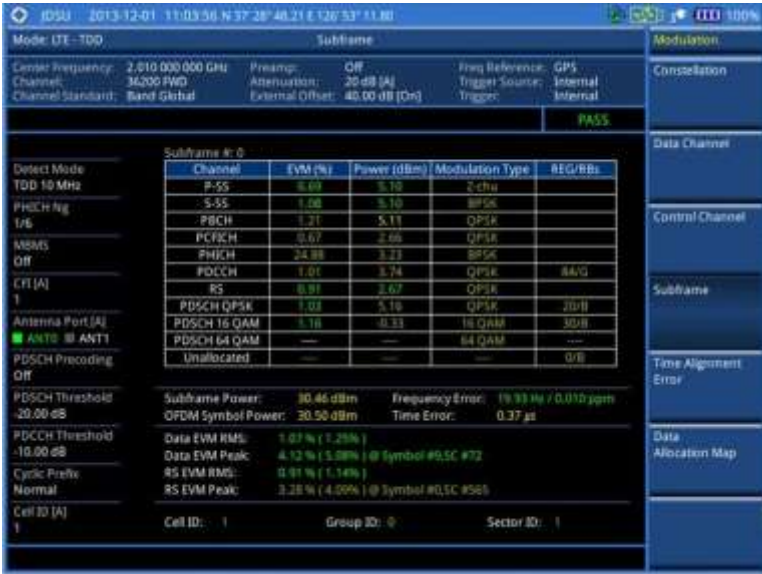
Figure 139 Subframe measurement with LTE-TDD signal analyzer
