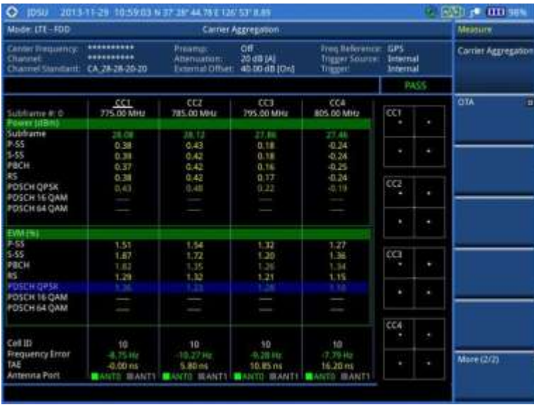
Figure 110 Carrier aggregation measurement with LTE-FDD signal analyzer (SA)
