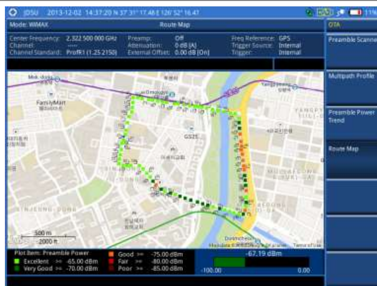
Figure 248 Route map measurement with Mobile WiMAX OTA signal analyzer
