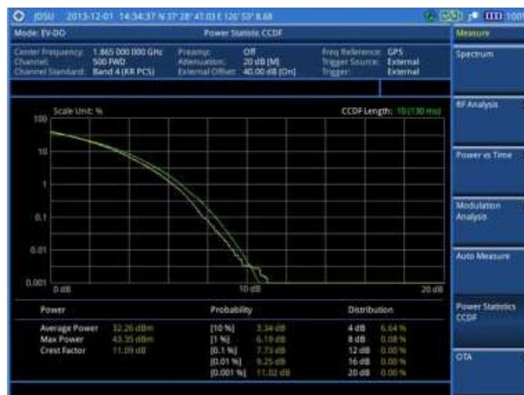
Figure 198 CCDF measurement with EV-DO signal analyzer
