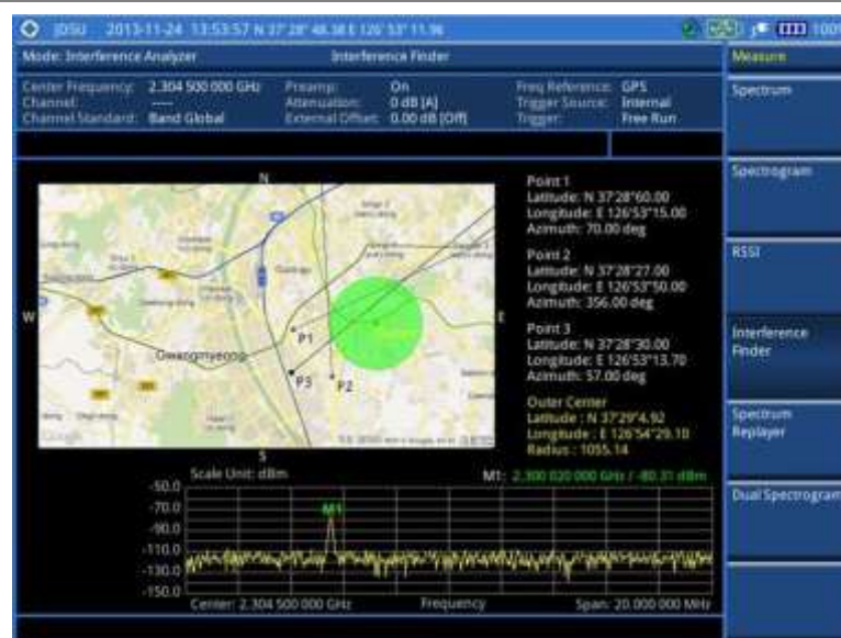
Figure 33 Interference finder measurement in map view
