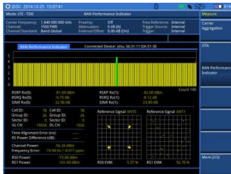
Figure 155 RAN performance indicator with LTE-TDD signal analyzer
