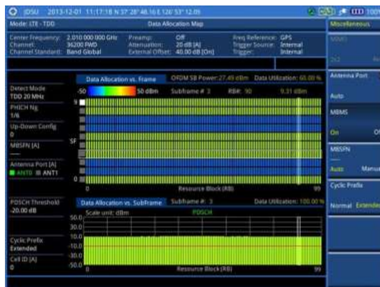
Figure 143 Data allocation map measurement with LTE-TDD signal analyzer (MBMS On)
