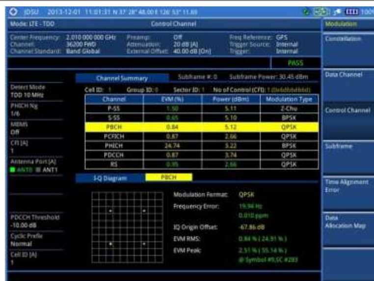
Figure 138 Control channel measurement with LTE-TDD signal analyzer (MBMS On)
