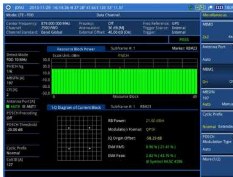
Figure 97 Data channel measurement with LTE-FDD signal analyzer (MBMS On)
