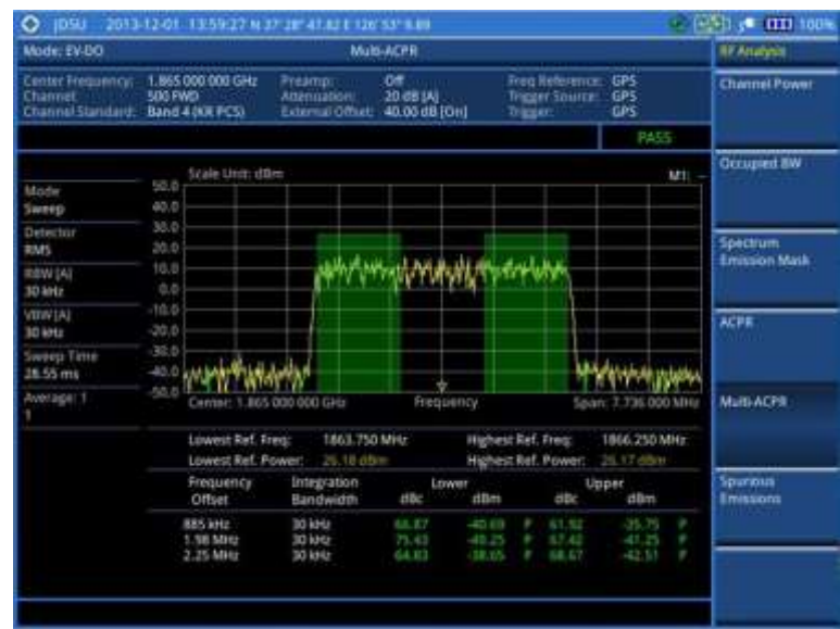
Figure 189 Multi-ACPR measurement with EV-DO signal analyzer
