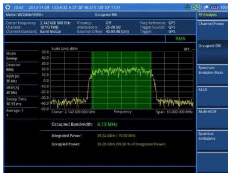
Figure 63 Occupied bandwidth measurement with WCDMA/HSPA+ signal analyzer
