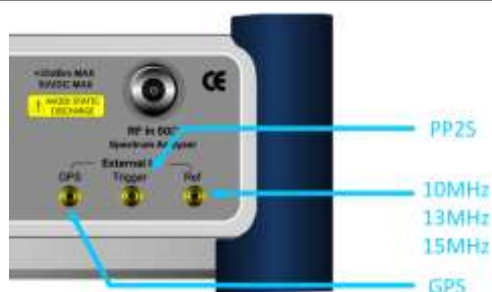
Figure 60 Connection ports for external reference clock
