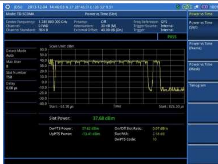
Figure 216 Power vs. time (slot) measurement with TD-SCDMA signal analyzer
