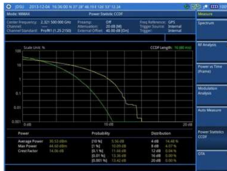
Figure 244 CCDF measurement with Mobile WiMAX signal analyzer
