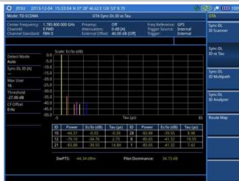
Figure 225 Sync-DL ID vs. Tau measurement with TD-SCDMA OTA signal analyzer
