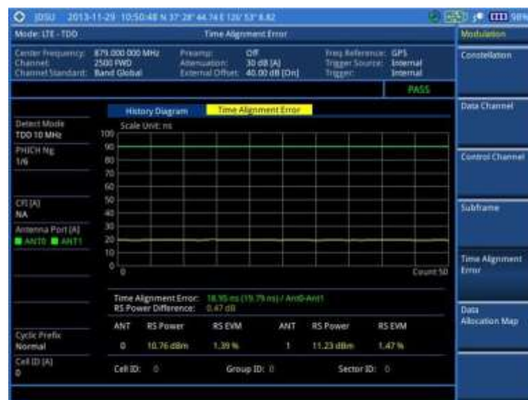
Figure 141 Time alignment error measurement with LTE-TDD signal analyzer
