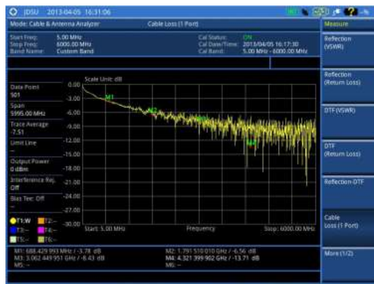
Figure 263 Cable loss (1 port) measurement
