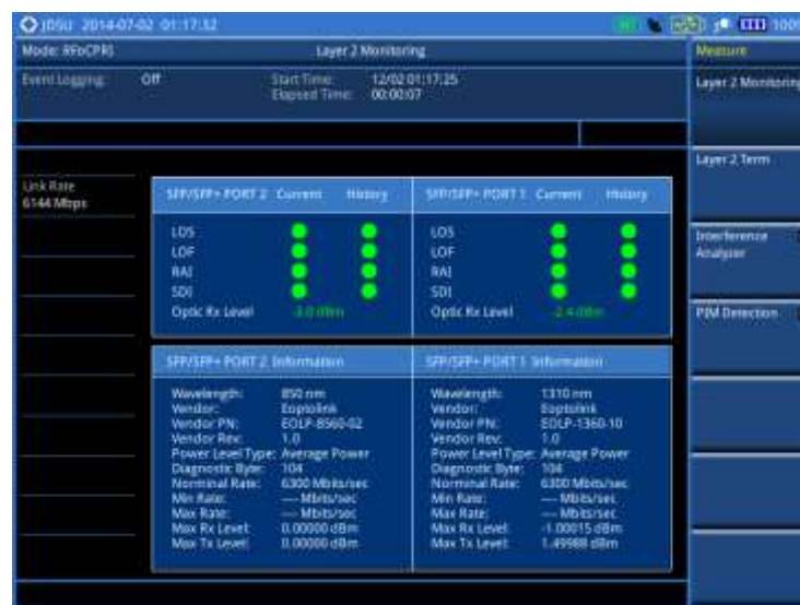
Figure 272 CPRI layer 2 monitoring
