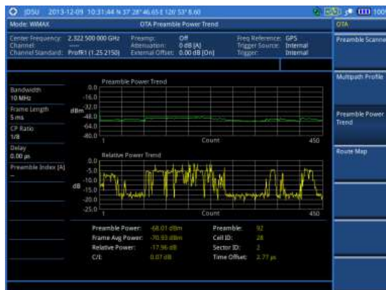
Figure 247 Preamble power trend with Mobile WiMAX OTA signal analyzer
