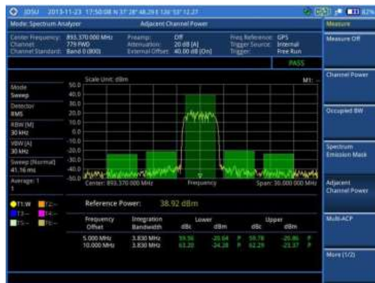
Figure 16 Adjacent channel power measurement with spectrum analyzer
