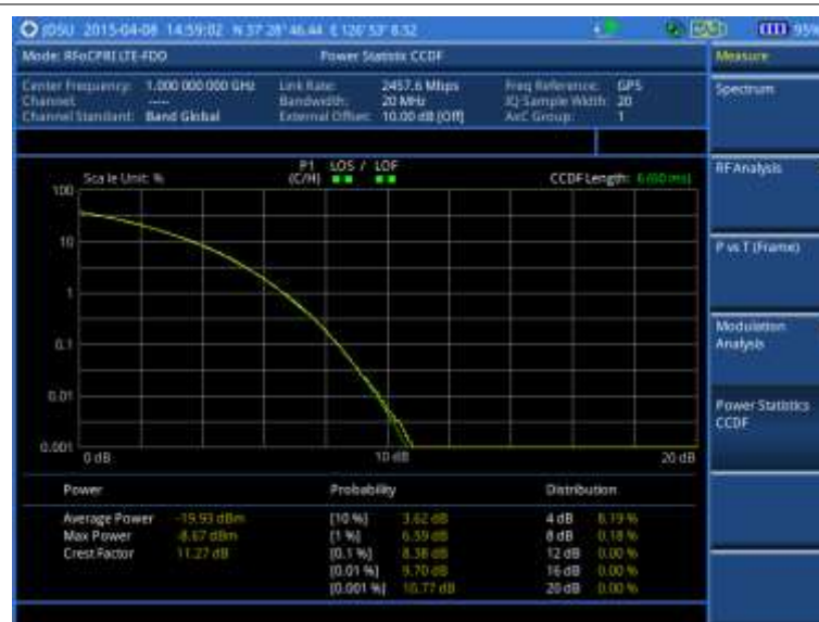
Figure 298 CCDF measurement with RFoCPRI LTE-FDD signal analyzer
