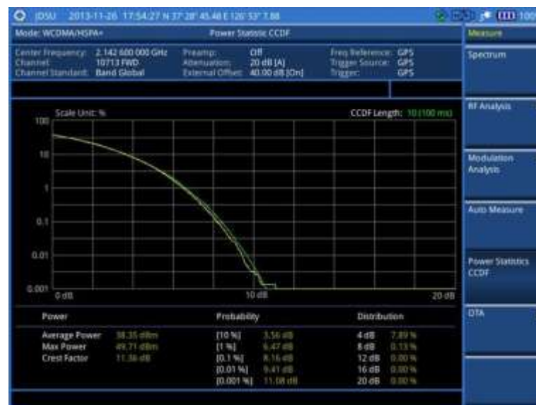
Figure 74 CCDF measurement with WCDMA/HSPA+ signal analyzer
