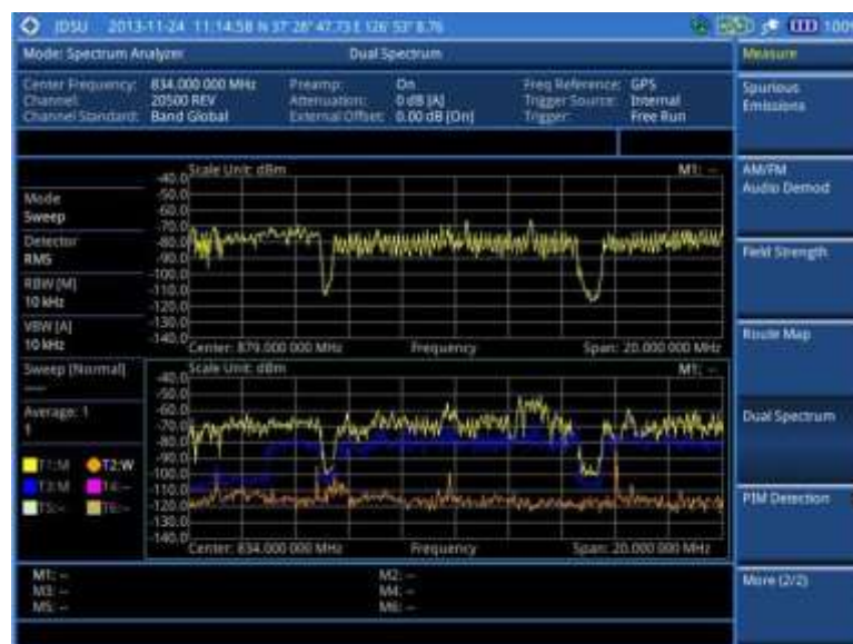
Figure 23 Dual spectrum measurement with spectrum analyzer
