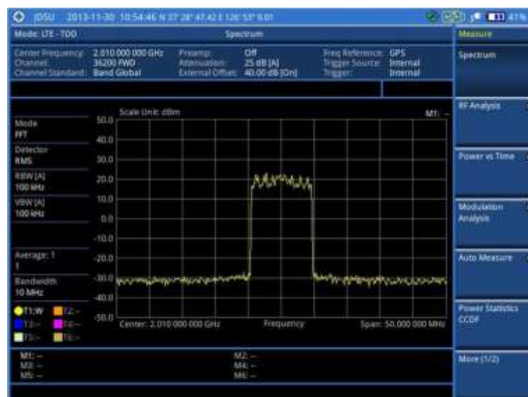
Figure 124 Spectrum measurement screen with LTE-TDD signal analyzer
