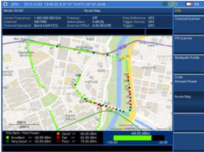
Figure 203 Route map measurement with EV-DO OTA signal analyzer
