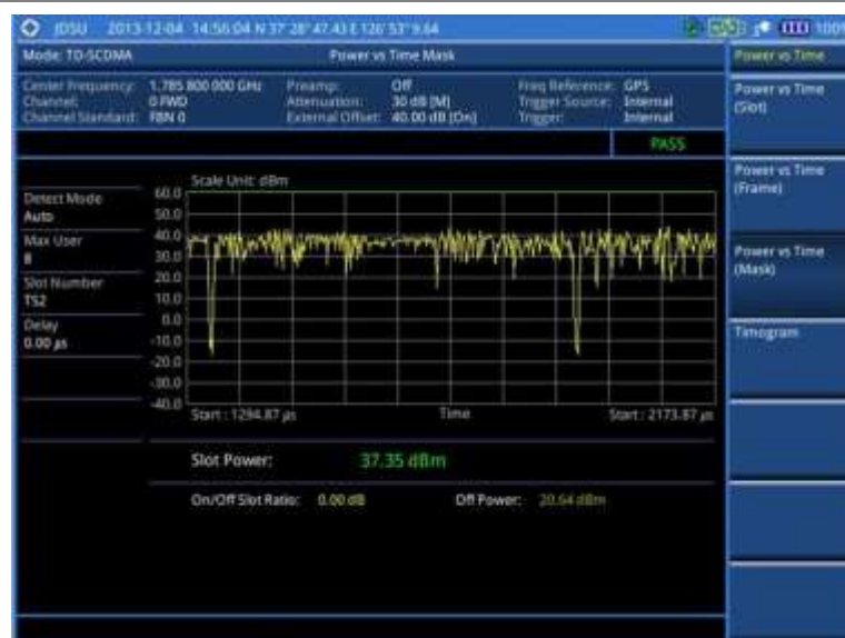
Figure 218 Power vs. time (mask) measurement with TD-SCDMA signal analyzer
