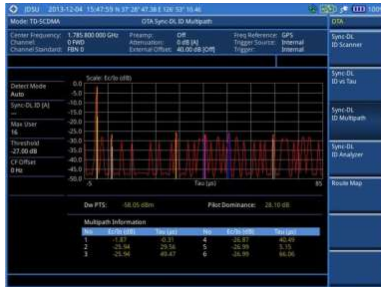
Figure 226 Sync-DL ID multipath measurement with TD-SCDMA OTA signal analyzer
