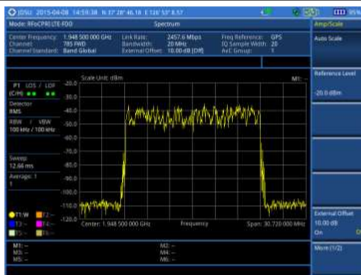
Figure 287 Spectrum measurement with RFoCPRI LTE-FDD signal analyzer
