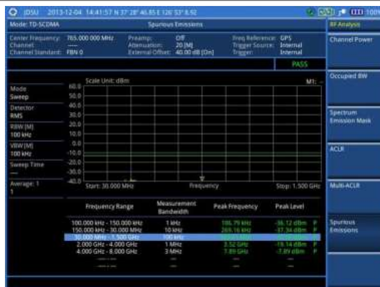
Figure 215 Spurious emissions measurement with TD-SCDMA signal analyzer
