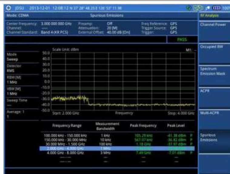
Figure 167 Spurious emissions measurement with CDMA signal analyzer
