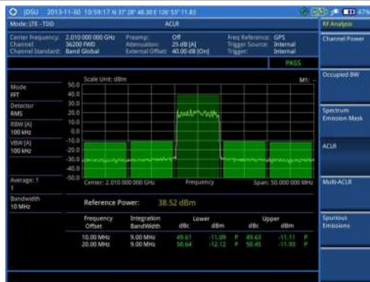
Figure 128 ACLR measurement with LTE-TDD signal analyzer
