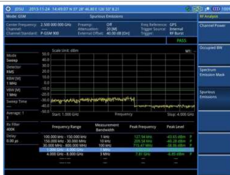
Figure 46 Spurious emissions measurement with GSM signal analyzer
