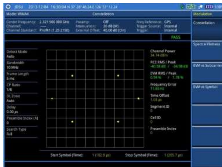
Figure 240 Constellation measurement with Mobile WiMAX signal analyzer
