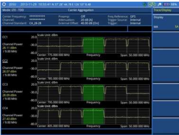
Figure 147 Carrier aggregation measurement with LTE-TDD signal analyzer (SA)
