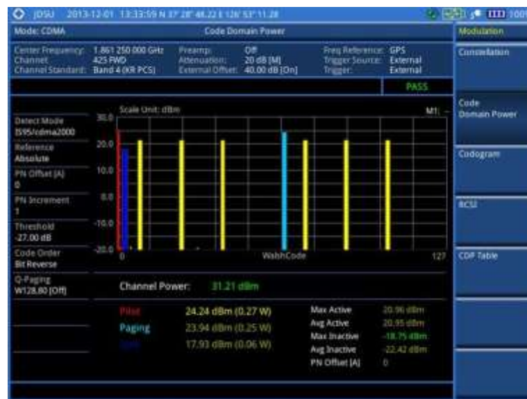
Figure 169 Code domain power measurement with CDMA signal analyzer
