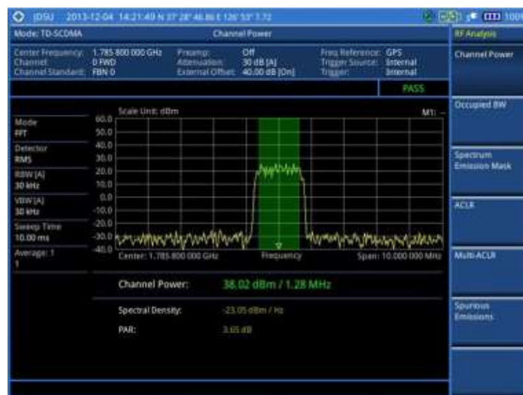
Figure 210 Channel power measurement with TD-SCDMA signal analyzer
