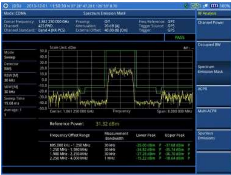
Figure 164 SEM measurement with CDMA signal analyzer
