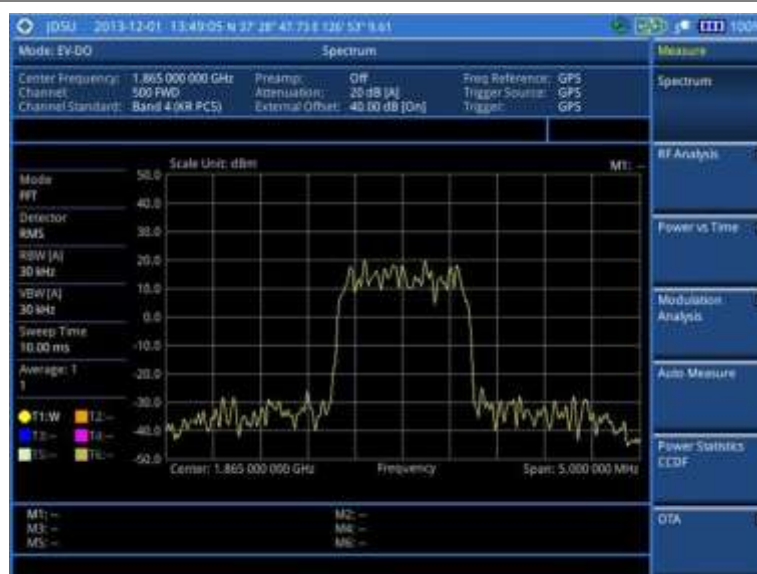
Figure 184 Spectrum measurement screen with EV-DO signal analyzer
