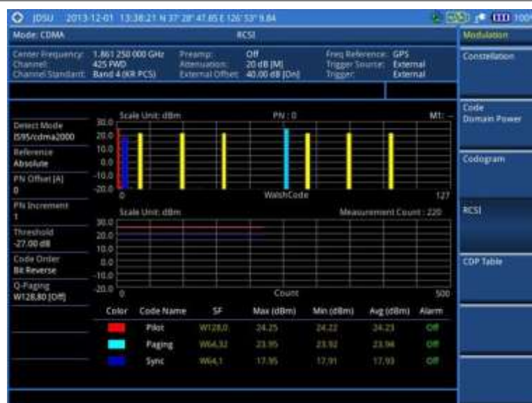
Figure 171 RCSI measurement with CDMA signal analyzer
