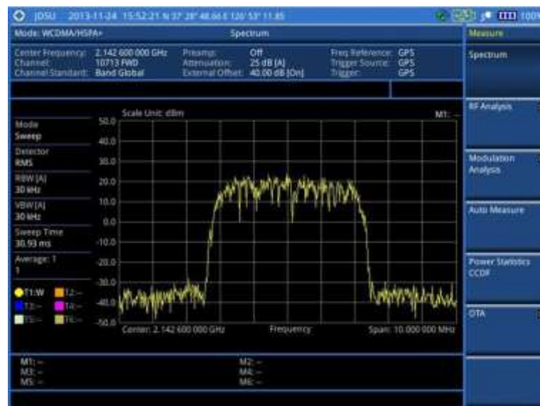
Figure 61 Spectrum measurement screen with WCDMA signal analyzer
