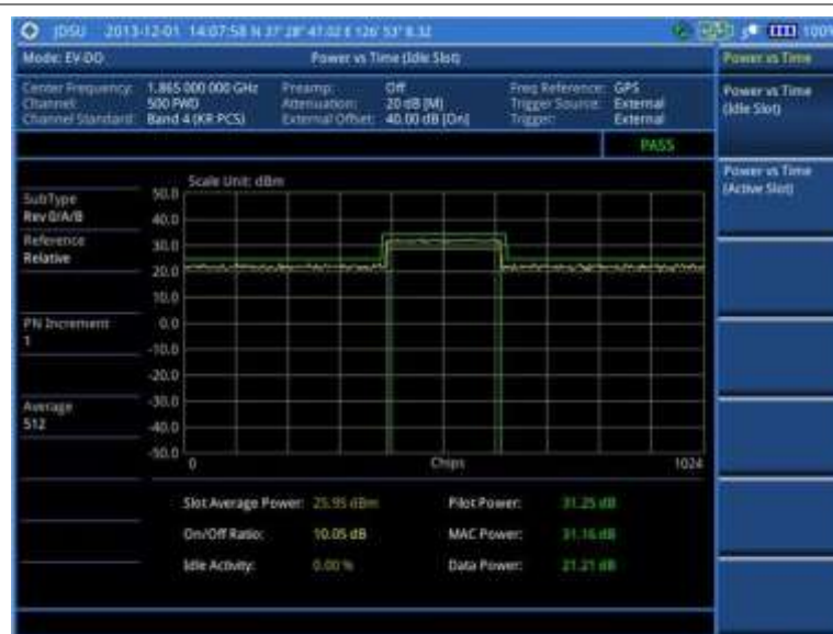
Figure 191 Power vs. time (idle slot) measurement with EV-DO signal analyzer
