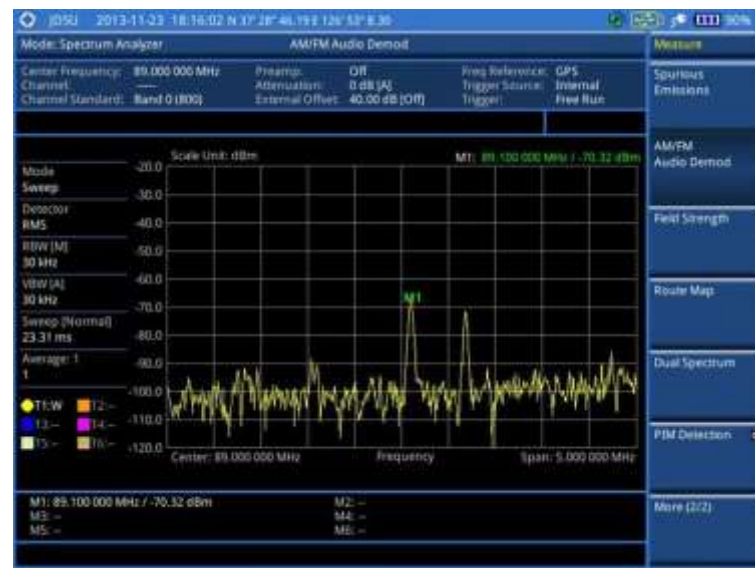
Figure 19 AM/FM audio demodulation with spectrum analyzer
