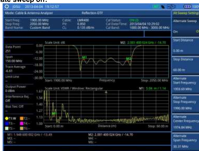
Figure 262 Reflection-DTF dual measurement
