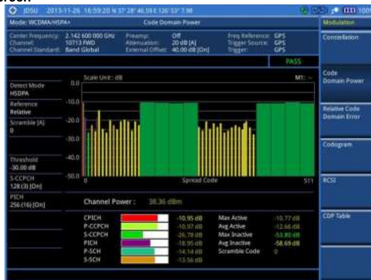
Figure 69 Code domain power measurement with WCDMA/HSPA+ signal analyzer
