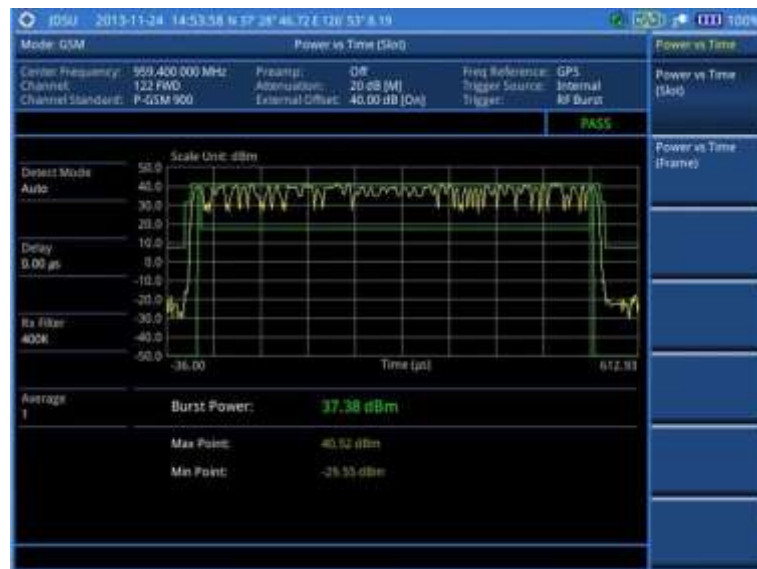
Figure 48 Power vs. time (slot) measurement with GSM signal analyzer
