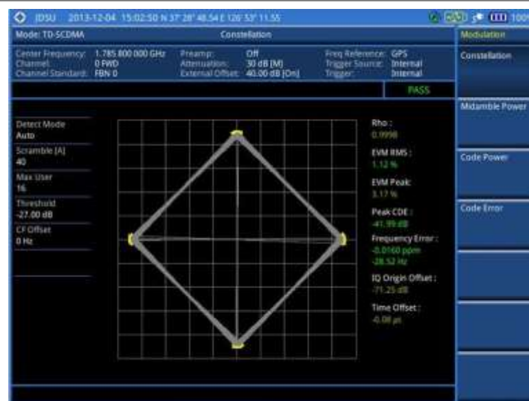
Figure 220 Constellation measurement with TD-SCDMA signal analyzer
