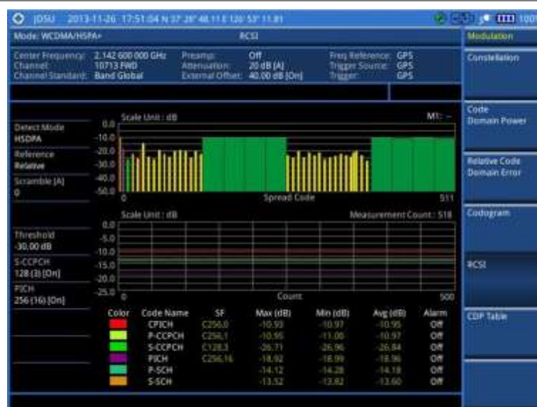
Figure 72 RCSI measurement with WCDMA/HSPA+ signal analyzer
