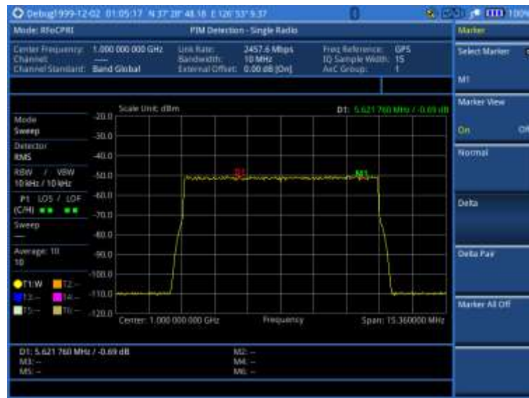
Figure 285 PIM detection of single radio
