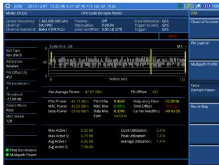
Figure 202 Code domain power measurement with EV-DO OTA signal analyzer
