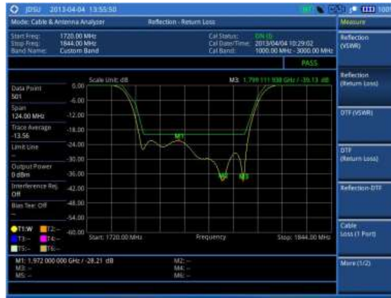
Figure 259 Reflection measurement in return loss scale
