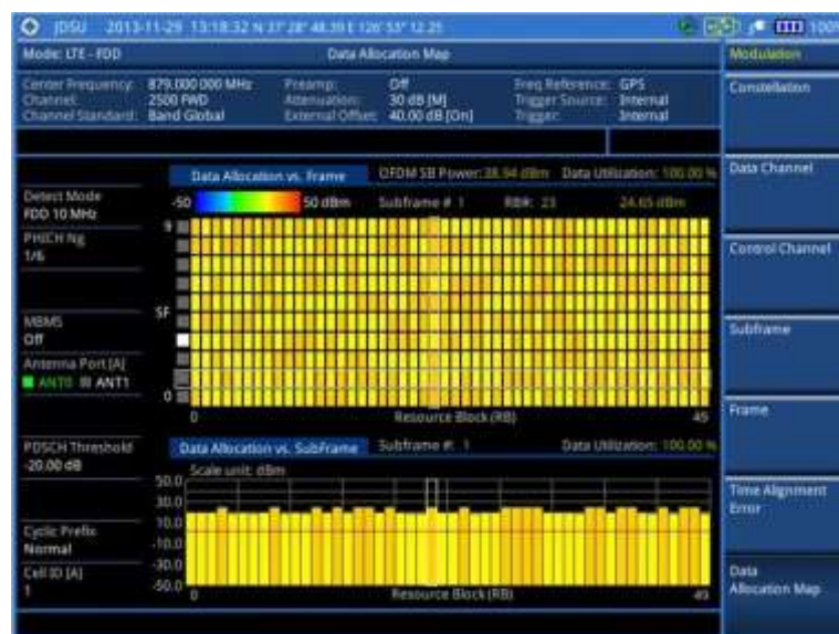
Figure 106 Data allocation map measurement with LTE-FDD signal analyzer (MBMS On)
