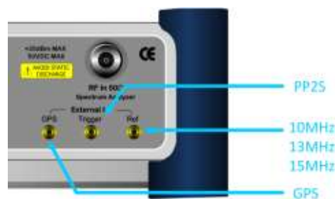
Figure 233 Connection ports for external reference clock
