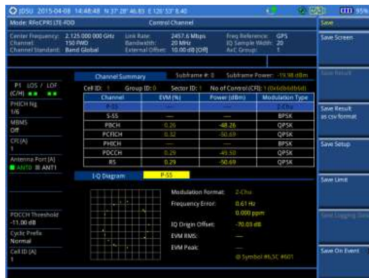
Figure 293 Control channel measurement with RFoCPRI LTE-FDD signal analyzer
