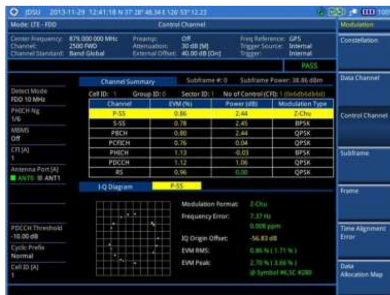
Figure 99 Control channel measurement with LTE-FDD signal analyzer (MBMS On)
