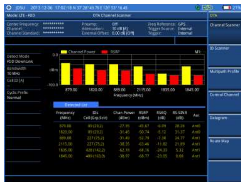
Figure 111 Channel scanner measurement with LTE-FDD OTA signal analyzer
