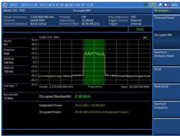
Figure 126 Occupied bandwidth measurement with LTE-TDD signal analyzer
