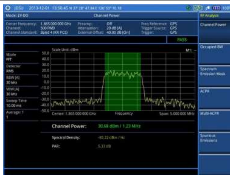
Figure 185 Channel power measurement with EV-DO signal analyzer
