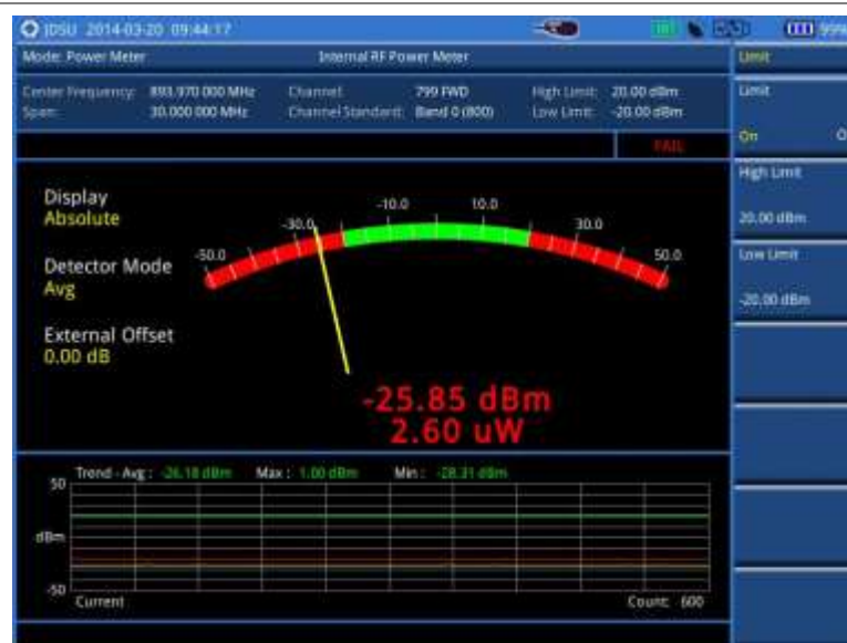
Figure 321 Internal power measurement
