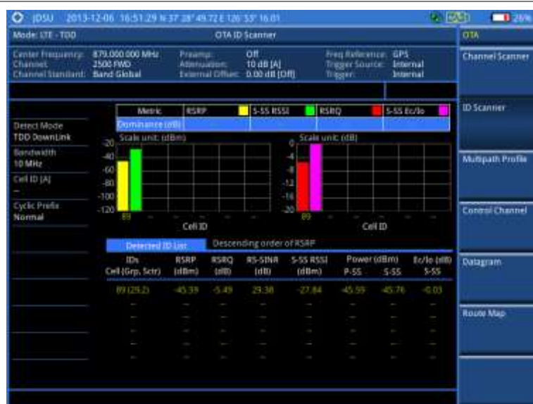
Figure 149 ID scanner measurement with LTE-TDD OTA signal analyzer
