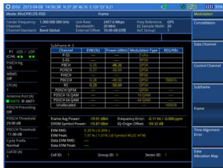
Figure 295 Frame measurement with RFoCPRI LTE-FDD signal analyzer
