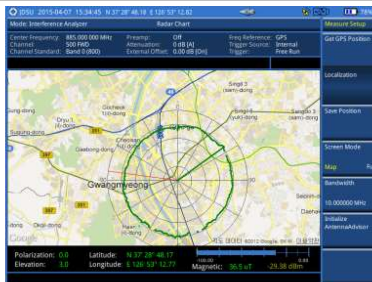
Figure 36 Localized RSSI data on the radar chart
