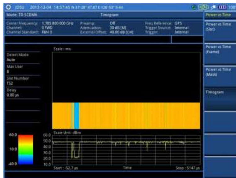
Figure 219 Timogram with TD-SCDMA signal analyzer
