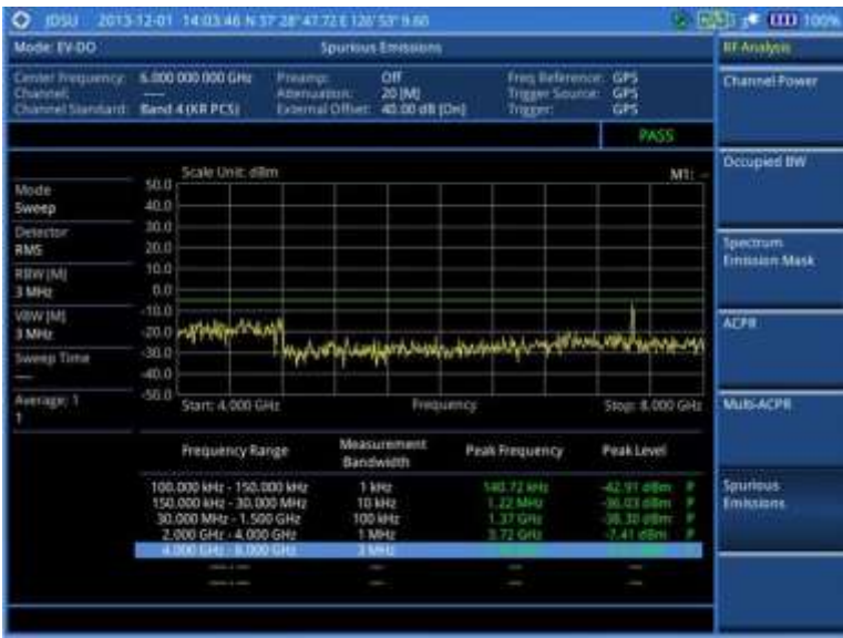
Figure 190 Spurious emissions measurement with EV-DO signal analyzer
