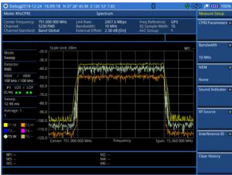
Figure 277 RFoCPRI spectrum analysis on LTE Uplink 10 MHz, antenna 1
