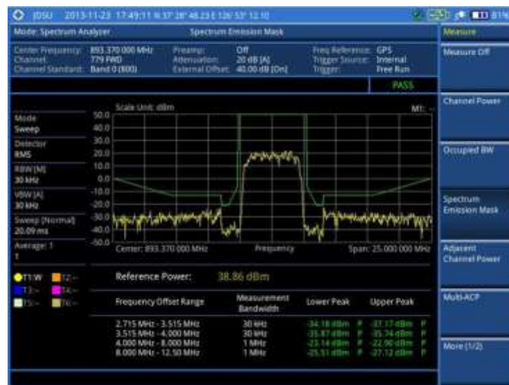
Figure 15 Spectrum emission mask measurement with spectrum analyzer
