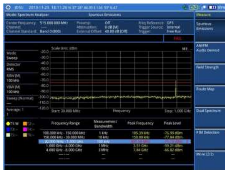
Figure 18 Spurious emissions measurement with spectrum analyzer
