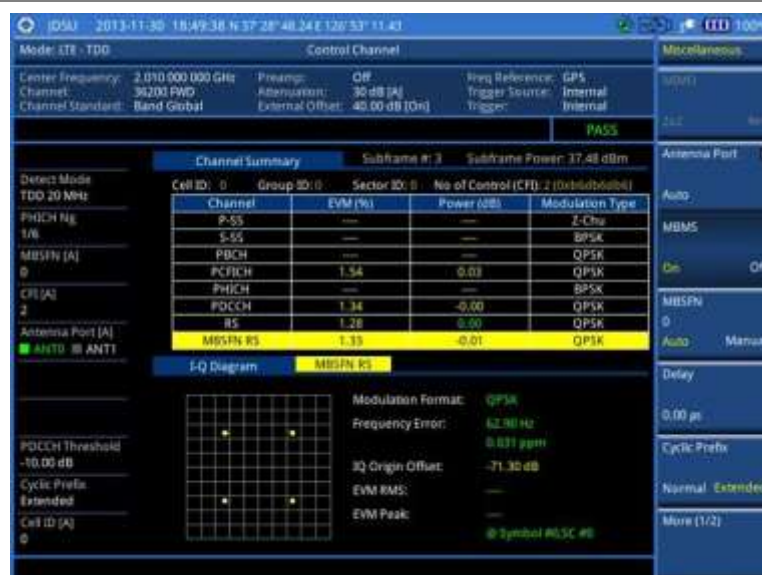
Figure 138 Control channel measurement with LTE-TDD signal analyzer (MBMS On)
