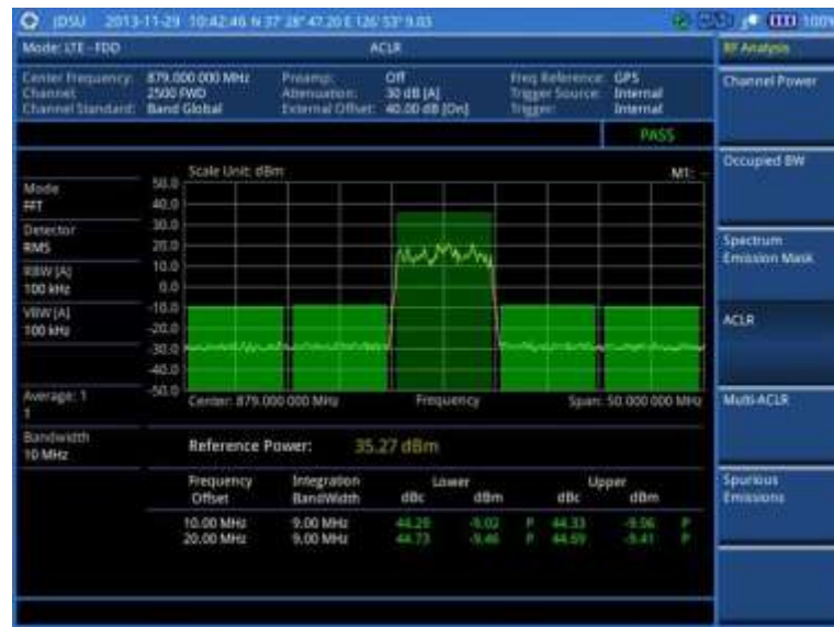
Figure 90 ACLR measurement with LTE-FDD signal analyzer
