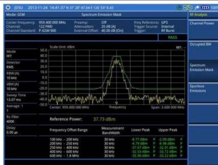
Figure 44 SEM measurement with GSM signal analyzer
