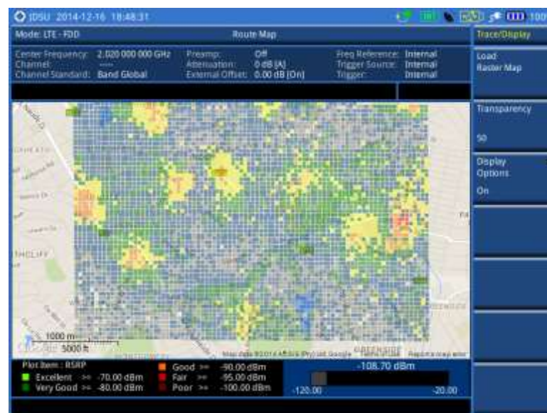
Figure 117 Raster image overlaid on the base map with LTE-FDD OTA signal analyzer
