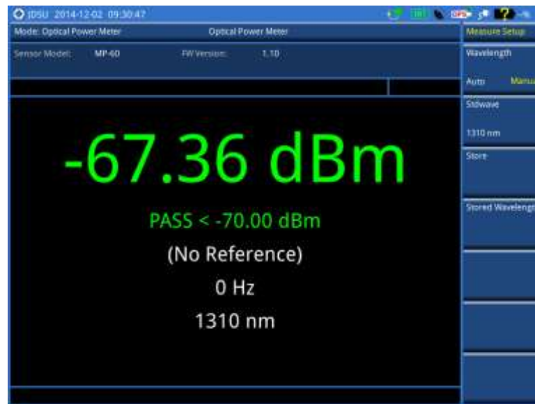
Figure 325 optical power measurement
