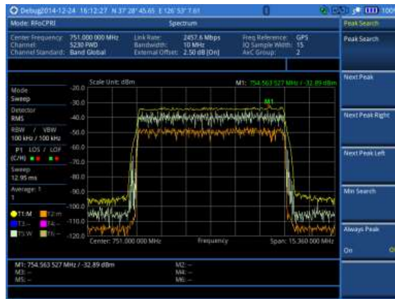
Figure 278 RFoCPRI spectrum analysis on LTE Uplink 10 MHz, antenna 2
