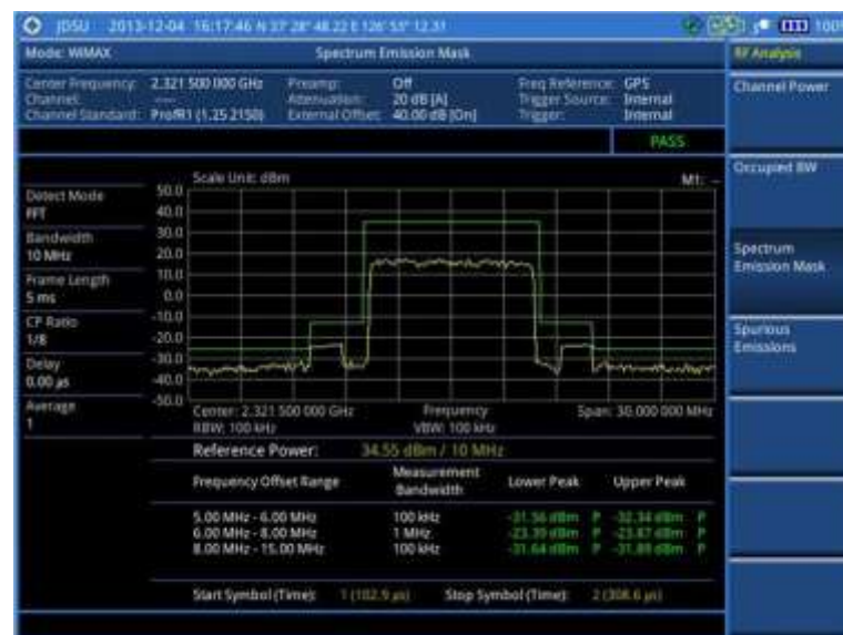
Figure 237 SEM measurement with Mobile WiMAX signal analyzer
