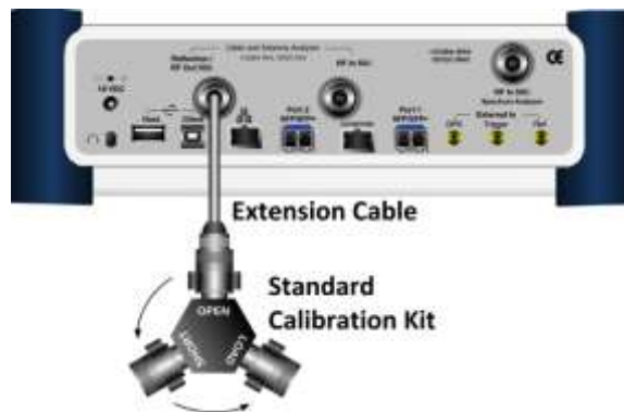
Figure 250 1-port calibration connection with mechanical Y-Cal kit
