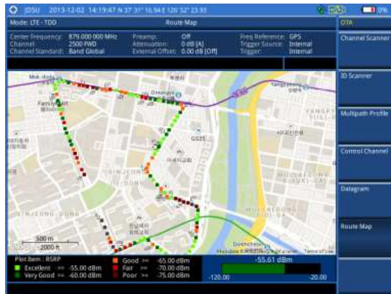
Figure 153 Route map measurement with LTE-TDD OTA signal analyzer
