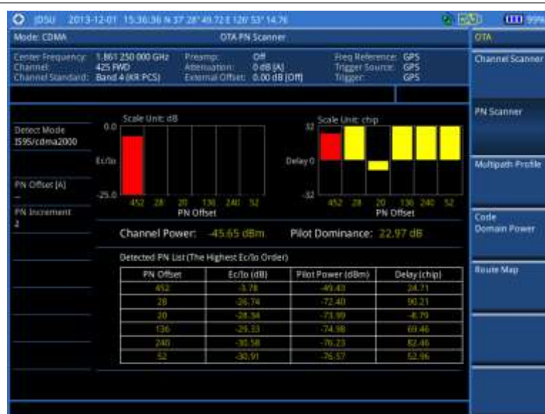
Figure 175 PN scanner measurement with CDMA OTA signal analyzer
