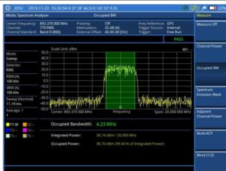
Figure 14 Occupied bandwidth measurement with spectrum analyzer
