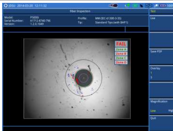
Figure 328 Analyzed fiber image and fiber inspection result
