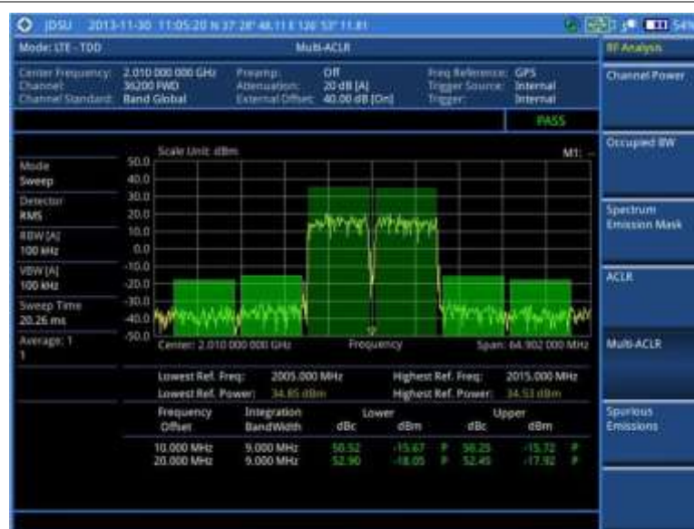
Figure 129 Multi-ACLR measurement with LTE-TDD signal analyzer
