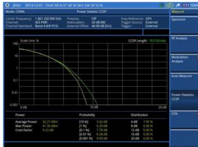
Figure 173 CCDF measurement with CDMA signal analyzer
