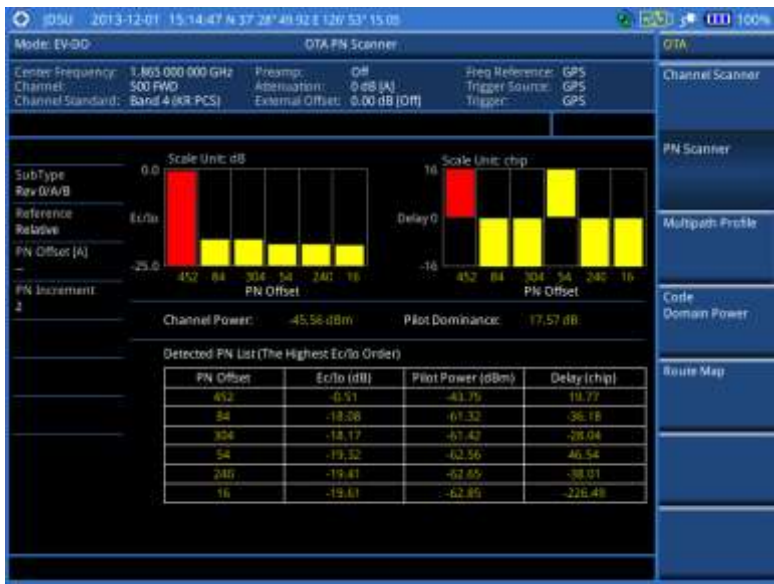
Figure 200 PN scanner measurement with EV-DO OTA signal analyzer
