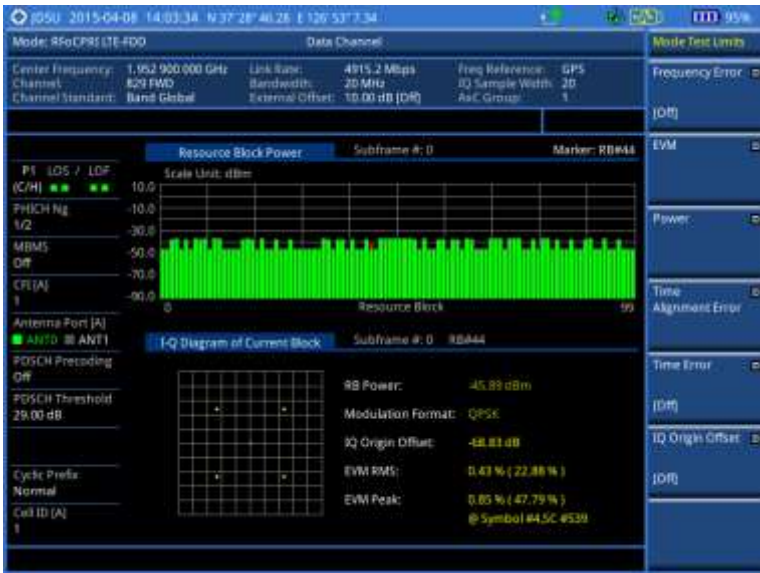
Figure 292 Data channel measurement with RFoCPRI TE-FDD signal analyzer
