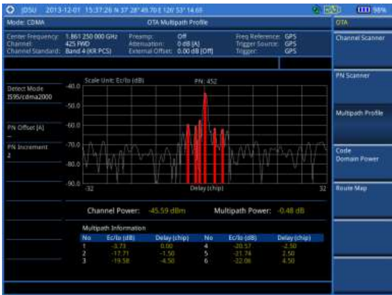
Figure 176 Multipath profile measurement with CDMA OTA signal analyzer
