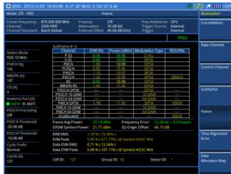
Figure 103 Frame measurement with LTE-FDD signal analyzer (MBMS On)
