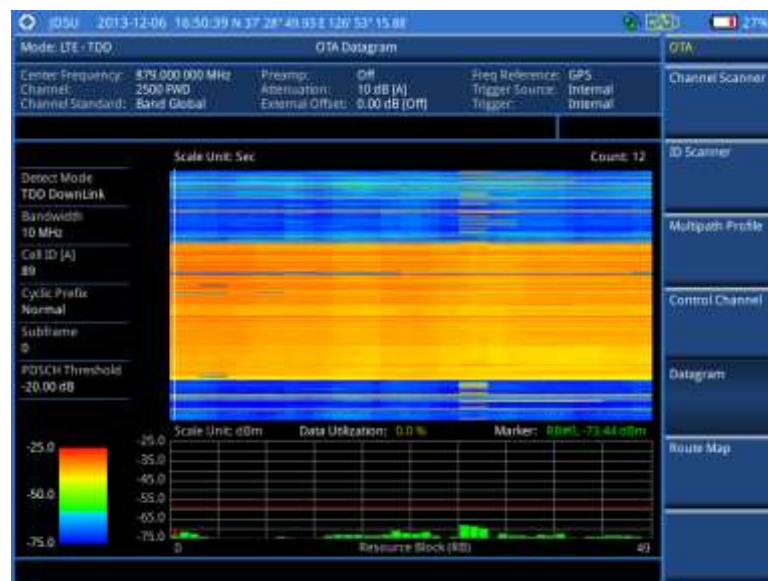
Figure 152 Datagram measurement with LTE-TDD signal analyzer
