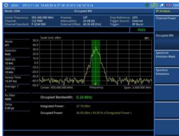
Figure 43 Occupied bandwidth measurement with GSM signal analyzer
