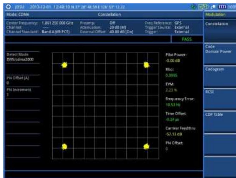
Figure 168 Constellation measurement with CDMA signal analyzer
