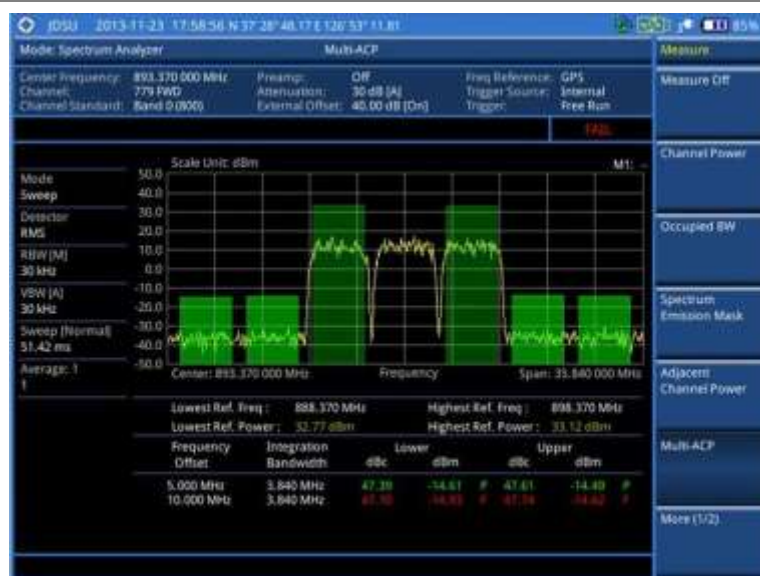
Figure 17 Multi-ACP measurement with spectrum analyzer
