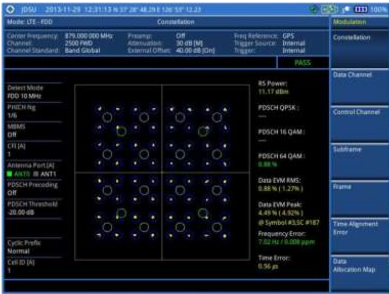
Figure 95 Constellation measurement with LTE-FDD signal analyzer (MBMS On)
