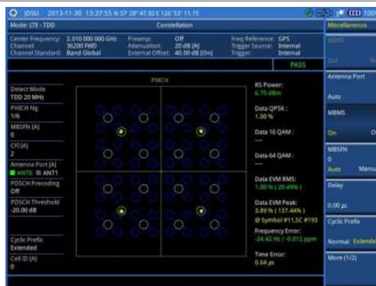
Figure 134 Constellation measurement with LTE-TDD signal analyzer (MBMS On)
