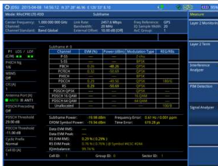
Figure 294 Subframe measurement (regular view) with RFoCPRI LTE-FDD signal analyzer
