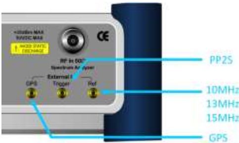
Figure 85 Connection ports for external reference clock
