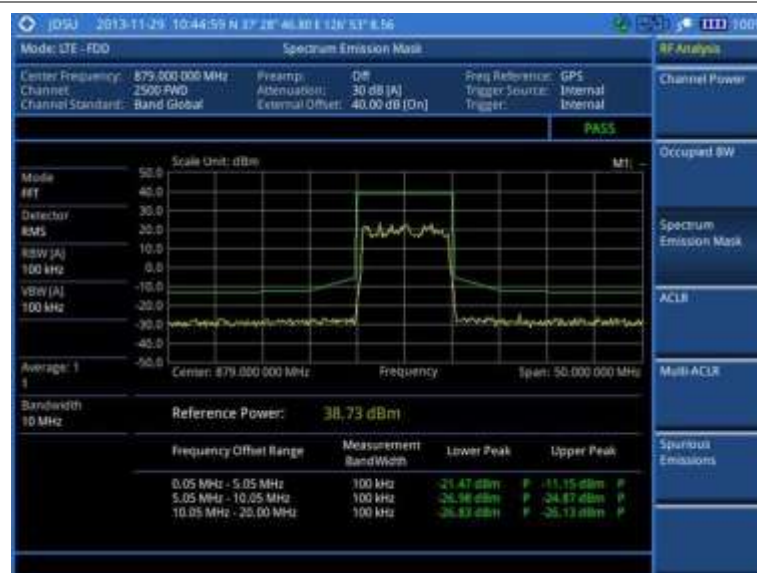
Figure 89 SEM measurement with LTE-FDD signal analyzer
