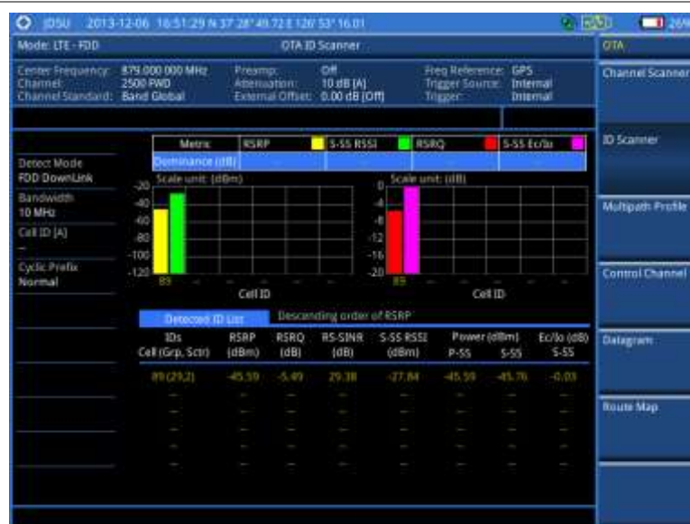
Figure 112 ID scanner measurement with LTE-FDD OTA signal analyzer
