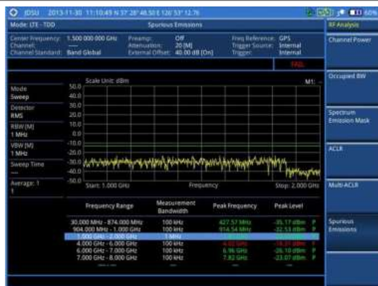
Figure 130 Spurious emissions measurement with LTE-TDD signal analyzer
