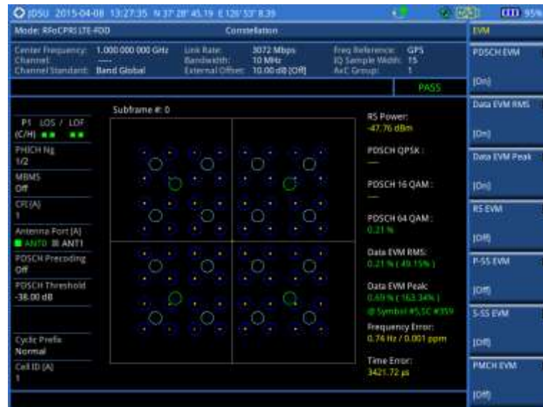
Figure 291 Constellation measurement with RFoCPRI LTE-FDD signal analyzer
