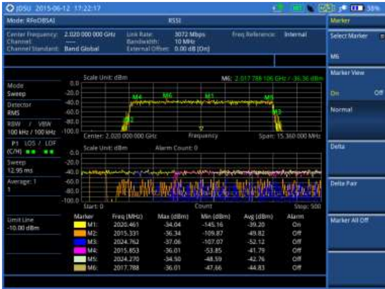
Figure 307 RFoBSAI interference measurement in RSSI
