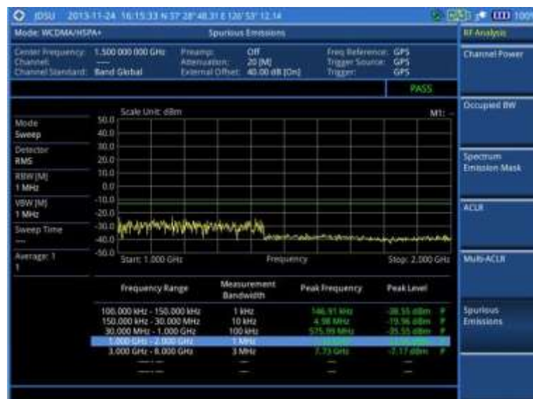
Figure 67 Spurious emissions measurement with WCDMA/HSPA+ signal analyzer
