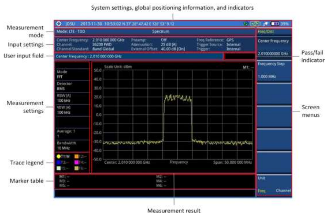
Figure 119 LTE-TDD signal analyzer measurement screen
