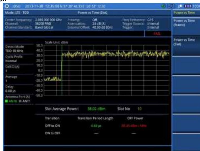
Figure 131 Power vs. time (slot) measurement with LTE – TDD signal analyzer
