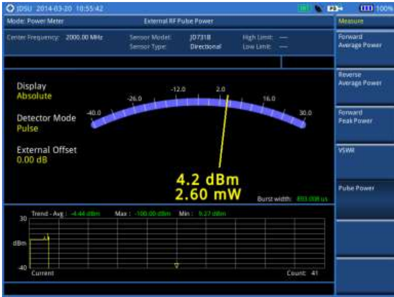
Figure 323 External power measurement of pulse power
