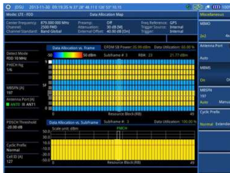
Figure 106 Data allocation map measurement with LTE-FDD signal analyzer (MBMS On)
