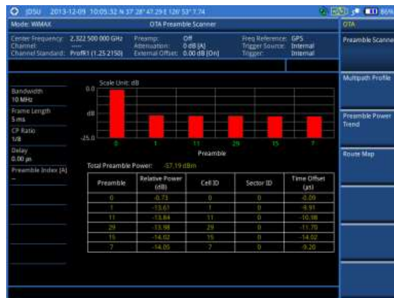
Figure 245 Preamble scanner measurement with Mobile WiMAX OTA signal analyzer
