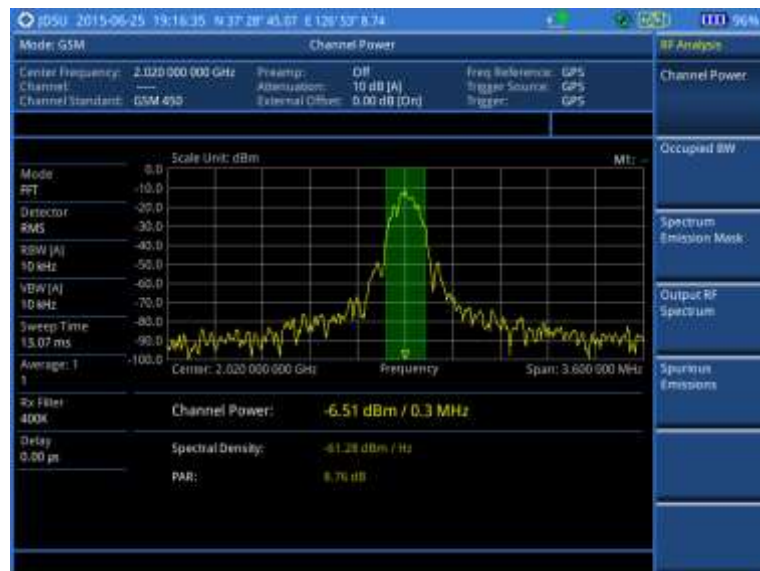
Figure 42 Channel power measurement with GSM signal analyzer
