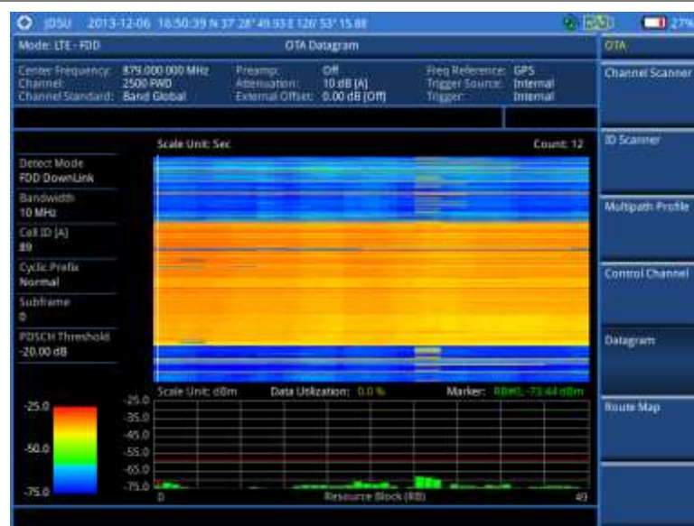
Figure 115 Datagram measurement with LTE-FDD signal analyzer
