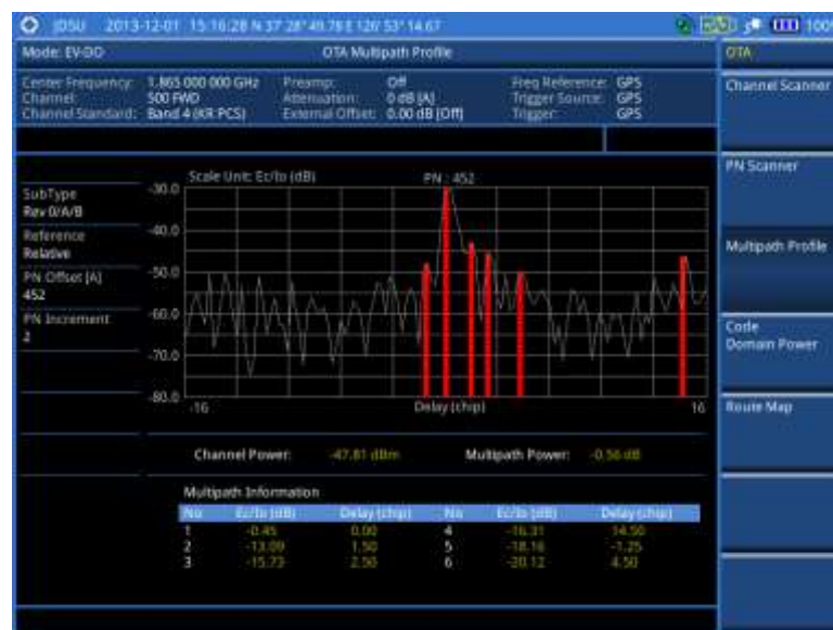
Figure 201 Multipath profile measurement with EV-DO OTA signal analyzer
