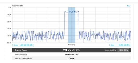
Channel power measurement result shows channel power and spectrum density in a user specified channel bandwidth. The peak to average ratio (PAR) is shown at the bottom of the screen as well. The shaded area on the display indicates the channel bandwidth.
