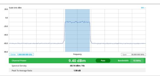
Channel power measurement result shows channel power and spectrum density in a user specified channel bandwidth. The peak to average ratio (PAR) is shown at the bottom of the screen as well. The shaded area on the display indicates the channel bandwidth.
