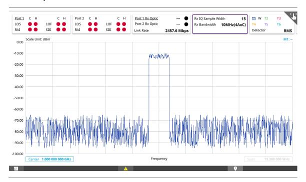
RFoCPRI spectrum measurement (Quad)
