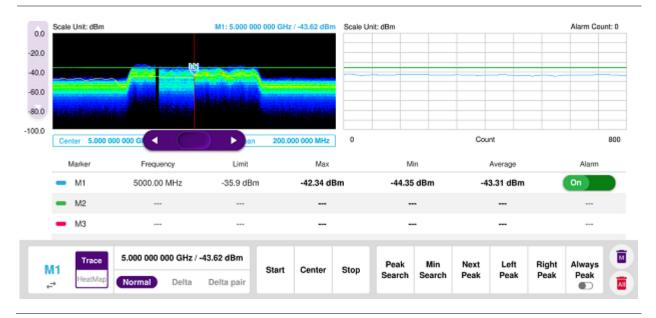
You can go to Menu > Limit to analyze your measurements with the display line, multi-segment line, and channel limit. See "<u>Setting limit</u>" for more details. Once you tap the vertical move bar and move it up and down, the reference line value changes.
