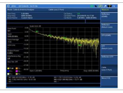
Figure 307 Cable loss (1 port) measurement with zoom
