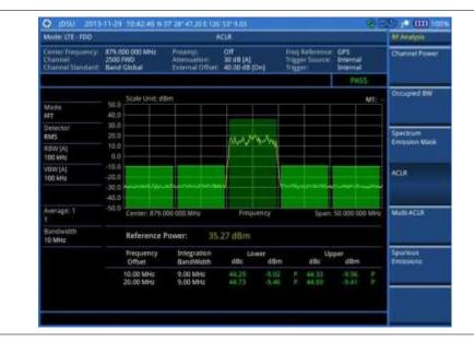
Figure 110 ACLR measurement with LTE - FDD signal analyzer
