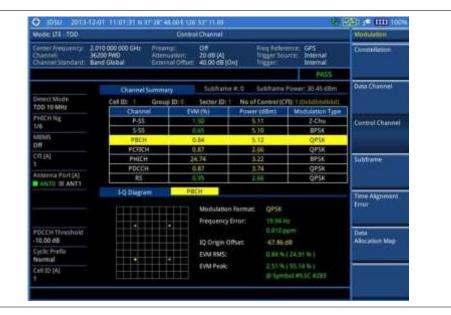
Figure 162 Control channel measurement with LTE - TDD signal analyzer (MBMS On)
