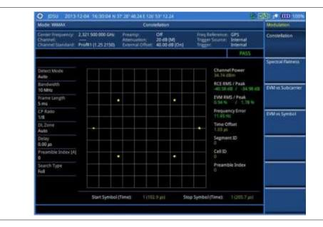
Figure 265 Constellation measurement with Mobile WiMAX signal analyzer
