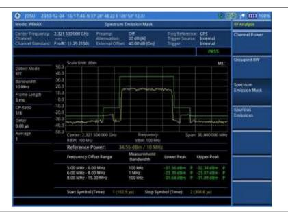
Figure 262 SEM measurement with Mobile WiMAX signal analyzer
