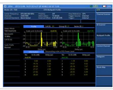
Figure 175 Multipath profile measurement with LTE - TDD OTA signal analyzer
