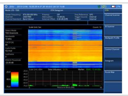
Figure 177 Datagram measurement with LTE - TDD signal analyzer
