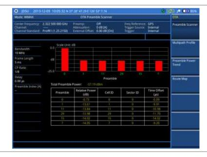
Figure 270 Preamble scanner measurement with Mobile WiMAX OTA signal analyzer
