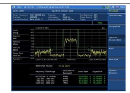
Figure 189 SEM measurement with CDMA signal analyzer
