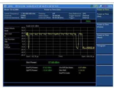
Figure 241 Power vs. time (slot) measurement with TD-SCDMA signal analyzer
