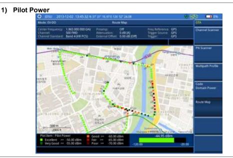
Figure 228 Route map measurement with EV-DO OTA signal analyzer
