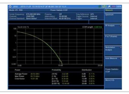
Figure 130 CCDF measurement with LTE - FDD signal analyzer
