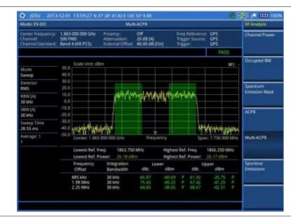
Figure 214 Multi-ACPR measurement with EV-DO signal analyzer
