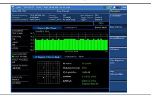
Figure 159 Data channel measurement with LTE - TDD signal analyzer
