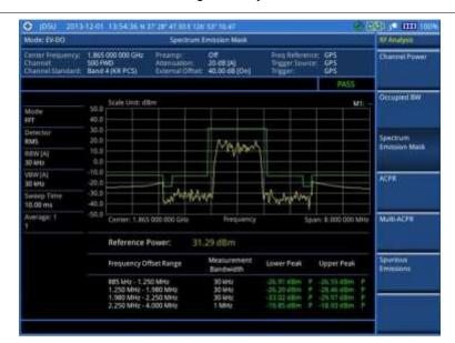
Figure 212 SEM measurement with EV-DO signal analyzer
