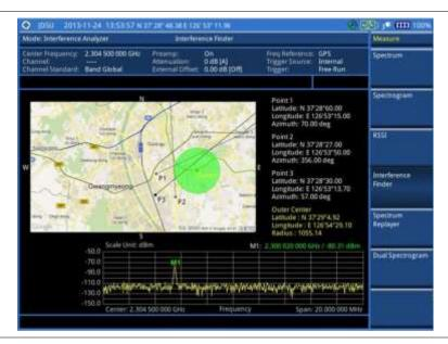
Figure 51 Interference finder measurement in map view
