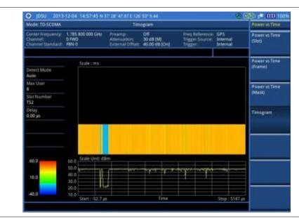
Figure 244 Timogram with TD-SCDMA signal analyzer
