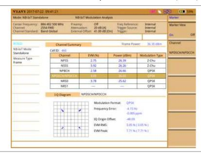
Figure 289 NB-IoT Standalone Modualtion Analysis measurement screen (Subframe 0- NPBCH)
