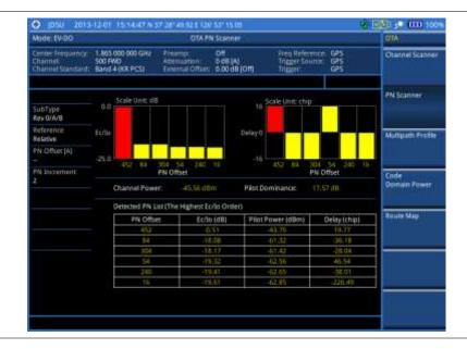
Figure 225 PN scanner measurement with EV-DO OTA signal analyzer
