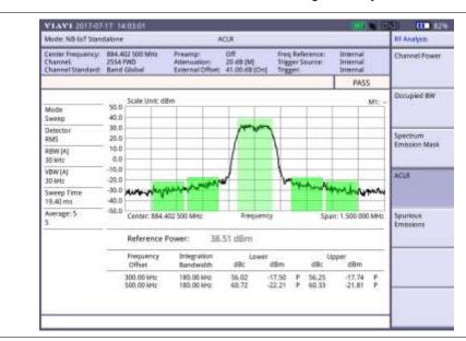
Figure 286 ACLR measurement with NB-IoT Standalond signal analyzer
