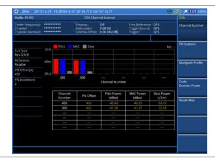
Figure 224 Channel scanner measurement with EV-DO OTA signal analyzer
