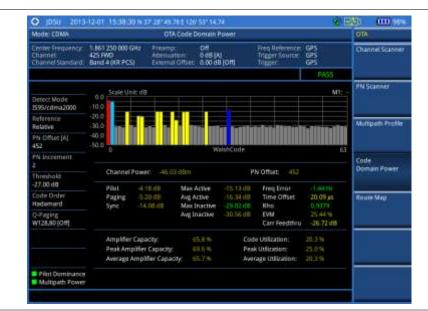
Figure 202 Code domain power measurement with CDMA OTA signal analyzer
