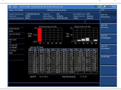
Figure 249 Sync-DL ID scanner measurement with TD-SCDMA OTA signal analyzer
