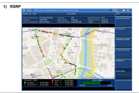
Figure 178 Route map measurement with LTE - TDD OTA signal analyzer
