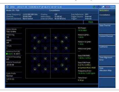
Figure 158 Constellation measurement with LTE - TDD signal analyzer (MBMS On)
