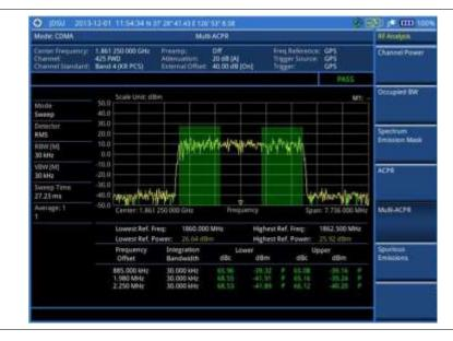
Figure 191 Multi-ACPR measurement with CDMA signal analyzer
