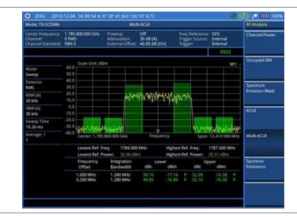
Figure 239 Multi-ACLR measurement with TD-SCDMA signal analyzer
