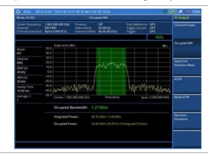
Figure 211 Occupied bandwidth measurement with EV-DO signal analyzer
