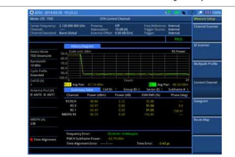
Figure 176 Control channel measurement with LTE - TDD OTA signal analyzer
