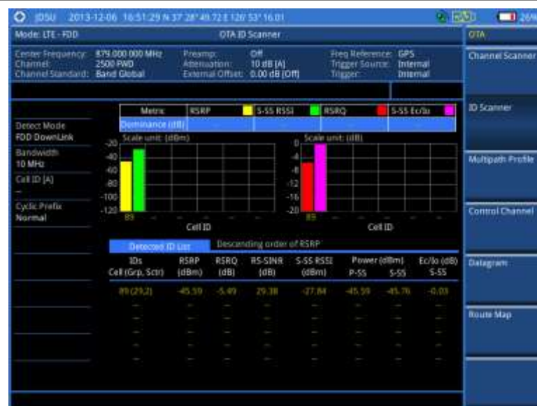
Figure 132 ID scanner measurement with LTE - FDD OTA signal analyzer
