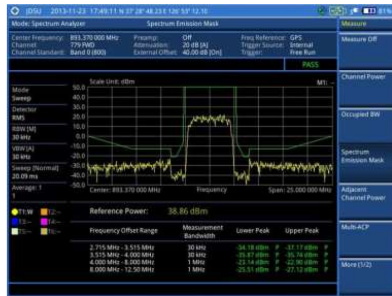
Figure 21 Spectrum emission mask measurement with spectrum analyzer (on 28 GHz downconverter)
