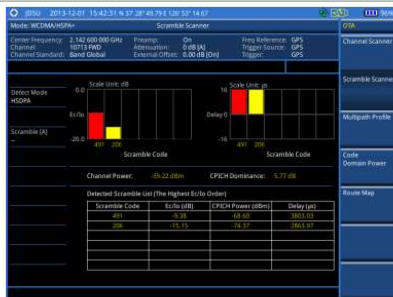
Figure 94 Scramble scanner measurement with WCDMA/HSPA+ OTA signal analyzer
