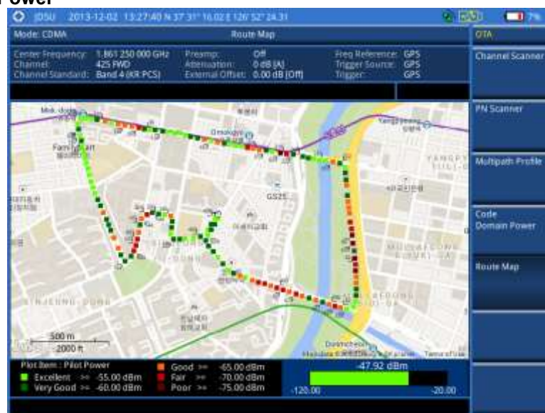
Figure 200 Route map measurement with CDMA OTA signal analyzer
