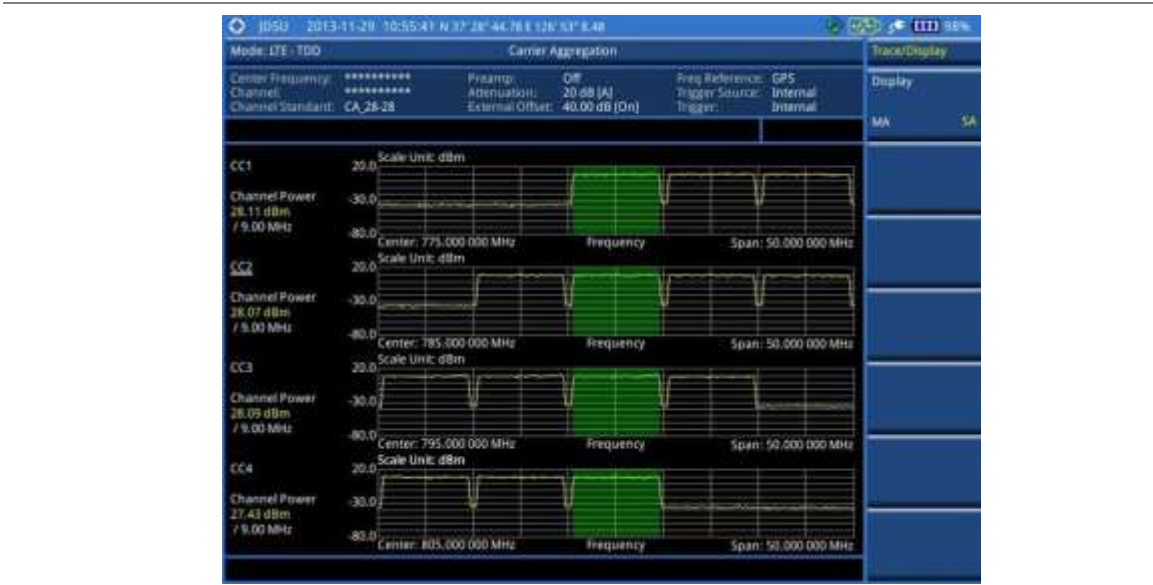
Figure 169 Carrier aggregation measurement with LTE - TDD signal analyzer (SA)
