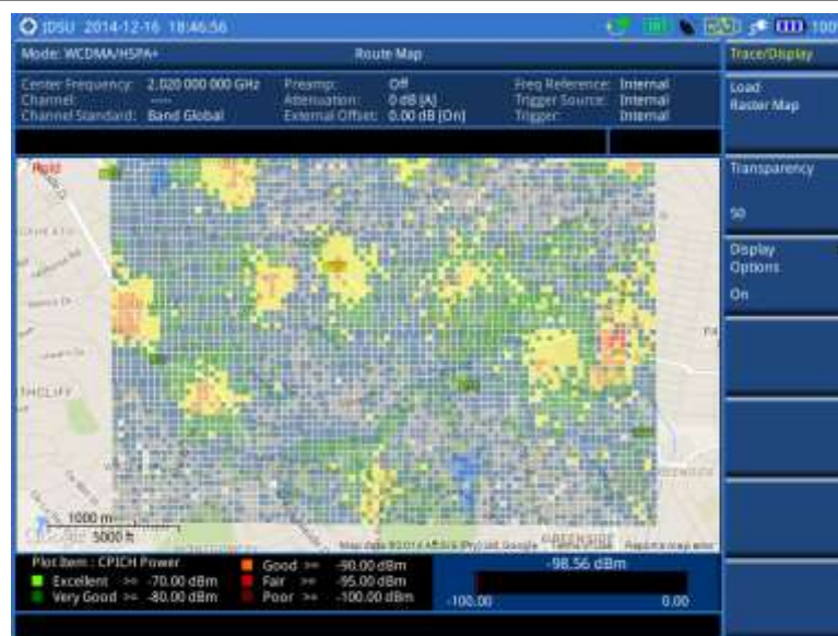
Figure 98 Raster image overlaid on the route map in WCDMA/HSPA+ OTA signal analyzer
