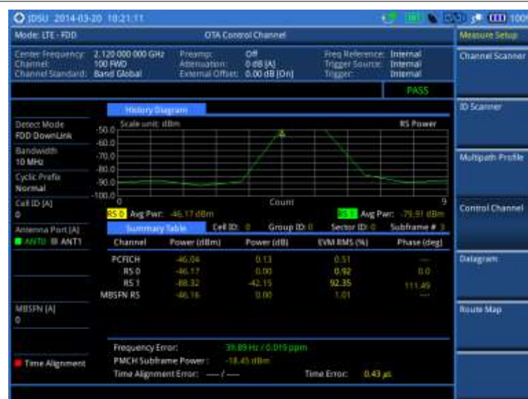
Figure 134 Control channel measurement with LTE - FDD OTA signal analyzer
