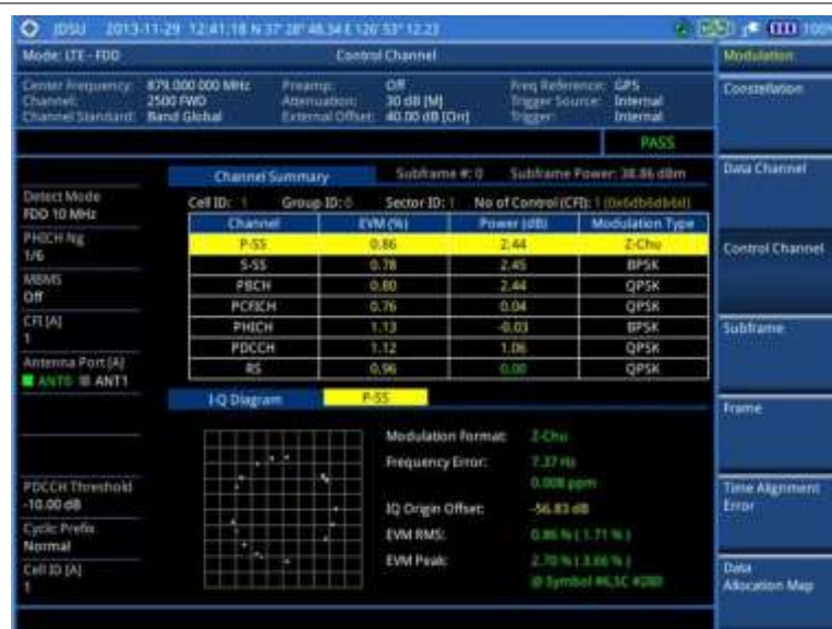
Figure 117 Control channel measurement with LTE - FDD signal analyzer
