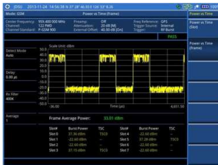
Figure 68 Power vs. time (frame) measurement with GSM signal analyzer
