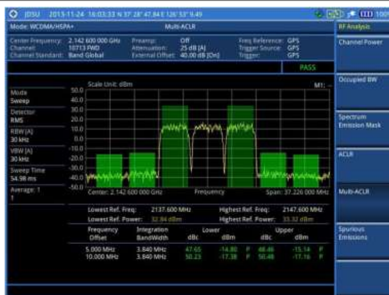
Figure 84 Multi-ACLR measurement with WCDMA/HSPA+ signal analyzer
