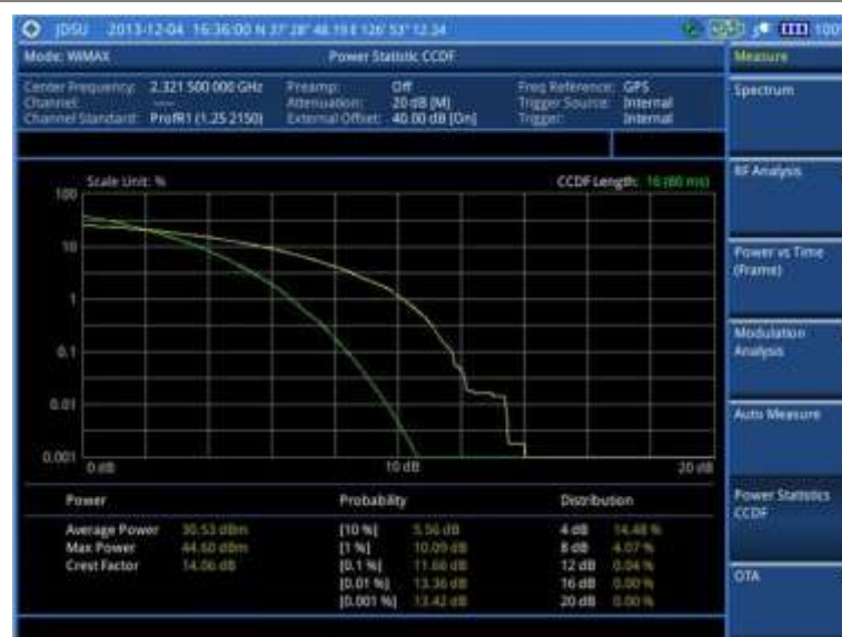
Figure 266 CCDF measurement with Mobile WiMAX signal analyzer
