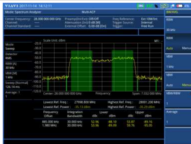
Figure 25 Multi-ACP measurement with spectrum analyzer (on 28 GHz downconverter)
