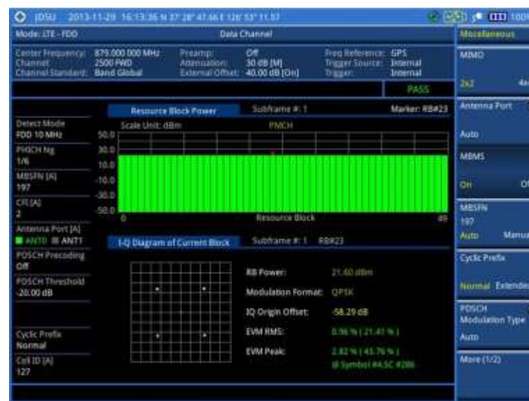
Figure 115 Data channel measurement with LTE - FDD signal analyzer (MBMS On)
