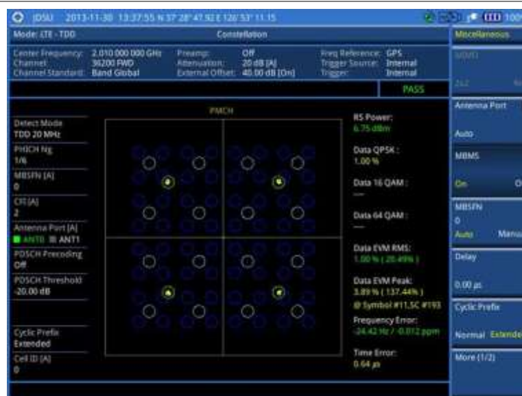
Figure 156 Constellation measurement with LTE - TDD signal analyzer (MBMS On)
