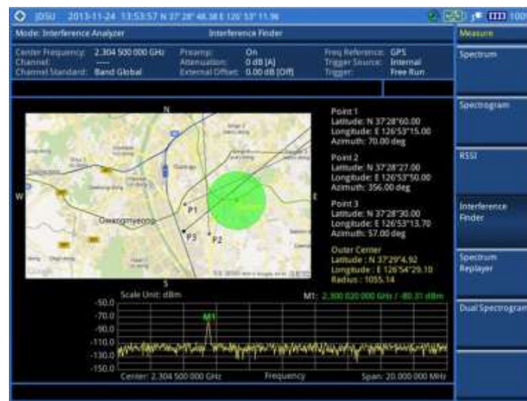
Figure 50 Interference finder measurement in map view (on 28 GHz downconverter)
