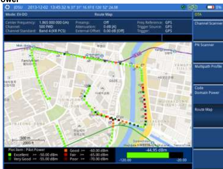
Figure 225 Route map measurement with EV-DO OTA signal analyzer
