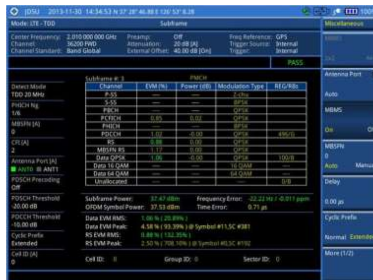
Figure 162 Subframe measurement with LTE - TDD signal analyzer (MBMS On)
