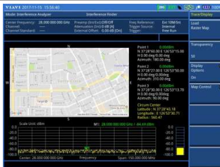
Figure 52 Raster image overlaid on the map in interference finder (on 28 GHz downconverter)
