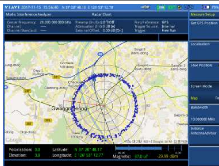
Figure 54 RSSI data plotted on the radar chart (on 28 GHz downconverter)
