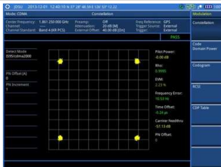
Figure 190 Constellation measurement with CDMA signal analyzer
