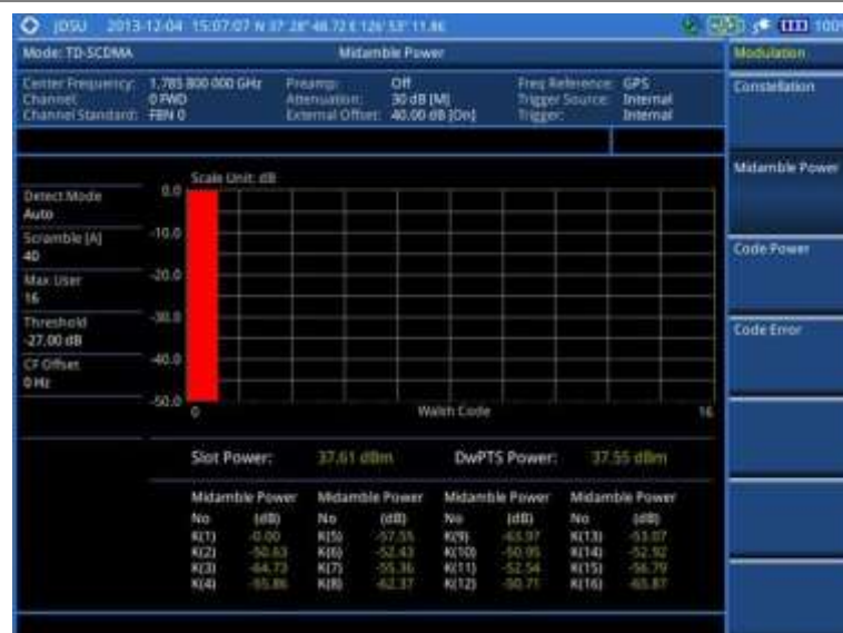
Figure 243 Midamble measurement with TD-SCDMA signal analyzer
