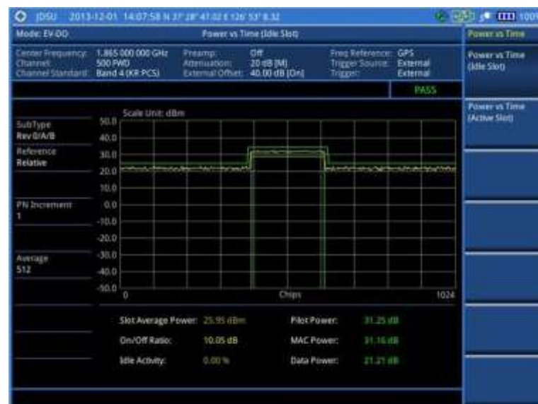
Figure 213 Power vs. time (idle slot) measurement with EV-DO signal analyzer
