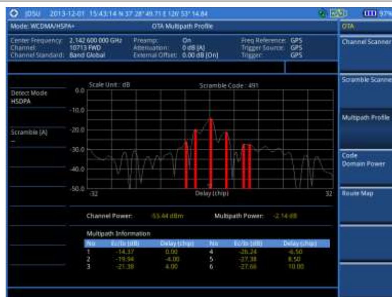
Figure 95 Multipath profile measurement with WCDMA/HSPA+ OTA signal analyzer
