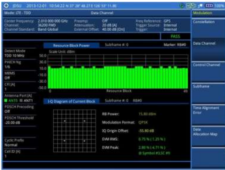
Figure 158 Data channel measurement with LTE - TDD signal analyzer (MBMS On)
