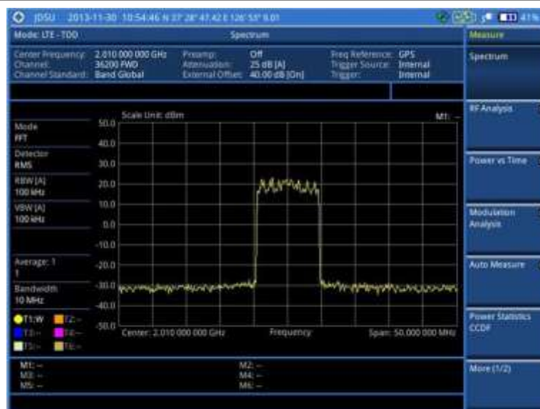
Figure 146 Spectrum measurement screen with LTE - TDD signal analyzer
