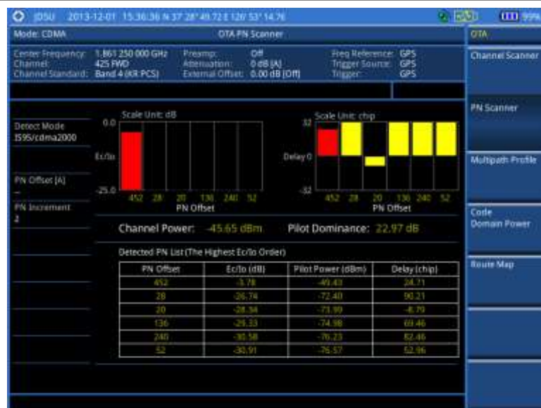
Figure 197 PN scanner measurement with CDMA OTA signal analyzer
