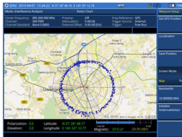
Figure 53 RSSI data plotted on the radar chart
