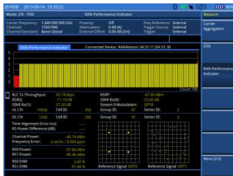
Figure 177 RAN performance indicator in LTE-TDD signal analyzer
