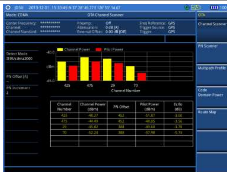
Figure 196 Channel scanner measurement with CDMA OTA signal analyzer
