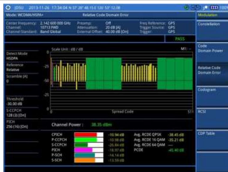
Figure 88 Relative code domain error with WCDMA/HSPA+ signal analyzer
