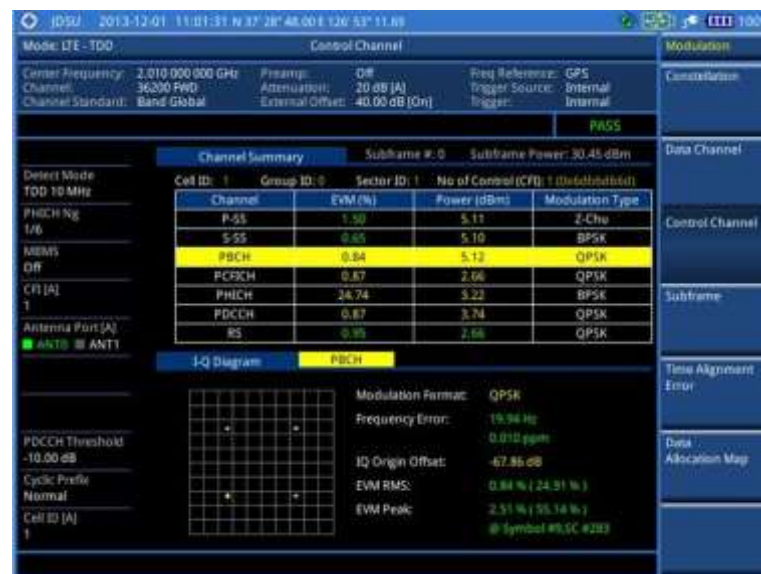
Figure 160 Control channel measurement with LTE - TDD signal analyzer (MBMS On)
