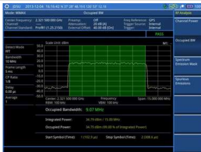
Figure 258 Occupied bandwidth measurement with Mobile WiMAX signal analyzer
