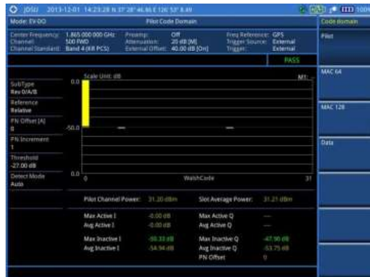
Figure 216 Code domain power measurement with EV-DO signal analyzer
