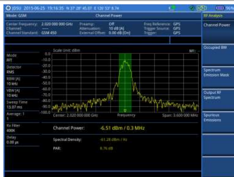
Figure 62 Channel power measurement with GSM signal analyzer
