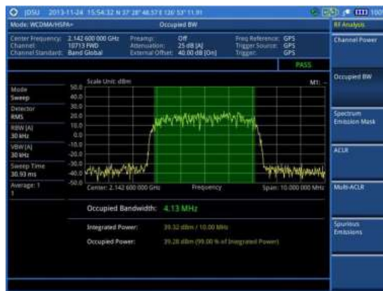
Figure 81 Occupied bandwidth measurement with WCDMA/HSPA+ signal analyzer
