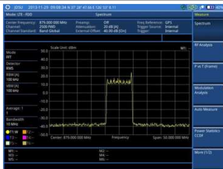
Figure 104 Spectrum measurement screen with LTE - FDD signal analyzer
