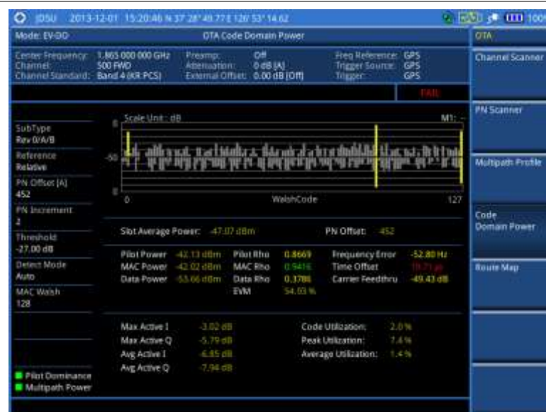
Figure 224 Code domain power measurement with EV-DO OTA signal analyzer
