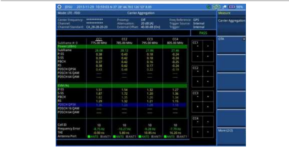
Figure 130 Carrier aggregation measurement with LTE - FDD signal analyzer (SA)
