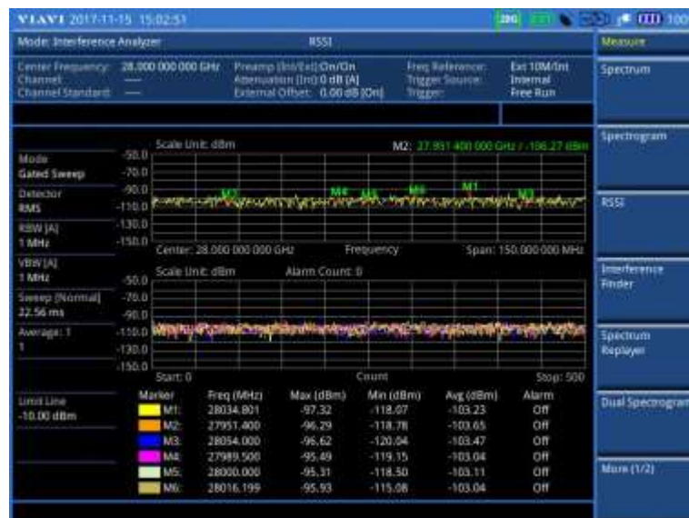
Figure 48 Interference measurement in RSSI (on 28 GHz downconverter)
