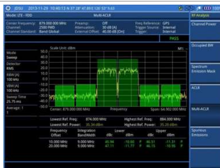
Figure 109 Multi-ACLR measurement with LTE - FDD signal analyzer
