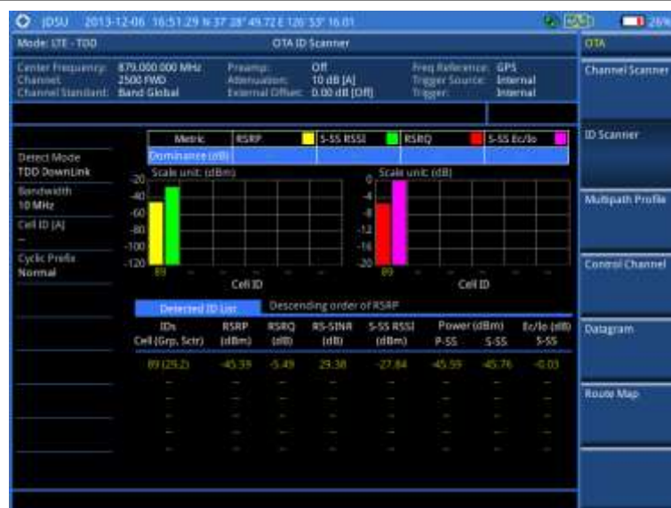
Figure 171 ID scanner measurement with LTE - TDD OTA signal analyzer
