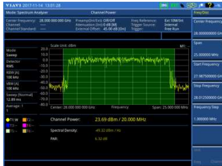
Figure 16 Channel power measurement with spectrum analyzer (on 28 GHz downconverter)
