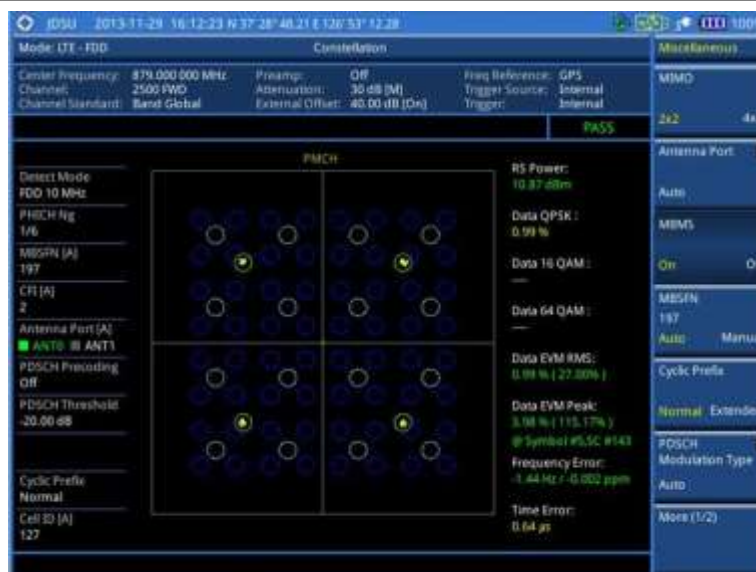
Figure 113 Constellation measurement with LTE - FDD signal analyzer (MBMS On)
