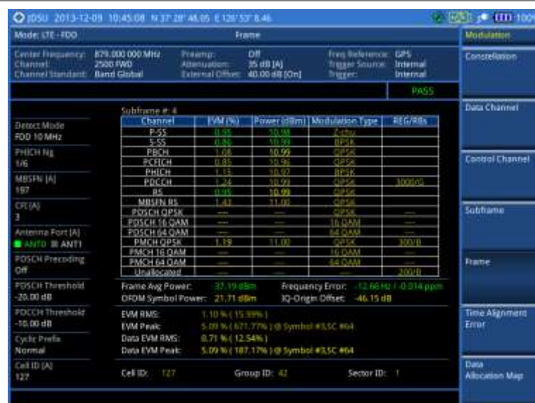
Figure 122 Frame measurement with LTE - FDD signal analyzer (MBMS On)
