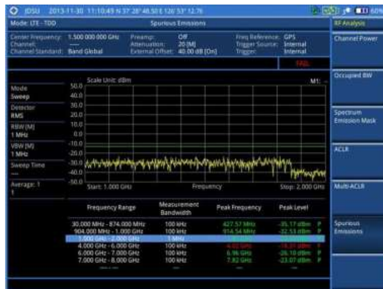
Figure 152 Spurious emissions measurement with LTE - TDD signal analyzer
