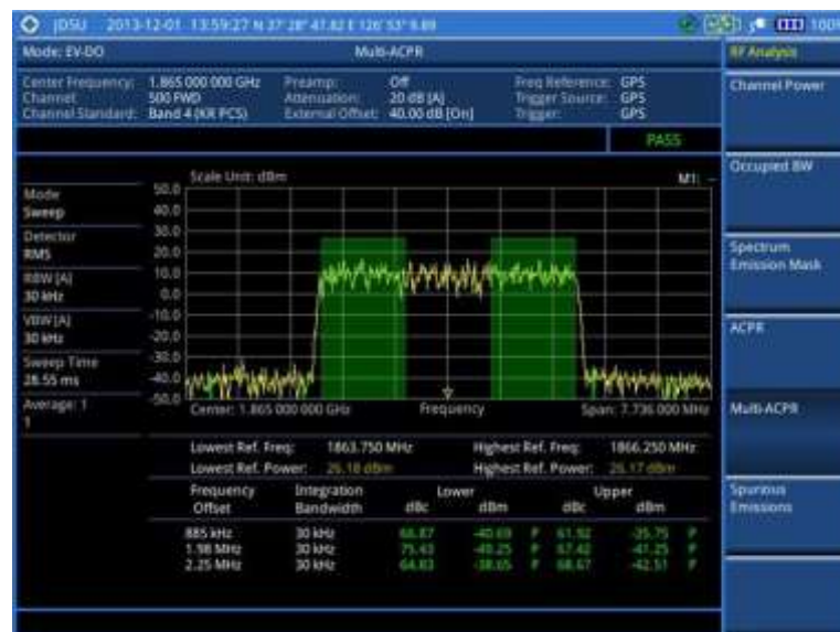
Figure 211 Multi-ACPR measurement with EV-DO signal analyzer
