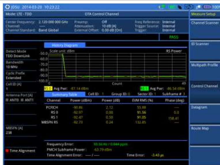
Figure 173 Control channel measurement with LTE - TDD OTA signal analyzer
