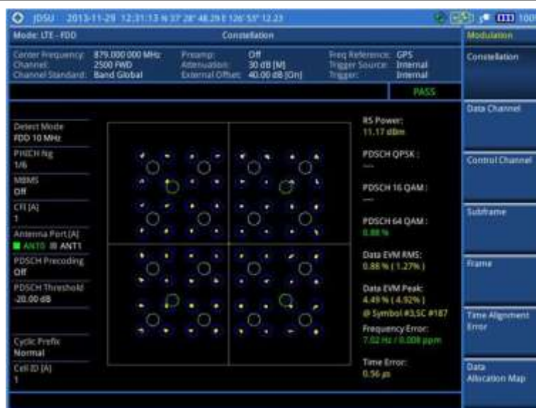
Figure 113 Constellation measurement with LTE - FDD signal analyzer (MBMS On)
