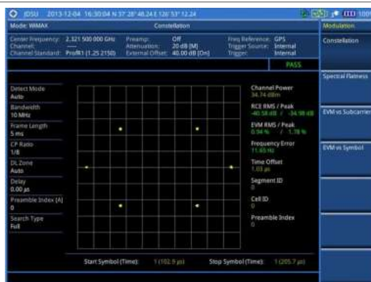
Figure 262 Constellation measurement with Mobile WiMAX signal analyzer
