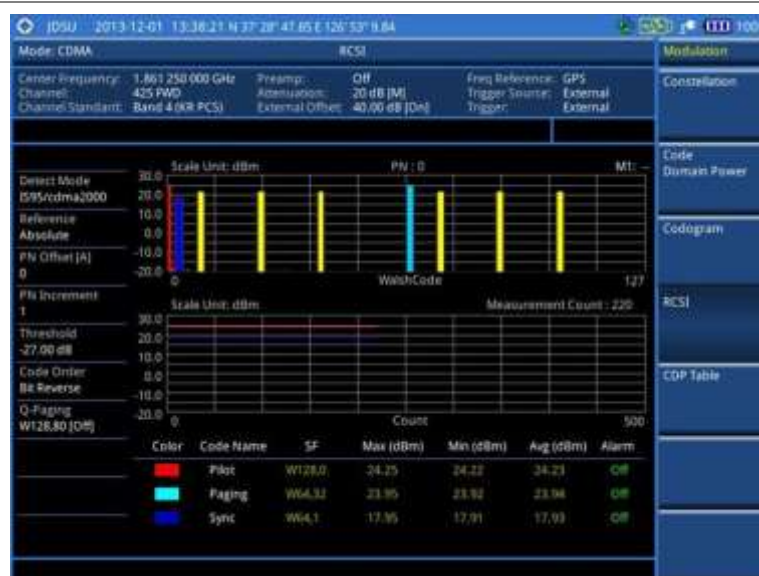
Figure 193 RCSI measurement with CDMA signal analyzer
