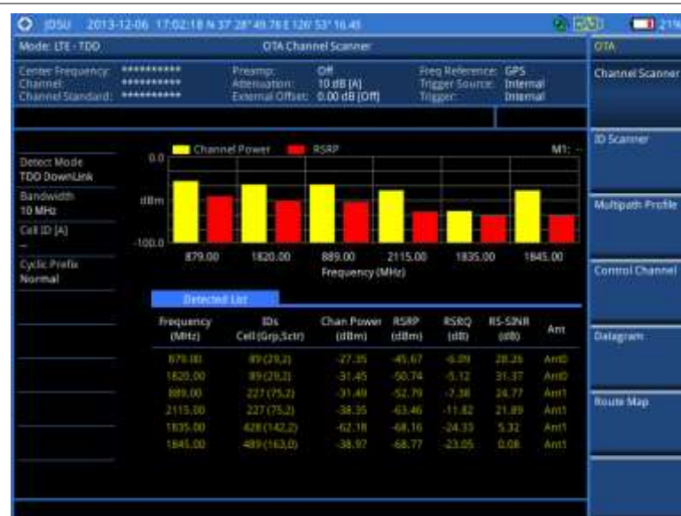
Figure 170 Channel scanner measurement with LTE - TDD OTA signal analyzer
