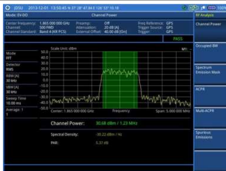
Figure 207 Channel power measurement with EV-DO signal analyzer
