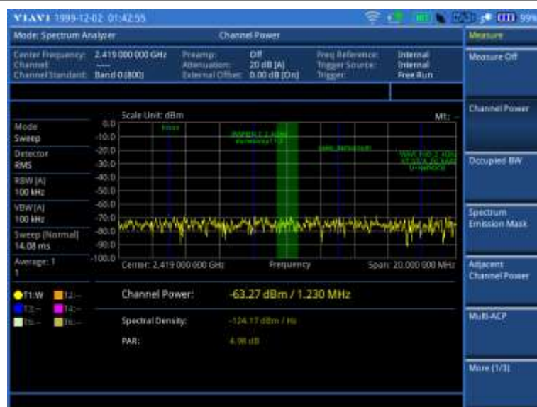
Figure 17 Wi-Fi SSID display in channel power measurement with spectrum analyzer
