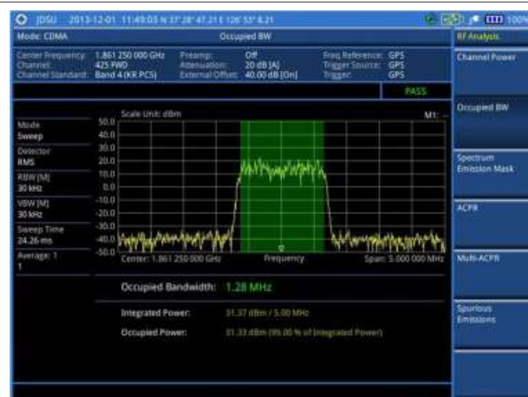
Figure 185 Occupied bandwidth measurement with CDMA signal analyzer
