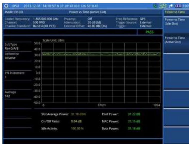
Figure 214 Power vs. time (active slot) measurement with EV-DO signal analyzer
