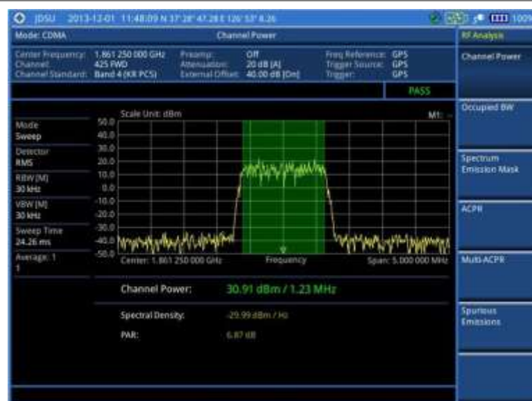
Figure 184 Channel power measurement with CDMA signal analyzer
