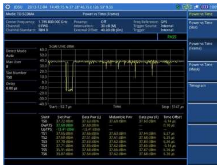
Figure 239 Power vs. time (frame) measurement with TD-SCDMA signal analyzer
