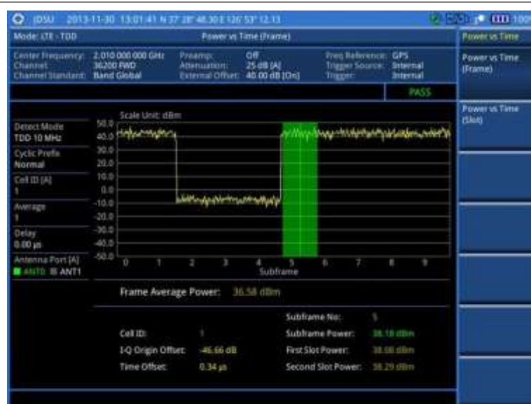
Figure 154 Power vs. time (frame) measurement with LTE – TDD signal analyzer
