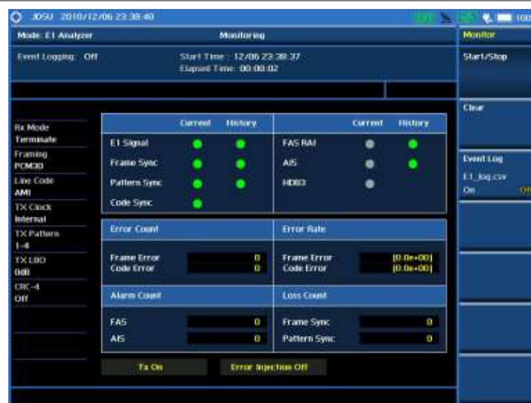
Figure 313 E1 transmission monitoring for framing PCM30
