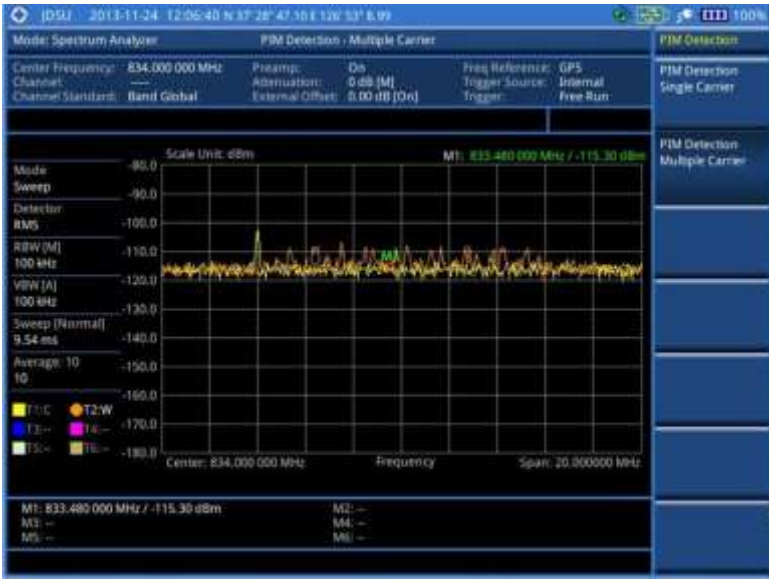
Figure 36 PIM detection for multiple carriers
