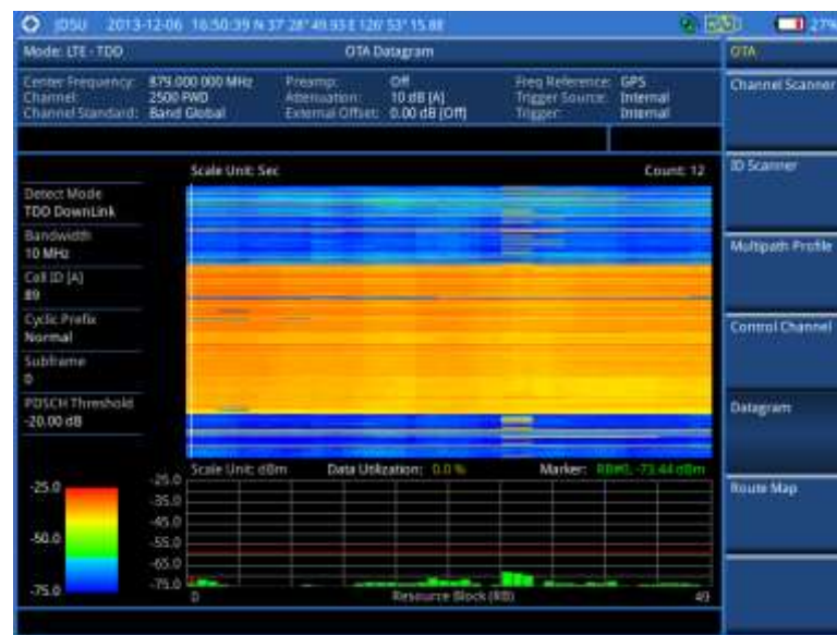
Figure 174 Datagram measurement with LTE - TDD signal analyzer
