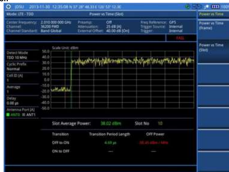
Figure 153 Power vs. time (slot) measurement with LTE – TDD signal analyzer
