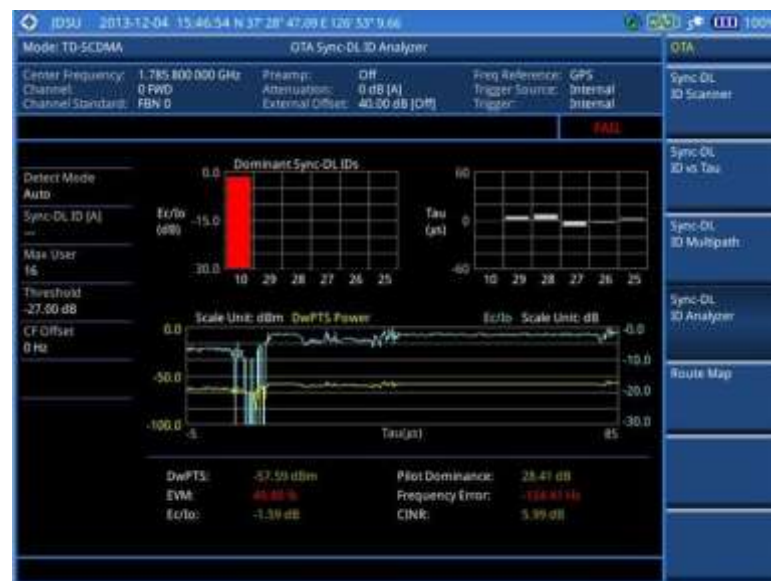
Figure 249 Sync-DL ID analyzer measurement with TD-SCDMA OTA signal analyzer
