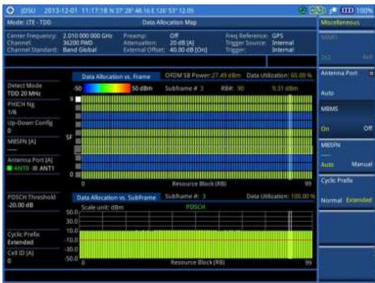
Figure 165 Data allocation map measurement with LTE - TDD signal analyzer (MBMS On)
