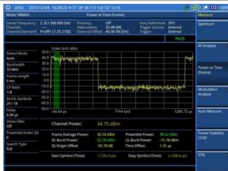
Figure 261 Power vs. time (frame) measurement with Mobile WiMAX signal analyzer
