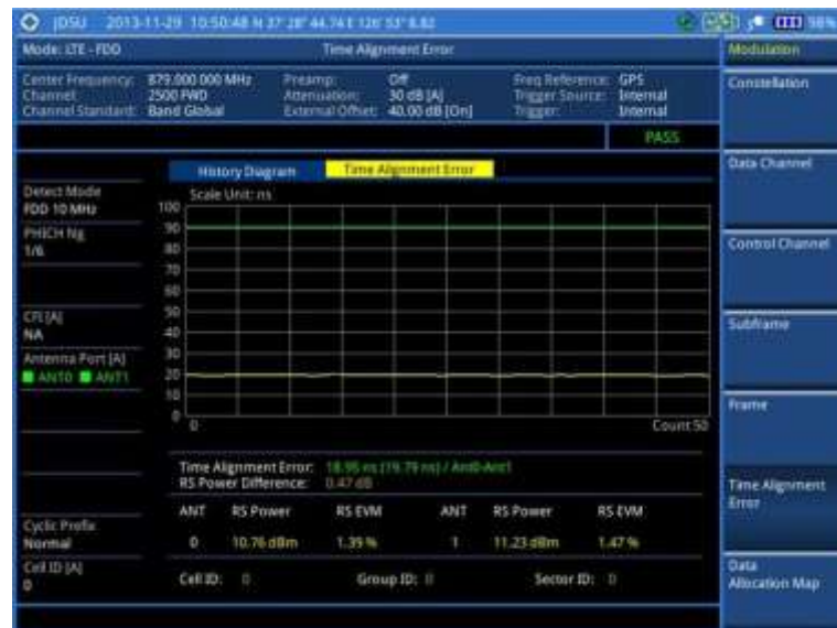
Figure 123 Time alignment error measurement with LTE - FDD signal analyzer
