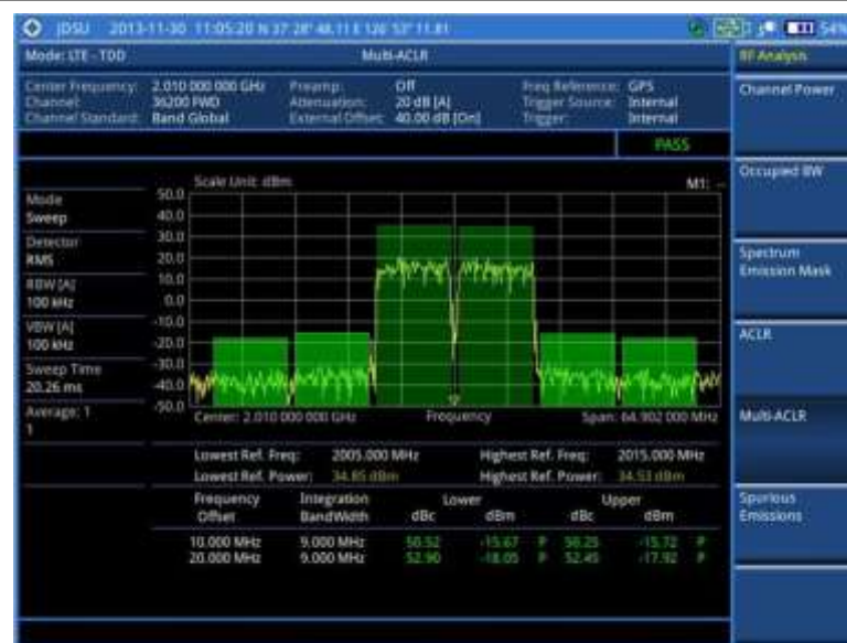
Figure 151 Multi-ACLR measurement with LTE - TDD signal analyzer
