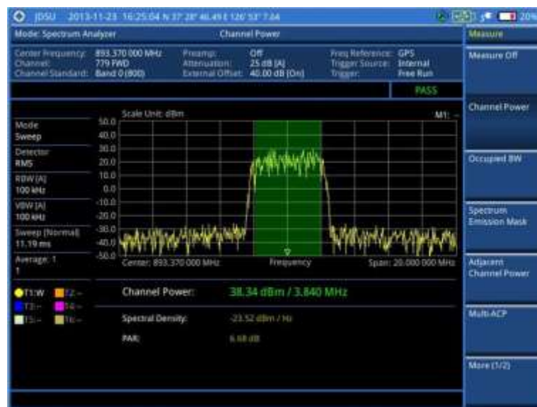
Figure 15 Channel power measurement with spectrum analyzer
