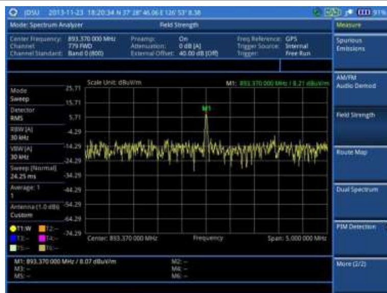
Figure 31 Field strength measurement with spectrum analyzer (on 28 GHz downconverter)
