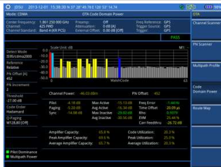
Figure 199 Code domain power measurement with CDMA OTA signal analyzer
