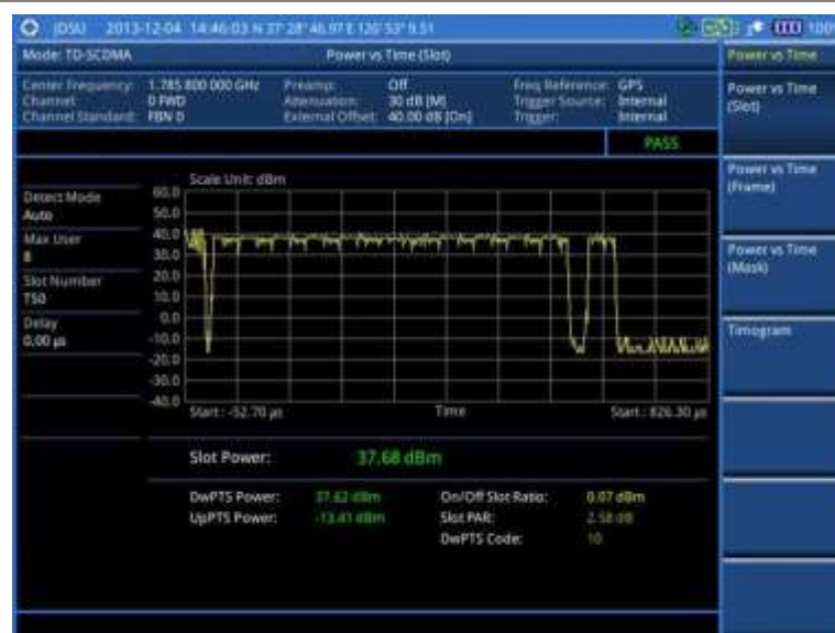
Figure 238 Power vs. time (slot) measurement with TD-SCDMA signal analyzer
