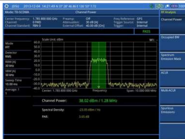
Figure 232 Channel power measurement with TD-SCDMA signal analyzer
