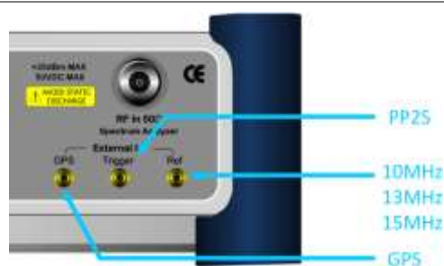
Figure 78 Connection ports for external reference clock
