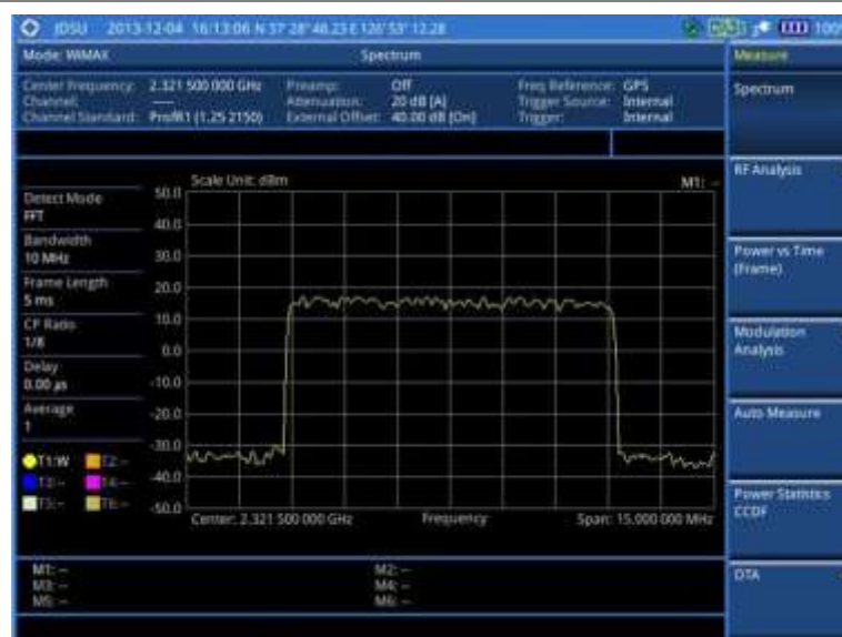
Figure 256 Spectrum measurement screen with Mobile WiMAX signal analyzer
