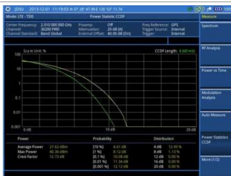
Figure 167 CCDF measurement with LTE - TDD signal analyzer
