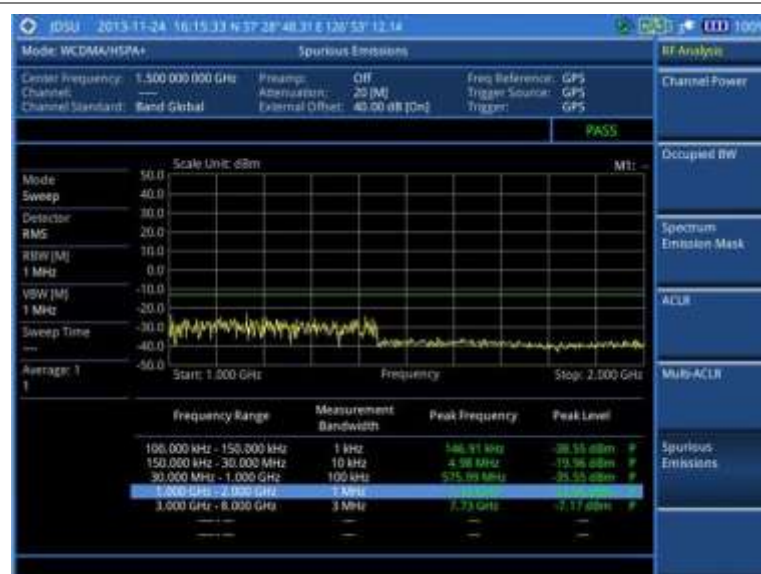
Figure 85 Spurious emissions measurement with WCDMA/HSPA+ signal analyzer
