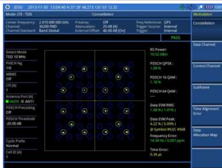
Figure 156 Constellation measurement with LTE - TDD signal analyzer (MBMS On)
