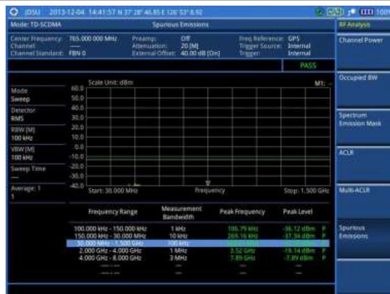
Figure 237 Spurious emissions measurement with TD-SCDMA signal analyzer
