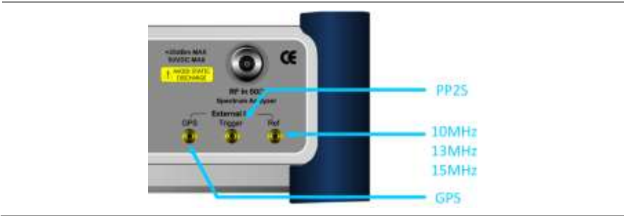
Figure 182 Connection ports for external reference clock
