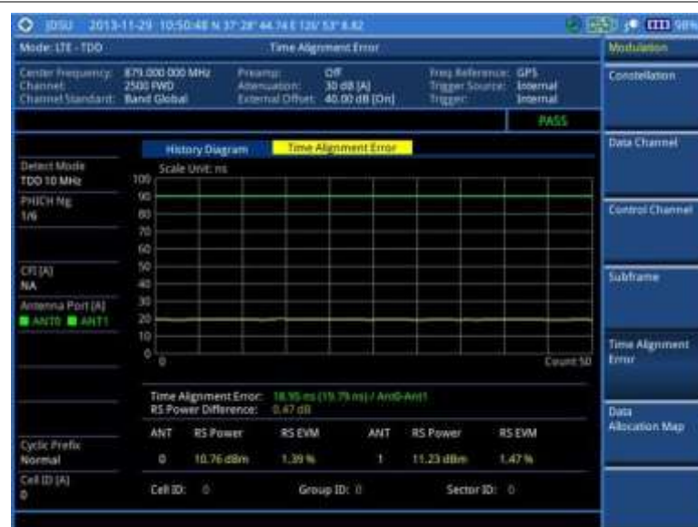
Figure 163 Time alignment error measurement with LTE - TDD signal analyzer
