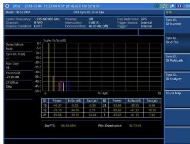
Figure 247 Sync-DL ID vs. Tau measurement with TD-SCDMA OTA signal analyzer
