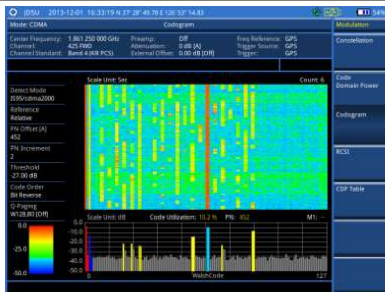
Figure 192 Codogram in full view with CDMA signal analyzer
