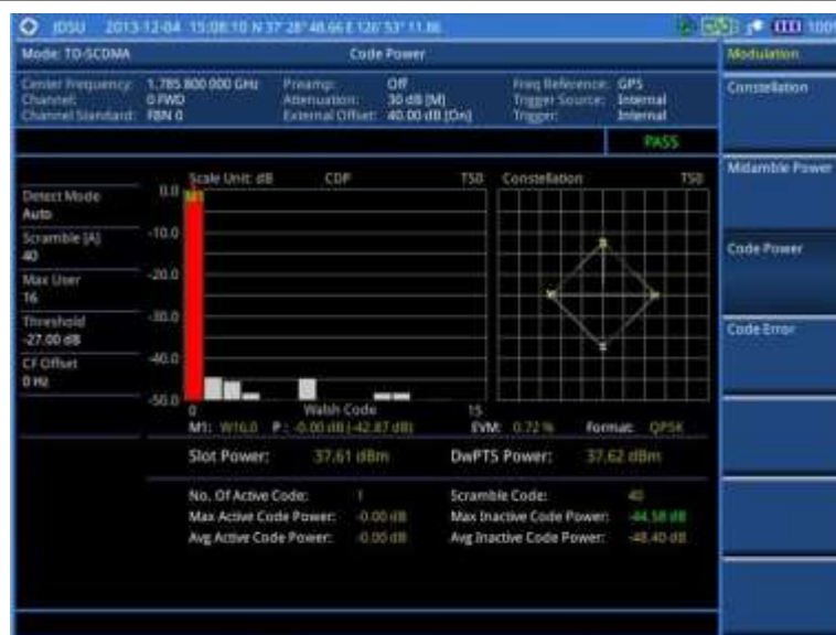
Figure 244 Code power measurement with TD-SCDMA signal analyzer
