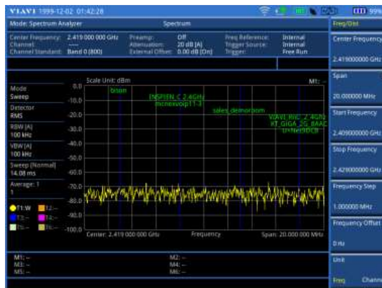
Figure 14 Wi-Fi SSID display with spectrum analyzer
