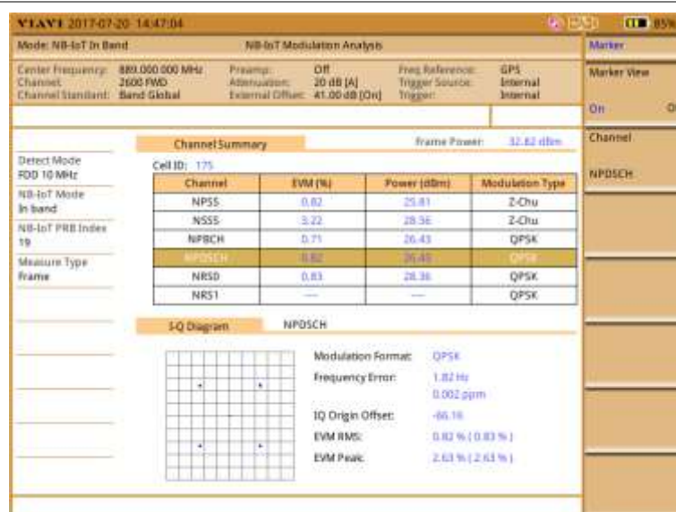
Figure 275 NB-IoT In Band Modulation Analysis measurement screen (Frame)
