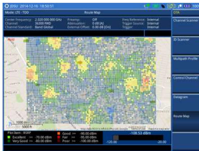
Figure 176 Raster image overlaid on the route map in LTE-TDD OTA signal analyzer
