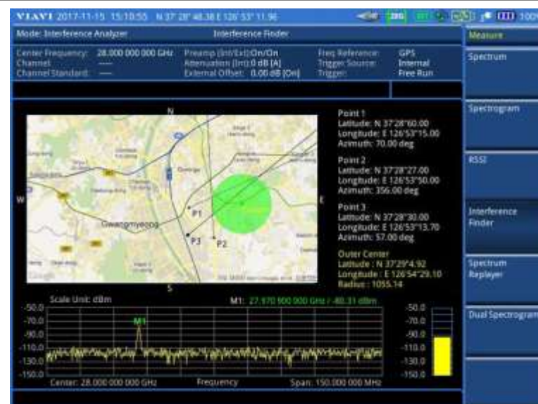
Figure 50 Interference finder measurement in map view (on 28 GHz downconverter)
