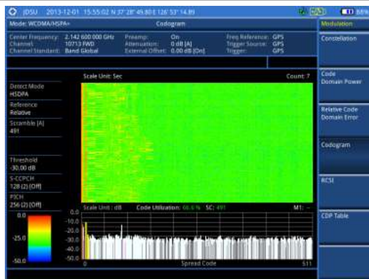
Figure 89 Codogram in full view with WCDMA/HSPA+ signal analyzer
