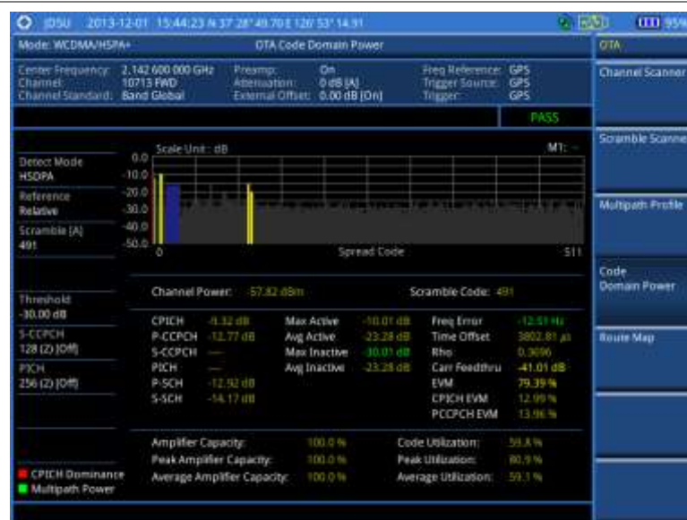
Figure 96 Code domain power measurement with WCDMA/HSPA+ OTA signal analyzer
