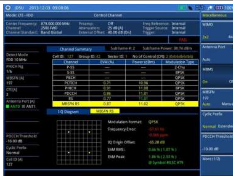
Figure 118 Control channel measurement with LTE - FDD signal analyzer (MBMS On)
