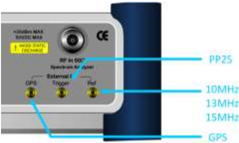
Figure 205 Connection ports for external reference clock
