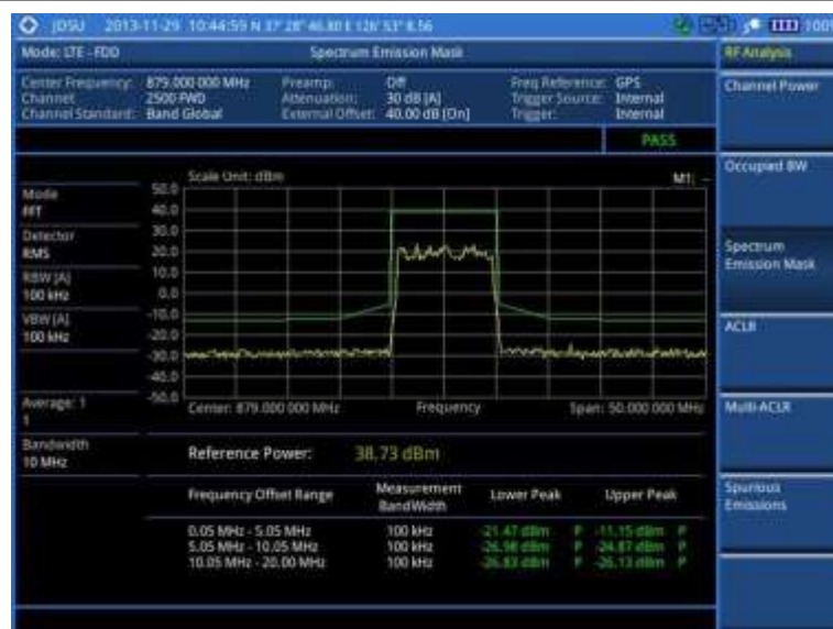
Figure 107 SEM measurement with LTE - FDD signal analyzer
