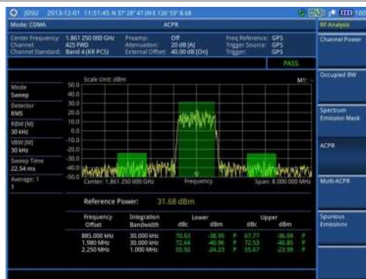
Figure 187 ACPR measurement with CDMA signal analyzer
