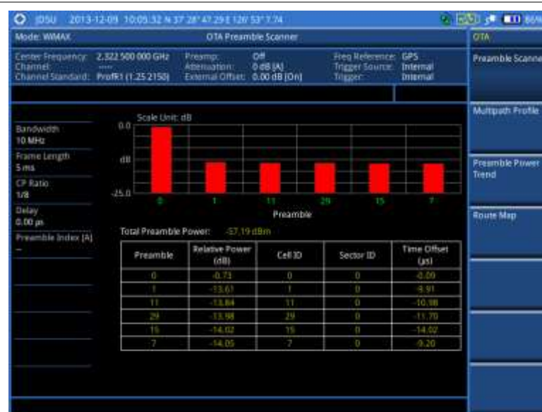
Figure 267 Preamble scanner measurement with Mobile WiMAX OTA signal analyzer
