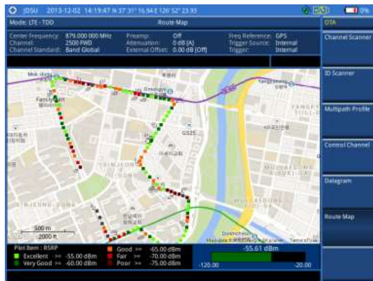
Figure 175 Route map measurement with LTE - TDD OTA signal analyzer
