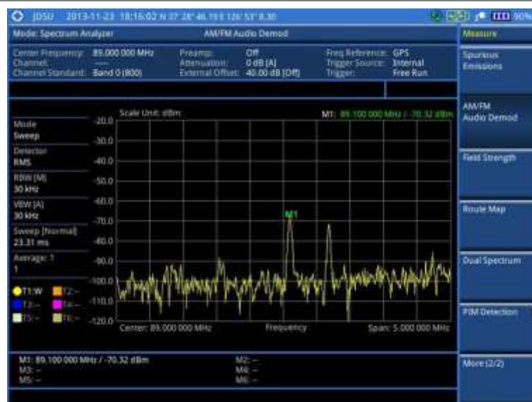
Figure 28 AM/FM audio demodulation with spectrum analyzer
