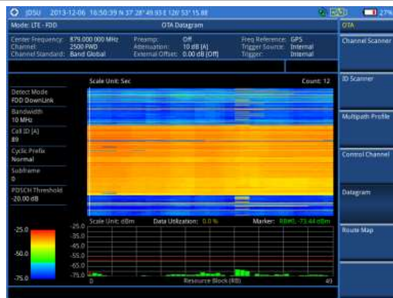
Figure 135 Datagram measurement with LTE - FDD signal analyzer
