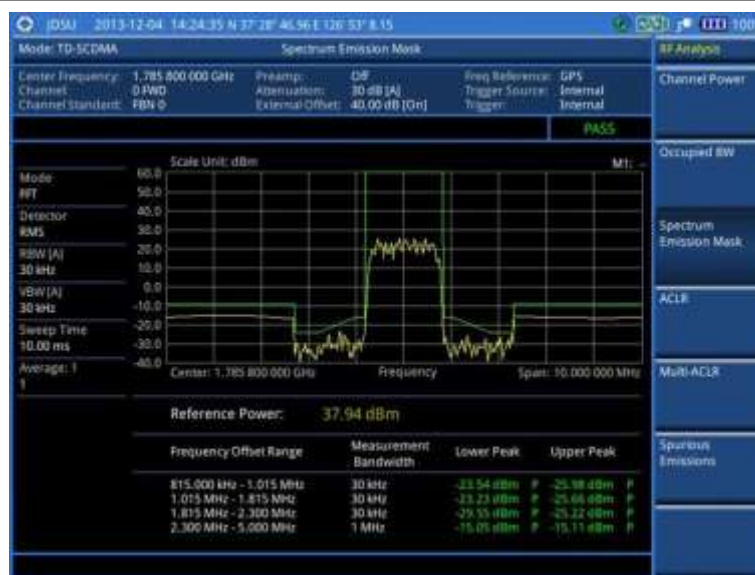
Figure 234 SEM measurement with TD-SCDMA signal analyzer
