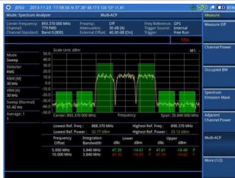
Figure 25 Multi-ACP measurement with spectrum analyzer (on 28 GHz downconverter)
