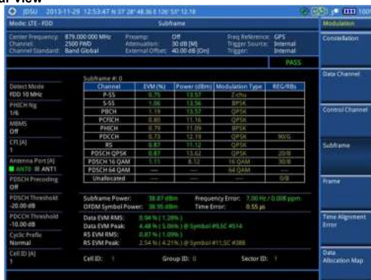
Figure 119 Subframe measurement with LTE - FDD signal analyzer
