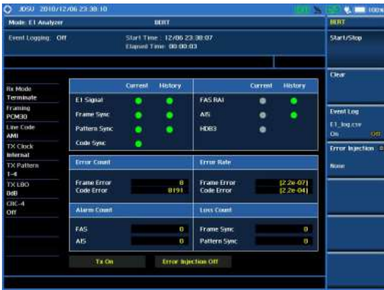
Figure 314 E1 BERT testing for framing PCM30
