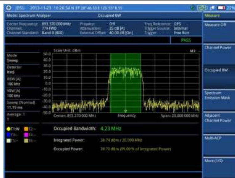
Figure 19 Occupied bandwidth measurement with spectrum analyzer (on 28 GHz)
