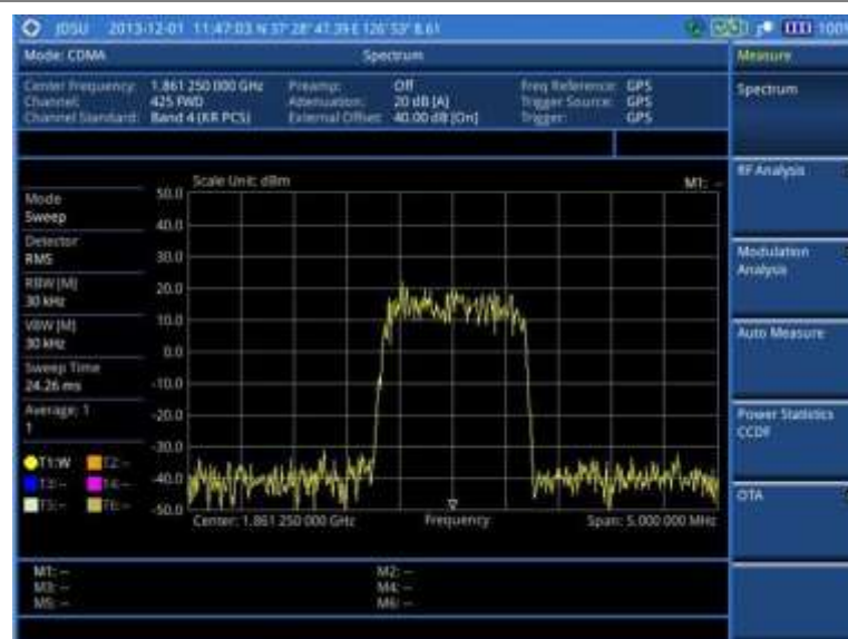
Figure 183 Spectrum measurement screen with CDMA signal analyzer
