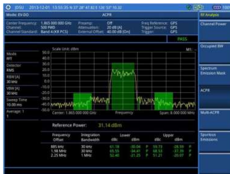
Figure 210 ACPR measurement with EV-DO signal analyzer
