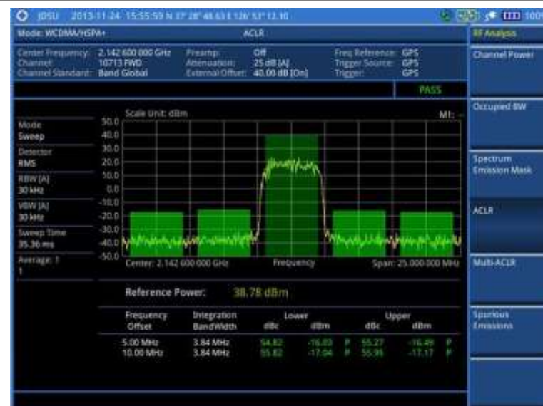
Figure 83 ACLR measurement with WCDMA/HSPA+ signal analyzer
