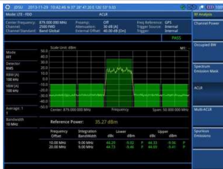
Figure 108 ACLR measurement with LTE - FDD signal analyzer
