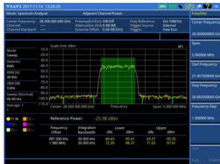
Figure 23 Adjacent channel power measurement with spectrum analyzer (on 28 GHz downconverter)
