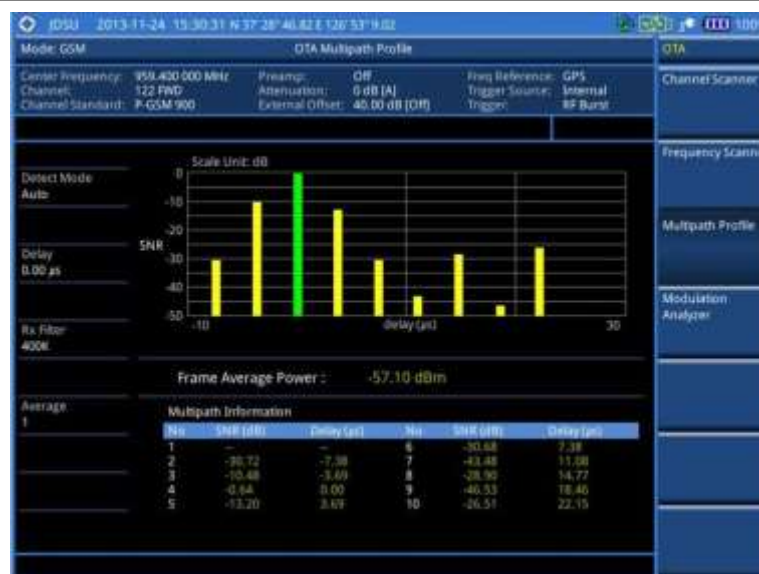
Figure 72 Multipath profile measurement with GSM OTA signal analyzer
