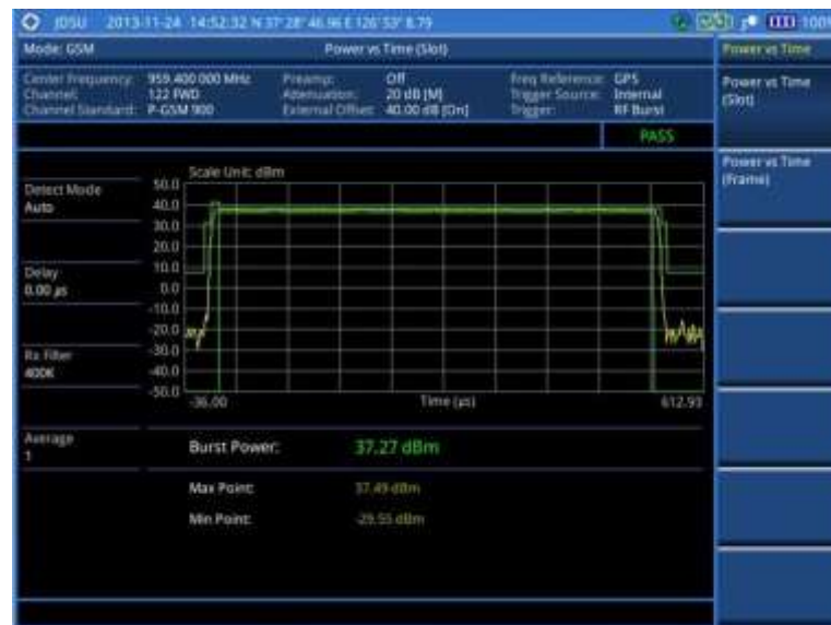
Figure 67 Power vs. time (slot) measurement with GSM/EDGE signal analyzer
