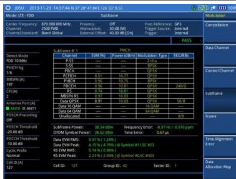
Figure 120 Subframe measurement with LTE - FDD signal analyzer (MBMS On)
