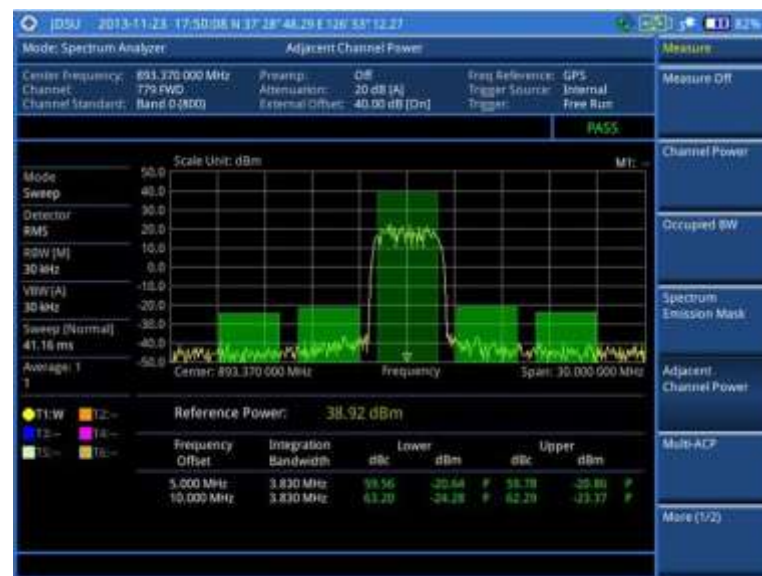
Figure 22 Adjacent channel power measurement with spectrum analyzer
