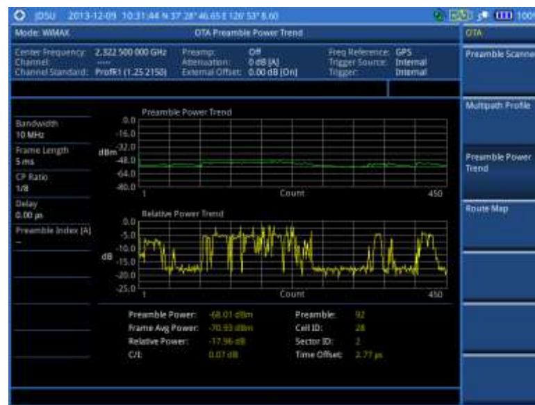
Figure 269 Preamble power trend with Mobile WiMAX OTA signal analyzer
