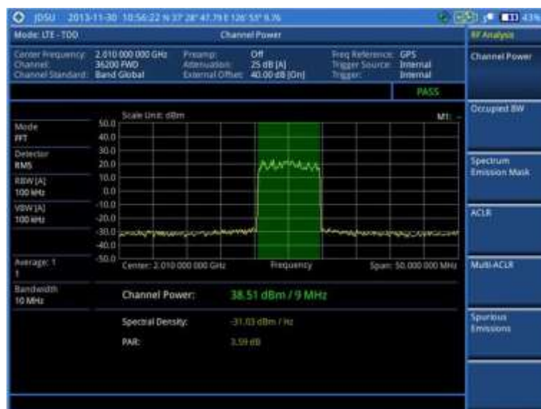
Figure 147 Channel power measurement with LTE - TDD signal analyzer
