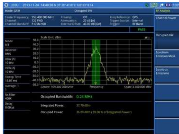
Figure 63 Occupied bandwidth measurement with GSM signal analyzer
