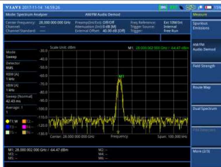
Figure 29 AM/FM audio demodulation with spectrum analyzer (on GHz downconverter)
