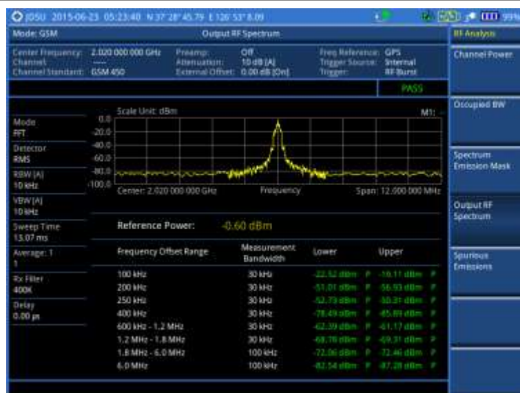
Figure 65 Output RF spectrum measurement with GSM signal analyzer
