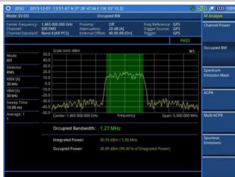
Figure 208 Occupied bandwidth measurement with EV-DO signal analyzer
