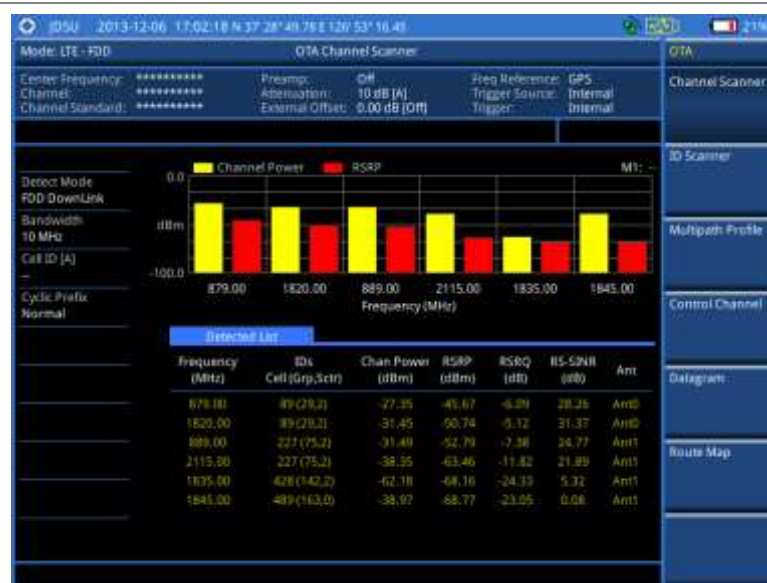
Figure 131 Channel scanner measurement with LTE - FDD OTA signal analyzer
