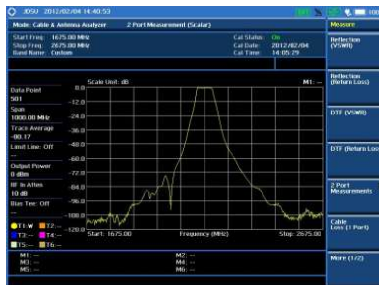
Figure 307 2-port scalar measurement
