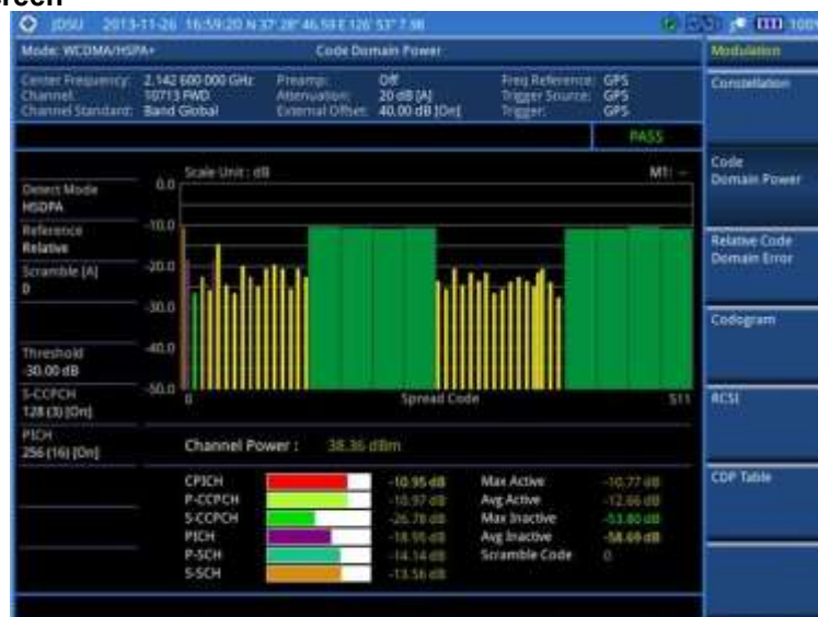
Figure 87 Code domain power measurement with WCDMA/HSPA+ signal analyzer
