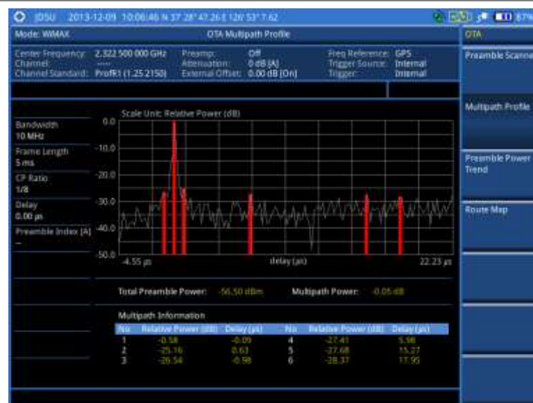
Figure 268 Multipath profile measurement with Mobile WiMAX OTA signal analyzer
