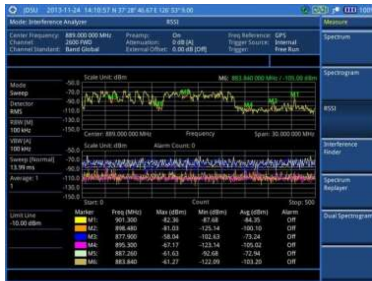
Figure 48 Interference measurement in RSSI (on 28 GHz downconverter)
