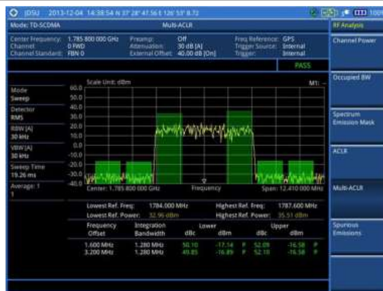
Figure 236 Multi-ACLR measurement with TD-SCDMA signal analyzer
