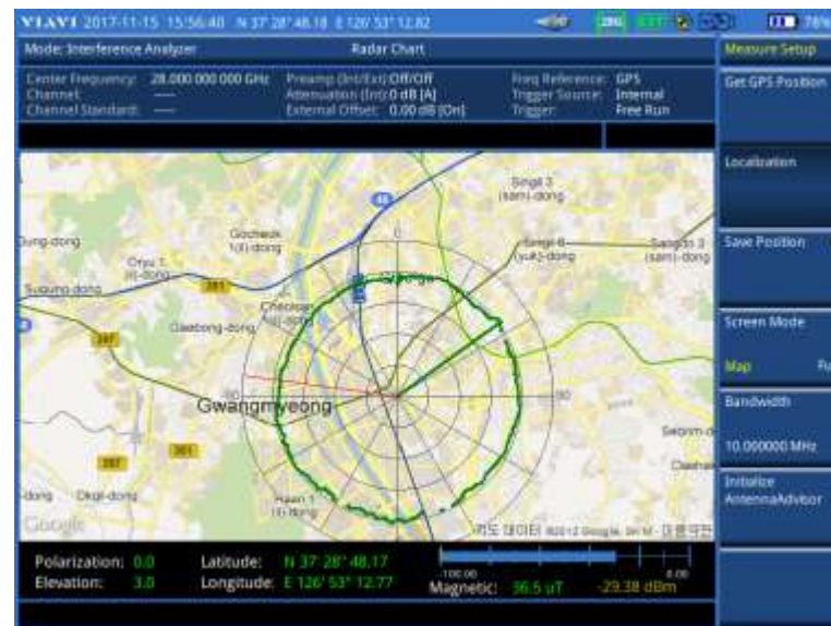
Figure 56 Localized RSSI data on the radar chart (on 28 GHz downconverter)
