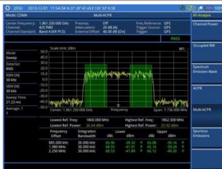
Figure 188 Multi-ACPR measurement with CDMA signal analyzer
