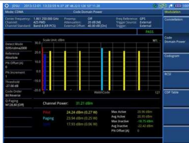
Figure 191 Code domain power measurement with CDMA signal analyzer
