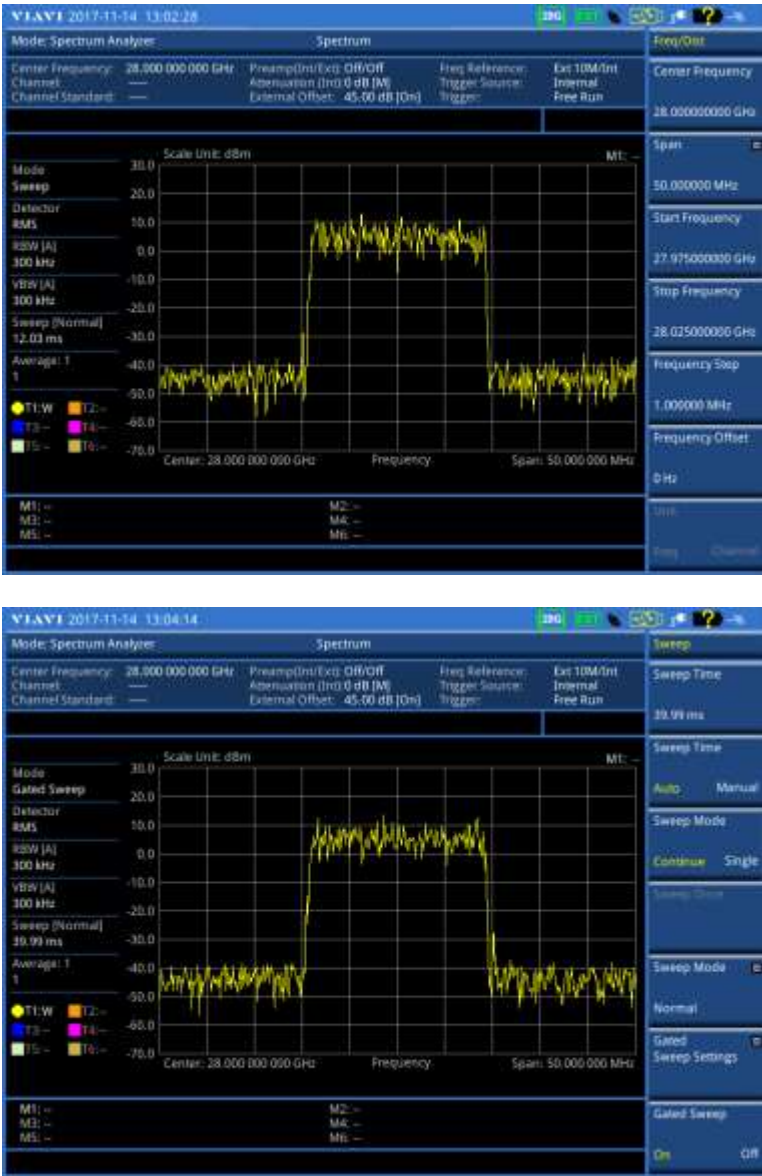
Figure 13 Spectrum measurement with spectrum analyzer (on 28 GHz downconverter)
