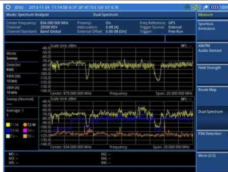
Figure 34 Dual spectrum measurement with spectrum analyzer
