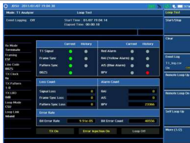
Figure 323 T1 loop testing
