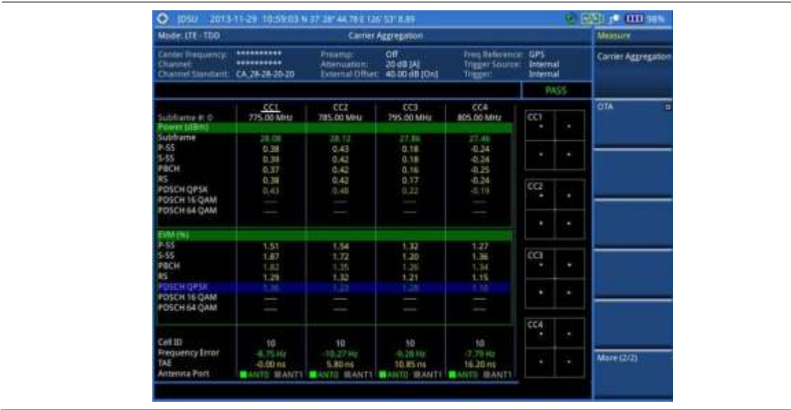
Figure 169 Carrier aggregation measurement with LTE - TDD signal analyzer (SA)
