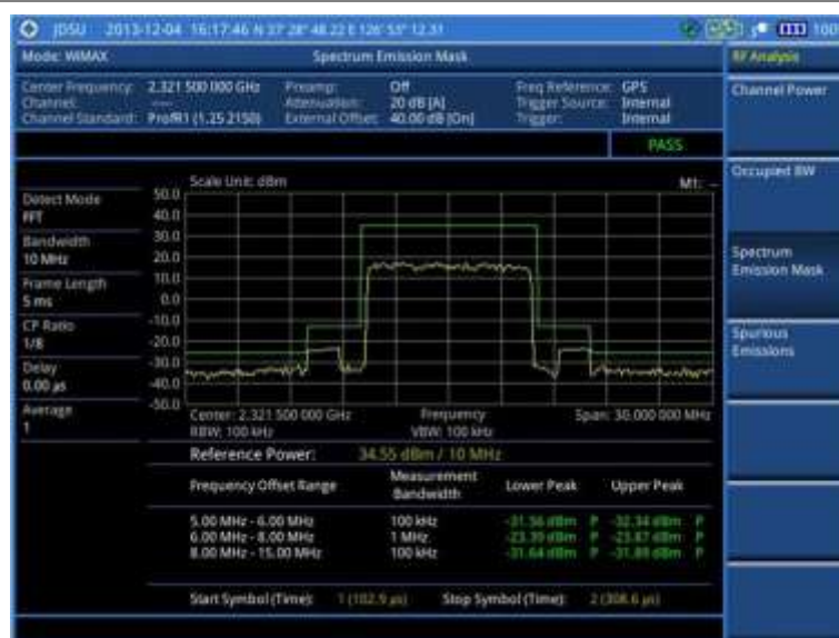
Figure 259 SEM measurement with Mobile WiMAX signal analyzer
