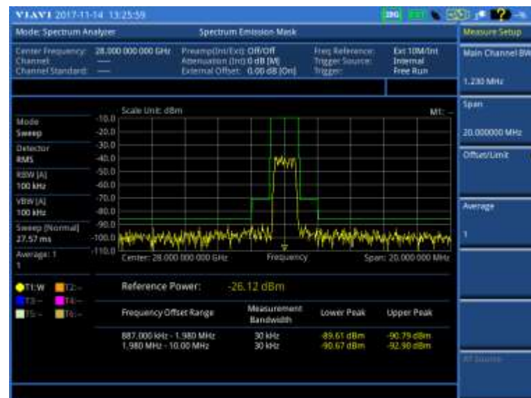
Figure 21 Spectrum emission mask measurement with spectrum analyzer (on 28 GHz downconverter)
