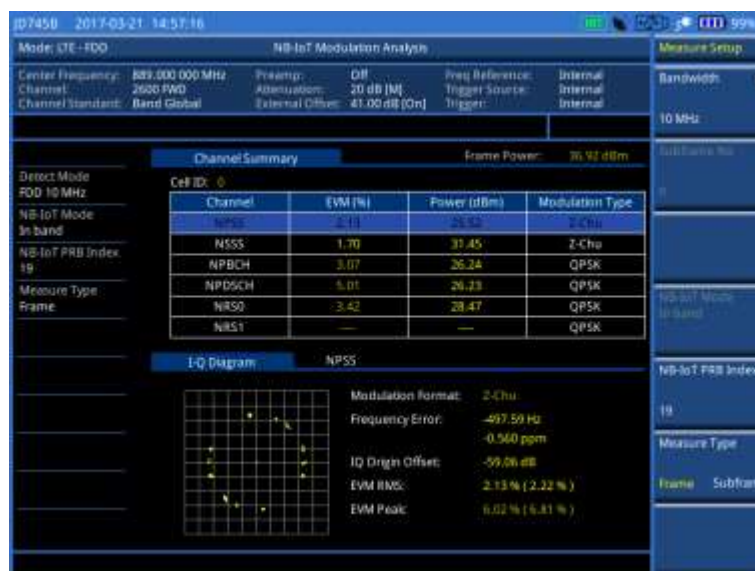
Figure 140 NB-IoT modulation measurement with LTE-FDD signal analyzer (Subframe 2)
