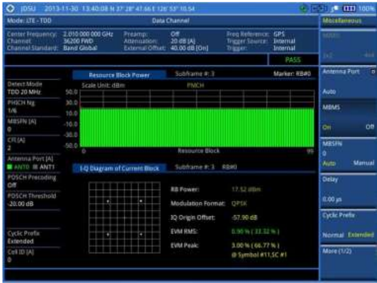
Figure 158 Data channel measurement with LTE - TDD signal analyzer (MBMS On)
