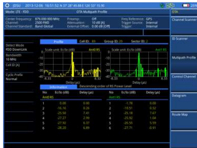
Figure 133 Multipath profile measurement with LTE - FDD OTA signal analyzer
