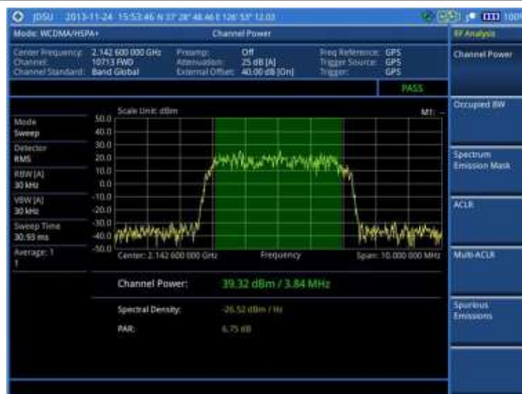
Figure 80 Channel power measurement with WCDMA/HSPA+ signal analyzer
