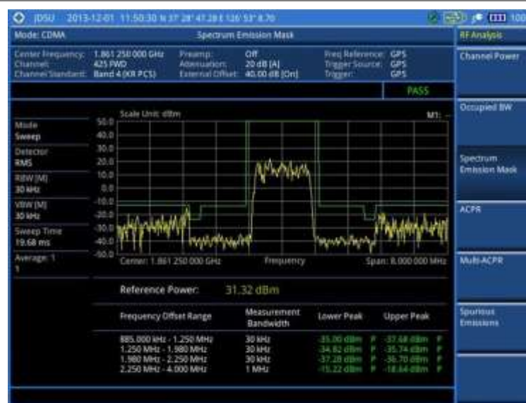
Figure 186 SEM measurement with CDMA signal analyzer
