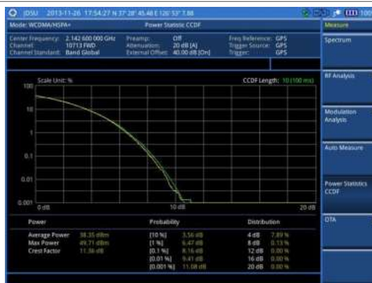
Figure 92 CCDF measurement with WCDMA/HSPA+ signal analyzer
