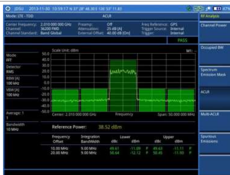
Figure 150 ACLR measurement with LTE - TDD signal analyzer
