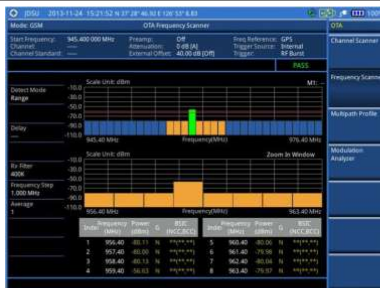
Figure 71 Frequency scanner measurement with GSM OTA signal analyzer
