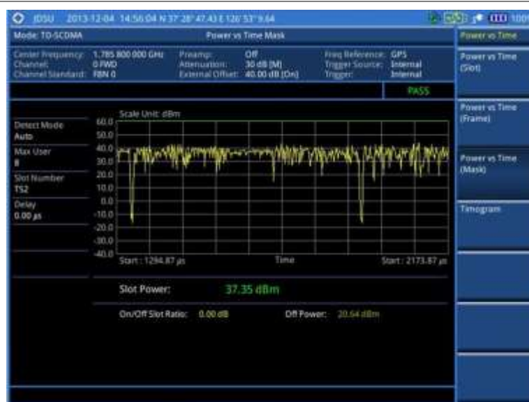
Figure 240 Power vs. time (mask) measurement with TD-SCDMA signal analyzer
