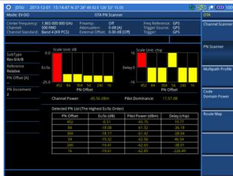
Figure 222 PN scanner measurement with EV-DO OTA signal analyzer
