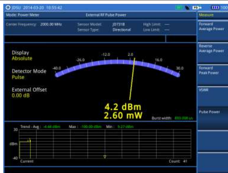
Figure 336 External power measurement of pulse power
