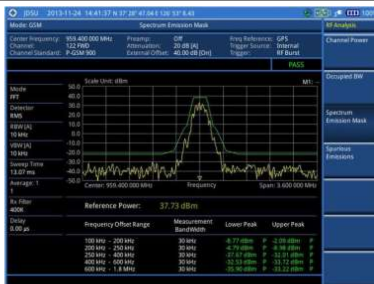
Figure 64 SEM measurement with GSM signal analyzer
