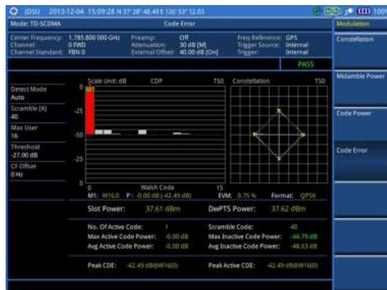
Figure 245 Code error measurement with TD-SCDMA signal analyzer
