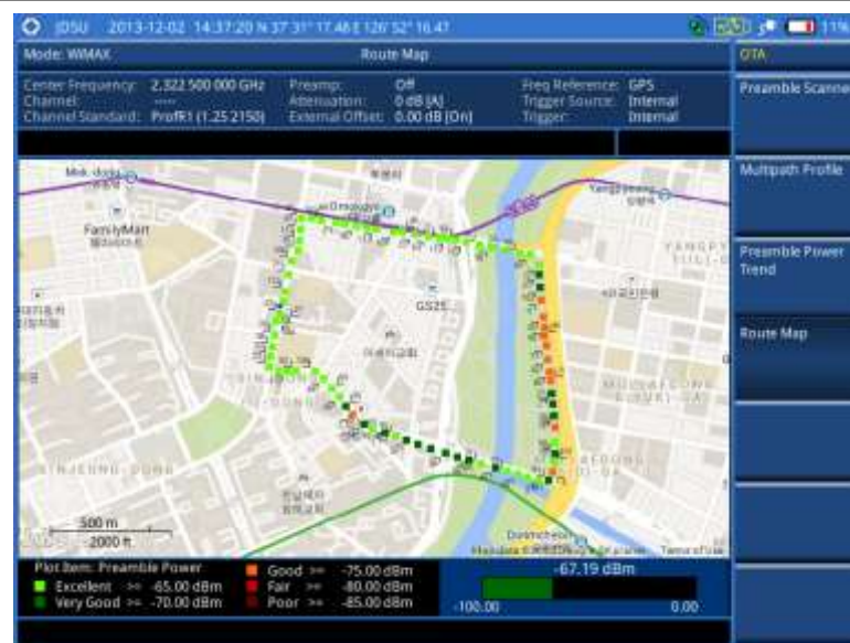
Figure 270 Route map measurement with Mobile WiMAX OTA signal analyzer
