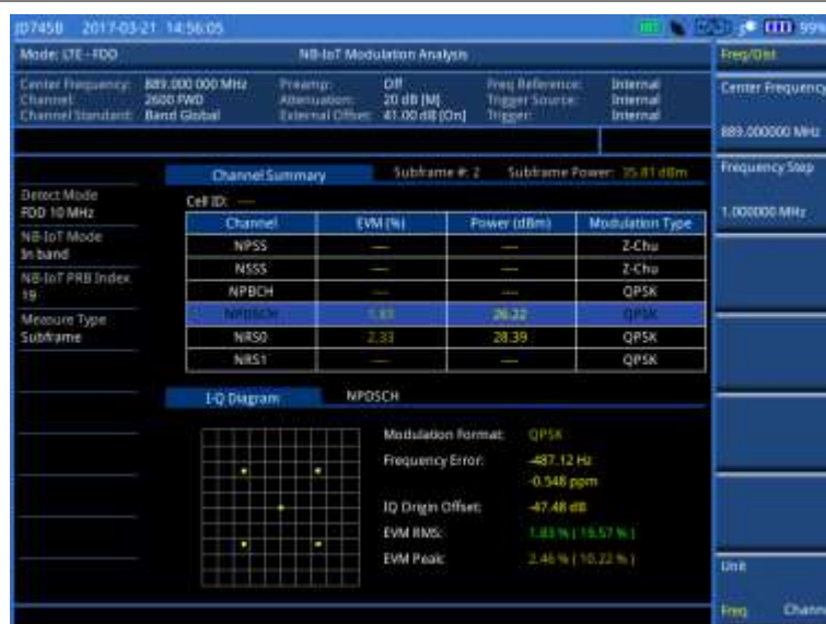
Figure 140 NB-IoT modulation measurement with LTE-FDD signal analyzer (Subframe 2)
