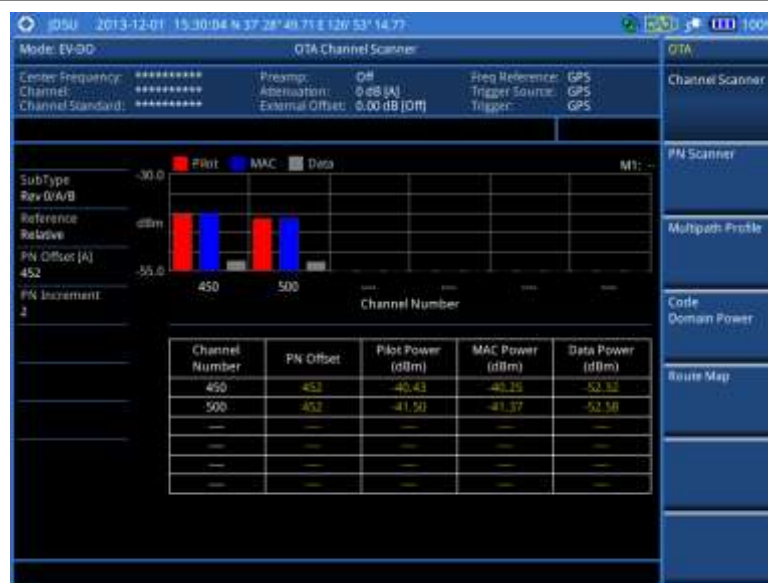
Figure 221 Channel scanner measurement with EV-DO OTA signal analyzer
