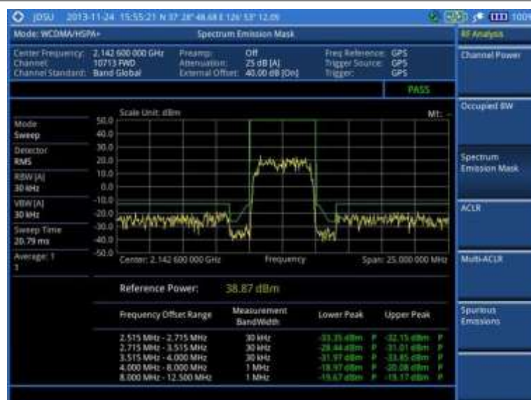
Figure 62 SEM measurement with WCDMA/HSPA+ signal analyzer
