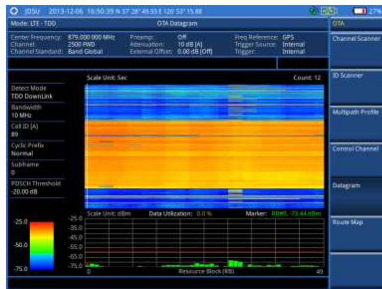
Figure 154 Datagram measurement with LTE - TDD signal analyzer
