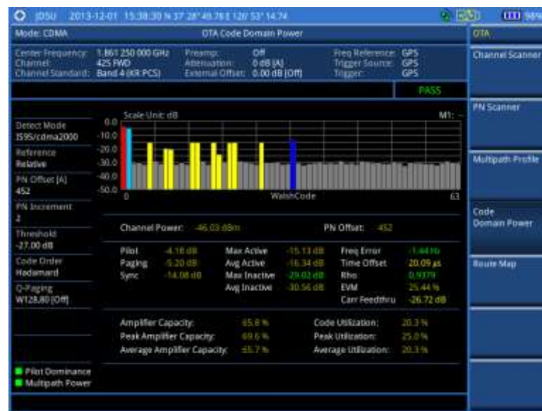
Figure 179 Code domain power measurement with CDMA OTA signal analyzer
