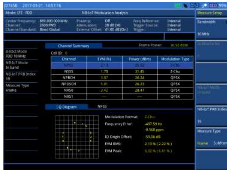
Figure 120 NB-IoT modulation measurement with LTE-FDD signal analyzer (Subframe 2)
