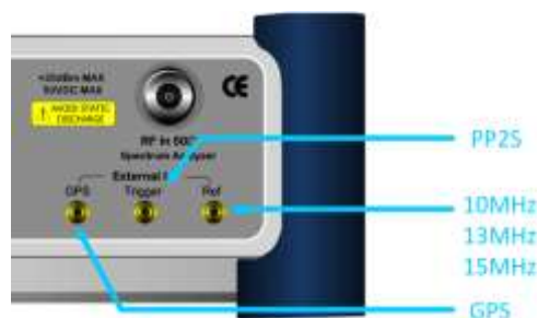
Figure 210 Connection ports for external reference clock
