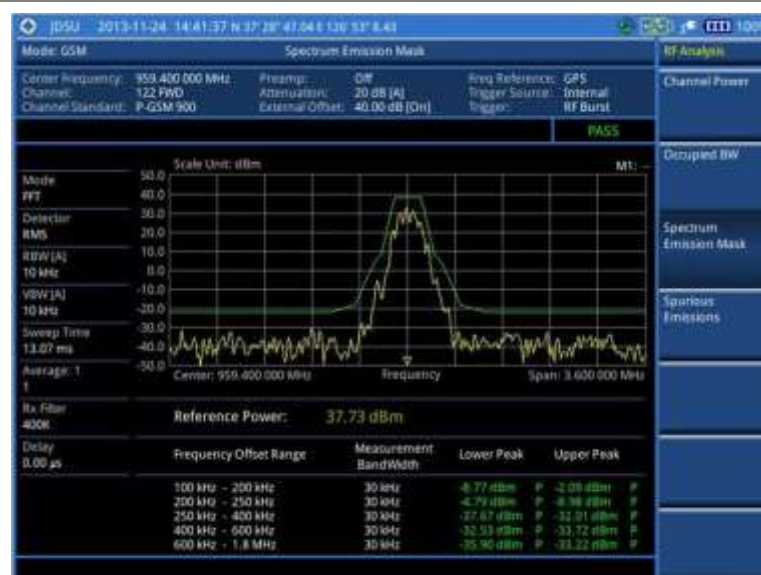
Figure 44 SEM measurement with GSM signal analyzer
