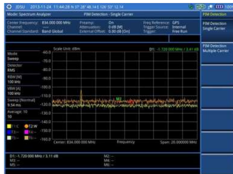
Figure 23 PIM detection for single carrier
