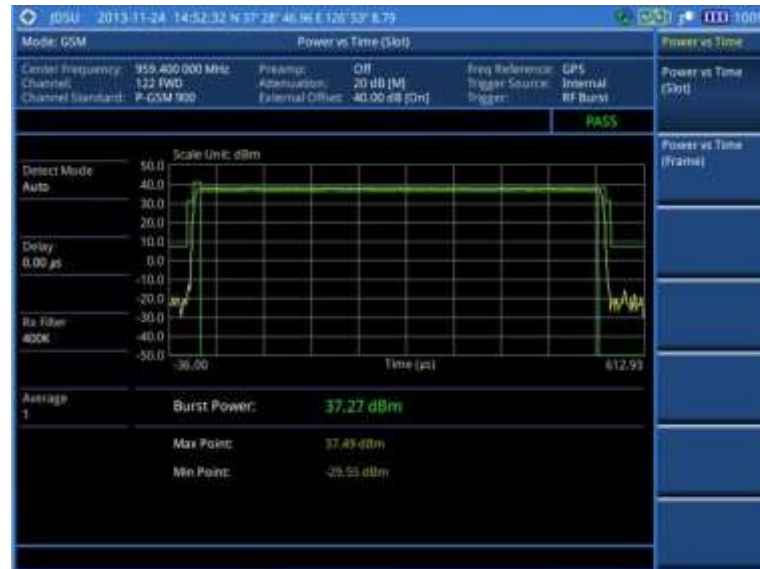
Figure 47 Power vs. time (slot) measurement with GSM/EDGE signal analyzer
