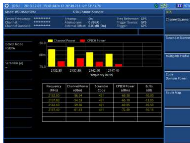
Figure 73 Channel scanner measurement with WCDMA/HSPA+ OTA signal analyzer
