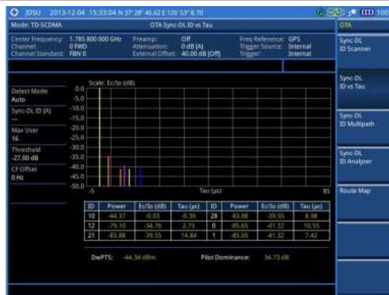
Figure 227 Sync-DL ID vs. Tau measurement with TD-SCDMA OTA signal analyzer
