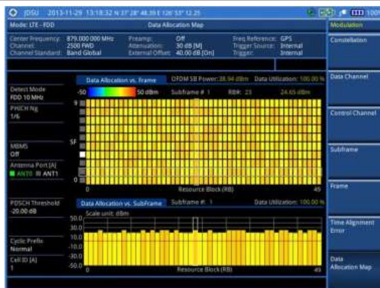
Figure 105 Data allocation map measurement with LTE - FDD signal analyzer (MBMS On)
