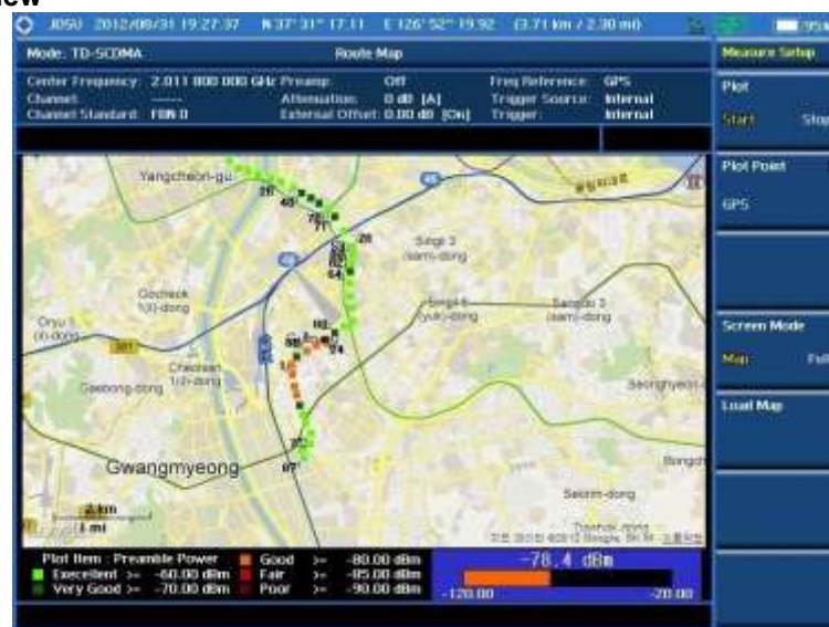
Figure 230 Route map measurement with TD-SCDMA OTA signal analyzer
