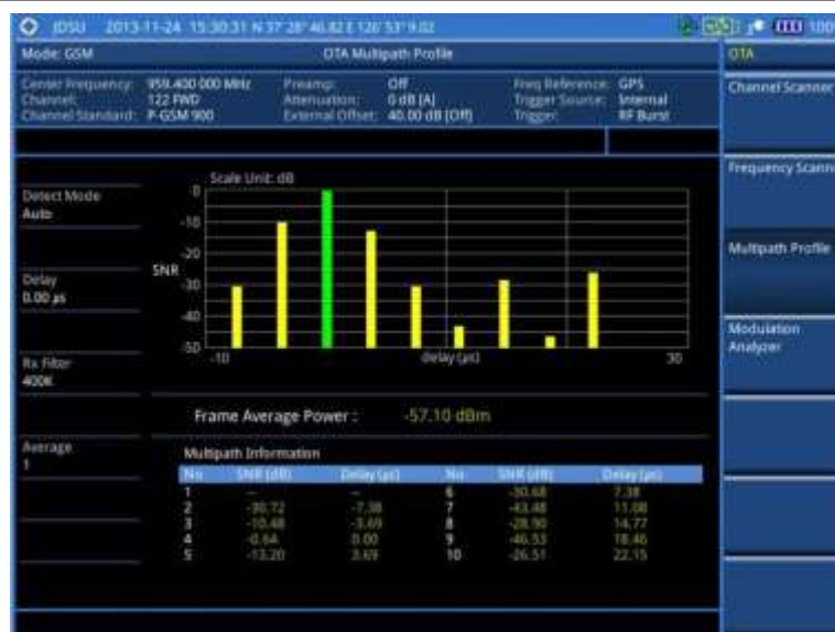
Figure 52 Multipath profile measurement with GSM OTA signal analyzer
