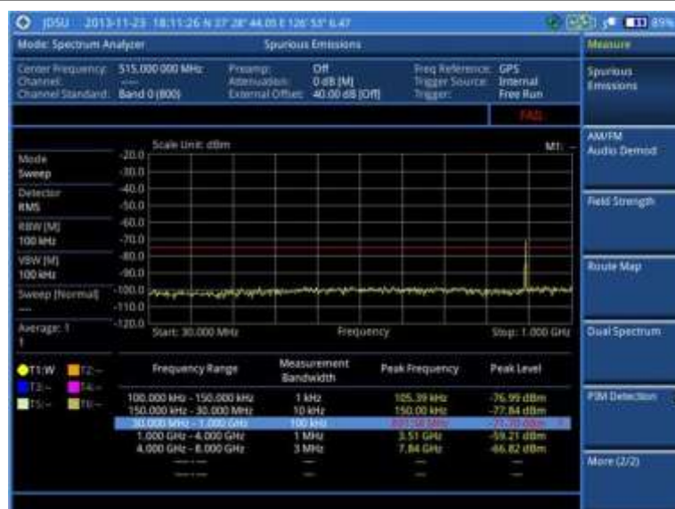
Figure 17 Spurious emissions measurement with spectrum analyzer
