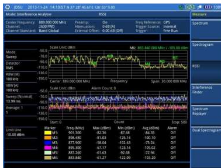
Figure 32 Interference measurement in RSSI
