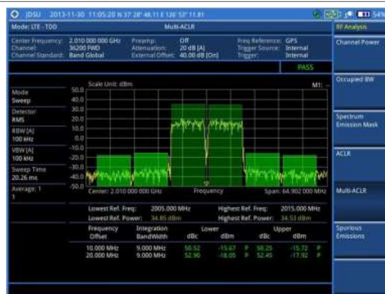
Figure 131 Multi-ACLR measurement with LTE - TDD signal analyzer
