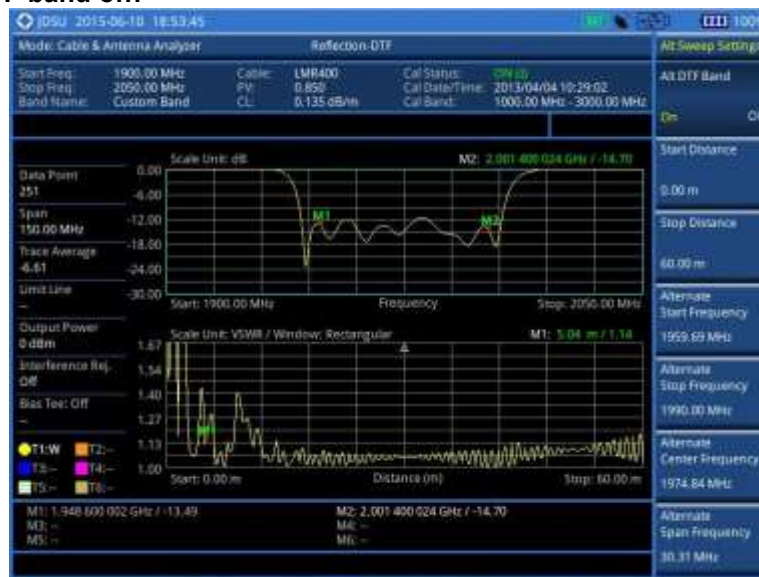
Figure 264 Reflection-DTF dual measurement
