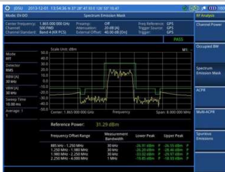
Figure 189 SEM measurement with EV-DO signal analyzer
