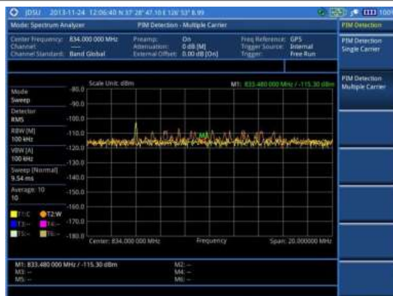
Figure 24 PIM detection for multiple carriers
