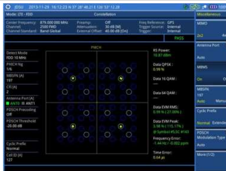
Figure 93 Constellation measurement with LTE - FDD signal analyzer (MBMS On)
