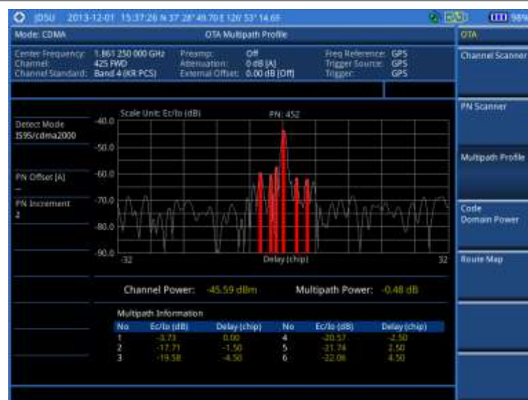
Figure 178 Multipath profile measurement with CDMA OTA signal analyzer
