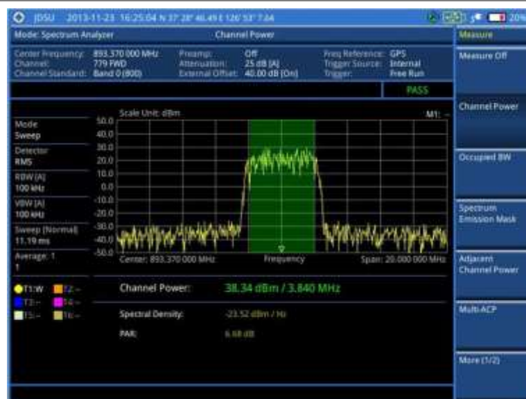
Figure 12 Channel power measurement with spectrum analyzer
