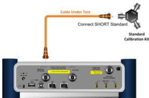
Figure 258 Connection for cable loss (1 port) measurement
