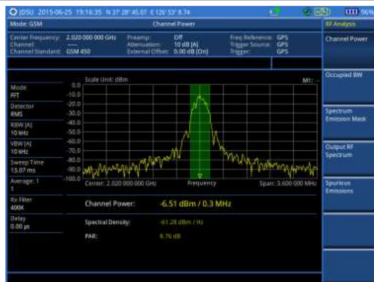
Figure 42 Channel power measurement with GSM signal analyzer
