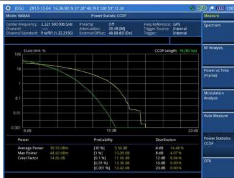
Figure 246 CCDF measurement with Mobile WiMAX signal analyzer
