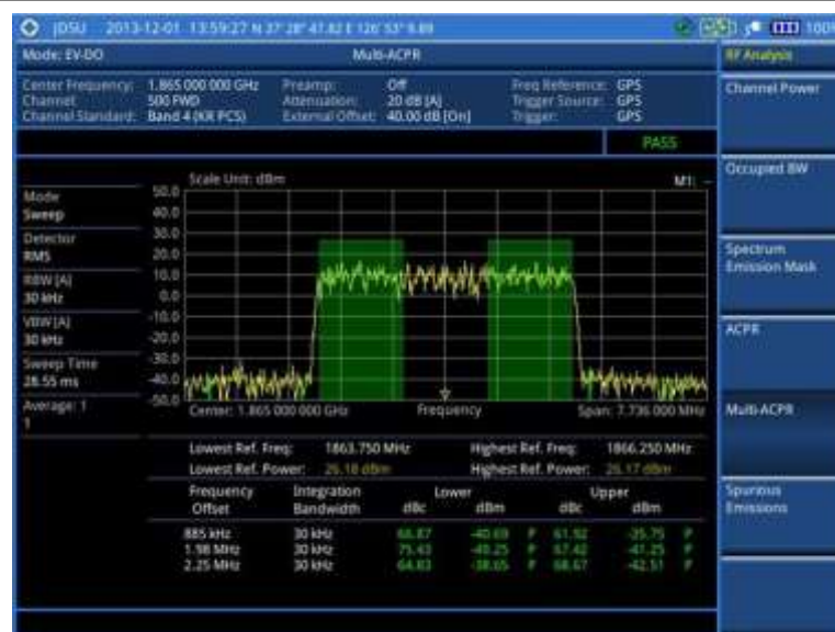
Figure 191 Multi-ACPR measurement with EV-DO signal analyzer
