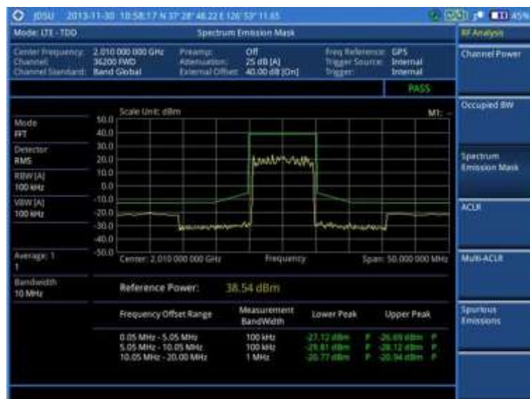
Figure 129 SEM measurement with LTE - TDD signal analyzer
