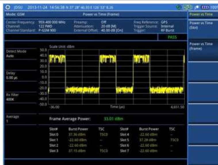
Figure 48 Power vs. time (frame) measurement with GSM signal analyzer
