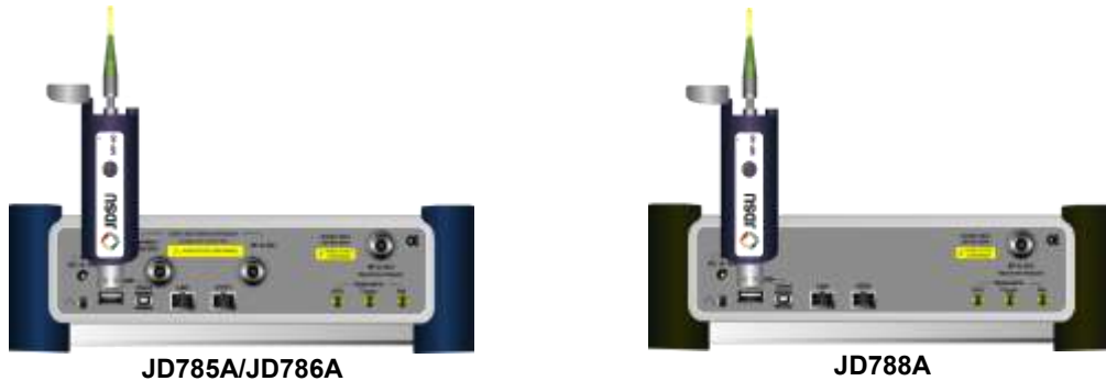
Figure 301 Optical power sensor connection
