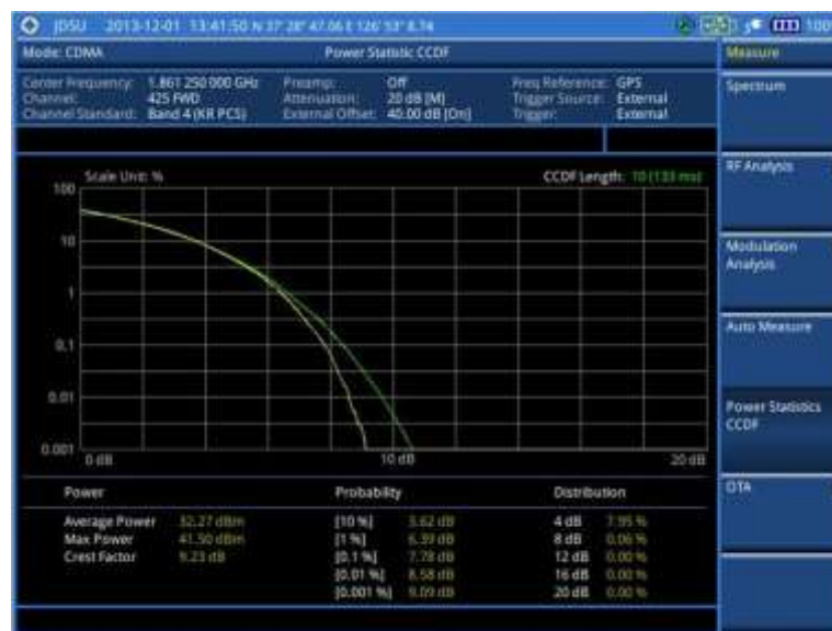
Figure 175 CCDF measurement with CDMA signal analyzer
