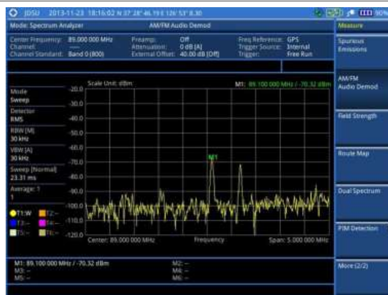
Figure 18 AM/FM audio demodulation with spectrum analyzer
