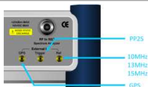
Figure 235 Connection ports for external reference clock
