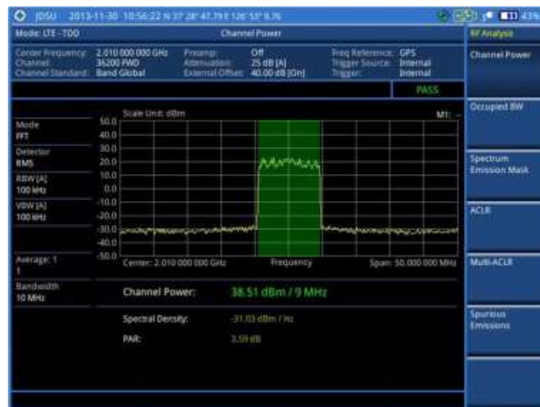
Figure 127 Channel power measurement with LTE - TDD signal analyzer
