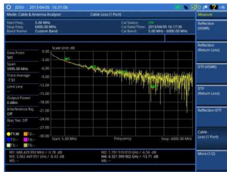
Figure 265 Cable loss (1 port) measurement
