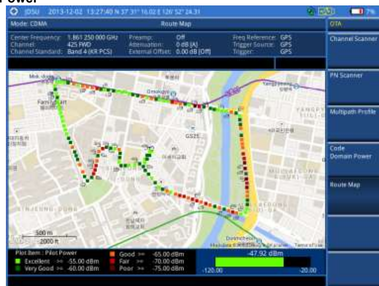
Figure 180 Route map measurement with CDMA OTA signal analyzer
