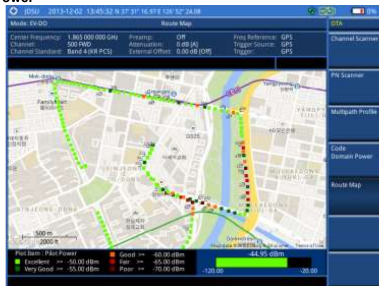
Figure 205 Route map measurement with EV-DO OTA signal analyzer
