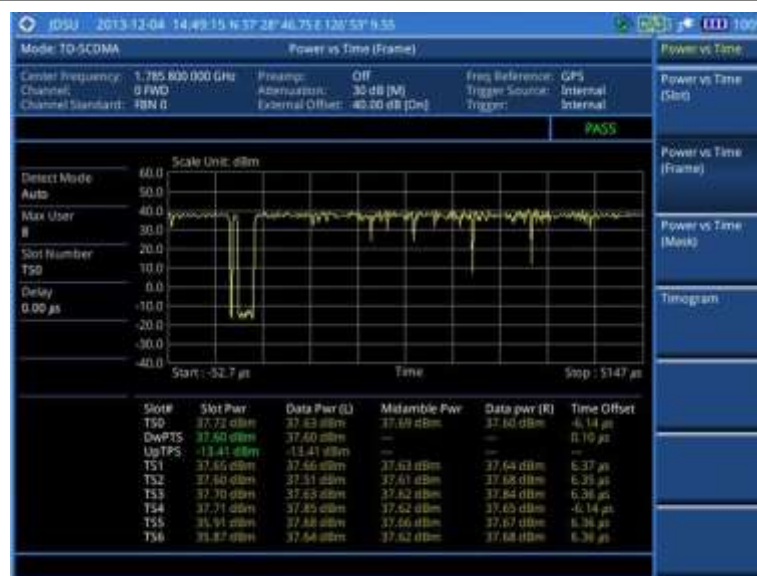
Figure 219 Power vs. time (frame) measurement with TD-SCDMA signal analyzer
