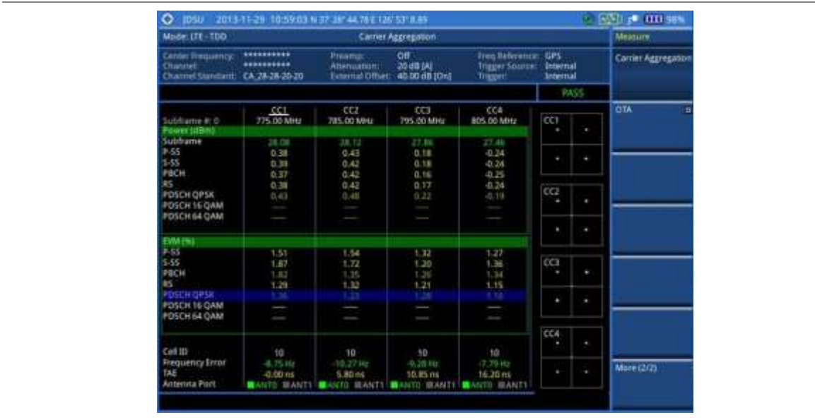
Figure 149 Carrier aggregation measurement with LTE - TDD signal analyzer (SA)
