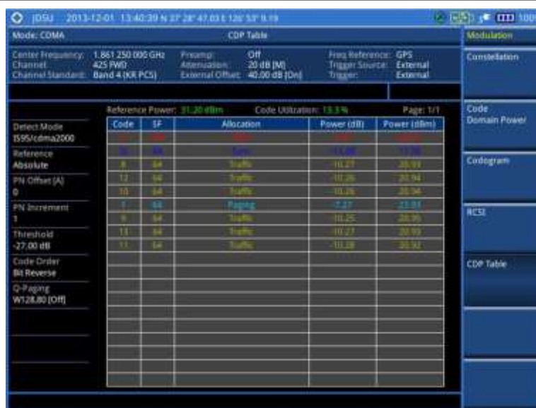
Figure 174 CDP Table measurement with CDMA signal analyzer
