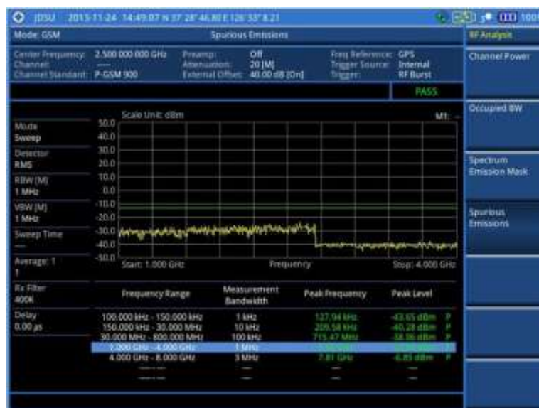
Figure 46 Spurious emissions measurement with GSM signal analyzer
