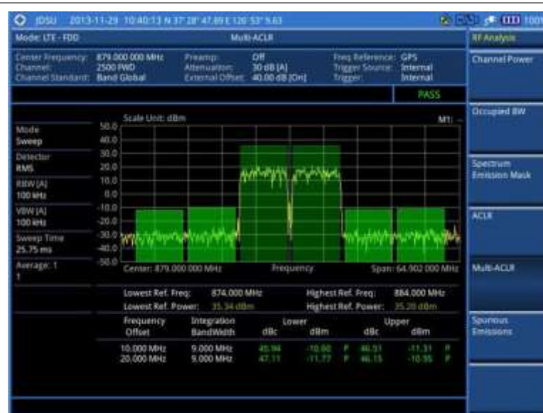
Figure 89 Multi-ACLR measurement with LTE - FDD signal analyzer
