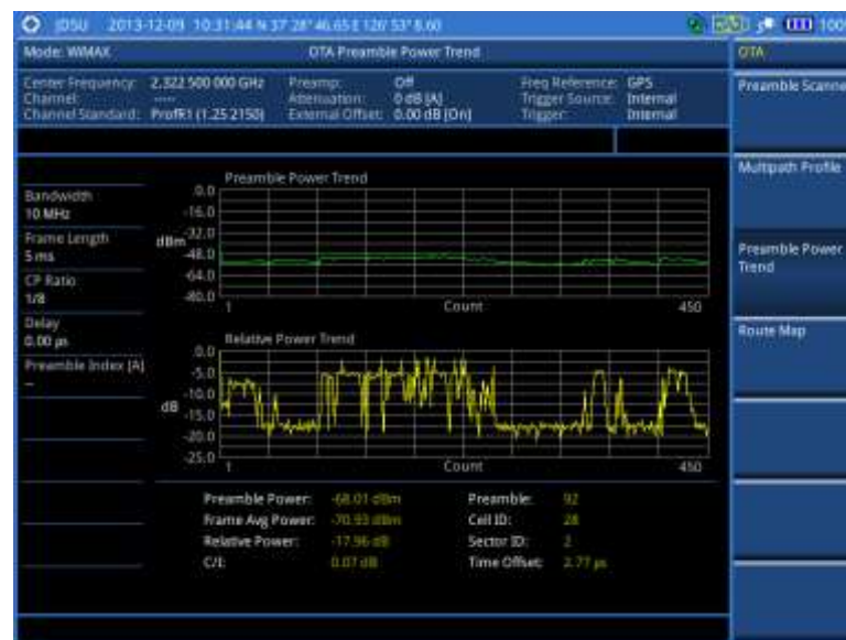
Figure 249 Preamble power trend with Mobile WiMAX OTA signal analyzer
