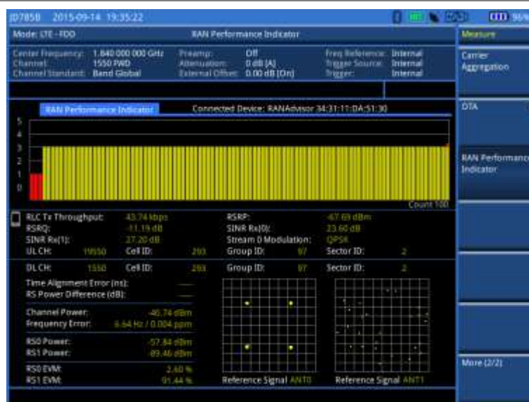
Figure 118 RAN performance indicator in LTE-FDD signal analyzer
