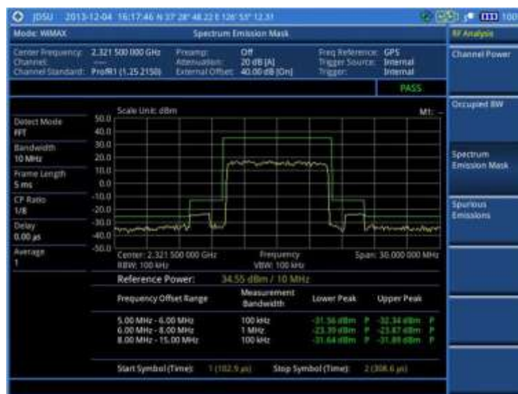
Figure 239 SEM measurement with Mobile WiMAX signal analyzer
