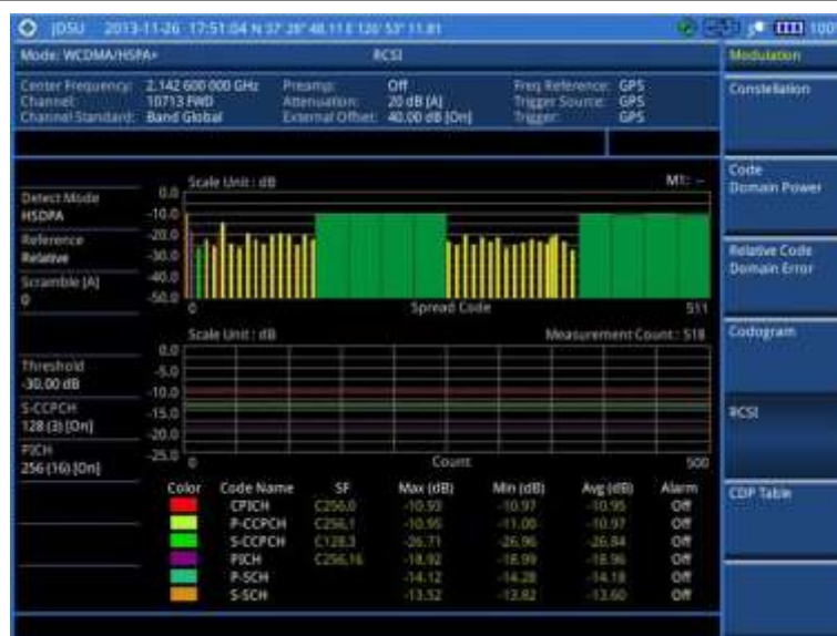
Figure 70 RCSI measurement with WCDMA/HSPA+ signal analyzer
