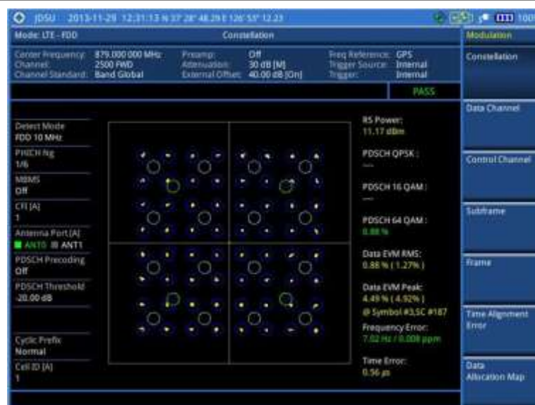
Figure 93 Constellation measurement with LTE - FDD signal analyzer (MBMS On)
