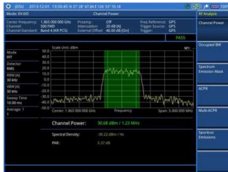
Figure 187 Channel power measurement with EV-DO signal analyzer
