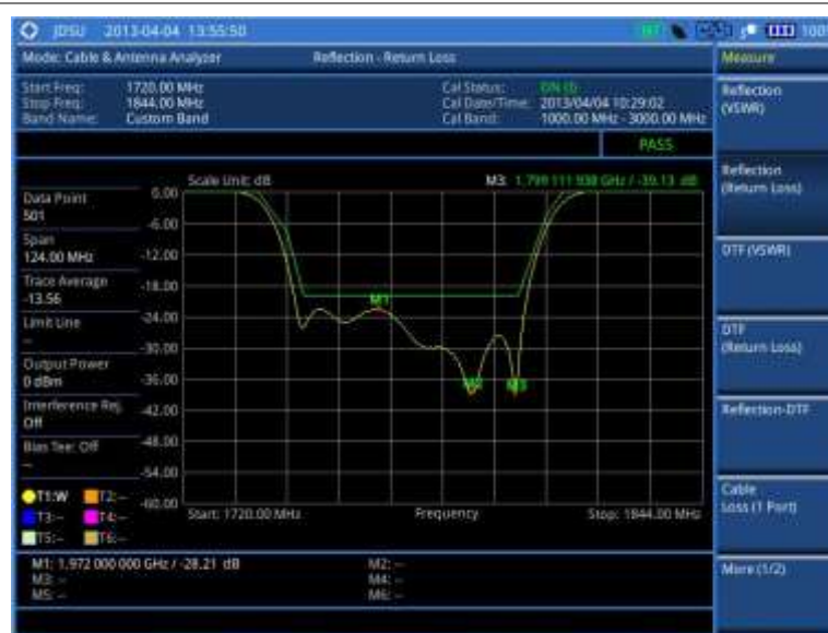
Figure 261 Reflection measurement in return loss scale
