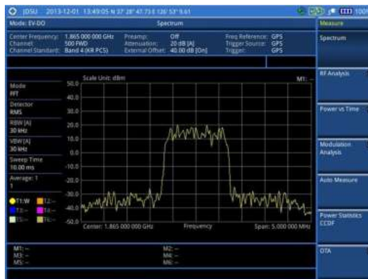
Figure 186 Spectrum measurement screen with EV-DO signal analyzer
