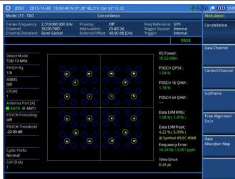
Figure 135 Constellation measurement with LTE - TDD signal analyzer
