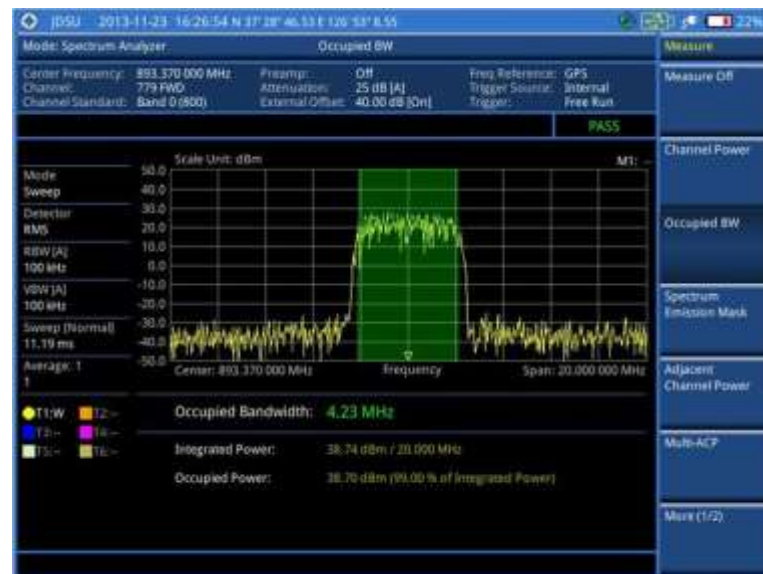
Figure 13 Occupied bandwidth measurement with spectrum analyzer
