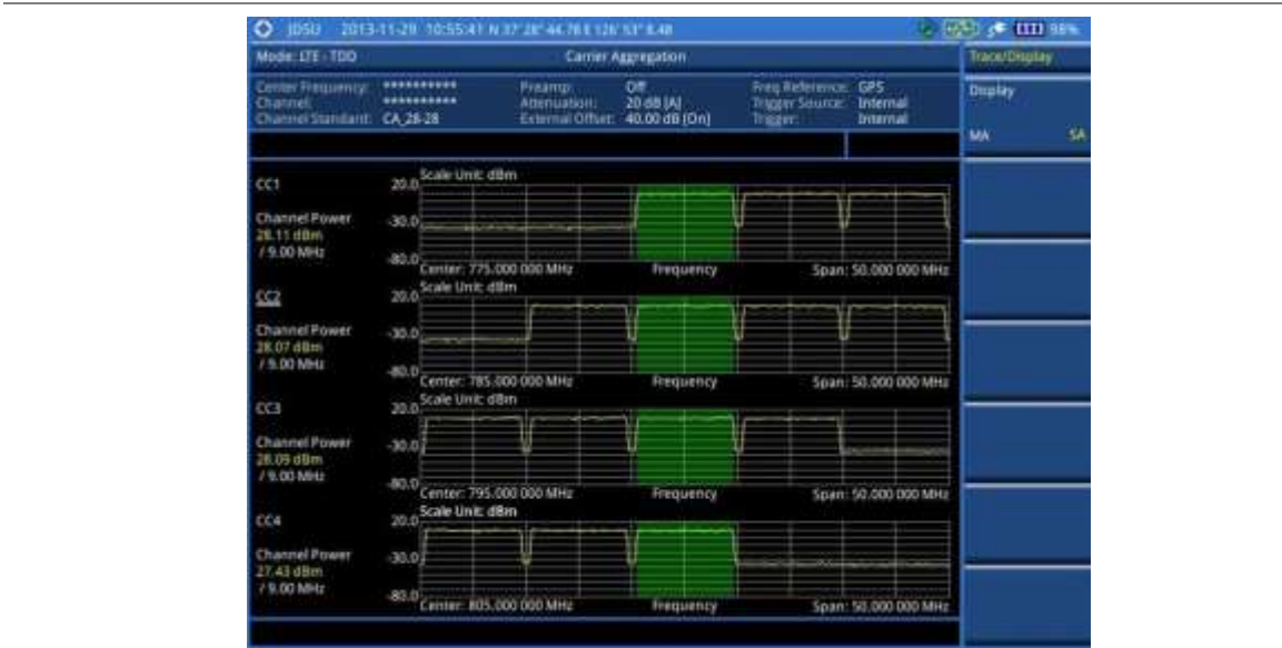
Figure 149 Carrier aggregation measurement with LTE - TDD signal analyzer (SA)
