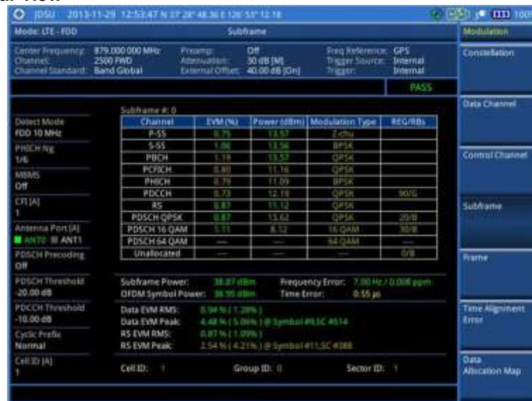
Figure 99 Subframe measurement with LTE - FDD signal analyzer
