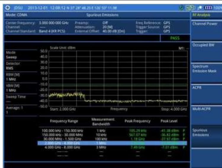
Figure 169 Spurious emissions measurement with CDMA signal analyzer
