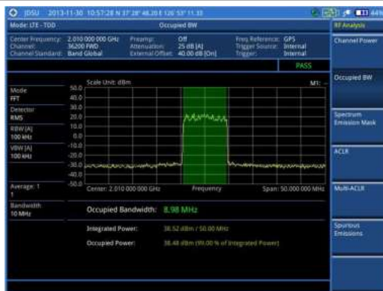
Figure 128 Occupied bandwidth measurement with LTE - TDD signal analyzer
