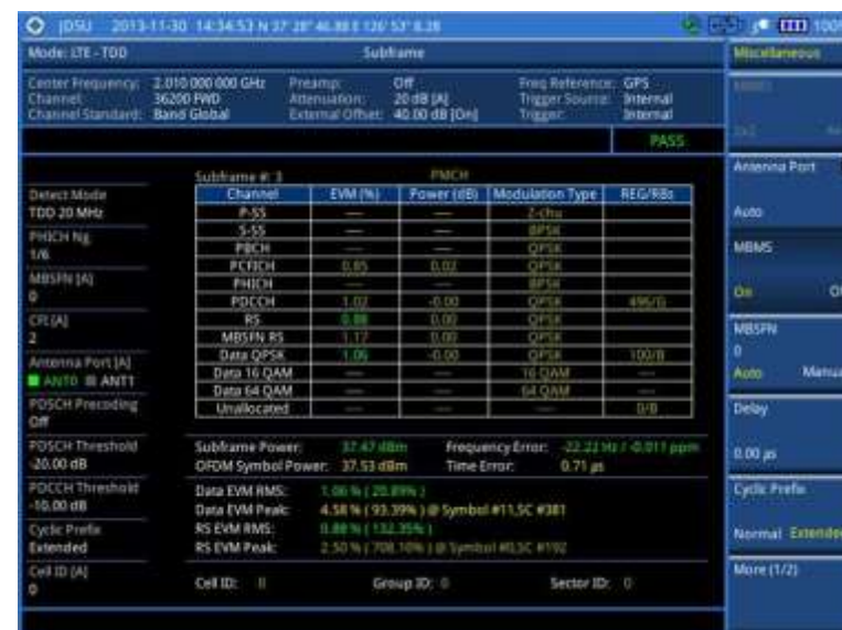
Figure 142 Subframe measurement with LTE - TDD signal analyzer (MBMS On)
