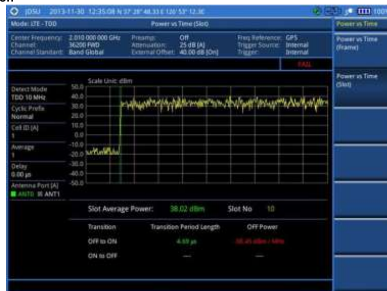
Figure 133 Power vs. time (slot) measurement with LTE – TDD signal analyzer
