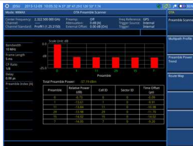
Figure 247 Preamble scanner measurement with Mobile WiMAX OTA signal analyzer
