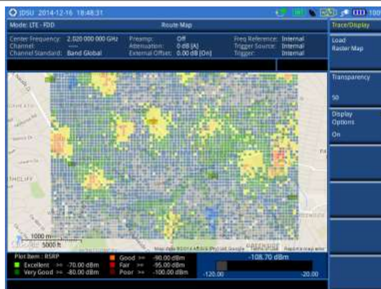
Figure 117 Raster image overlaid on the route map in LTE-FDD OTA signal analyzer
