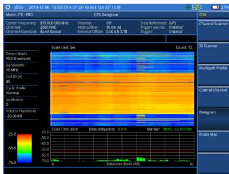
Figure 115 Datagram measurement with LTE - FDD signal analyzer
