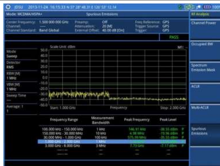
Figure 65 Spurious emissions measurement with WCDMA/HSPA+ signal analyzer
