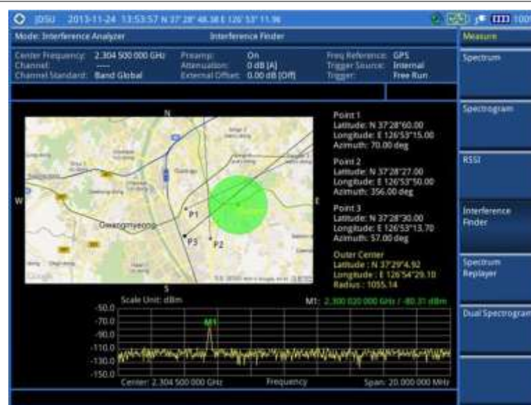
Figure 33 Interference finder measurement in map view
