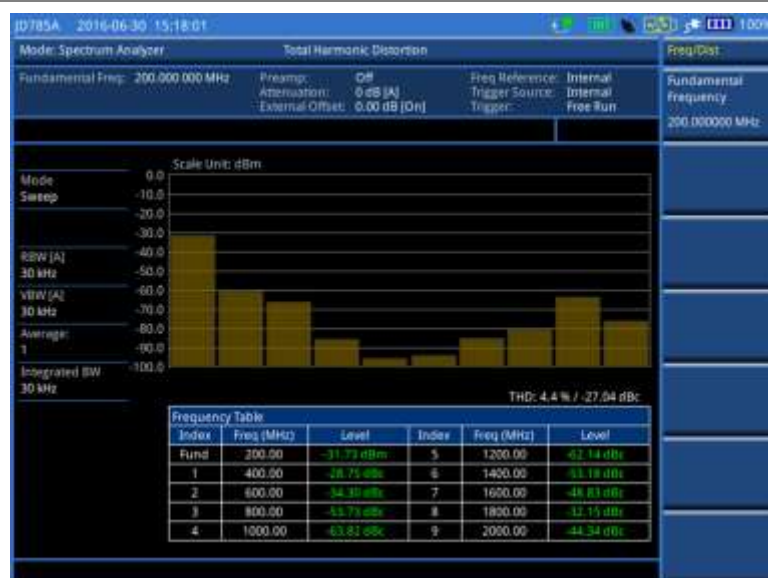
Figure 25 Total harmonic distortion screen
