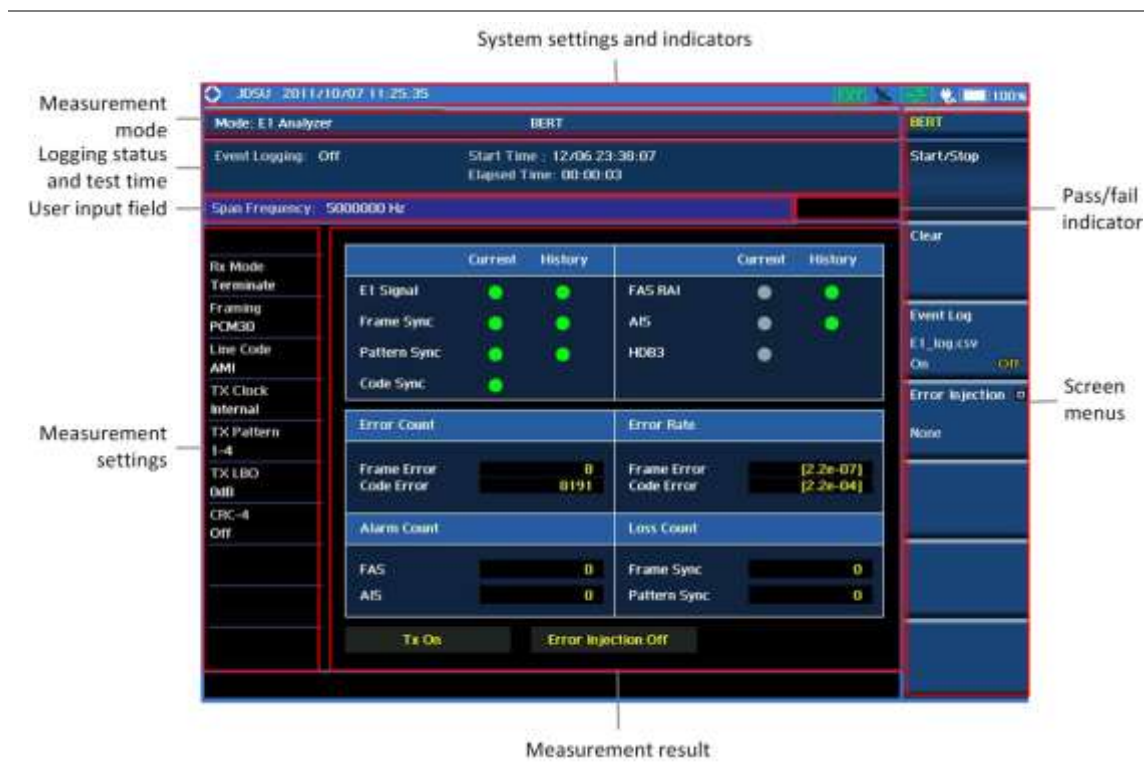
Figure 272 E1 analyzer screen
