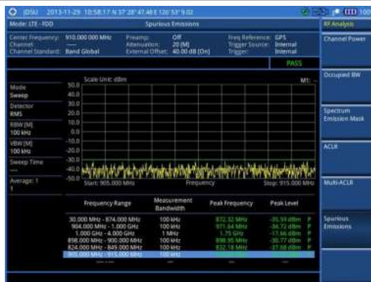
Figure 90 Spurious emissions measurement with LTE - FDD signal analyzer
