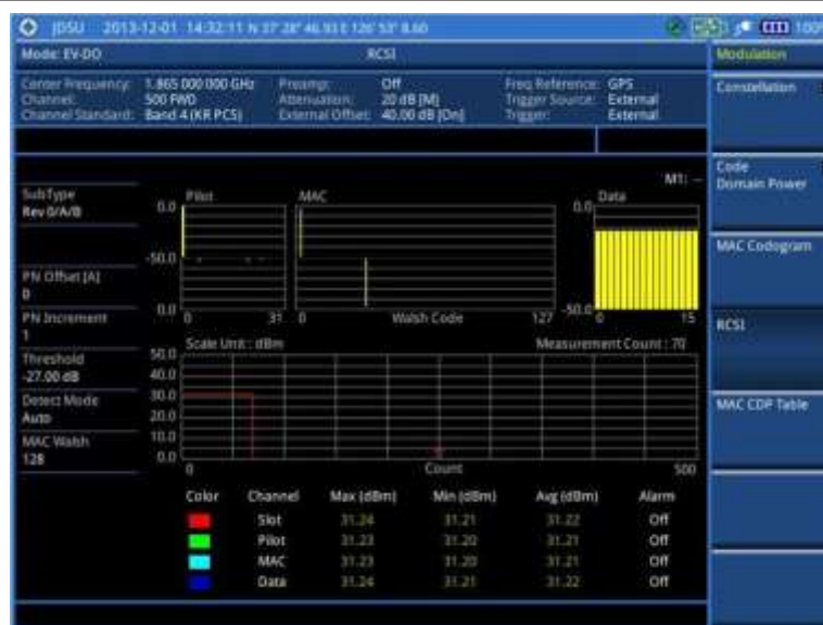
Figure 198 RCSI measurement with EV-DO signal analyzer
