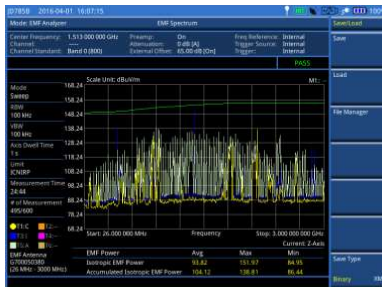
Figure 309 EMF spectrum measurement with EMF analyzer
