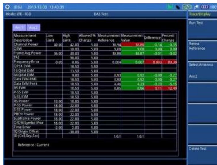
Figure 107 DAS measurement with LTE - FDD signal analyzer
