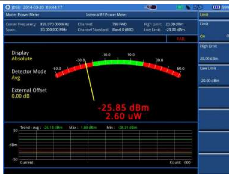
Figure 298 Internal power measurement
