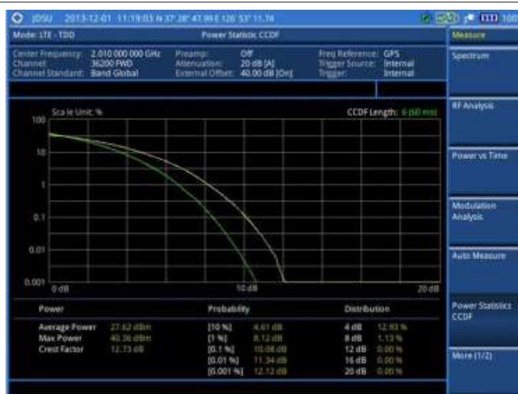
Figure 147 CCDF measurement with LTE - TDD signal analyzer
