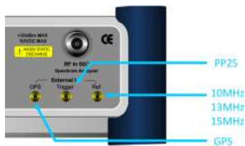
Figure 83 Connection ports for external reference clock
