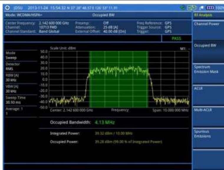
Figure 61 Occupied bandwidth measurement with WCDMA/HSPA+ signal analyzer
