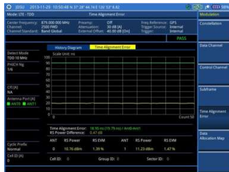
Figure 143 Time alignment error measurement with LTE - TDD signal analyzer
