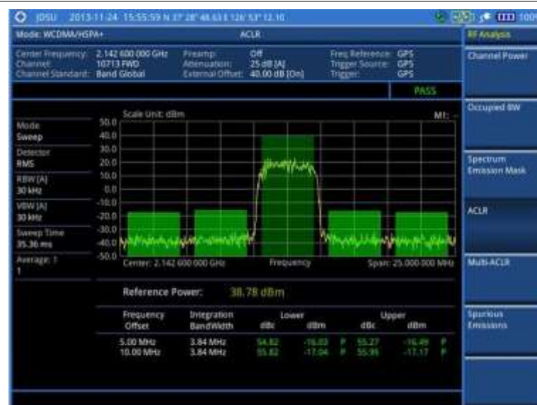
Figure 63 ACLR measurement with WCDMA/HSPA+ signal analyzer
