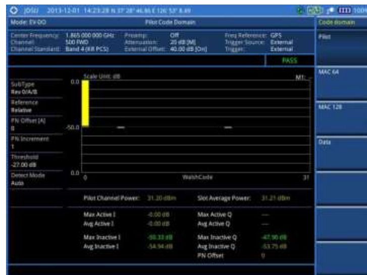
Figure 196 Code domain power measurement with EV-DO signal analyzer
