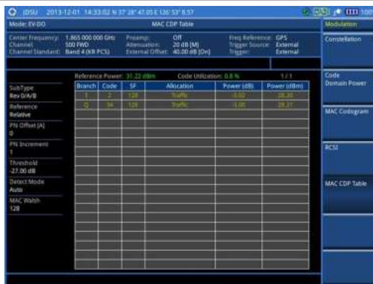
Figure 199 MAC CDP Table measurement with EV-DO signal analyzer
