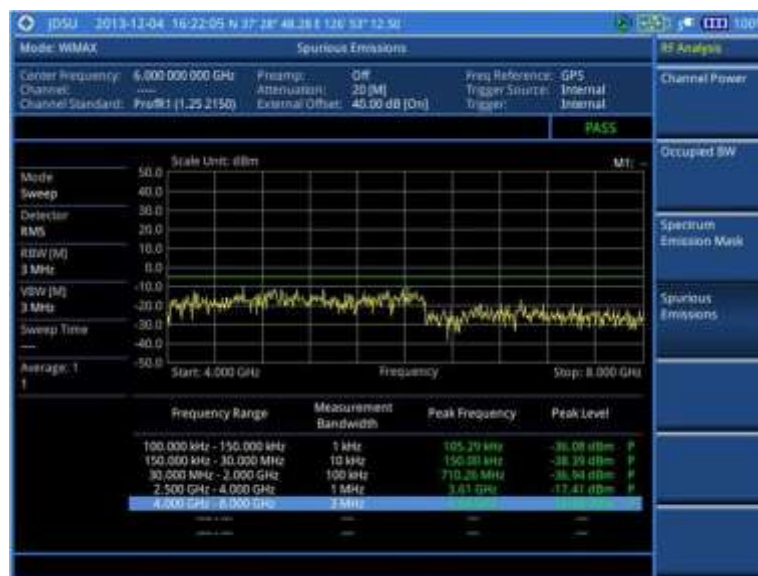
Figure 240 Spurious emissions measurement with Mobile WiMAX signal analyzer
