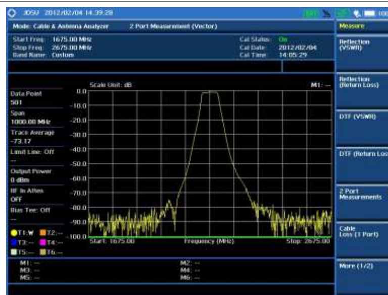
Figure 270 2-port vector measurement
