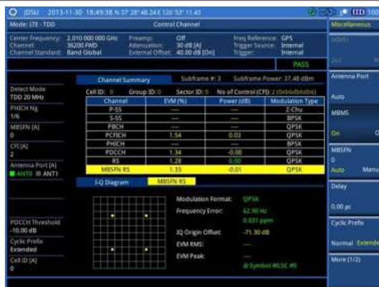
Figure 140 Control channel measurement with LTE - TDD signal analyzer (MBMS On)
