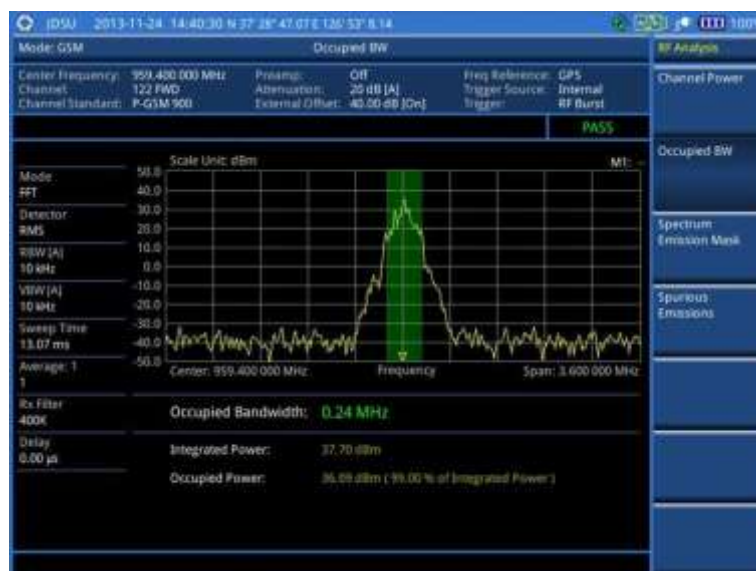
Figure 43 Occupied bandwidth measurement with GSM signal analyzer
