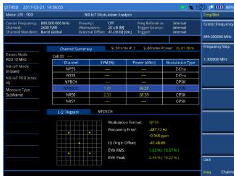
Figure 120 NB-IoT modulation measurement with LTE-FDD signal analyzer (Subframe 2)
