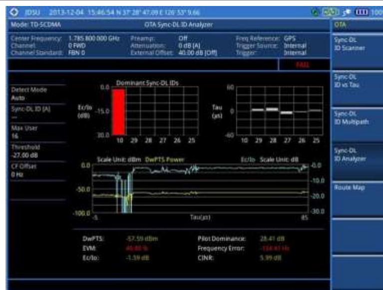
Figure 229 Sync-DL ID analyzer measurement with TD-SCDMA OTA signal analyzer
