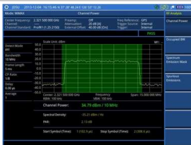
Figure 237 Channel power measurement with Mobile WiMAX signal analyzer
