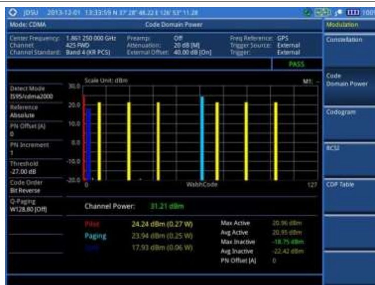
Figure 171 Code domain power measurement with CDMA signal analyzer
