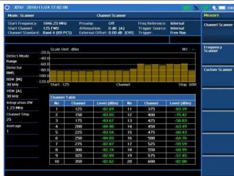
Figure 292 Channel scanner measurement
