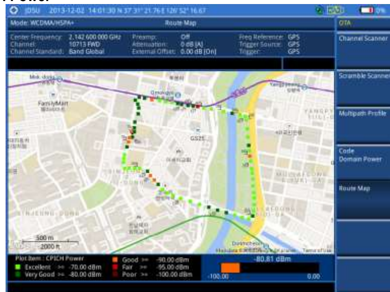
Figure 77 Route map measurement with WCDMA/HSPA+ OTA signal analyzer
