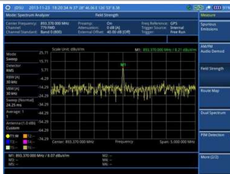
Figure 19 Field strength measurement with spectrum analyzer
