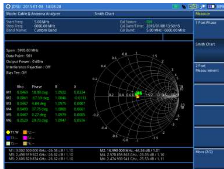
Figure 269 Smith chart measurement
