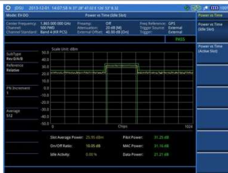
Figure 193 Power vs. time (idle slot) measurement with EV-DO signal analyzer
