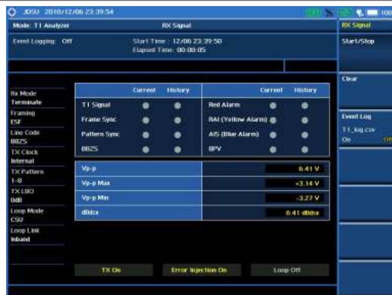
Figure 286 T1 RX signal testing
