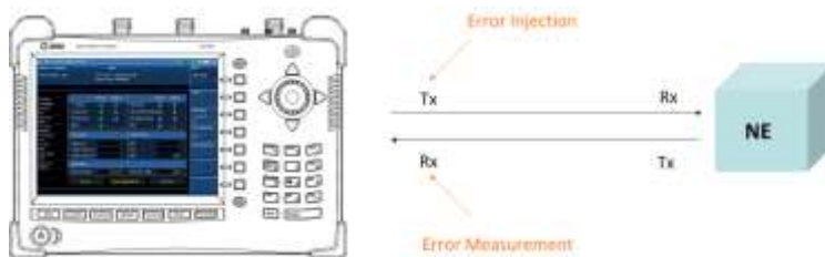
Figure 275 Error injection and measurement connection
