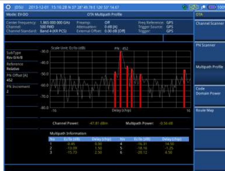
Figure 203 Multipath profile measurement with EV-DO OTA signal analyzer
