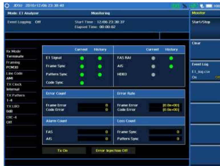
Figure 277 E1 transmission monitoring for framing PCM30
