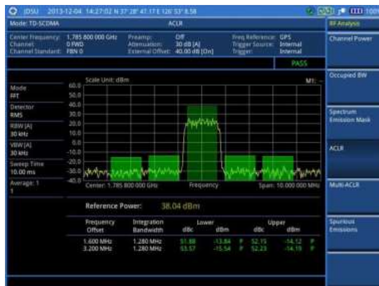
Figure 215 ACLR measurement with TD-SCDMA signal analyzer
