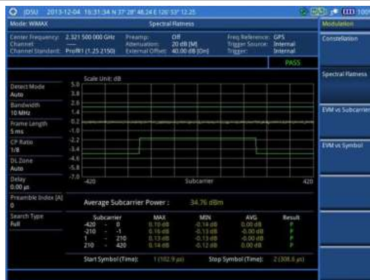
Figure 243 Spectral flatness measurement with Mobile WiMAX signal analyzer
