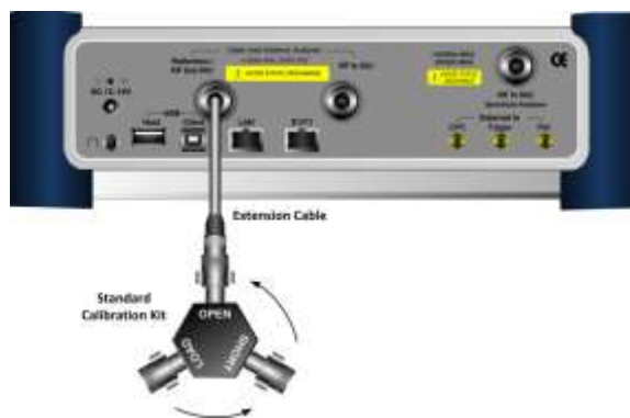
Figure 252 1-port calibration connection with mechanical Y-Cal kit
