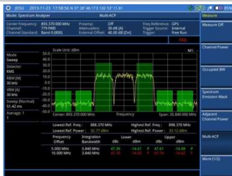
Figure 16 Multi-ACP measurement with spectrum analyzer
