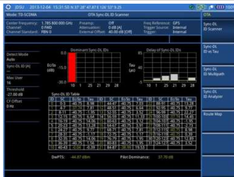
Figure 226 Sync-DL ID scanner measurement with TD-SCDMA OTA signal analyzer
