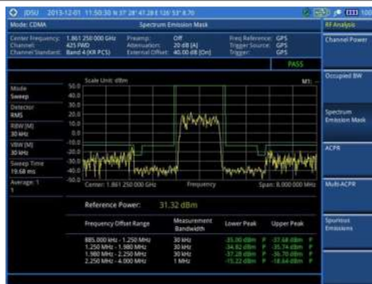
Figure 166 SEM measurement with CDMA signal analyzer
