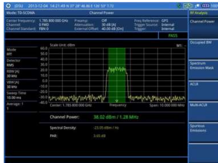
Figure 212 Channel power measurement with TD-SCDMA signal analyzer
