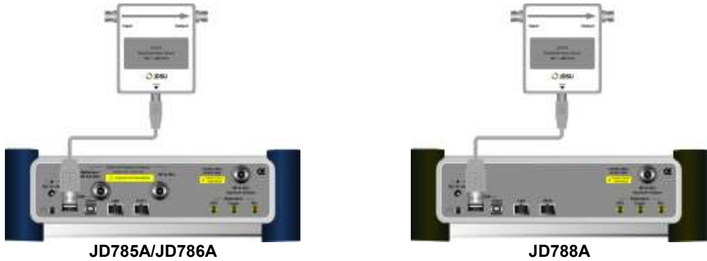
Figure 299 Directional power sensor connection
