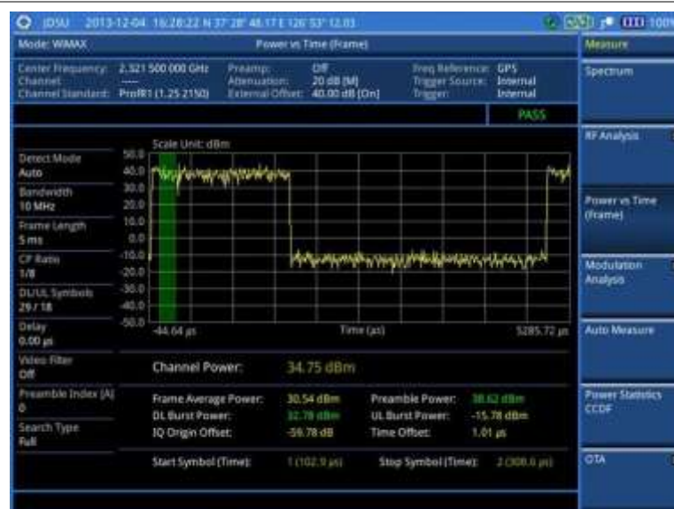
Figure 241 Power vs. time (frame) measurement with Mobile WiMAX signal analyzer
