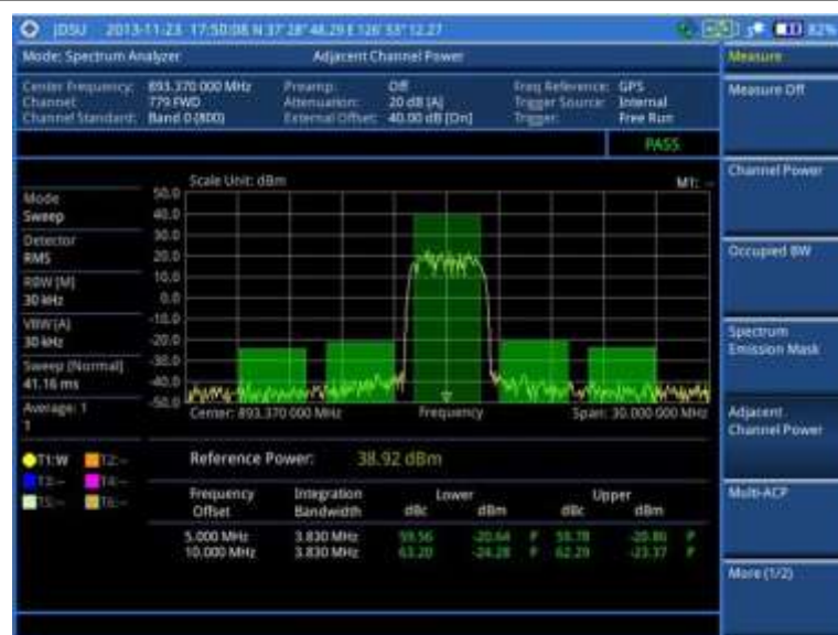
Figure 15 Adjacent channel power measurement with spectrum analyzer
