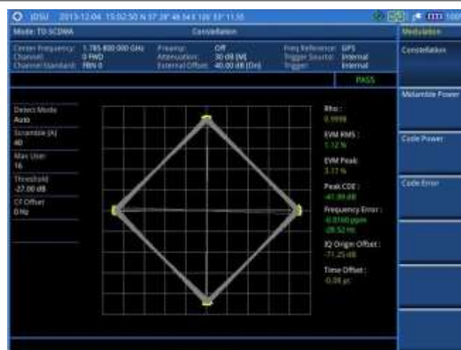
Figure 222 Constellation measurement with TD-SCDMA signal analyzer
