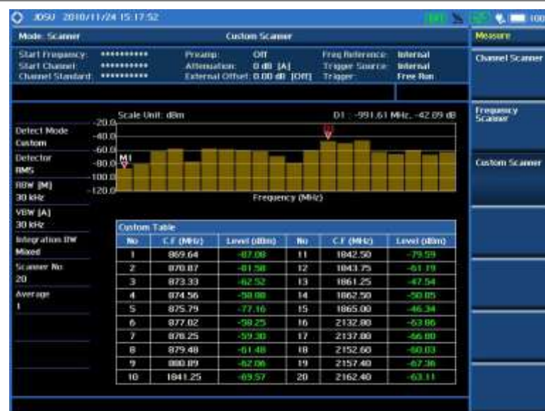
Figure 294 Custom scanner measurement
