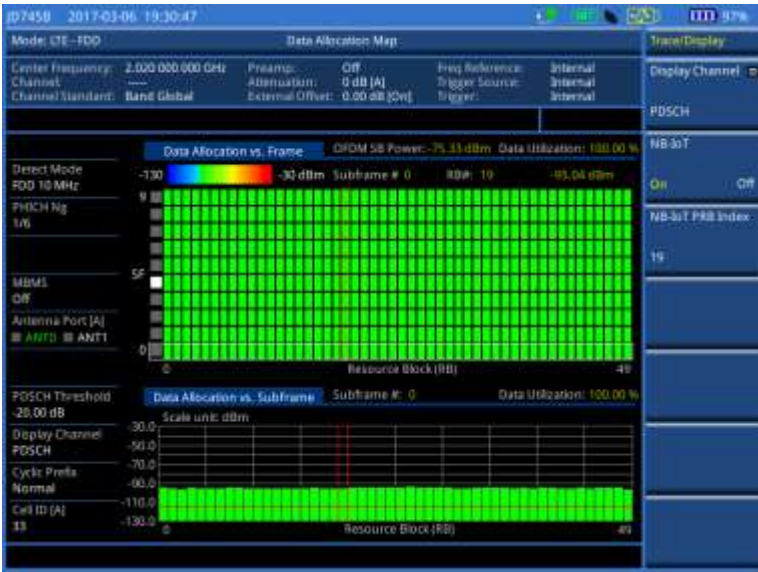
Figure 106 Data allocation map measurement with LTE - FDD signal analyzer (NB-IoT On)
