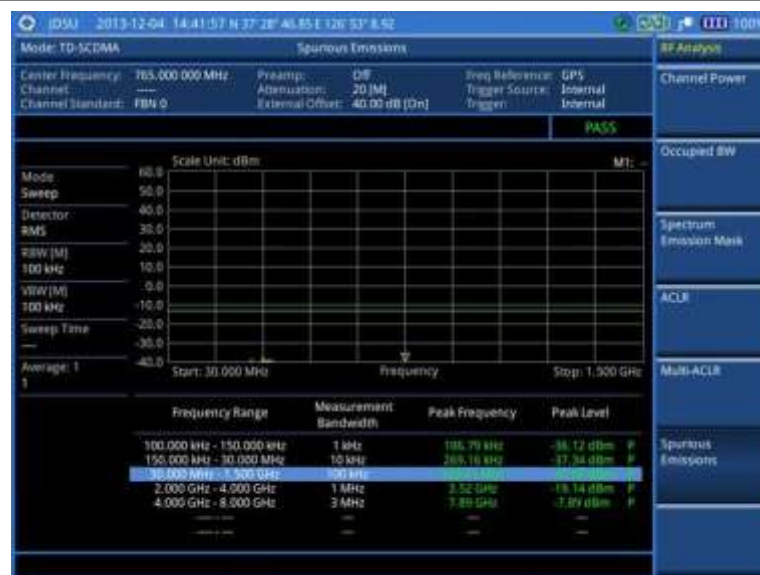
Figure 217 Spurious emissions measurement with TD-SCDMA signal analyzer
