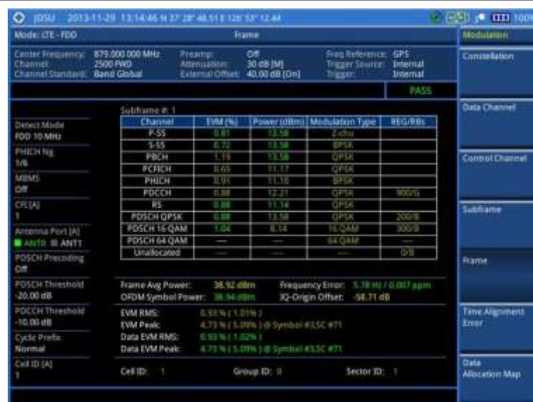
Figure 101 Frame measurement with LTE - FDD signal analyzer
