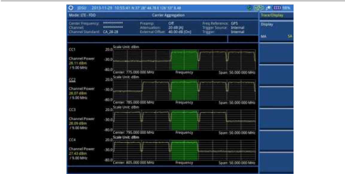
Figure 110 Carrier aggregation measurement with LTE - FDD signal analyzer (SA)
