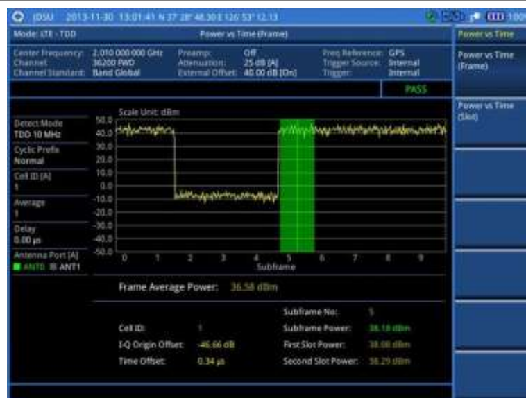
Figure 134 Power vs. time (frame) measurement with LTE – TDD signal analyzer
