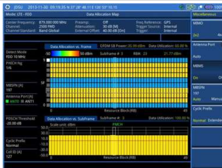
Figure 105 Data allocation map measurement with LTE - FDD signal analyzer (MBMS On)
