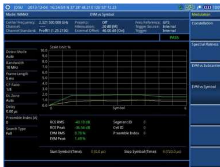
Figure 245 EVM vs. symbol measurement with Mobile WiMAX signal analyzer
