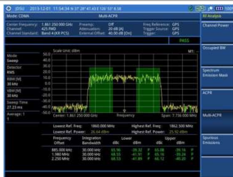
Figure 168 Multi-ACPR measurement with CDMA signal analyzer
