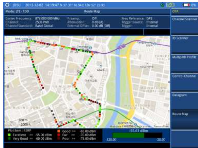
Figure 155 Route map measurement with LTE - TDD OTA signal analyzer
