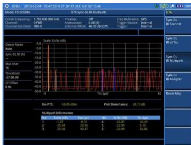
Figure 228 Sync-DL ID multipath measurement with TD-SCDMA OTA signal analyzer
