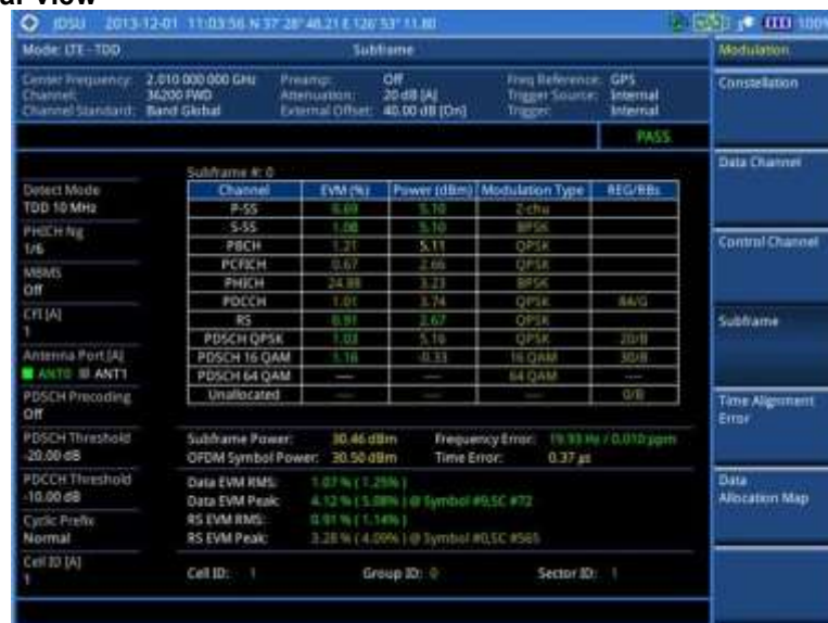
Figure 141 Subframe measurement with LTE - TDD signal analyzer
