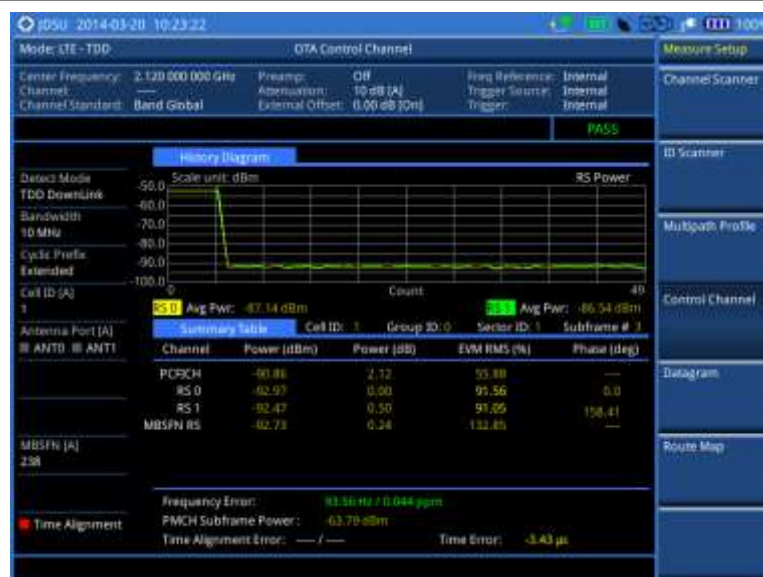
Figure 153 Control channel measurement with LTE - TDD OTA signal analyzer
