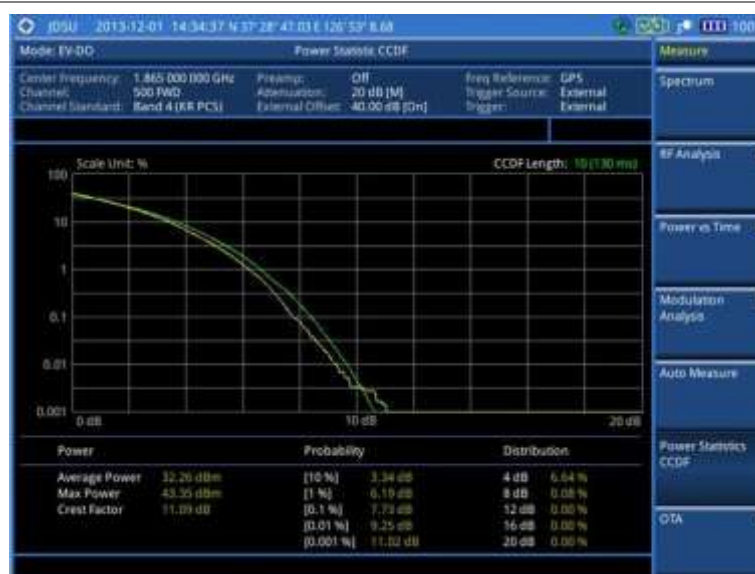
Figure 200 CCDF measurement with EV-DO signal analyzer
