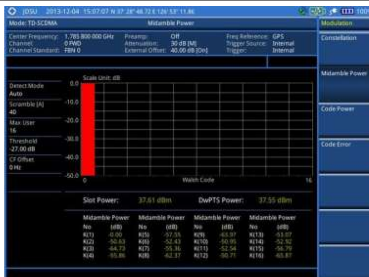
Figure 223 Midamble measurement with TD-SCDMA signal analyzer
