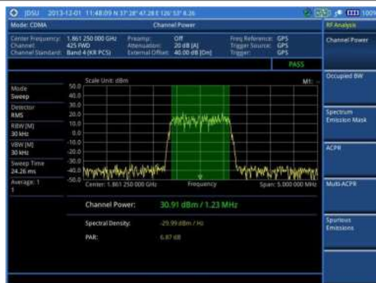
Figure 164 Channel power measurement with CDMA signal analyzer
