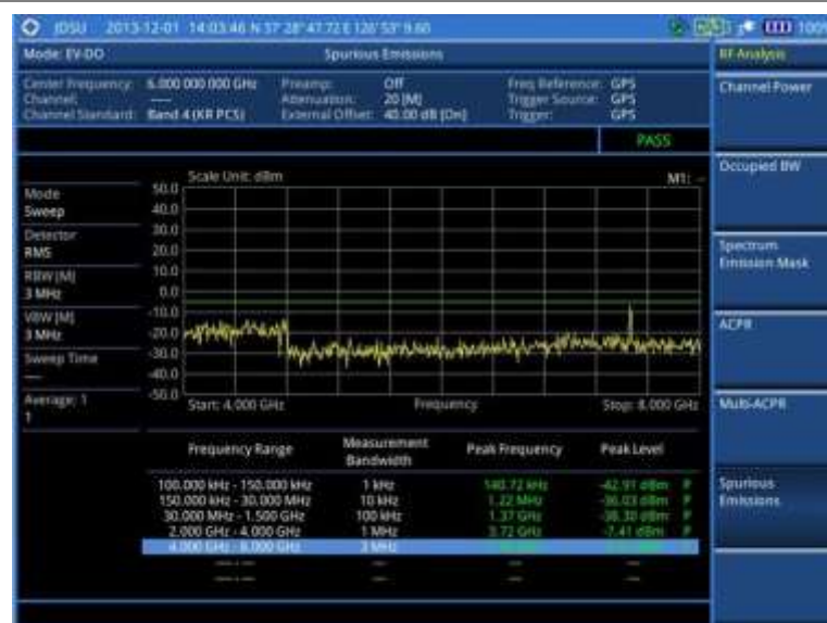
Figure 192 Spurious emissions measurement with EV-DO signal analyzer
