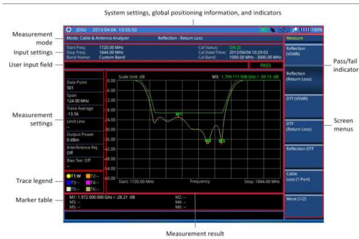
Figure 251 Reflection measurement screen
