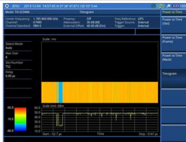
Figure 221 Timogram with TD-SCDMA signal analyzer
