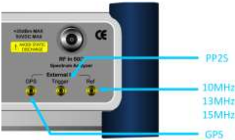
Figure 185 Connection ports for external reference clock
