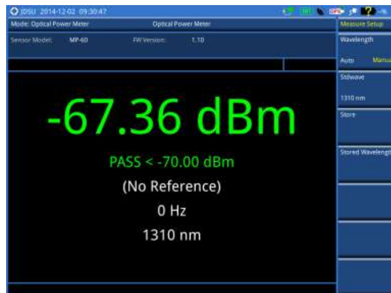
Figure 302 optical power measurement
