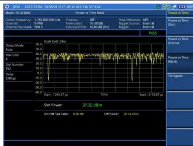
Figure 220 Power vs. time (mask) measurement with TD-SCDMA signal analyzer
