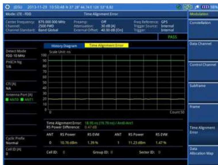
Figure 103 Time alignment error measurement with LTE - FDD signal analyzer
