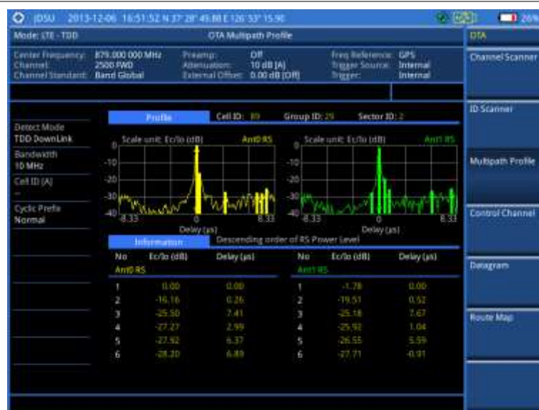
Figure 152 Multipath profile measurement with LTE - TDD OTA signal analyzer
