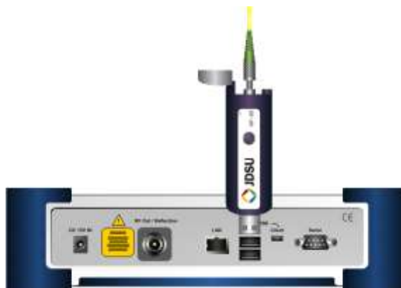
Figure 73 Cable connection diagram for optical power meter
