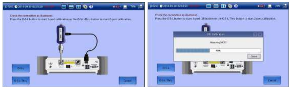
Figure 11 Electronic calibration on JD725C using EZ-Cal kit
