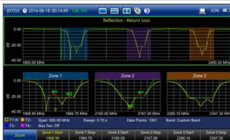
Figure 83 Reflection return loss measurement with zoom zones
