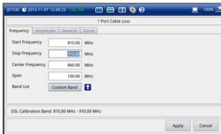
Figure 34 Frequency setup window for cable loss measurements
