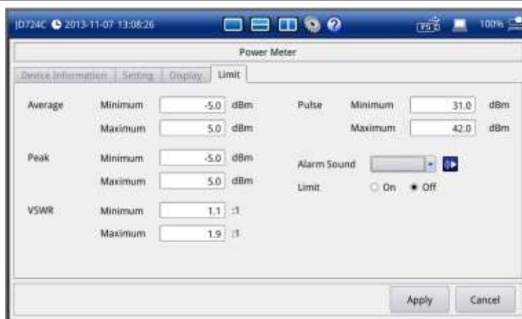
Figure 69 Limit setup window for RF power measurements
