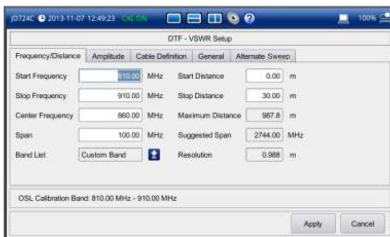
Figure 25 Frequency/distance setup window for DTF measurements
