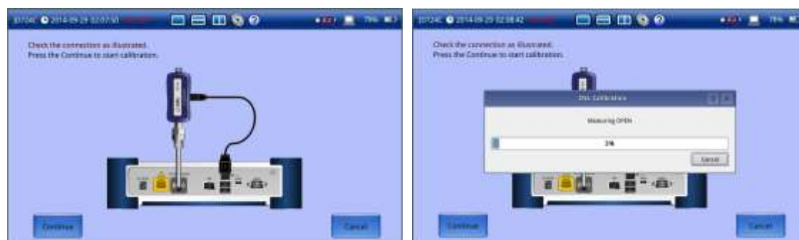
Figure 10 e-Calibration on JD724C using EZ-Cal kit
