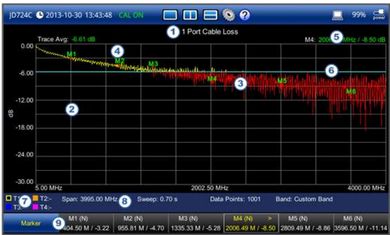
Figure 33 1 port cable loss measurement screen
