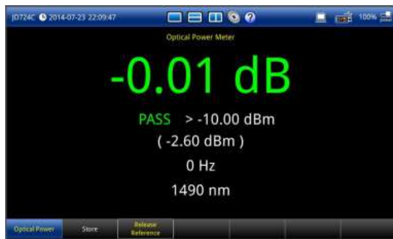
Figure 75 Relative optical power measurement vs. reference
