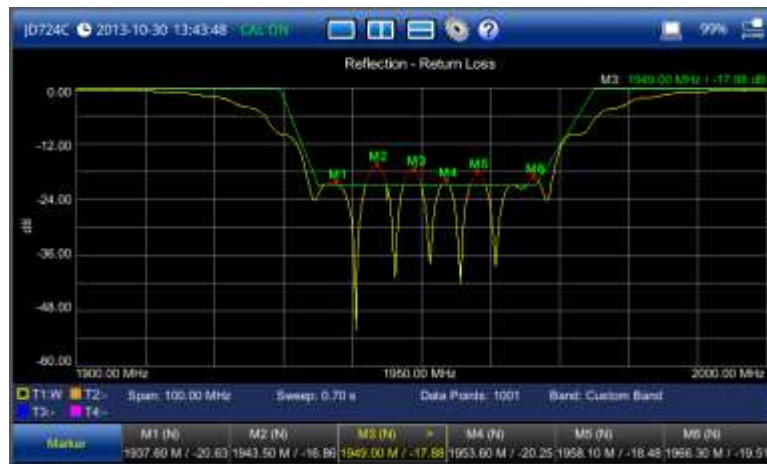
Figure 20 Reflection return loss measurement screen (single layout)
