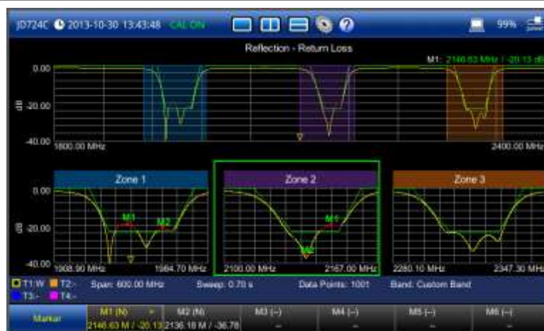
Figure 21 Reflection return loss measurement screen (zoom zones)
