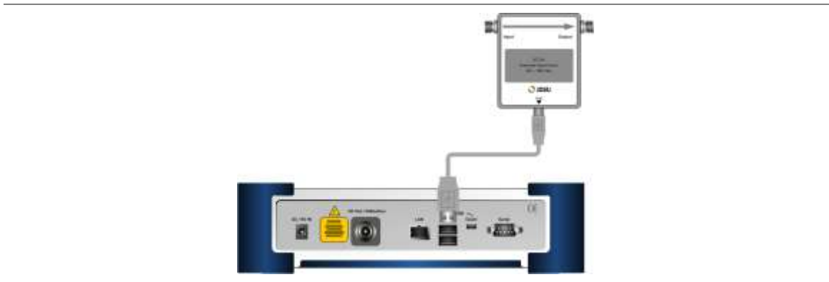
Figure 67 Cable connection diagram for directional power sensor
