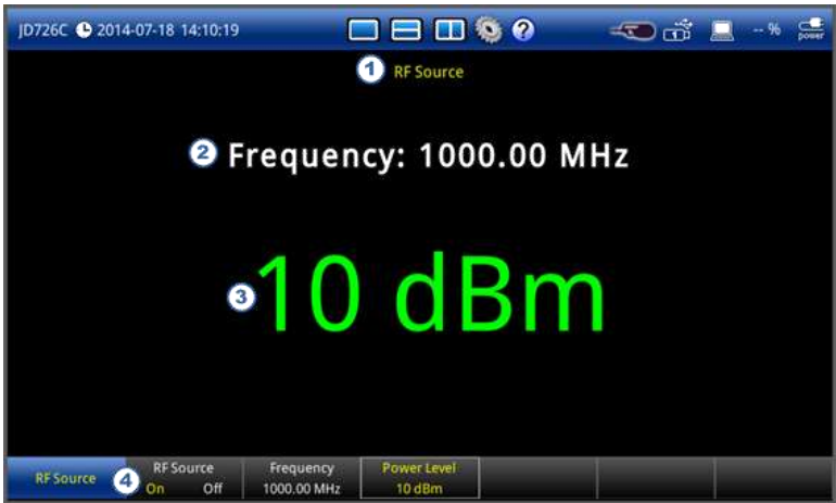
Figure 61 RF source screen
