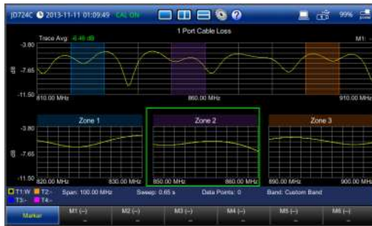
Figure 38 1 port cable loss measurement screen (zoom zones)
