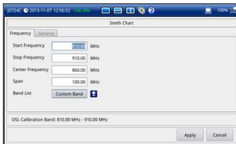
Figure 45 Frequency setup window for Smith chart measurements
