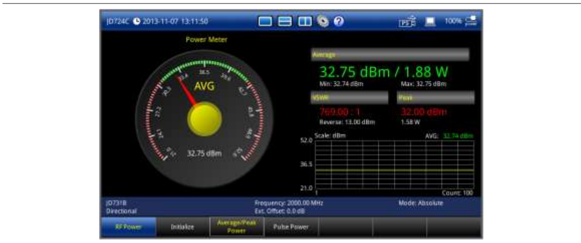
Figure 68 RF power measurement screen
