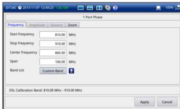
Figure 40 Frequency setup window for 1 port phase measurements
