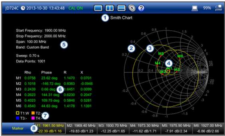
Figure 44 Smith chart measurement screen
