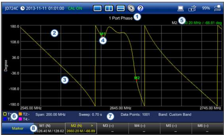
Figure 39 1 port phase measurement screen
