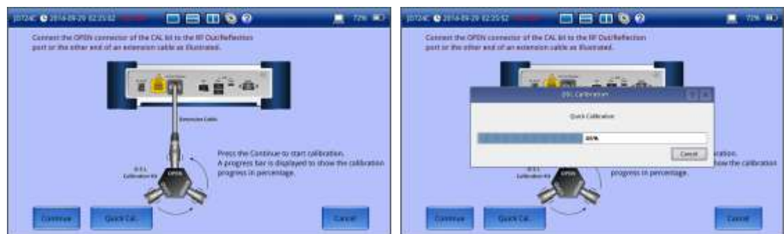
Figure 12 Quick calibration on JD724C
