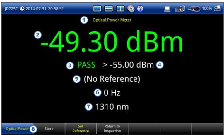
Figure 70 Optical power measurement screen
