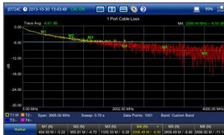
Figure 37 1 port cable loss measurement screen (single layout)
