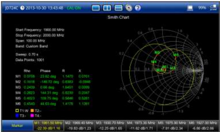
Figure 48 Smith chart measurement screen (single layout)
