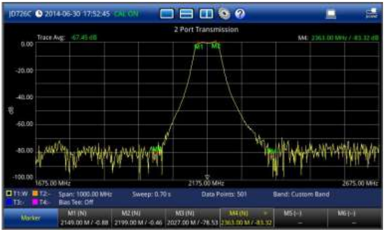
Figure 55 2 port transmission measurement screen (single layout)
