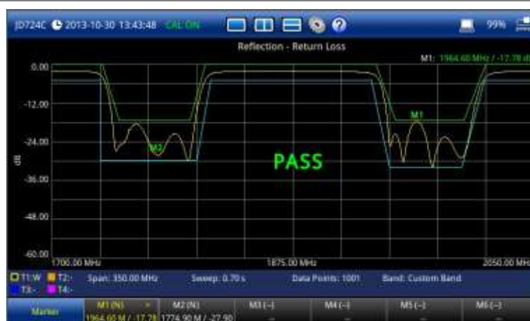
Figure 88 Upper and lower MSL line
