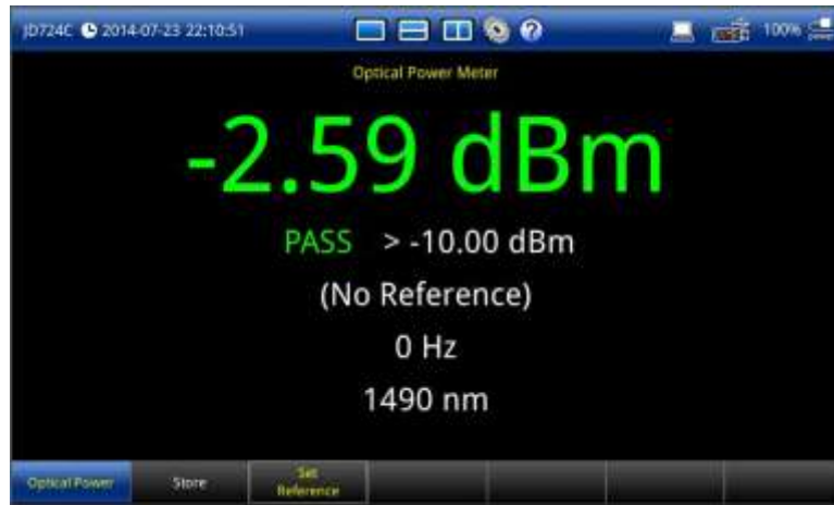
Figure 74 Absolute optical power measurement
