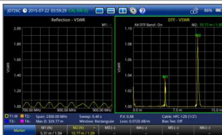
Figure 85 DTF VSWR measurement with alternate DTF band on
