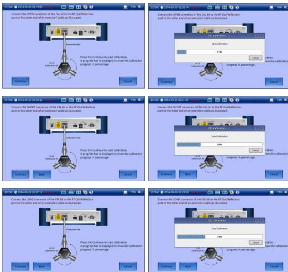
Figure 7 O-S-L calibration on JD724C using Y-Cal kit
