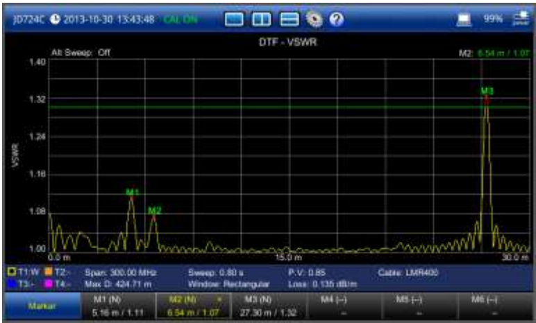
Figure 28 DTF VSWR measurement screen (single layout)
