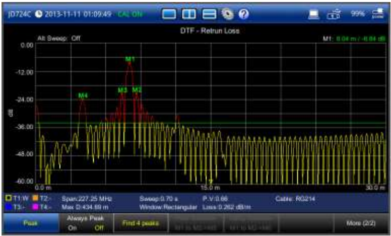
Figure 29 DTF return loss measurement screen (single layout)
