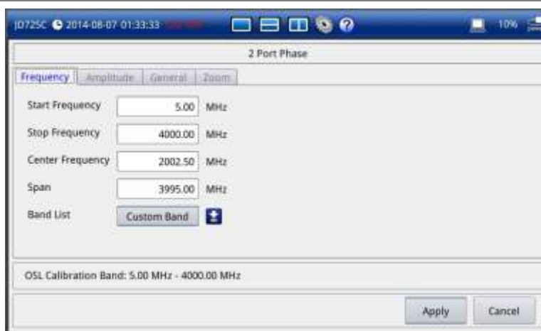
Figure 57 Frequency setup window for 2 port phase measurements
