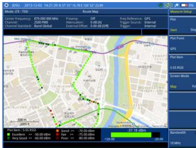
Figure 198 Route map measurement (S-SS RSSI) with LTE-TDD OTA signal analyzer
