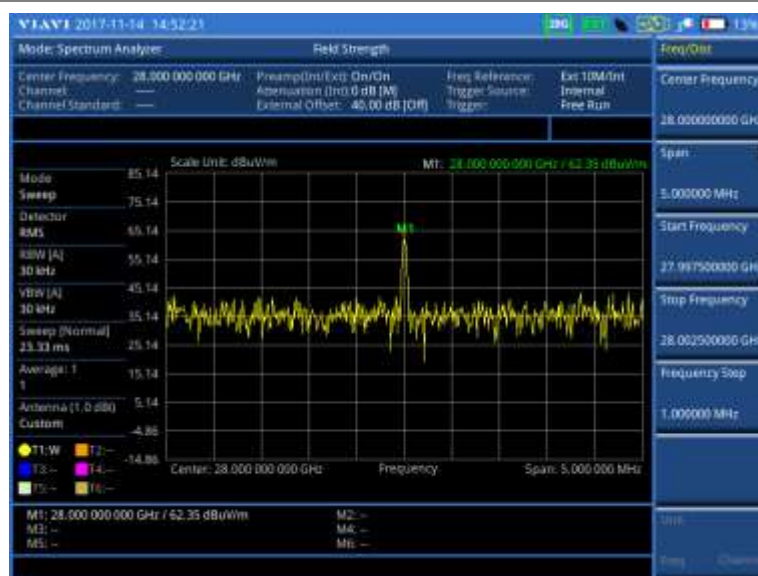
Figure 39 Field strength measurement with spectrum analyzer (on 28 GHz downconverter)
