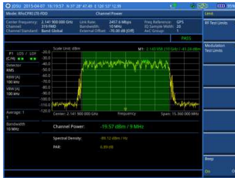
Figure 364 Channel power measurement with RFoCPRI LTE-FDD signal analyzer
