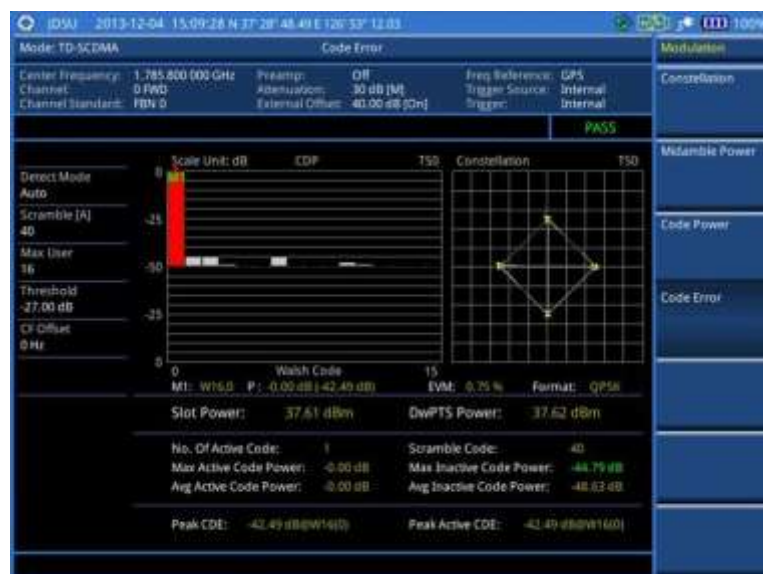
Figure 271 Code error measurement with TD-SCDMA signal analyzer
