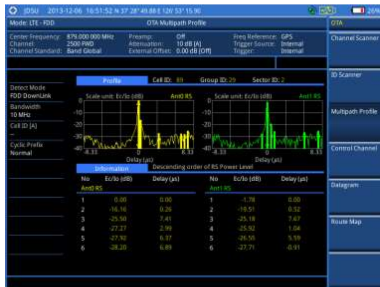
Figure 147 Multipath profile measurement with LTE-FDD OTA signal analyzer
