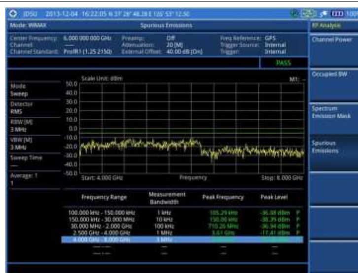
Figure 286 Spurious emissions measurement with Mobile WiMAX signal analyzer
