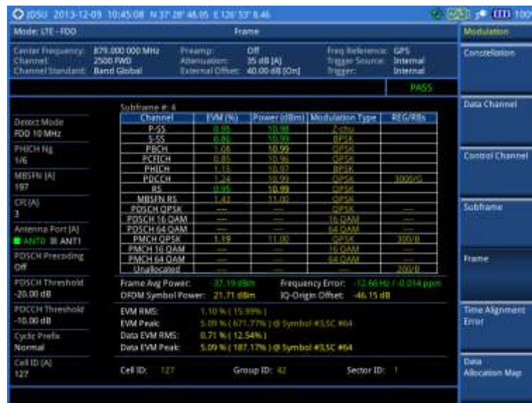
Figure 134 Frame measurement with LTE-FDD signal analyzer (MBMS On)
