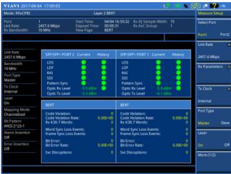
Figure 340 CPRI layer 2 BERT test
