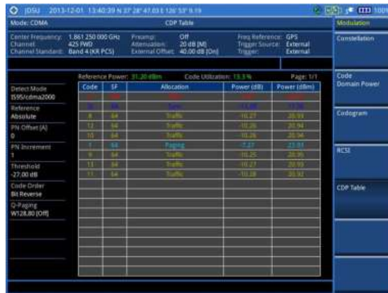
Figure 220 CDP Table measurement with CDMA signal analyzer
