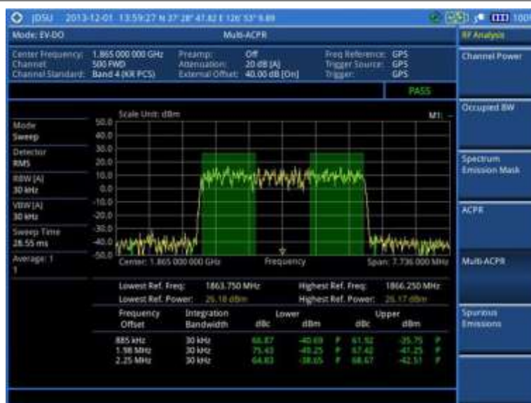
Figure 237 Multi-ACPR measurement with EV-DO signal analyzer
