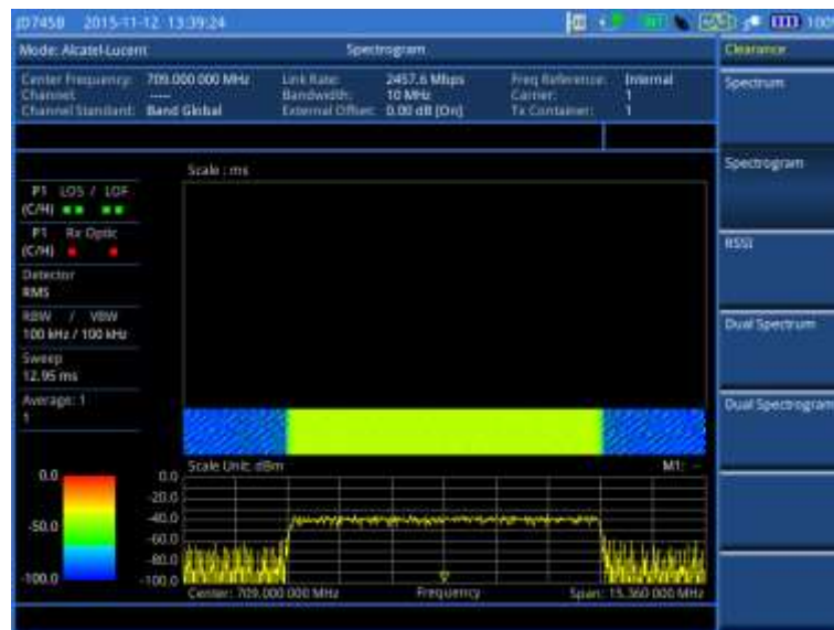
Figure 429 Example of spectrogram in Alcatel-Lucent BBU emulation
