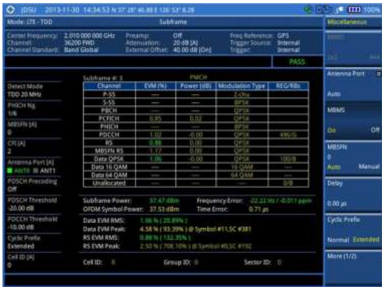
Figure 181 Subframe measurement with LTE-TDD signal analyzer (MBMS On)
