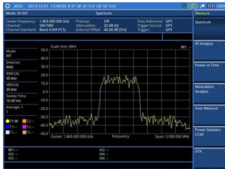
Figure 232 Spectrum measurement screen with EV-DO signal analyzer
