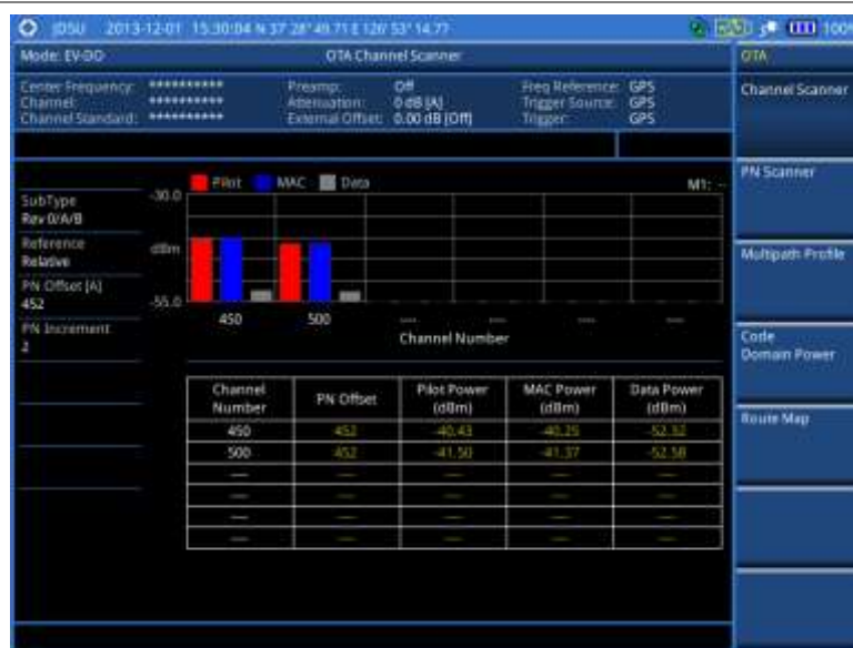
Figure 247 Channel scanner measurement with EV-DO OTA signal analyzer
