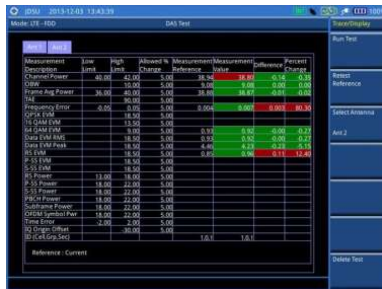
Figure 139 DAS measurement with LTE-FDD signal analyzer
