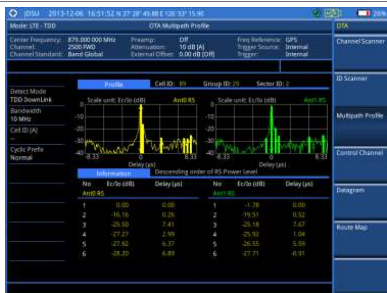
Figure 192 Multipath profile measurement with LTE-TDD OTA signal analyzer
