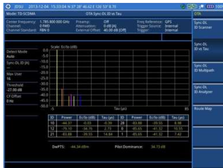
Figure 273 Sync-DL ID vs. Tau measurement with TD-SCDMA OTA signal analyzer
