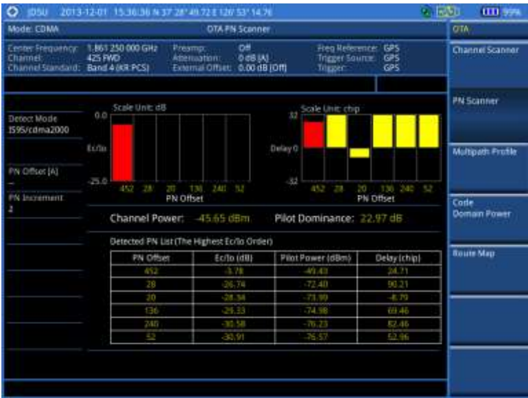
Figure 223 PN scanner measurement with CDMA OTA signal analyzer
