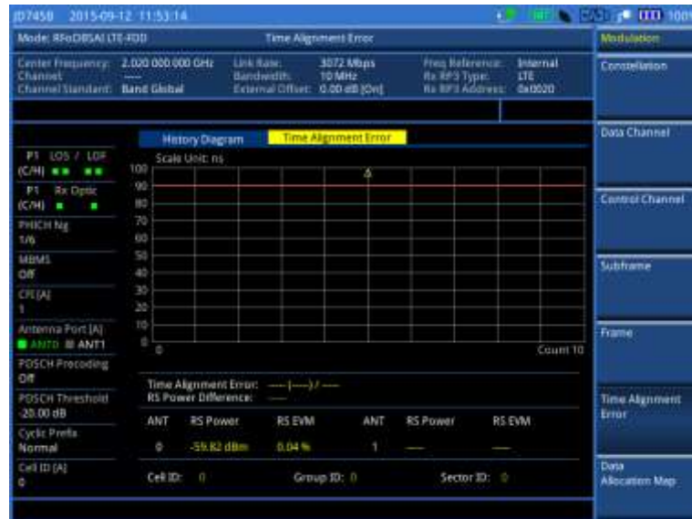
Figure 411 Time alignment error measurement with RFoBSAI LTE-FDD signal analyzer
