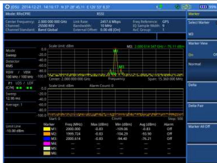
Figure 357 RFoCPRI interference measurement in RSSI
