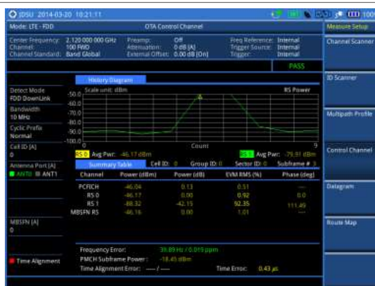
Figure 148 Control channel measurement with LTE-FDD OTA signal analyzer
