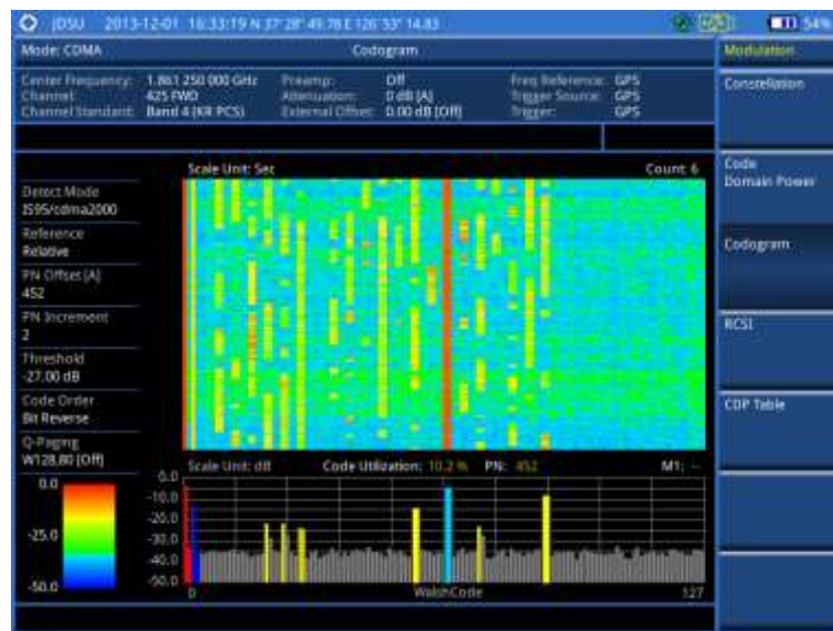
Figure 218 Codogram in full view with CDMA signal analyzer
