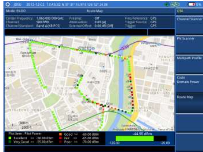
Figure 251 Route map measurement with EV-DO OTA signal analyzer
