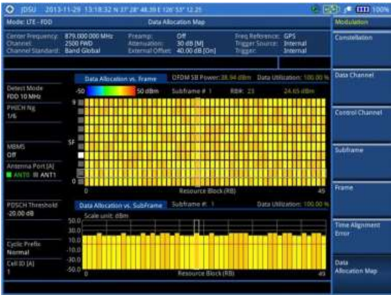
Figure 137 Data allocation map measurement with LTE-FDD signal analyzer (MBMS On)
