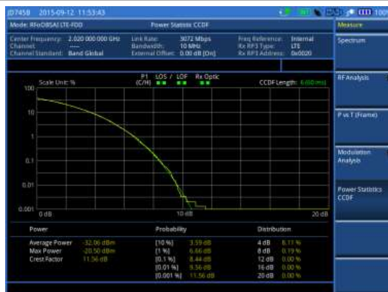
Figure 413 CCDF measurement with RFoBSAI LTE-FDD signal analyzer
