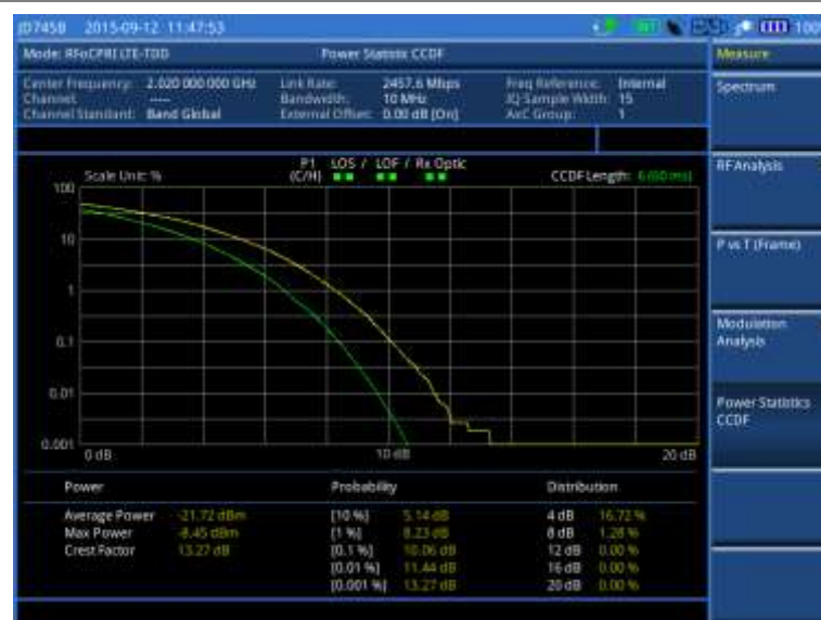
Figure 387 CCDF measurement with RFoCPRI LTE-TDD signal analyzer
