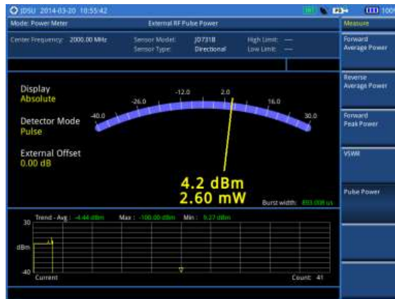
Figure 455 External power measurement of pulse power
