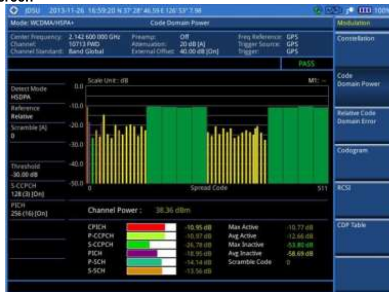
Figure 97 Code domain power measurement with WCDMA/HSPA+ signal analyzer
