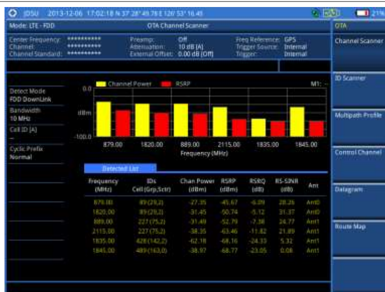
Figure 145 Channel scanner measurement with LTE-FDD OTA signal analyzer
