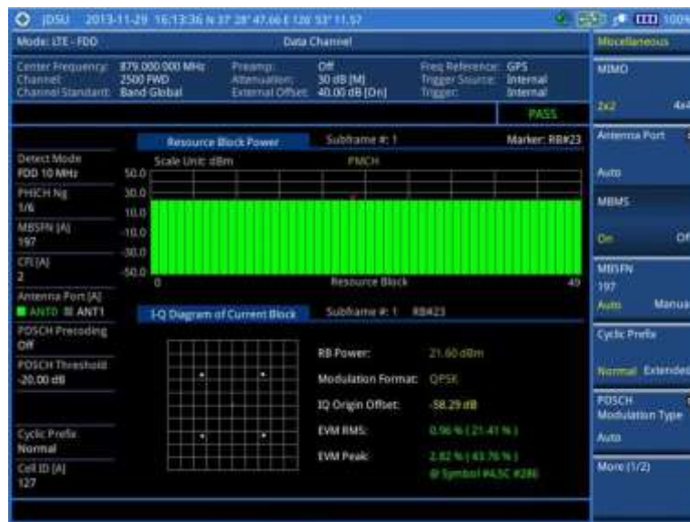
Figure 126 Data channel measurement with LTE-FDD signal analyzer (MBMS On)
