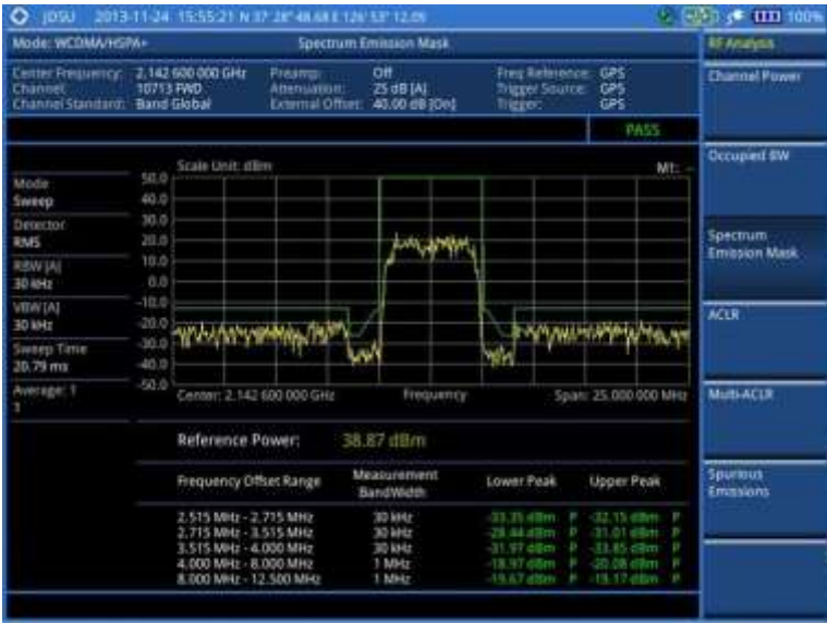
Figure 92 SEM measurement with WCDMA/HSPA+ signal analyzer
