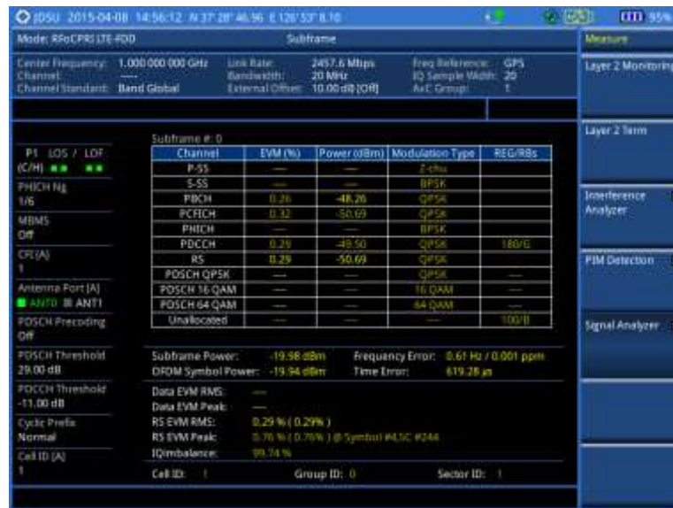
Figure 371 Subframe measurement (regular view) with RFoCPRI LTE-FDD signal analyzer
