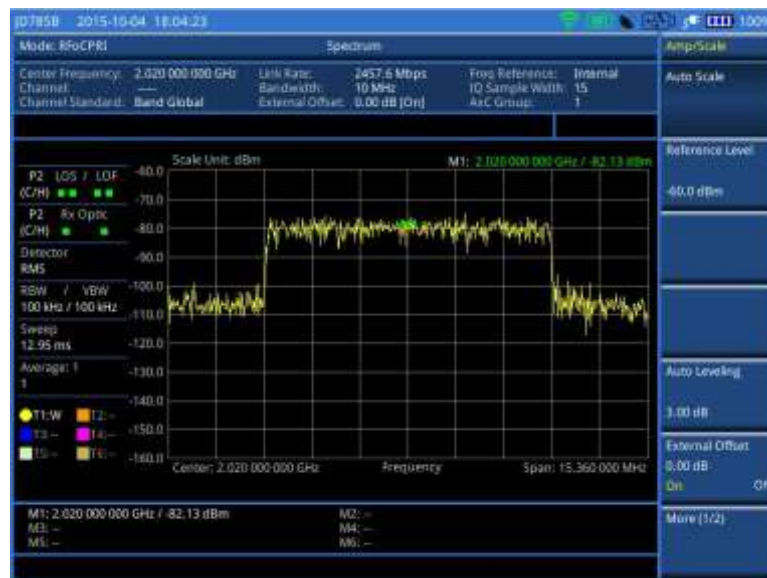
Figure 342 Before enabling Auto Leveling
