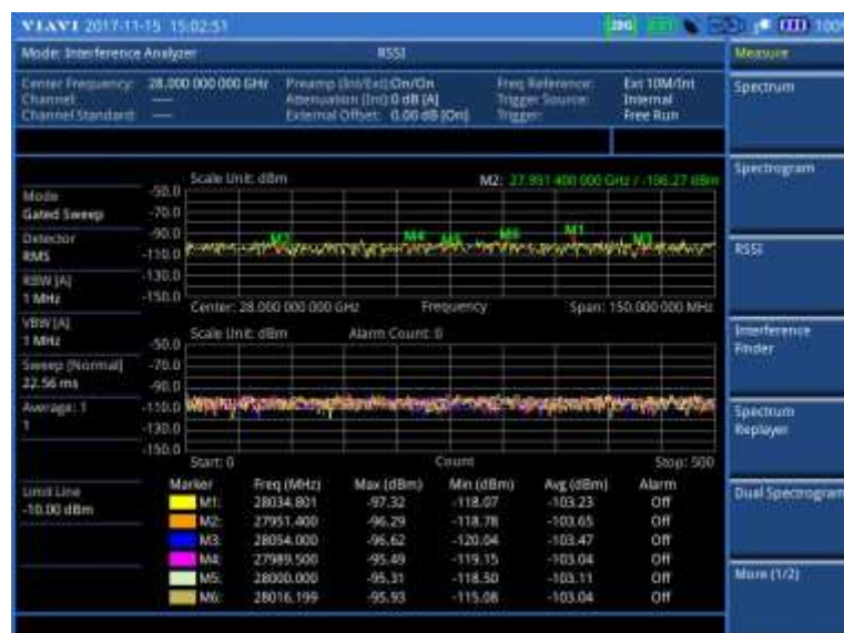
Figure 56 Interference measurement in RSSI (on 28 GHz downconverter)
