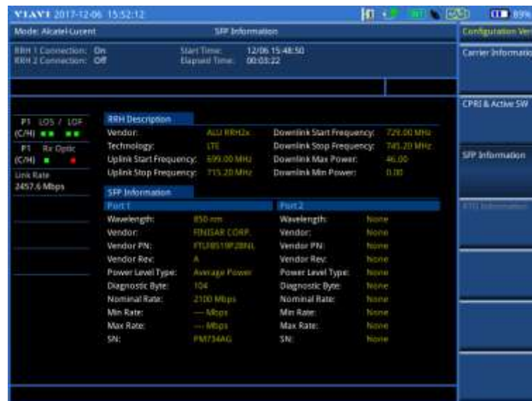
Figure 423 Example of verification of SFP information
