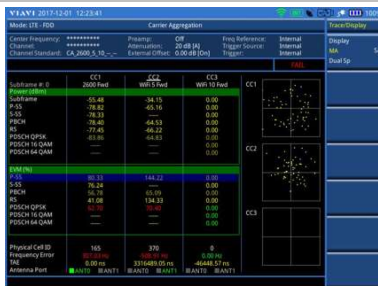
Figure 142 Carrier aggregation measurement with LTE-FDD signal analyzer (MA)
