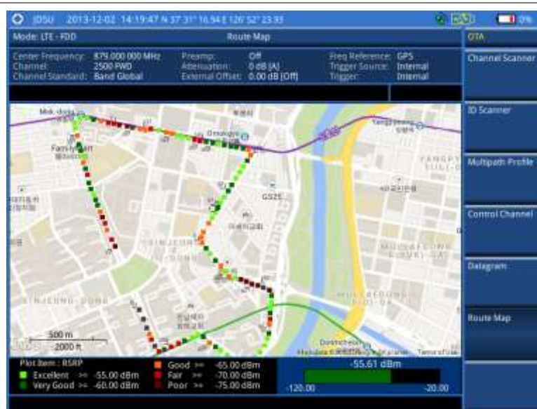
Figure 150 Route map measurement (RSRP) with LTE-FDD OTA signal analyzer
