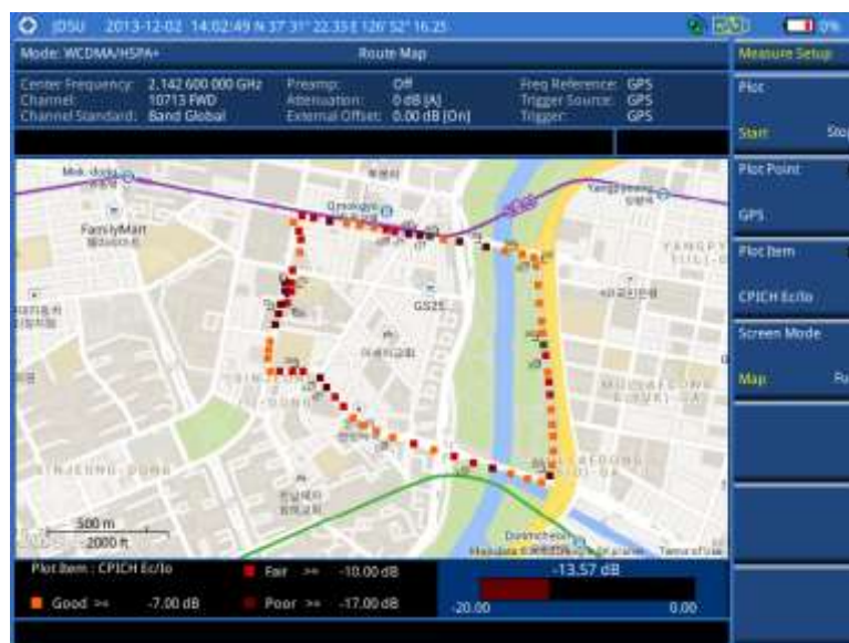
Figure 108 Route map measurement (CPICH Ec/Io) with WCDMA/HSPA+ OTA signal analyzer
