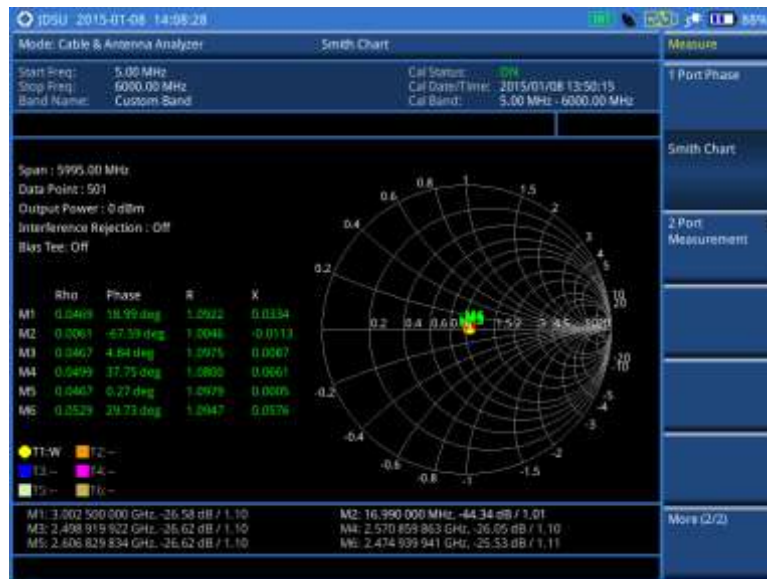
Figure 331 Smith chart measurement
