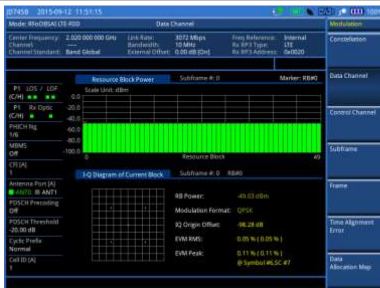
Figure 406 Data channel measurement with RFoBSAI LTE-FDD signal analyzer
