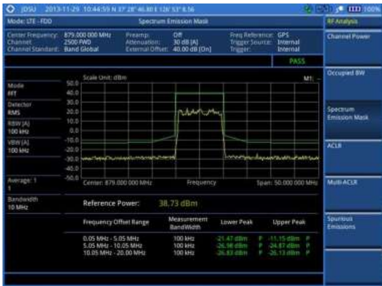
Figure 118 SEM measurement with LTE-FDD signal analyzer
