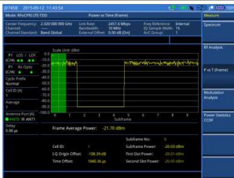
Figure 380 Power vs. time (frame) measurement with RFoCPRI LTE-TDD signal analyzer
