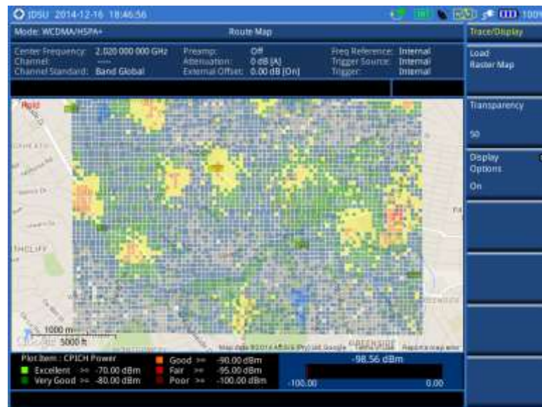
Figure 109 Raster image overlaid on the base map in WCDMA/HSPA+ OTA signal analyzer
