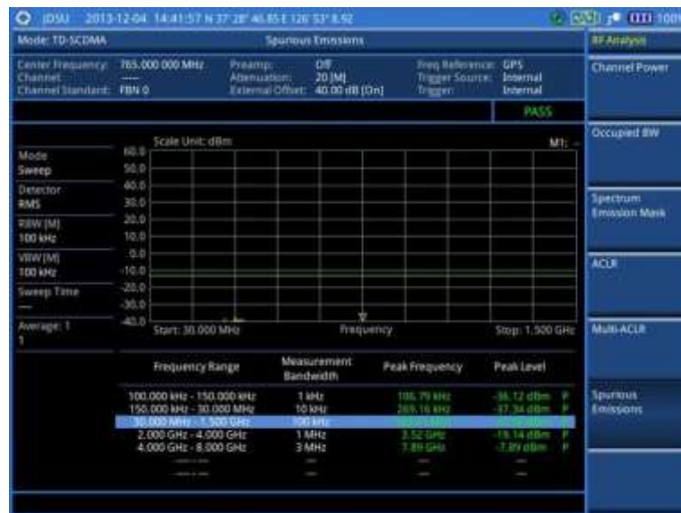
Figure 263 Spurious emissions measurement with TD-SCDMA signal analyzer
