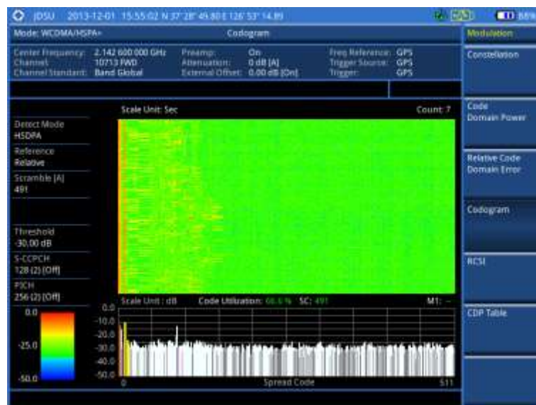
Figure 99 Codogram in full view with WCDMA/HSPA+ signal analyzer
