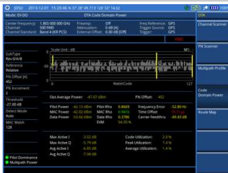
Figure 250 Code domain power measurement with EV-DO OTA signal analyzer
