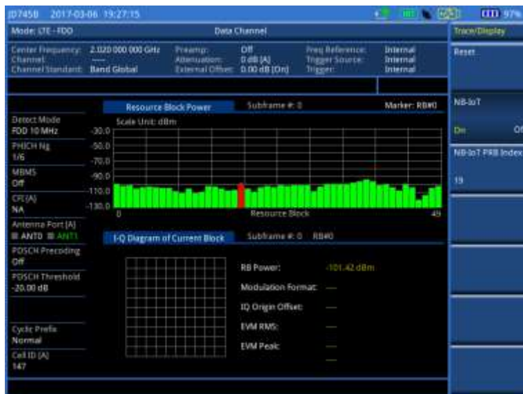
Figure 127 Data channel measurement with LTE-FDD signal analyzer (NB-IoT On)
