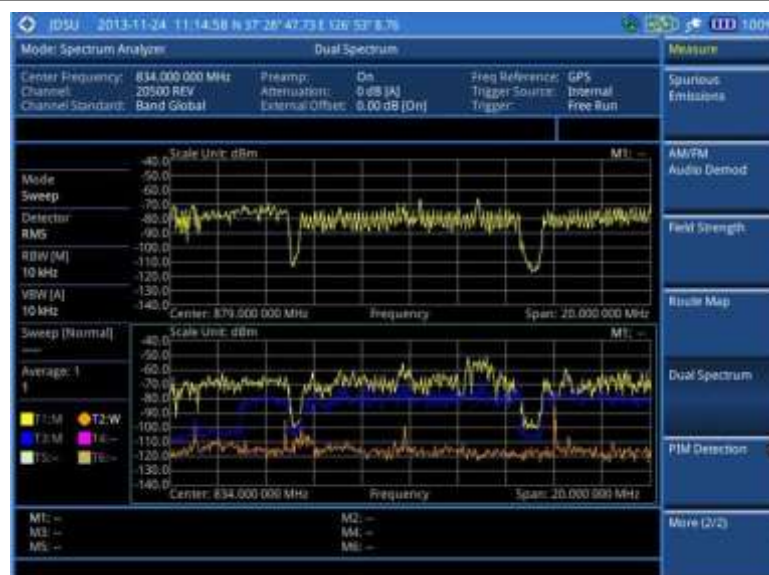
Figure 42 Dual spectrum measurement with spectrum analyzer
