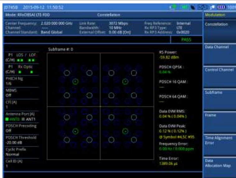
Figure 405 Constellation measurement with RFoBSAI LTE-FDD signal analyzer
