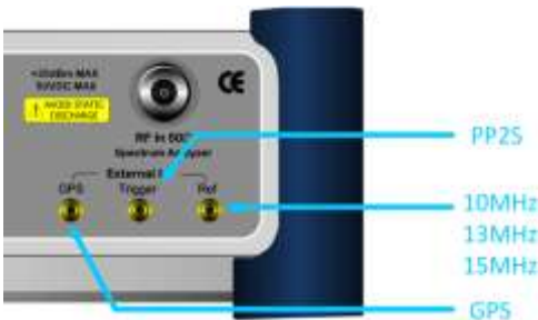
Figure 114 Connection ports for external reference clock
