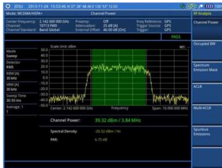
Figure 90 Channel power measurement with WCDMA/HSPA+ signal analyzer
