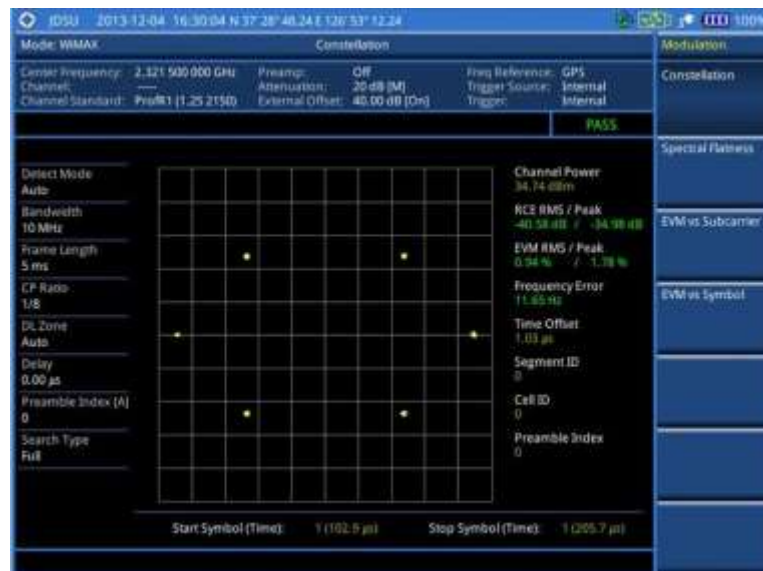
Figure 288 Constellation measurement with Mobile WiMAX signal analyzer
