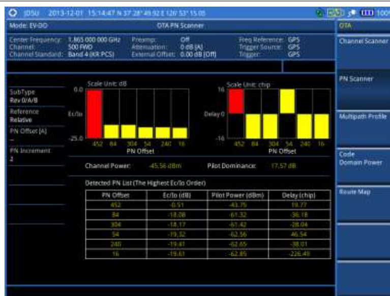
Figure 248 PN scanner measurement with EV-DO OTA signal analyzer
