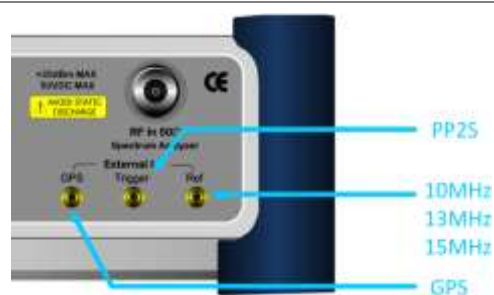
Figure 208 Connection ports for external reference clock
