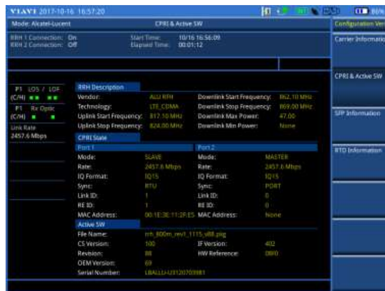
Figure 422 Example of verification of CPRI state and active software
