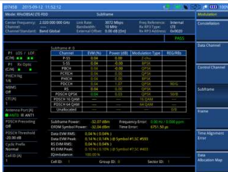
Figure 409 Subframe measurement with RFoBSAI LTE-FDD signal analyzer
