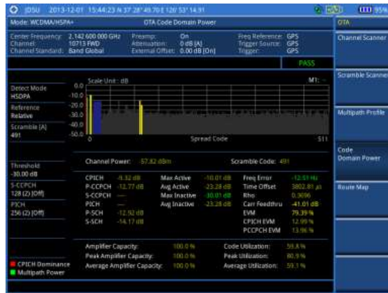
Figure 106 Code domain power measurement with WCDMA/HSPA+ OTA signal analyzer
