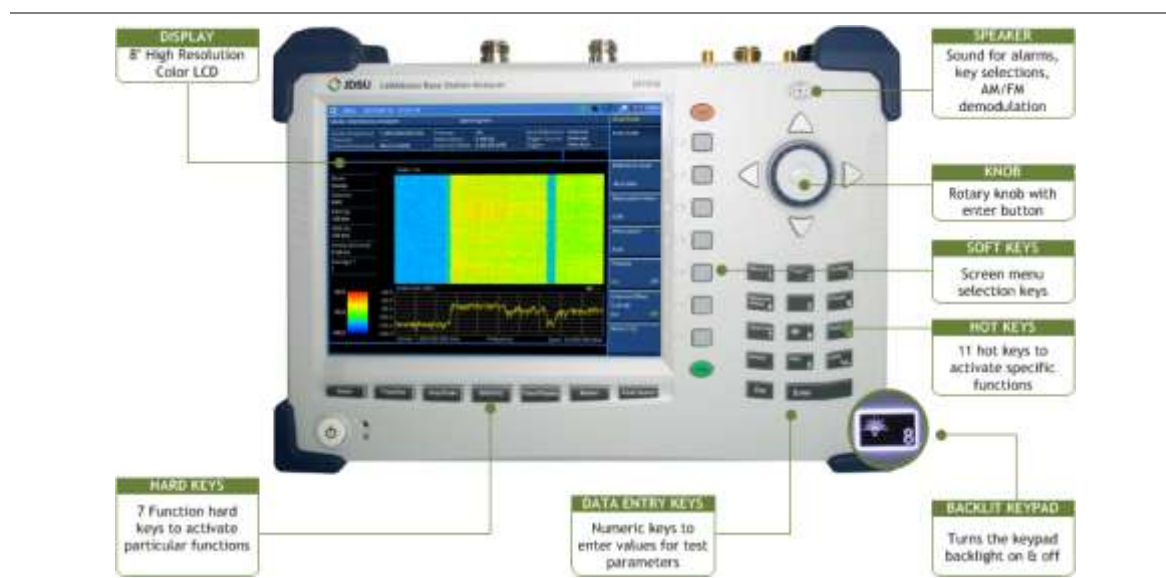
Figure 1 JD785B front panel view
