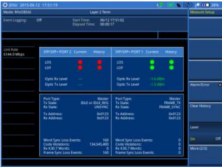
Figure 392 OBSAI layer 2 term test
