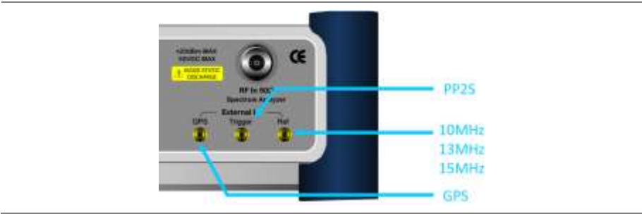
Figure 281 Connection ports for external reference clock
