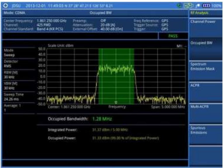
Figure 211 Occupied bandwidth measurement with CDMA signal analyzer
