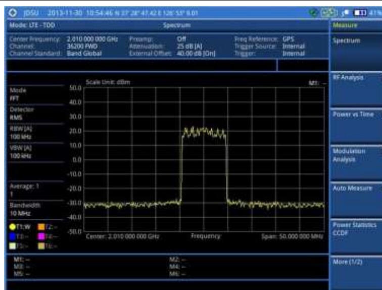
Figure 164 Spectrum measurement screen with LTE-TDD signal analyzer
