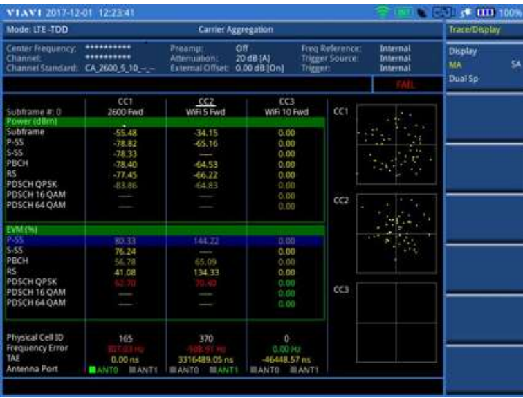
Figure 188 Carrier aggregation measurement with LTE-TDD signal analyzer (SA with Wi-Fi on)
