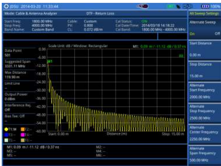
Figure 325 DTF measurement with the alternate sweep on
