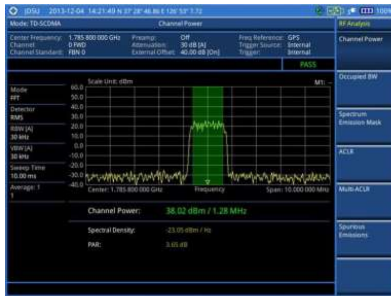
Figure 258 Channel power measurement with TD-SCDMA signal analyzer
