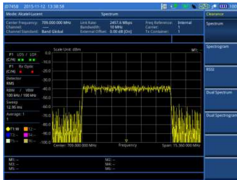
Figure 427 Example of spectrum measurement in Alcatel-Lucent BBU emulation
