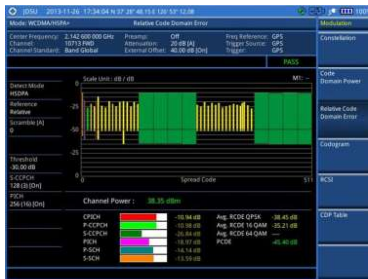
Figure 98 Relative code domain error with WCDMA/HSPA+ signal analyzer
