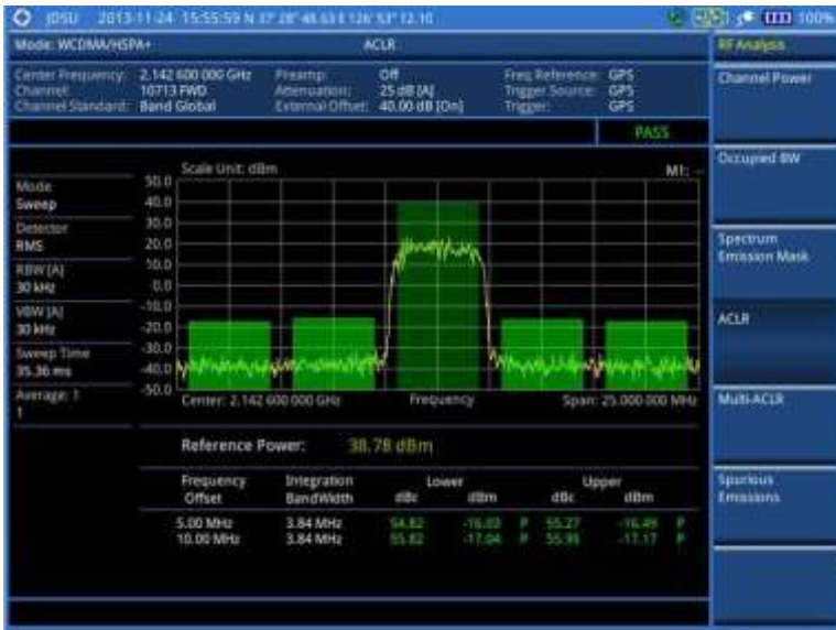
Figure 93 ACLR measurement with WCDMA/HSPA+ signal analyzer
