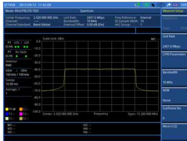
Figure 377 Spectrum measurement with RFoCPRI LTE-TDD signal analyzer
