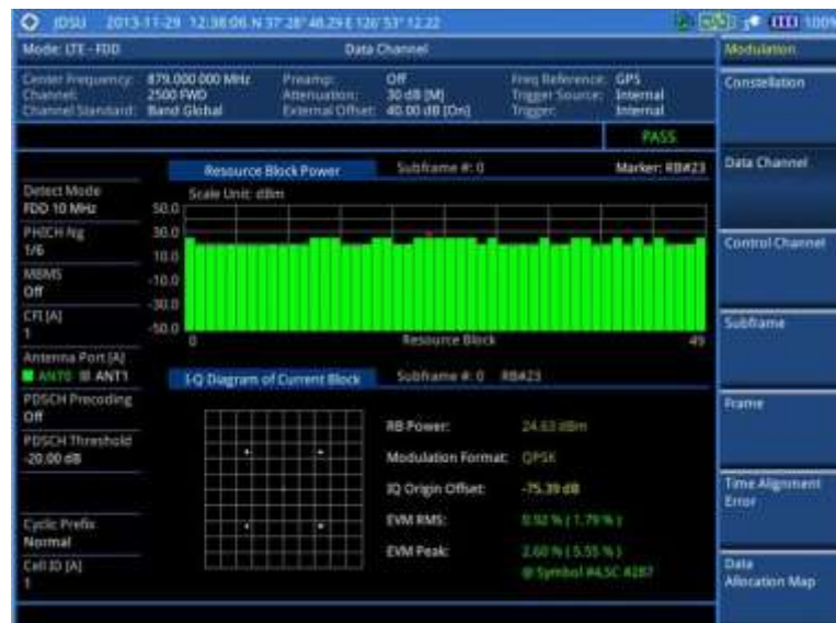
Figure 125 Data channel measurement with LTE-FDD signal analyzer
