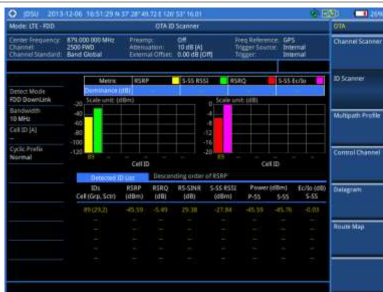
Figure 146 ID scanner measurement with LTE-FDD OTA signal analyzer
