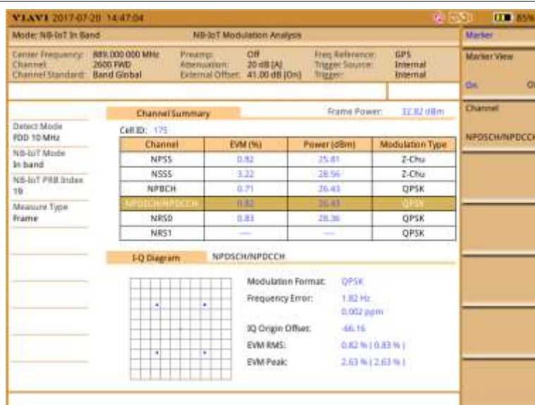
Figure 301 NB-IoT In Band Modulation Analysis measurement screen (Frame)
