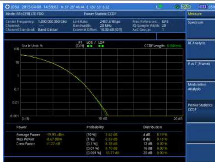
Figure 375 CCDF measurement with RFoCPRI LTE-FDD signal analyzer
