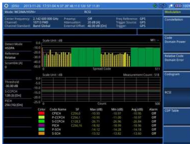
Figure 100 RCSI measurement with WCDMA/HSPA+ signal analyzer
