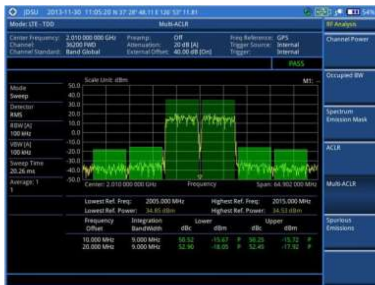
Figure 169 Multi-ACLR measurement with LTE-TDD signal analyzer
