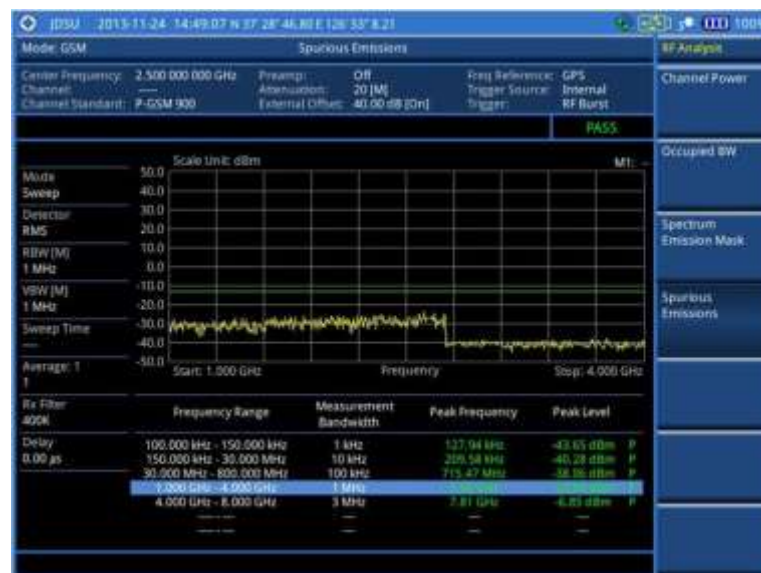
Figure 74 Spurious emissions measurement with GSM signal analyzer
