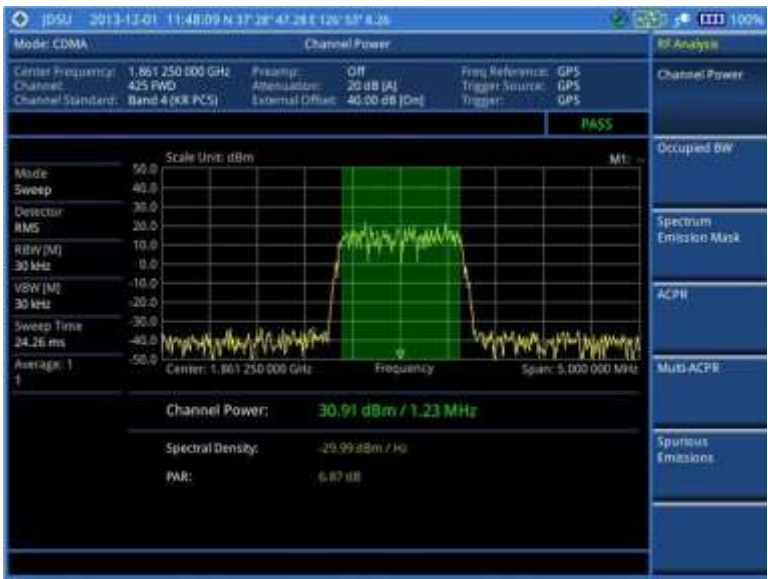
Figure 210 Channel power measurement with CDMA signal analyzer
