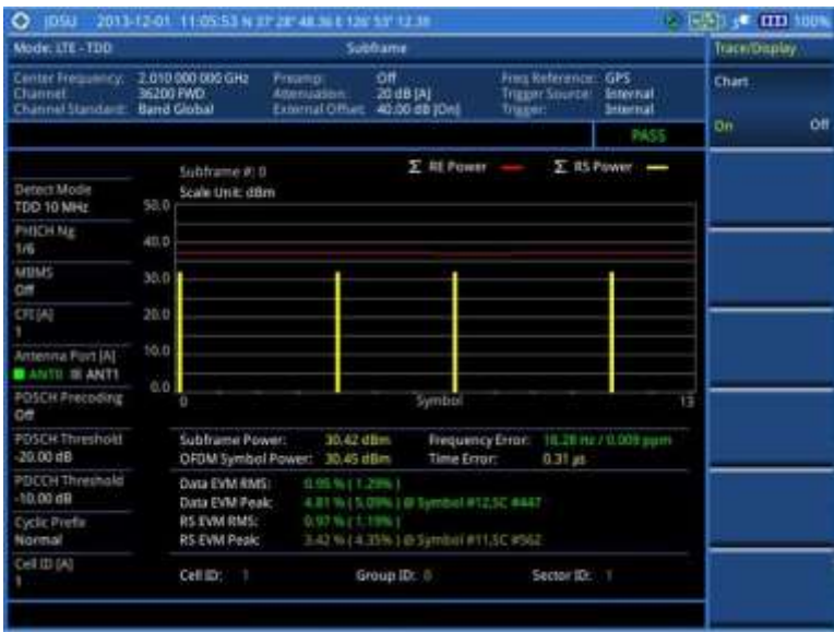
Figure 181 Subframe measurement with LTE-TDD signal analyzer (MBMS On)
