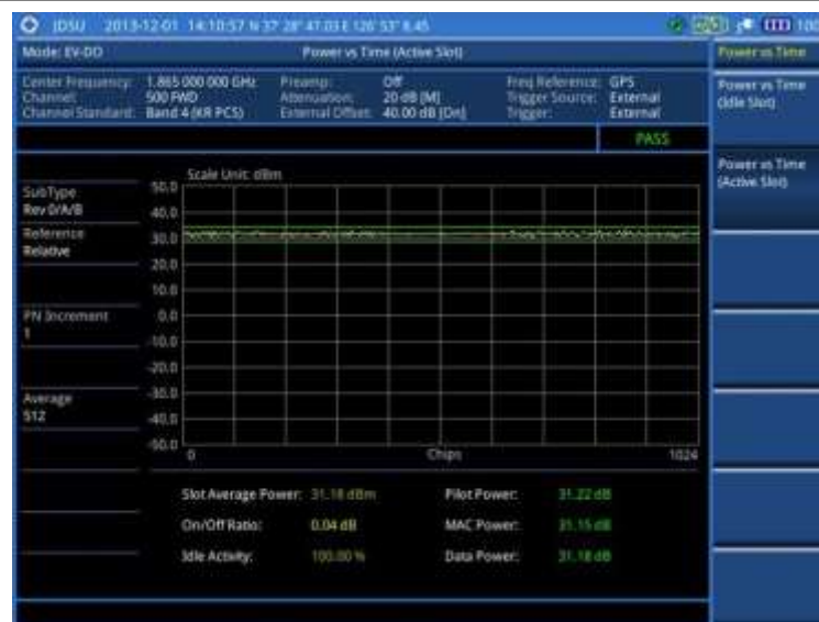
Figure 240 Power vs. time (active slot) measurement with EV-DO signal analyzer
