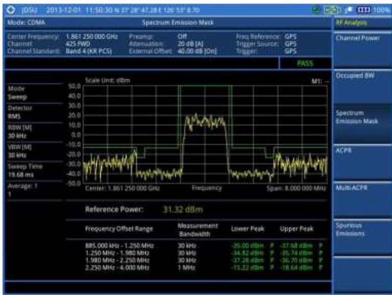
Figure 212 SEM measurement with CDMA signal analyzer
