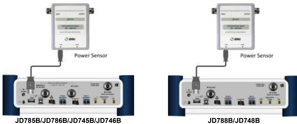
Figure 454 Directional power sensor connection
