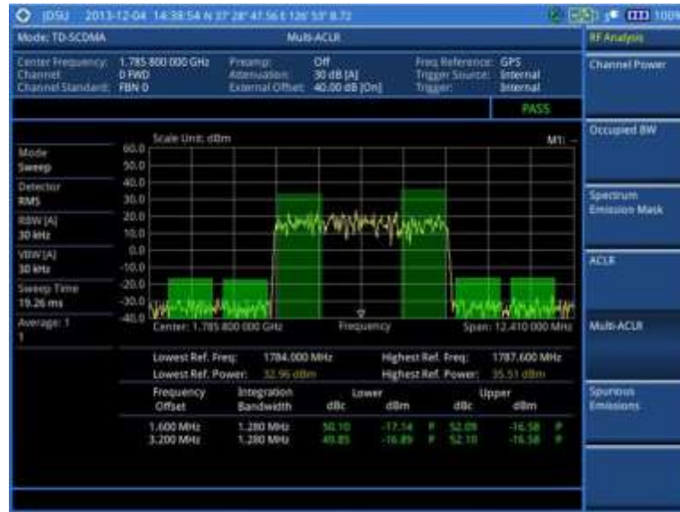
Figure 262 Multi-ACLR measurement with TD-SCDMA signal analyzer
