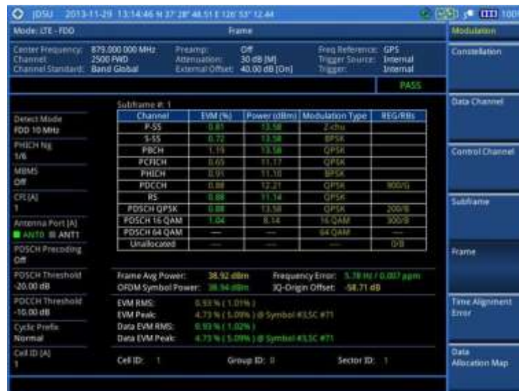
Figure 133 Frame measurement with LTE-FDD signal analyzer
