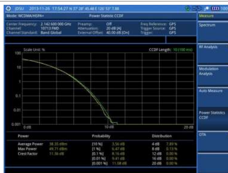
Figure 102 CCDF measurement with WCDMA/HSPA+ signal analyzer
