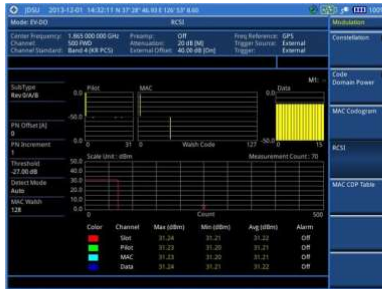
Figure 244 RCSI measurement with EV-DO signal analyzer
