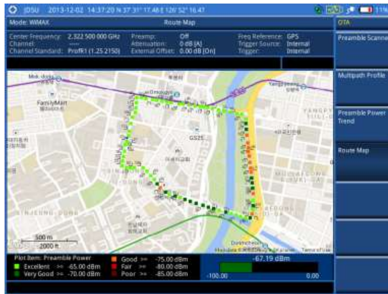
Figure 296 Route map measurement with Mobile WiMAX OTA signal analyzer
