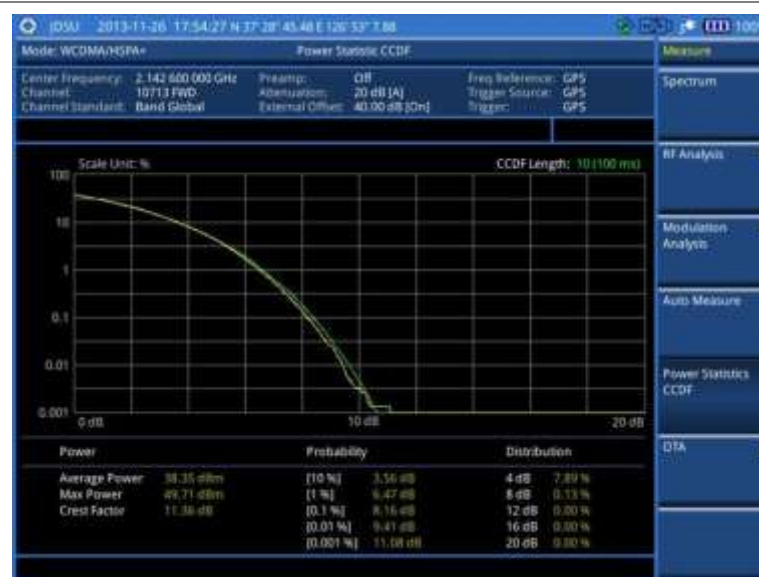
Figure 78 CCDF measurement with WCDMA/HSPA+ signal analyzer
