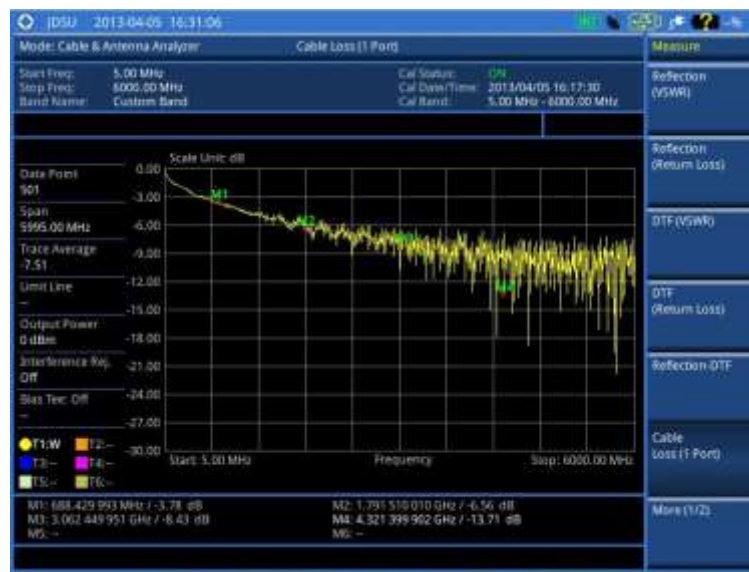
Figure 284 Cable loss (1 port) measurement
