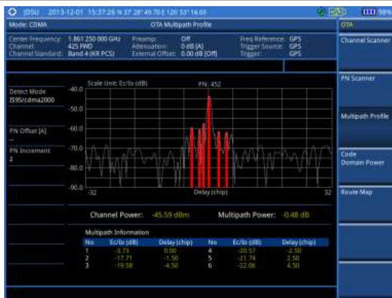
Figure 195 Multipath profile measurement with CDMA OTA signal analyzer
