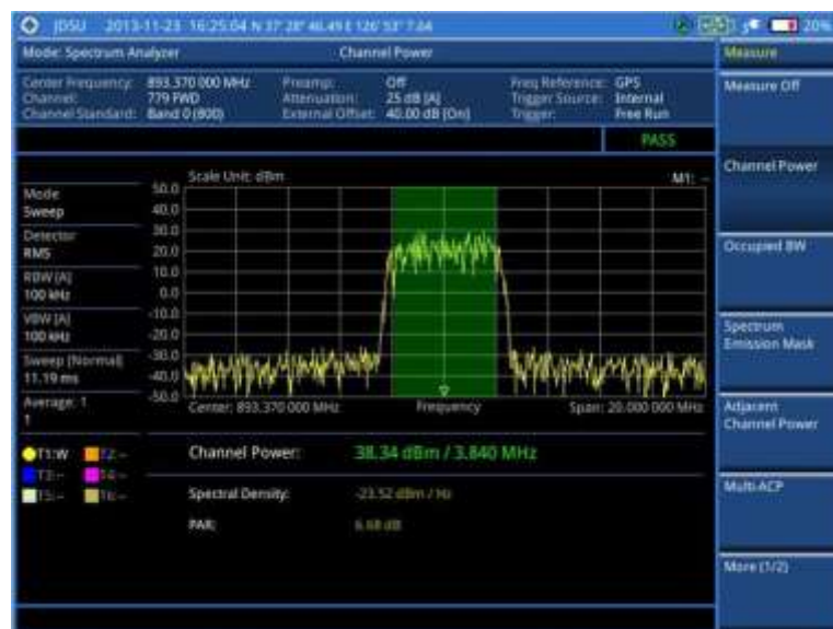
Figure 16 Channel power measurement with spectrum analyzer
