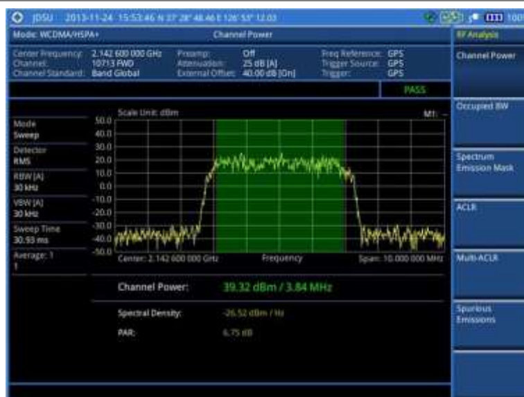
Figure 66 Channel power measurement with WCDMA/HSPA+ signal analyzer
