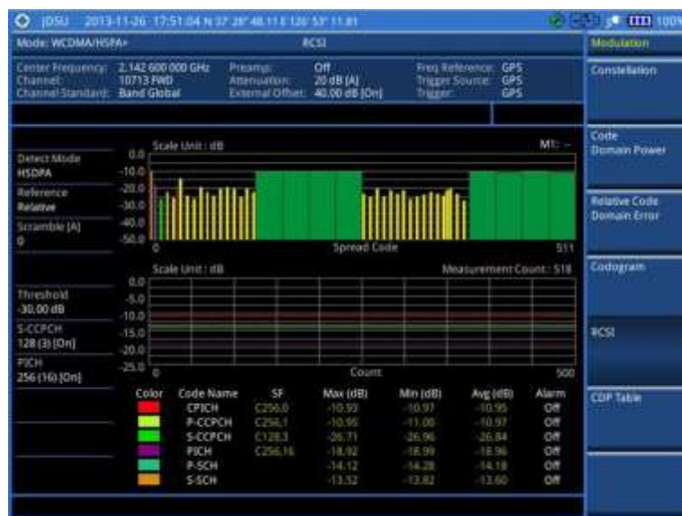
Figure 76 RCSI measurement with WCDMA/HSPA+ signal analyzer
