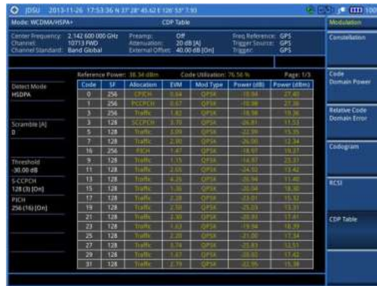
Figure 77 CDP Table measurement with WCDMA/HSPA+ signal analyzer
