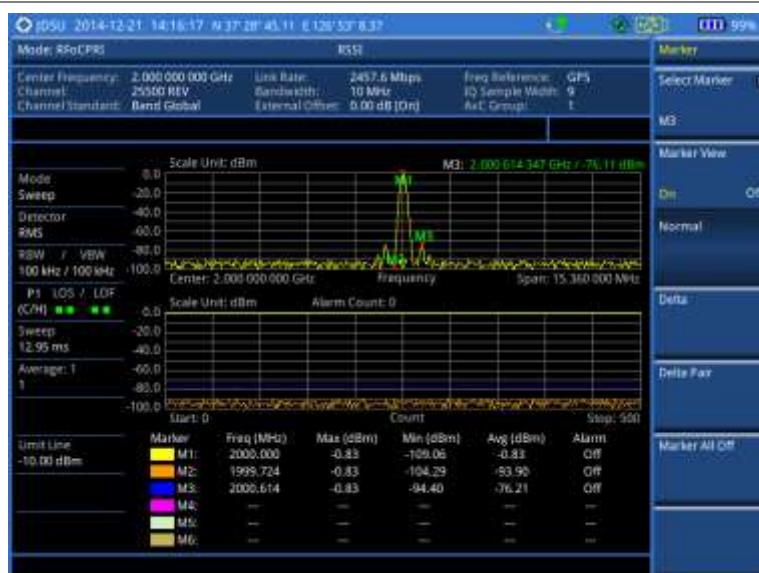
Figure 310 RFoCPRI interference measurement in RSSI
