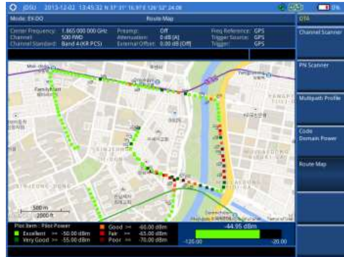
Figure 222 Route map measurement with EV-DO OTA signal analyzer
