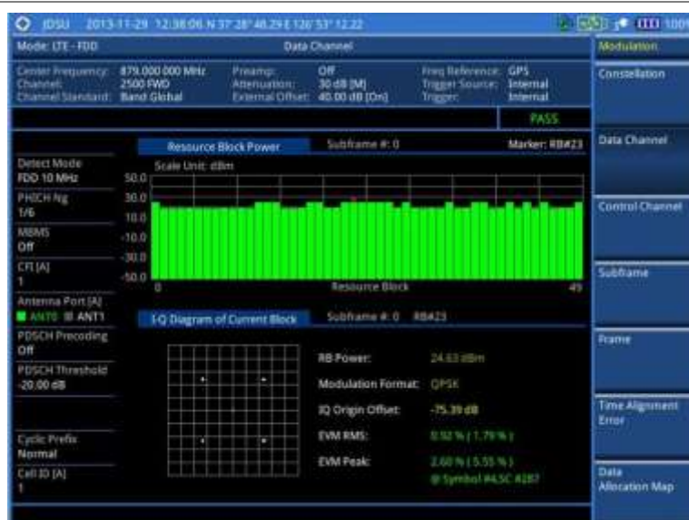
Figure 101 Data channel measurement with LTE-FDD signal analyzer
