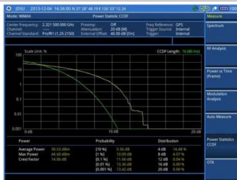
Figure 263 CCDF measurement with Mobile WiMAX signal analyzer
