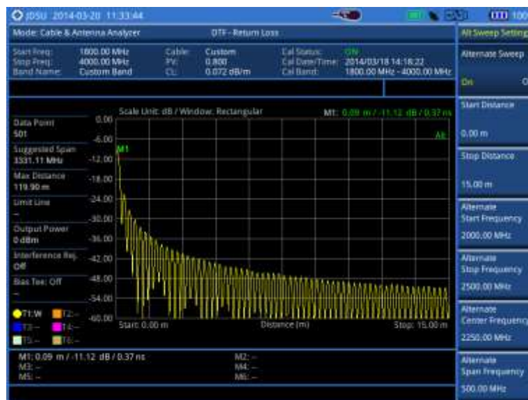
Figure 280 DTF measurement with the alternate sweep on
