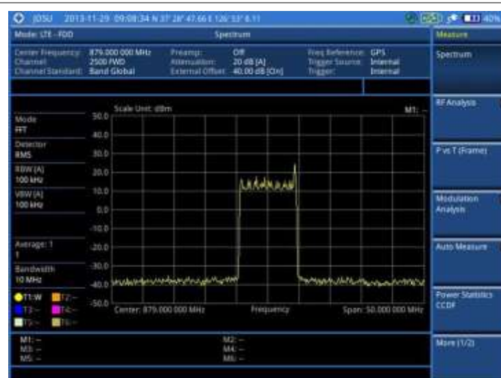
Figure 91 Spectrum measurement screen with LTE-FDD signal analyzer
