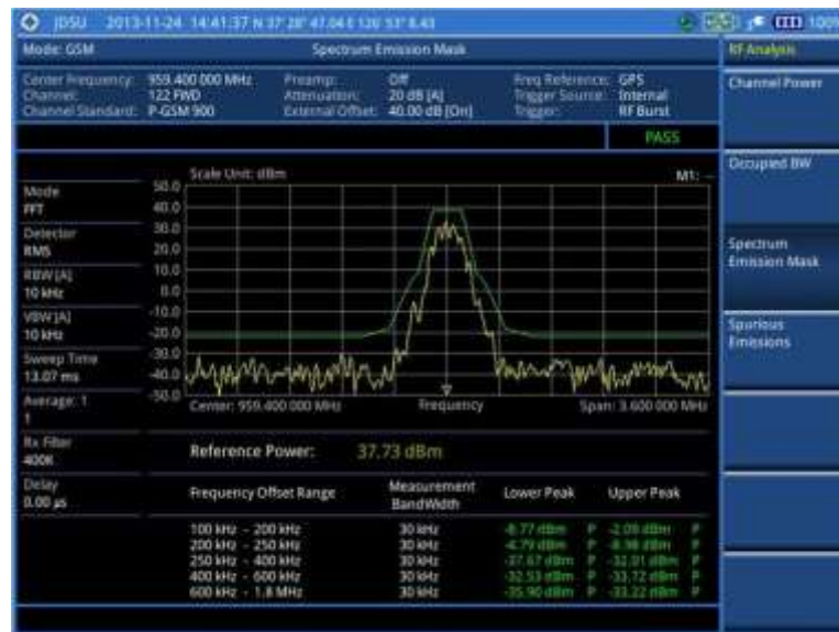
Figure 48 SEM measurement with GSM signal analyzer
