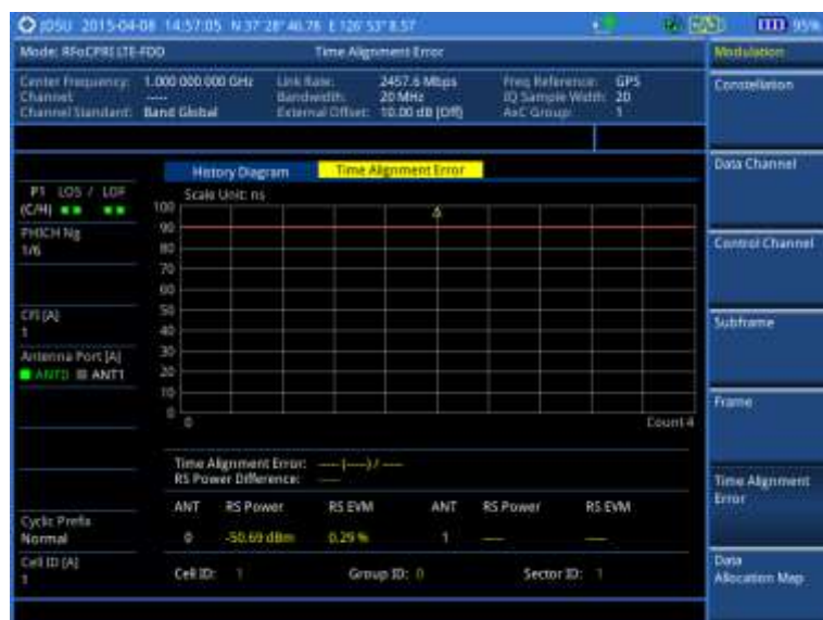
Figure 326 Time alignment error measurement with RFoCPRI LTE-FDD signal analyzer
