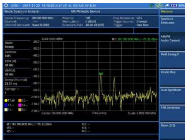
Figure 22 AM/FM audio demodulation with spectrum analyzer
