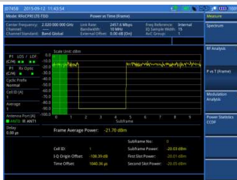
Figure 333 Power vs. time (frame) measurement with RFoCPRI LTE-TDD signal analyzer
