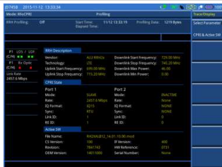
Figure 344 Example of RRH profiling results with CPRI state and activated SW
