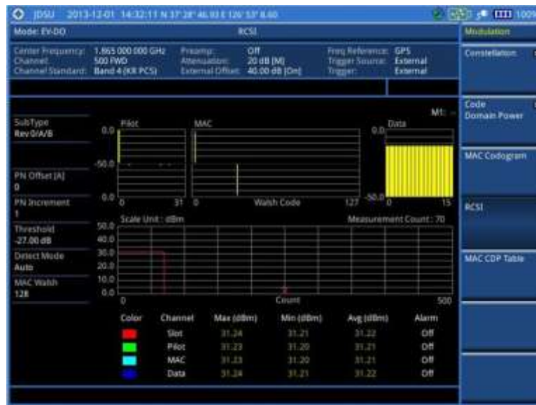
Figure 215 RCSI measurement with EV-DO signal analyzer
