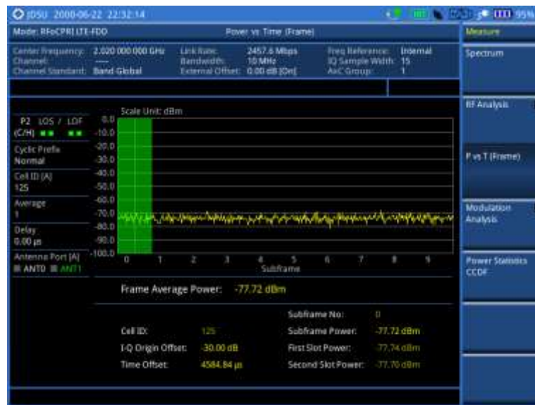
Figure 320 Power vs. time (frame) measurement with RFoCPRI LTE-FDD signal analyzer
