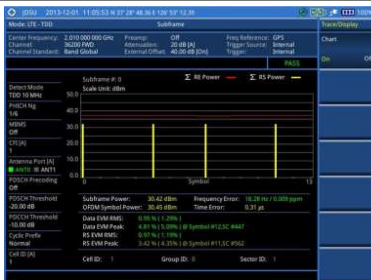
Figure 153 Subframe measurement with LTE-TDD signal analyzer (MBMS On)
