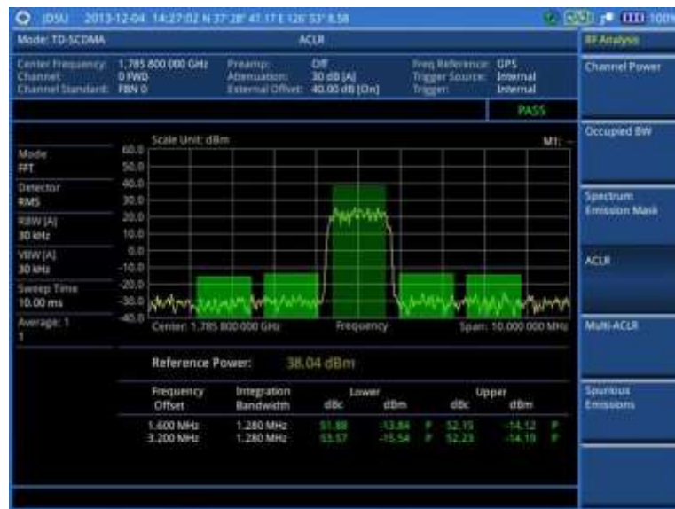
Figure 232 ACLR measurement with TD-SCDMA signal analyzer
