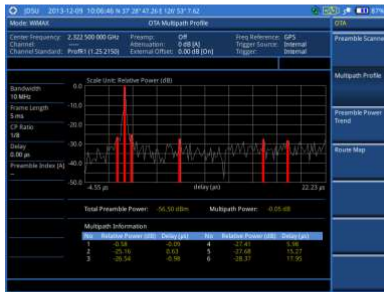
Figure 265 Multipath profile measurement with Mobile WiMAX OTA signal analyzer
