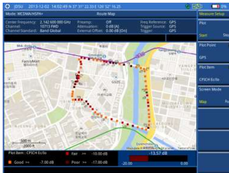
Figure 84 Route map measurement ( CPICH Ec/Io ) with WCDMA/HSPA+ OTA signal analyzer
