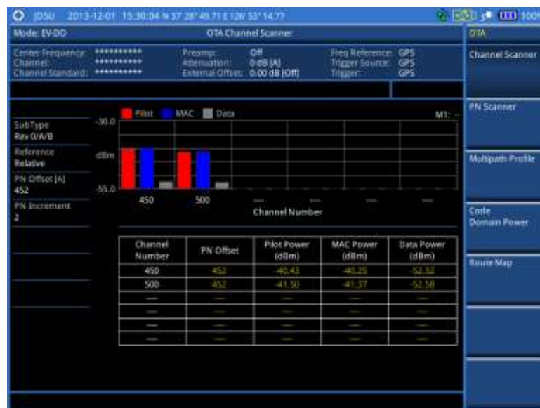
Figure 218 Channel scanner measurement with EV-DO OTA signal analyzer
