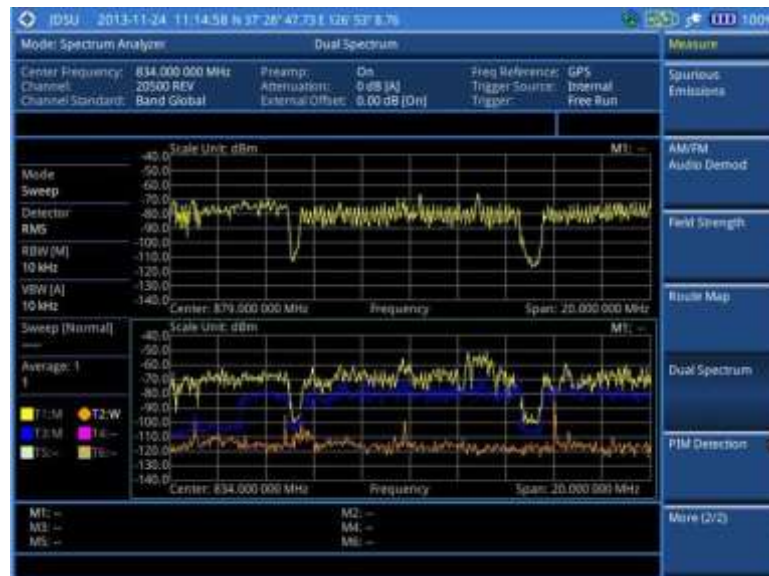
Figure 26 Dual spectrum measurement with spectrum analyzer
