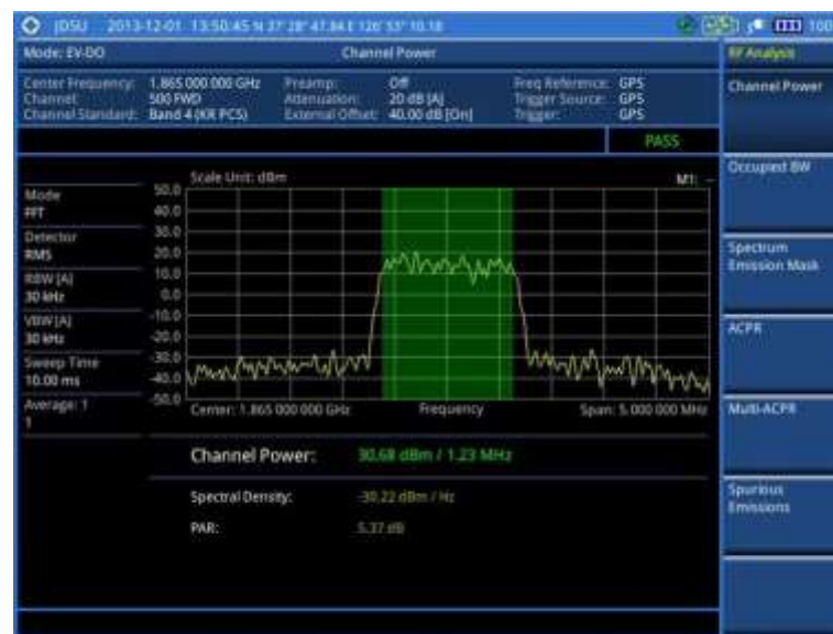
Figure 204 Channel power measurement with EV-DO signal analyzer
