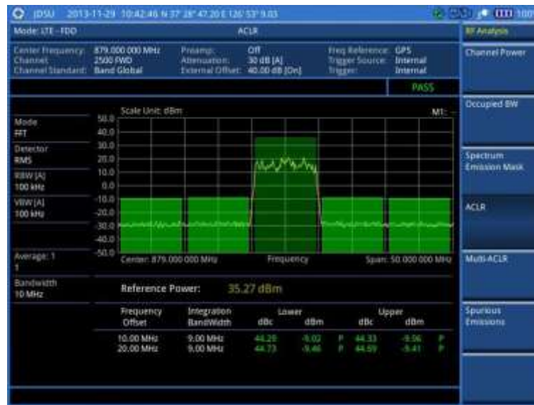
Figure 95 ACLR measurement with LTE-FDD signal analyzer
