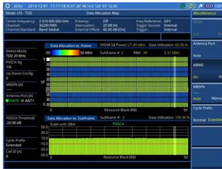
Figure 156 Data allocation map measurement with LTE-TDD signal analyzer (MBMS On)
