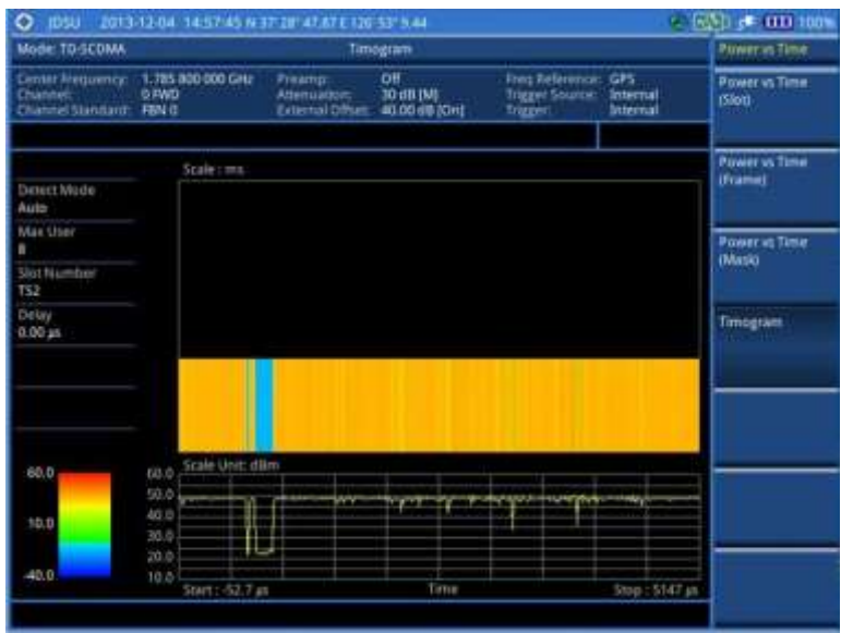
Figure 238 Timogram with TD-SCDMA signal analyzer
