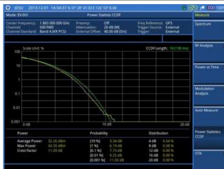
Figure 217 CCDF measurement with EV-DO signal analyzer
