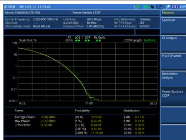
Figure 385 CCDF measurement with RFoBSAI LTE-FDD signal analyzer
