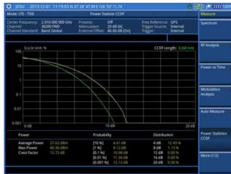
Figure 158 CCDF measurement with LTE-TDD signal analyzer
