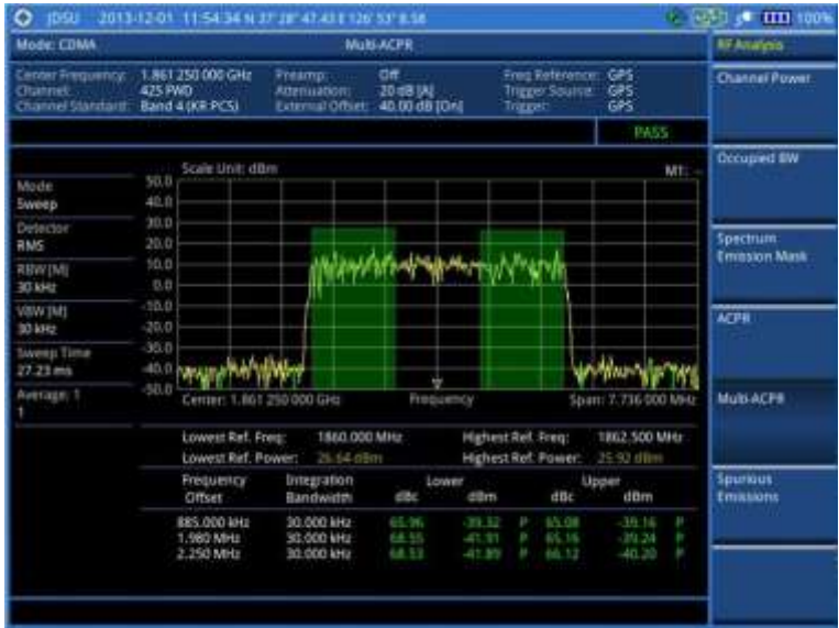
Figure 185 Multi-ACPR measurement with CDMA signal analyzer
