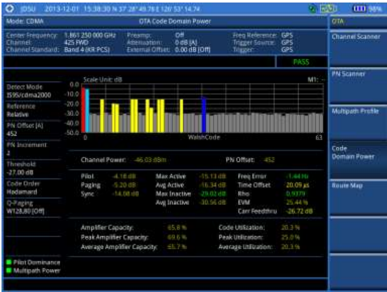
Figure 196 Code domain power measurement with CDMA OTA signal analyzer
