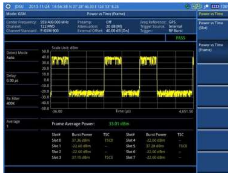
Figure 53 Power vs. time (frame) measurement with GSM signal analyzer
