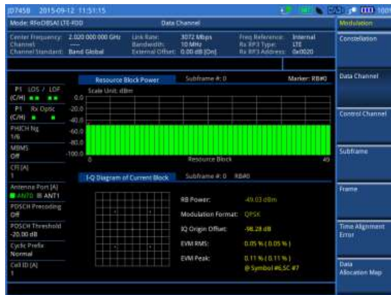
Figure 379 Data channel measurement with RFoBSAI LTE-FDD signal analyzer
