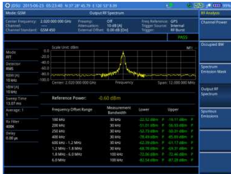
Figure 49 Output RF spectrum measurement with GSM signal analyzer
