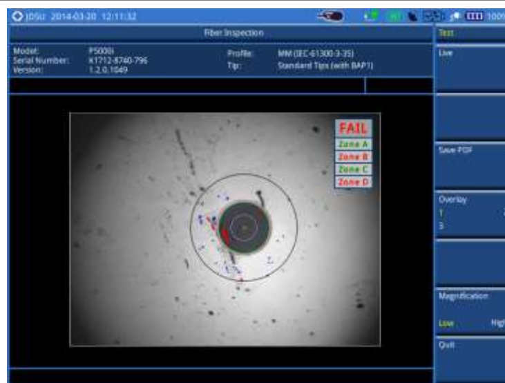
Figure 403 Analyzed fiber image and fiber inspection result
