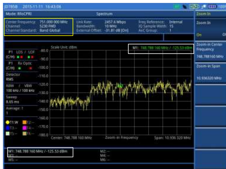
Figure 311 Zoomed-in spectrum view in RFoCPRI interference analyzer
