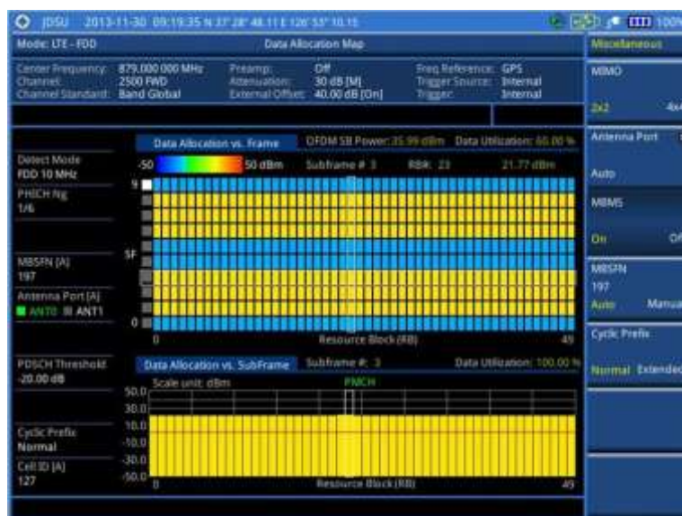
Figure 112 Data allocation map measurement with LTE-FDD signal analyzer (MBMS On)
