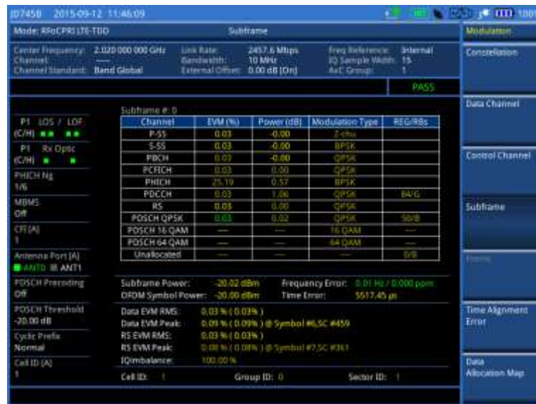
Figure 337 Subframe measurement (regular view) with RFoCPRI LTE-TDD signal analyzer
