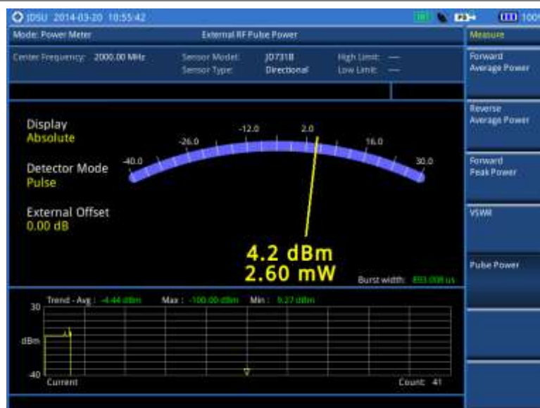
Figure 398 External power measurement of pulse power
