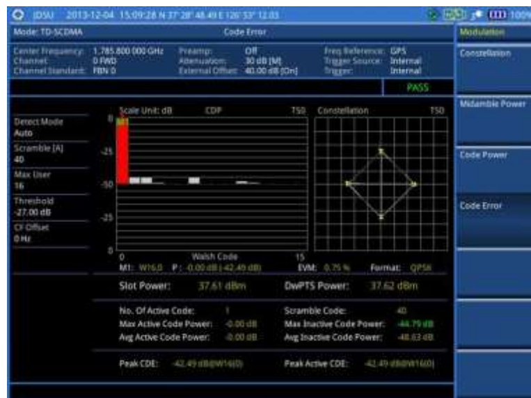
Figure 242 Code error measurement with TD-SCDMA signal analyzer
