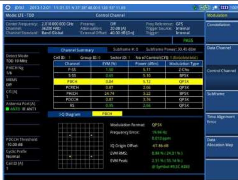
Figure 149 Control channel measurement with LTE-TDD signal analyzer
