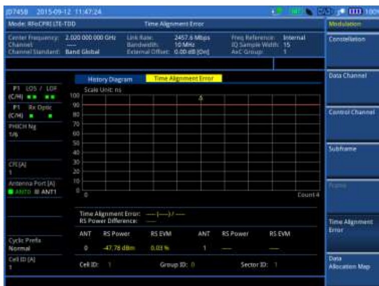
Figure 338 Time alignment error measurement with RFoCPRI LTE-TDD signal analyzer
