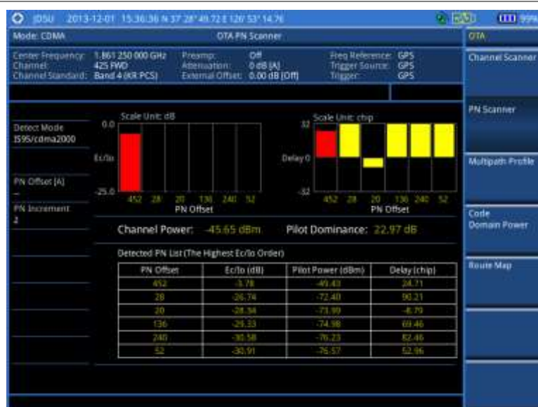
Figure 194 PN scanner measurement with CDMA OTA signal analyzer
