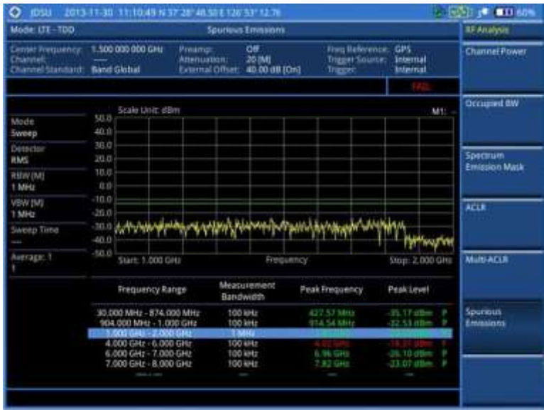
Figure 142 Spurious emissions measurement with LTE-TDD signal analyzer
