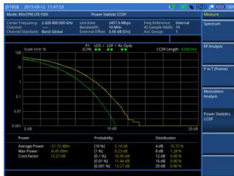
Figure 340 CCDF measurement with RFoCPRI LTE-TDD signal analyzer
