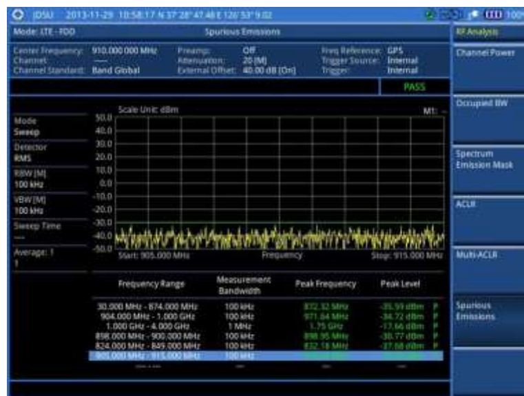
Figure 97 Spurious emissions measurement with LTE-FDD signal analyzer
