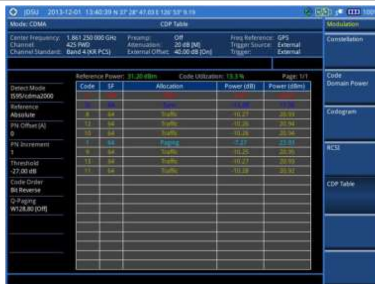
Figure 191 CDP Table measurement with CDMA signal analyzer
