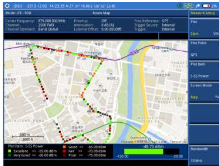
Figure 127 Route map measurement (S-SS Power) with LTE-FDD OTA signal analyzer
