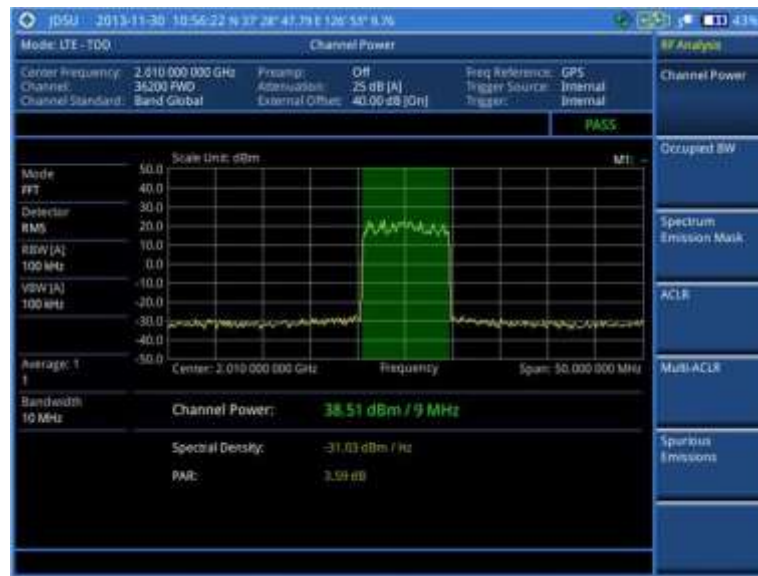
Figure 137 Channel power measurement with LTE-TDD signal analyzer
