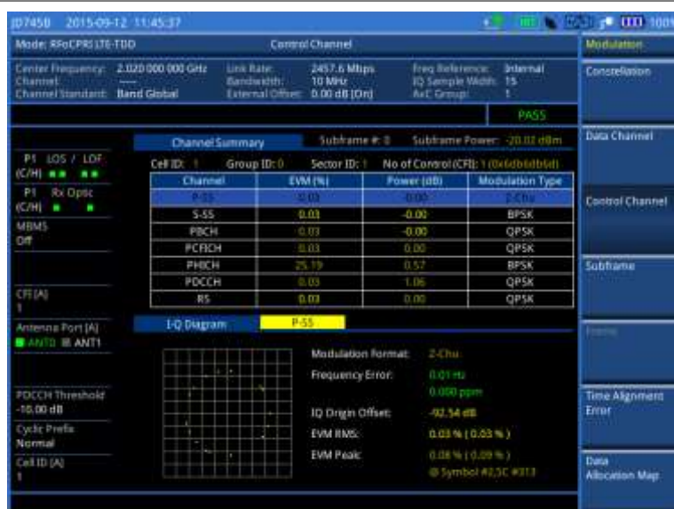
Figure 336 Control channel measurement with RFoCPRI LTE-TDD signal analyzer
