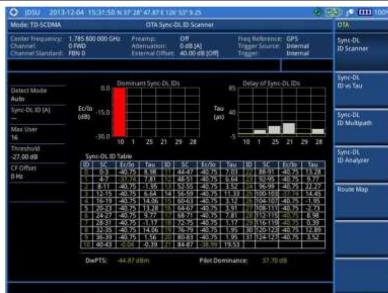
Figure 243 Sync-DL ID scanner measurement with TD-SCDMA OTA signal analyzer
