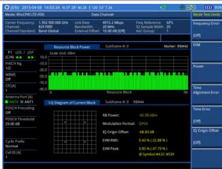
Figure 322 Data channel measurement with RFoCPRI LTE-FDD signal analyzer
