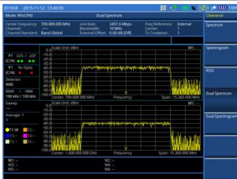
Figure 353 Example of dual spectrum analysis in BBU emulation
