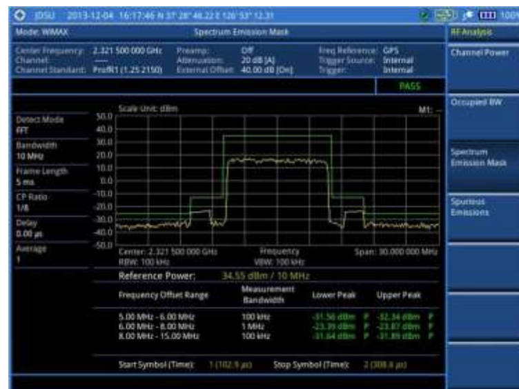
Figure 256 SEM measurement with Mobile WiMAX signal analyzer
