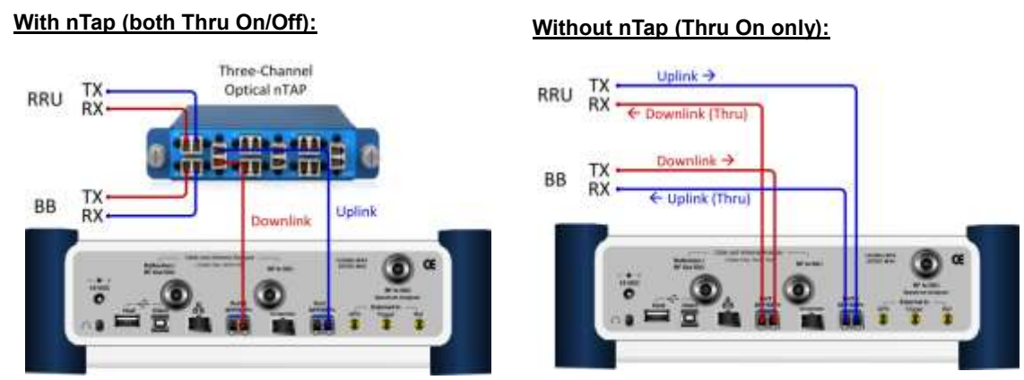
Figure 362 Connection diagram for Layer-2 monitoring mode
