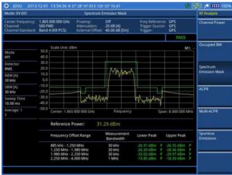
Figure 206 SEM measurement with EV-DO signal analyzer
