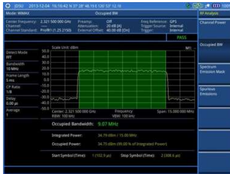
Figure 255 Occupied bandwidth measurement with Mobile WiMAX signal analyzer
