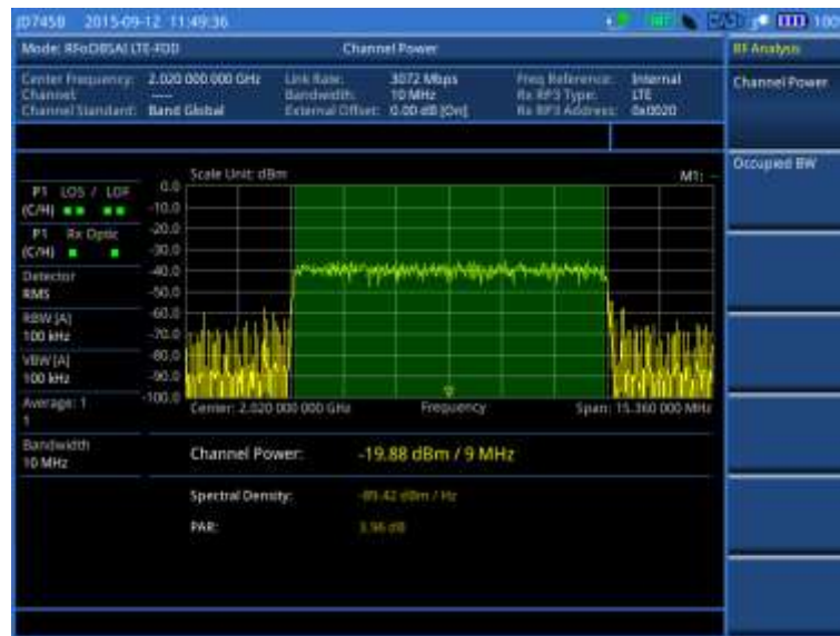
Figure 375 Channel power measurement with RFoBSAI LTE-FDD signal analyzer
