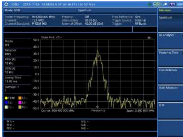
Figure 45 Spectrum measurement screen with GSM signal analyzer
