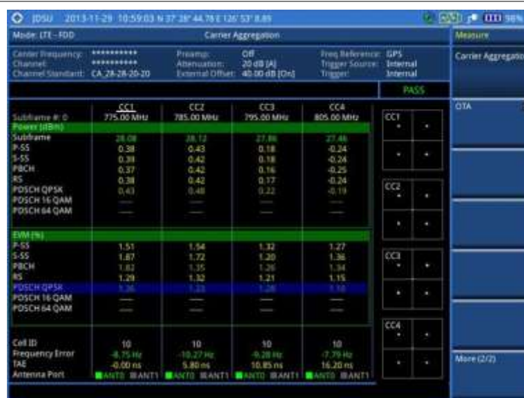
Figure 116 Carrier aggregation measurement with LTE-FDD signal analyzer (SA)
