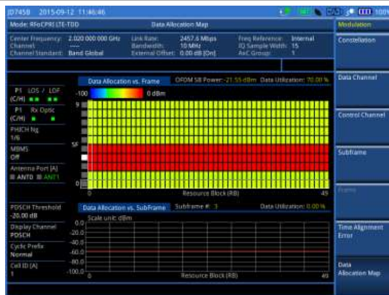
Figure 339 Data allocation map measurement with RFoCPRI LTE-TDD signal analyzer
