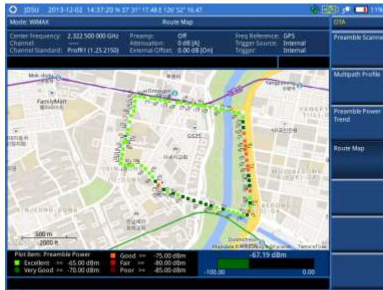
Figure 267 Route map measurement with Mobile WiMAX OTA signal analyzer
