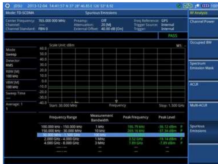
Figure 234 Spurious emissions measurement with TD-SCDMA signal analyzer
