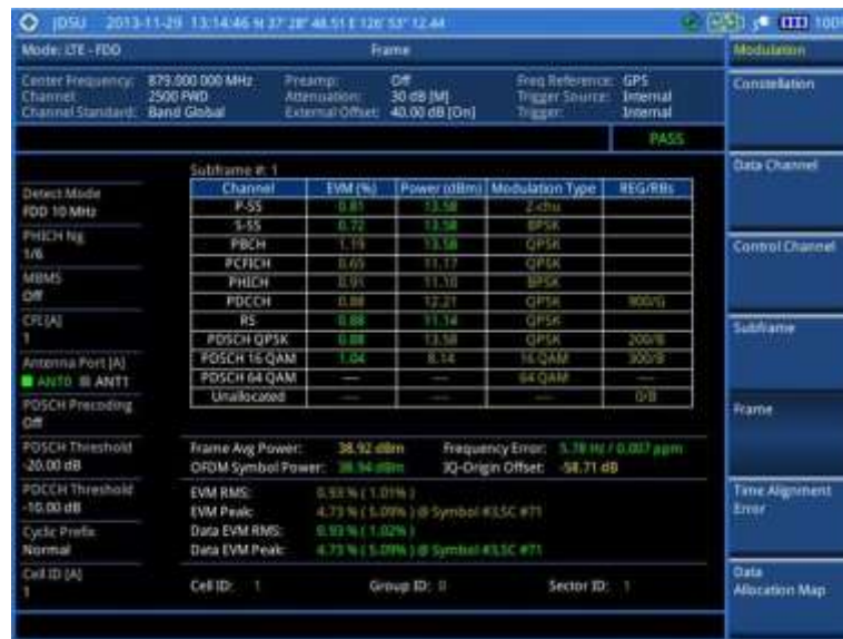
Figure 109 Frame measurement with LTE-FDD signal analyzer (MBMS On)
