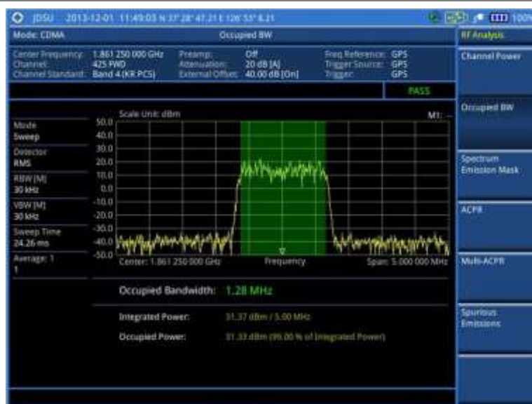
Figure 182 Occupied bandwidth measurement with CDMA signal analyzer
