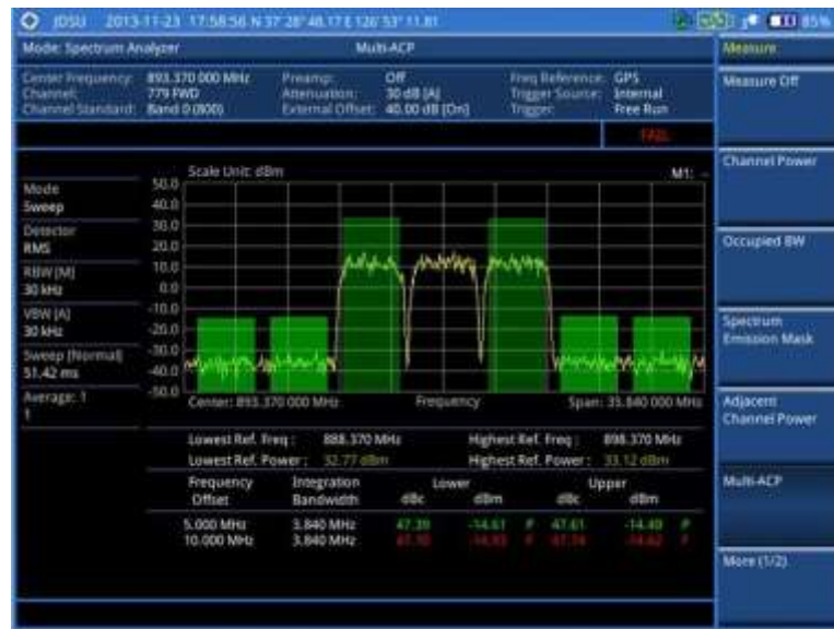
Figure 20 Multi-ACP measurement with spectrum analyzer
