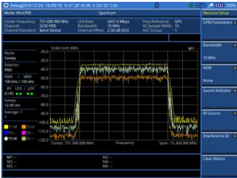
Figure 300 RFoCPRI spectrum analysis on LTE Uplink 10 MHz, antenna 1
