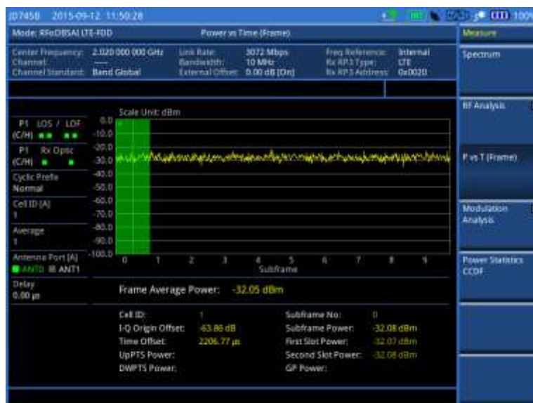
Figure 377 Power vs. time (frame) measurement with RFoBSAI LTE-FDD signal analyzer
