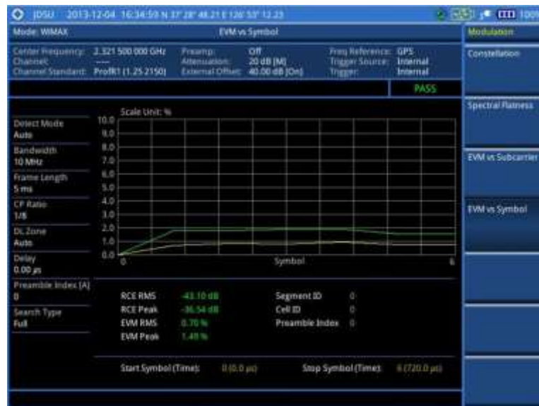
Figure 262 EVM vs. symbol measurement with Mobile WiMAX signal analyzer
