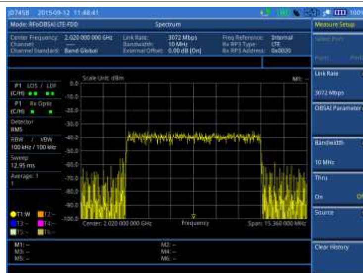
Figure 374 Spectrum measurement with RFoBSAI LTE-FDD signal analyzer
