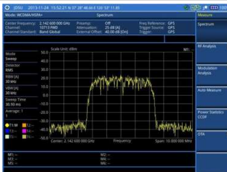
Figure 65 Spectrum measurement screen with WCDMA signal analyzer
