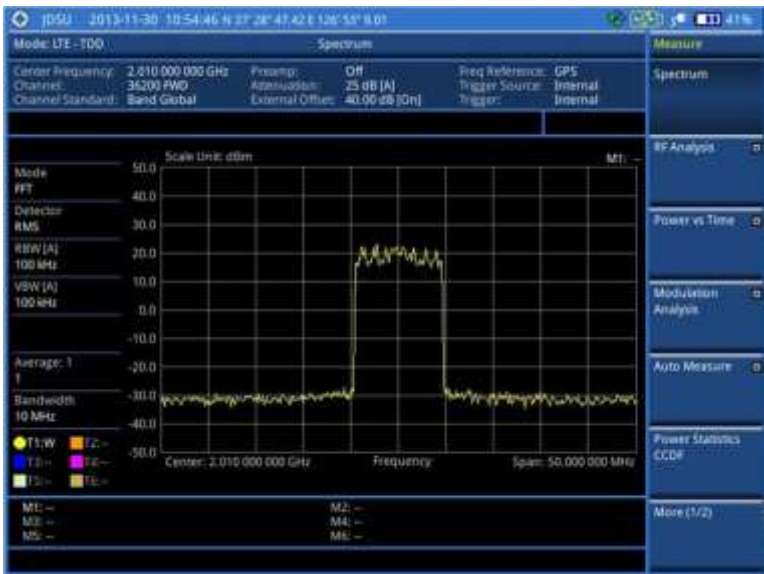
Figure 136 Spectrum measurement screen with LTE-TDD signal analyzer
