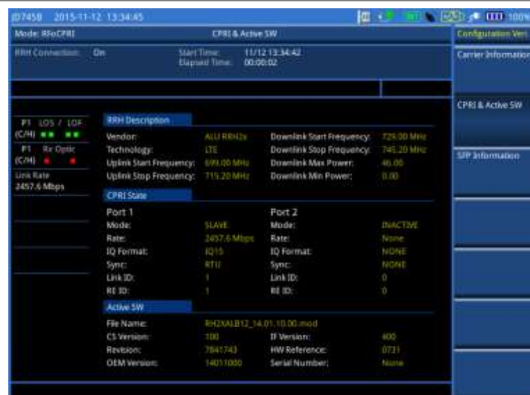
Figure 348 Example of verification of CPRI state and active software
