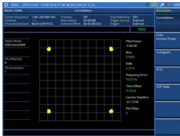
Figure 187 Constellation measurement with CDMA signal analyzer
