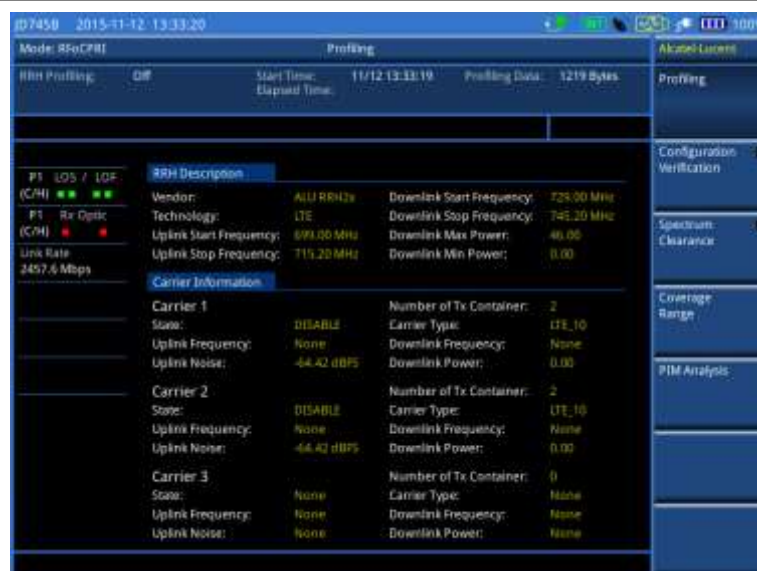
Figure 343 Example of RRH profiling results with carrier information
