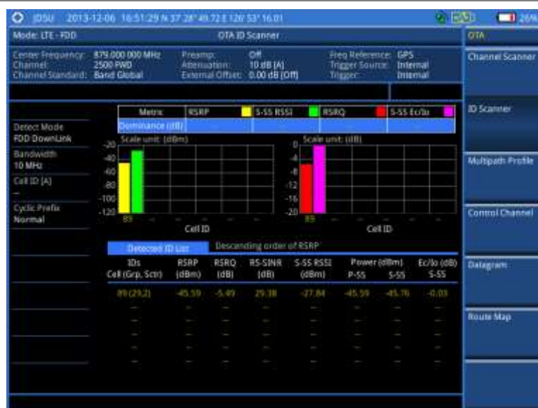
Figure 118 ID scanner measurement with LTE-FDD OTA signal analyzer
