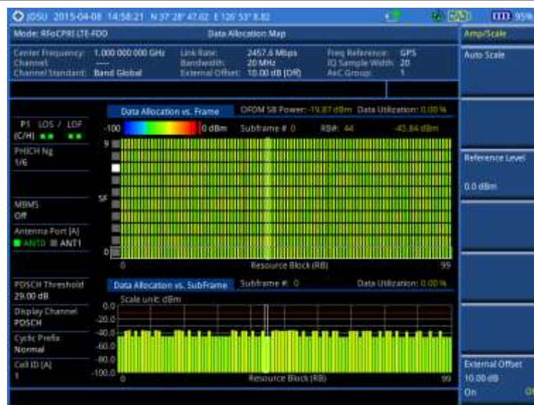
Figure 327 Data allocation map measurement with RFoCPRI LTE-FDD signal analyzer
