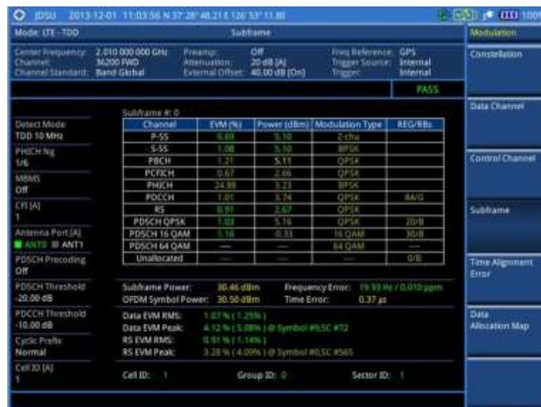
Figure 151 Subframe measurement with LTE-TDD signal analyzer
