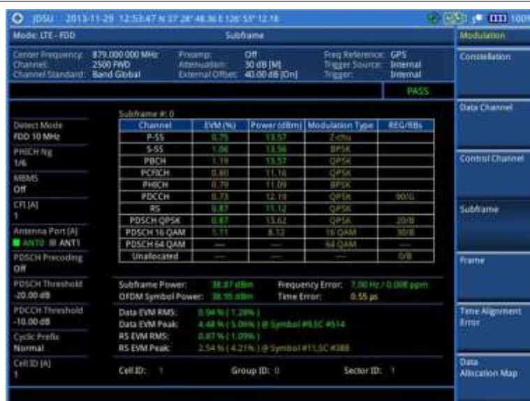
Figure 105 Subframe measurement with LTE-FDD signal analyzer
