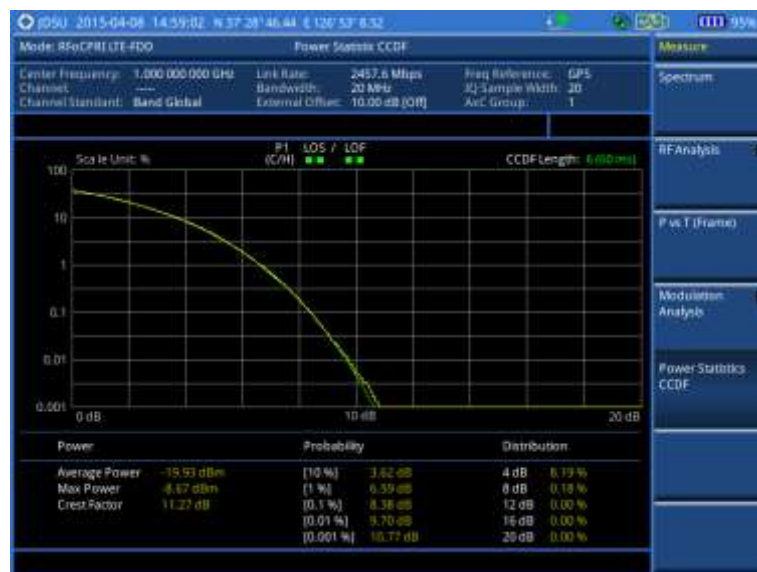
Figure 328 CCDF measurement with RFoCPRI LTE-FDD signal analyzer
