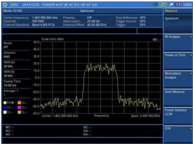
Figure 203 Spectrum measurement screen with EV-DO signal analyzer
