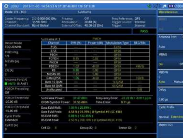
Figure 153 Subframe measurement with LTE-TDD signal analyzer (MBMS On)
