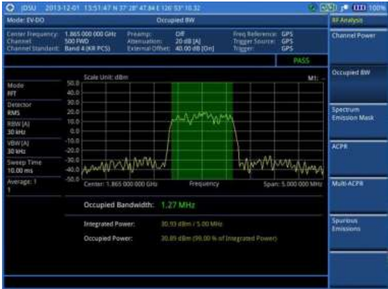
Figure 205 Occupied bandwidth measurement with EV-DO signal analyzer
