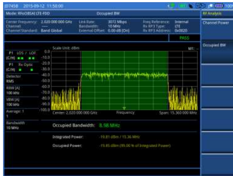
Figure 376 Occupied bandwidth measurement with RFoBSAI LTE-FDD signal analyzer
