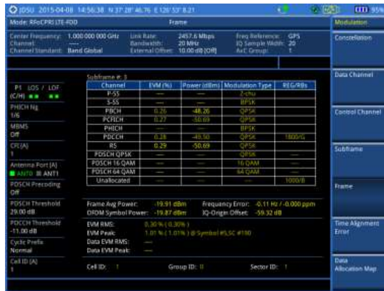
Figure 325 Frame measurement with RFoCPRI LTE-FDD signal analyzer
