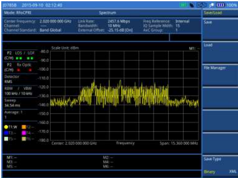
Figure 300 RFoCPRI spectrum analysis on LTE Uplink 10 MHz, antenna 1
