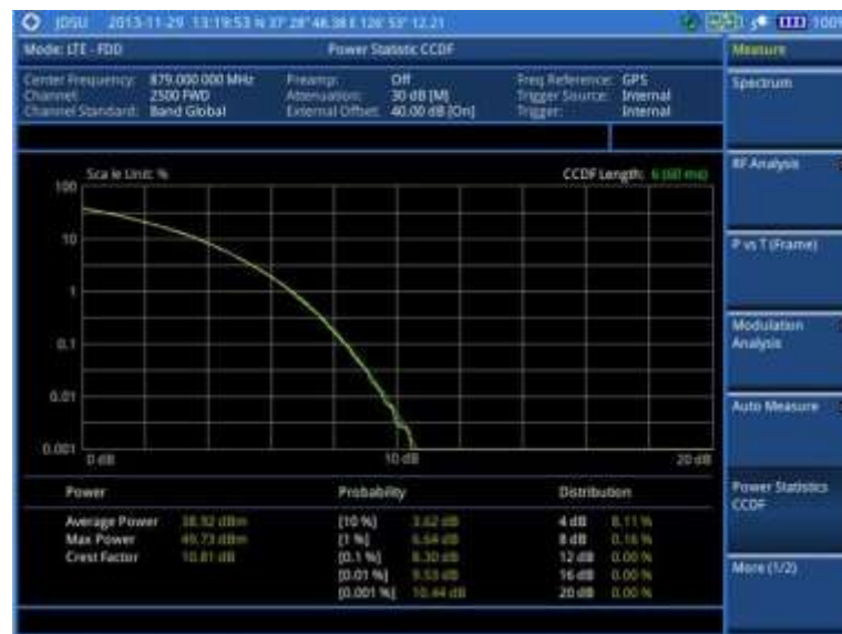
Figure 114 CCDF measurement with LTE-FDD signal analyzer
