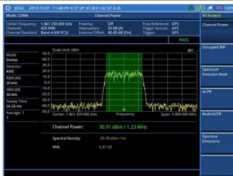
Figure 181 Channel power measurement with CDMA signal analyzer
