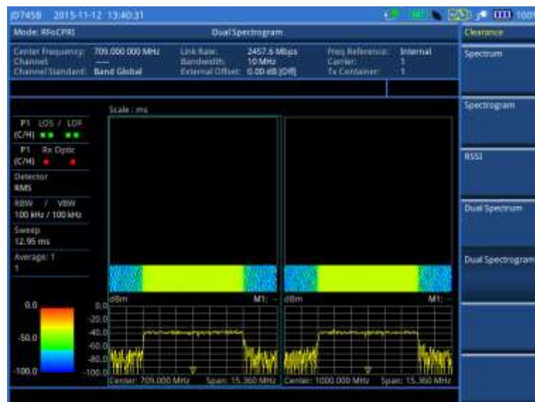
Figure 355 Example of dual spectrogram analysis in BBU emulation
