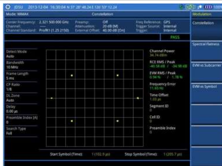
Figure 259 Constellation measurement with Mobile WiMAX signal analyzer
