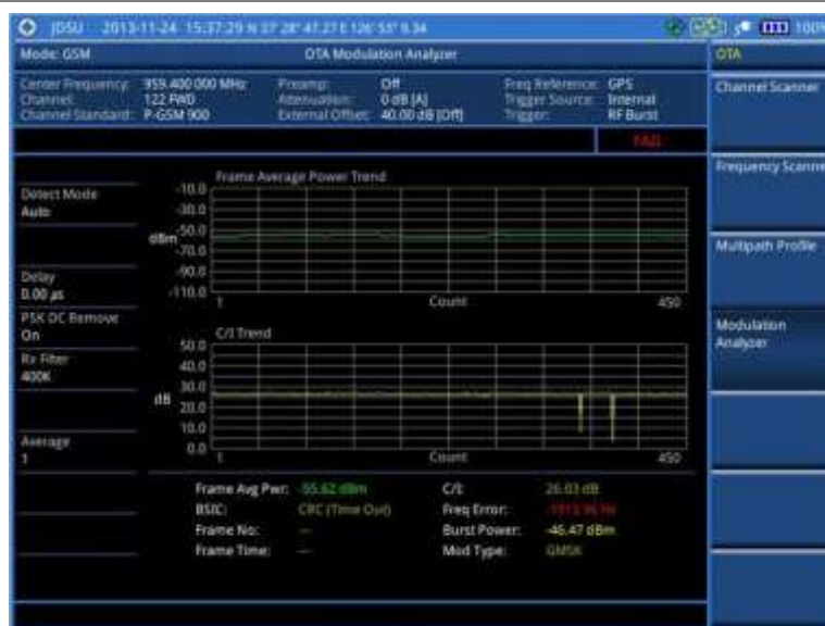
Figure 59 Modulation analyzer measurement with GSM OTA signal analyzer
