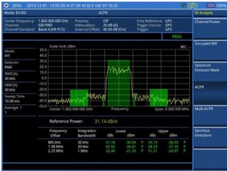
Figure 207 ACPR measurement with EV-DO signal analyzer
