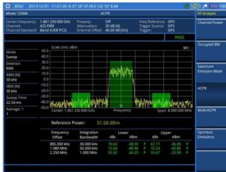
Figure 184 ACPR measurement with CDMA signal analyzer
