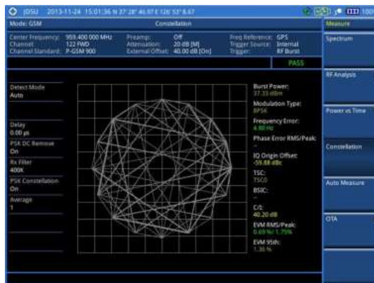
Figure 55 Constellation measurement (PSK on) with GSM signal analyzer
