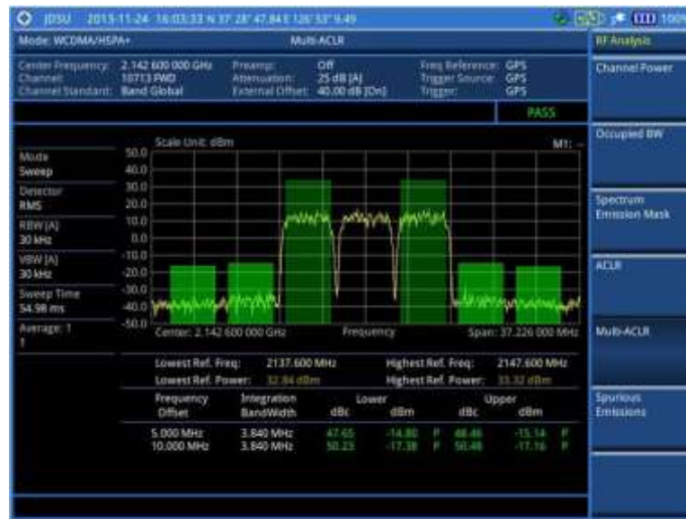
Figure 70 Multi-ACLR measurement with WCDMA/HSPA+ signal analyzer
