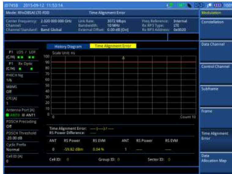
Figure 383 Time alignment error measurement with RFoBSAI LTE-FDD signal analyzer
