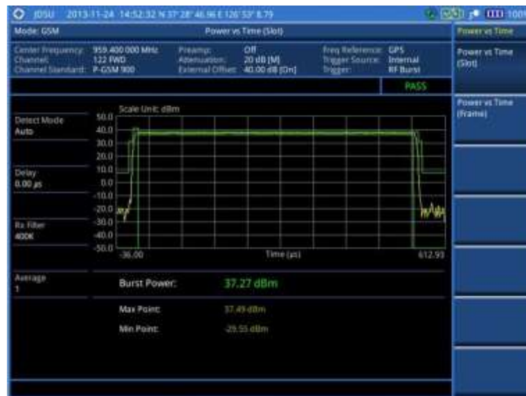
Figure 51 Power vs. time (slot) measurement with GSM signal analyzer
