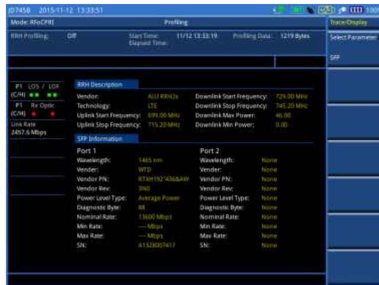
Figure 345 Example of RRH profiling results with SFP information
