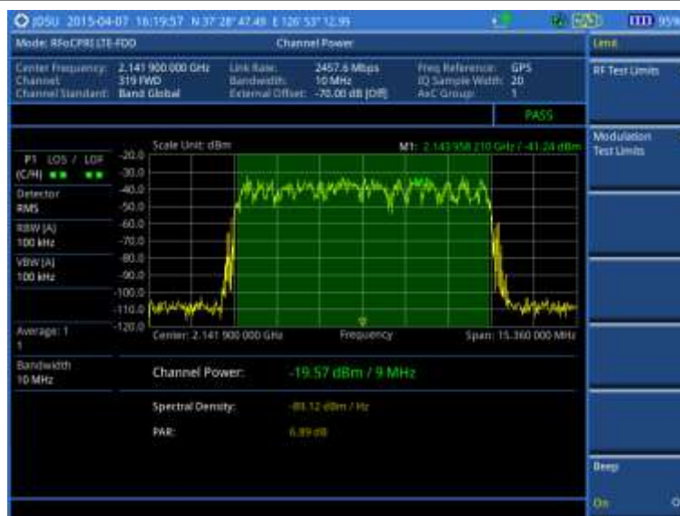
Figure 318 Channel power measurement with RFoCPRI LTE-FDD signal analyzer
