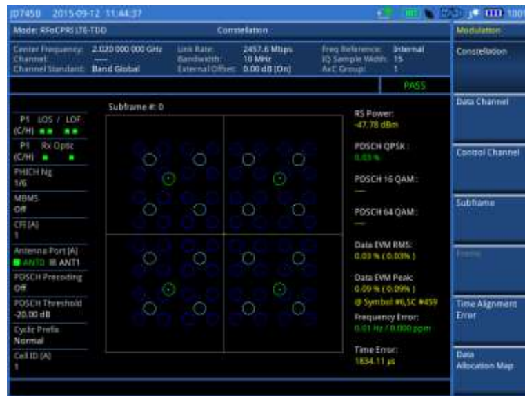
Figure 334 Constellation measurement with RFoCPRI LTE-TDD signal analyzer
