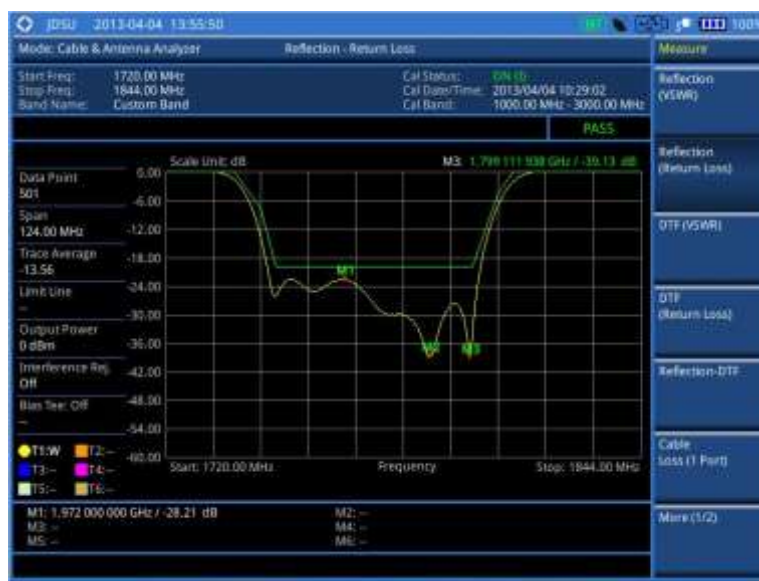
Figure 278 Reflection measurement in return loss scale
