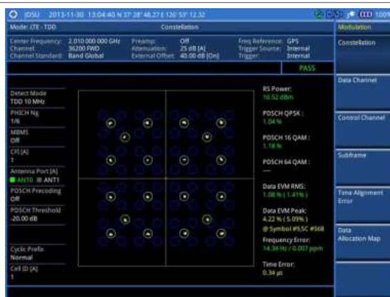
Figure 145 Constellation measurement with LTE-TDD signal analyzer
