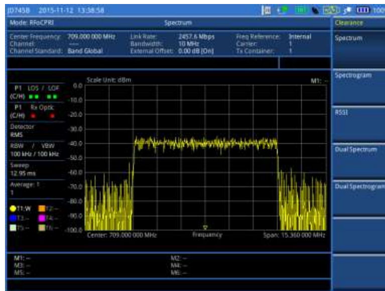
Figure 352 Example of spectrum measurement in BBU emulation
