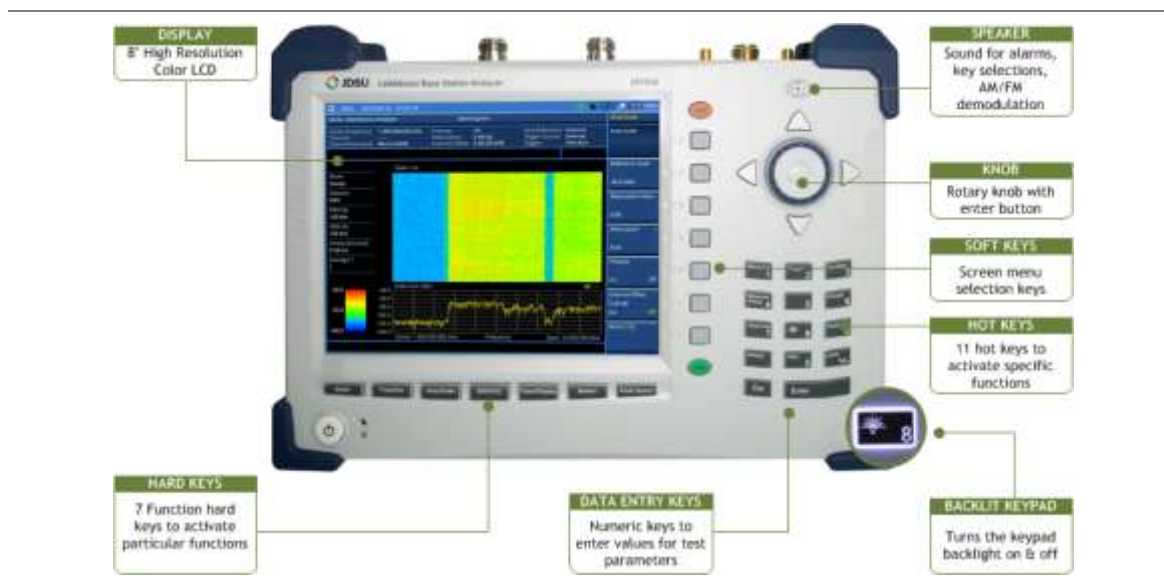
Figure 1 JD785B front panel view
