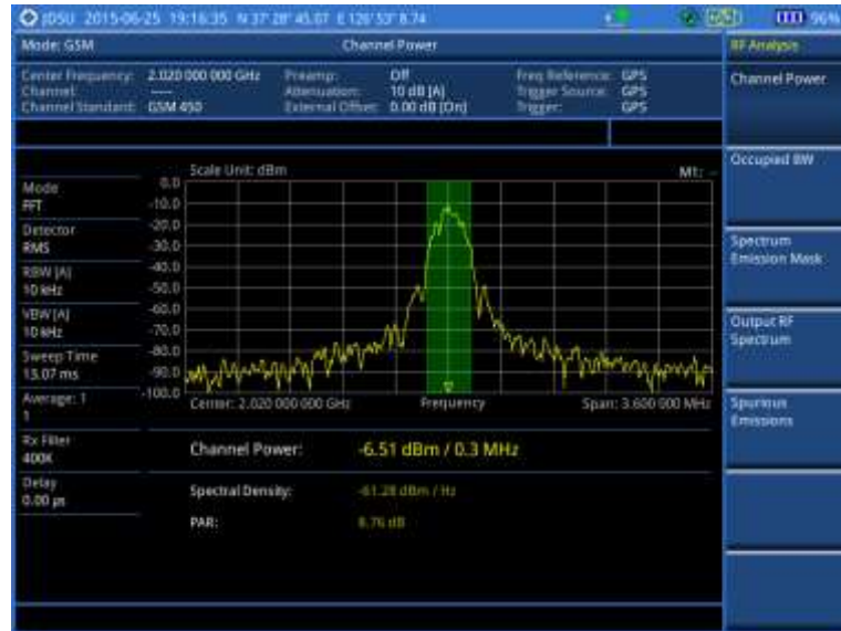
Figure 46 Channel power measurement with GSM signal analyzer
