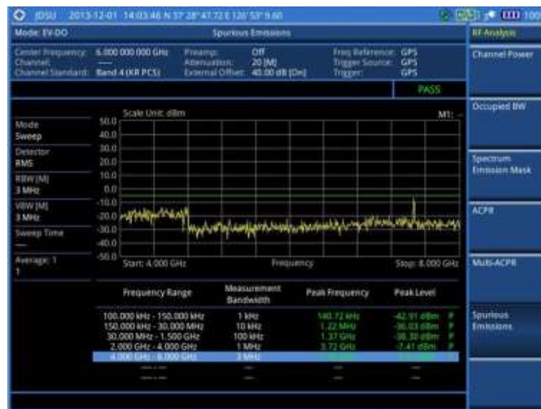
Figure 209 Spurious emissions measurement with EV-DO signal analyzer
