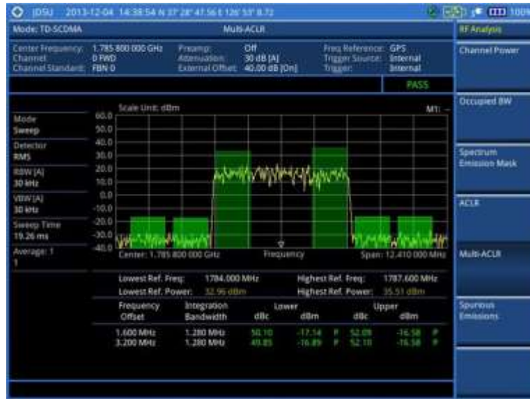
Figure 233 Multi-ACLR measurement with TD-SCDMA signal analyzer
