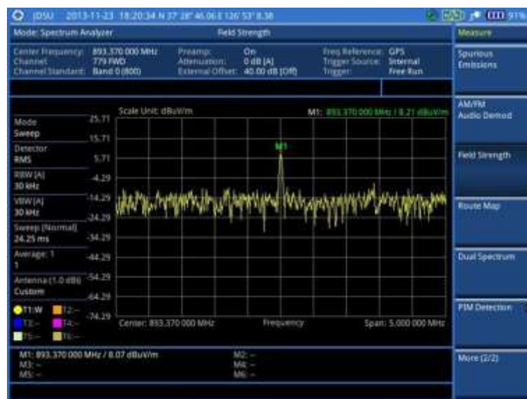
Figure 23 Field strength measurement with spectrum analyzer
