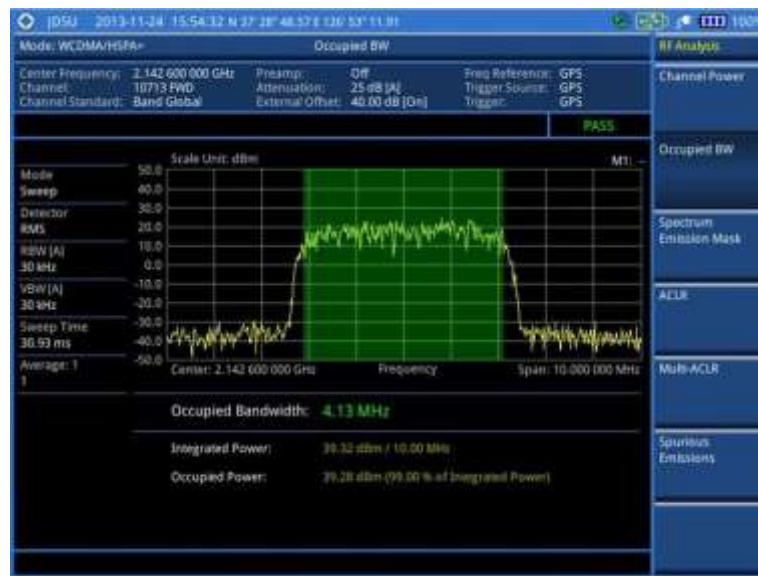
Figure 67 Occupied bandwidth measurement with WCDMA/HSPA+ signal analyzer
