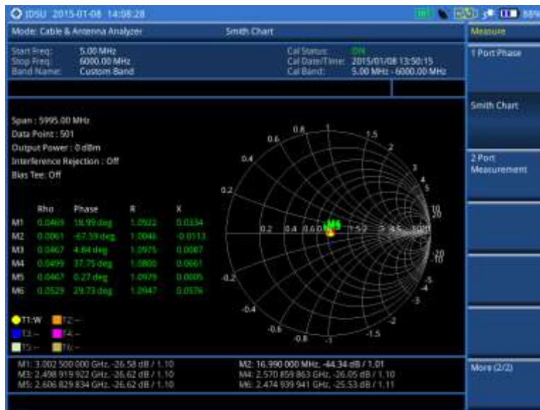
Figure 286 Smith chart measurement
