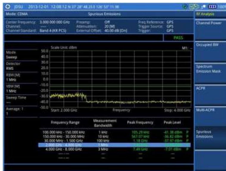
Figure 186 Spurious emissions measurement with CDMA signal analyzer
