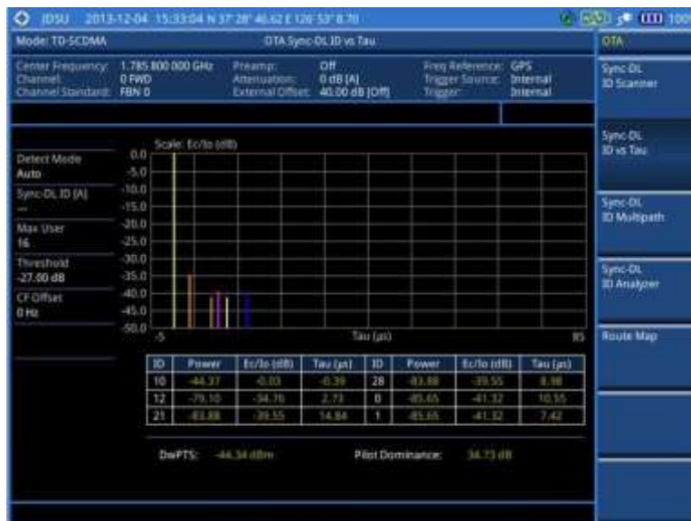
Figure 244 Sync-DL ID vs. Tau measurement with TD-SCDMA OTA signal analyzer
