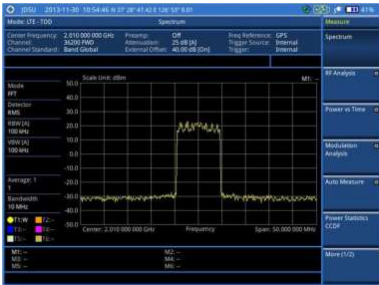
Figure 136 Spectrum measurement screen with LTE-TDD signal analyzer
