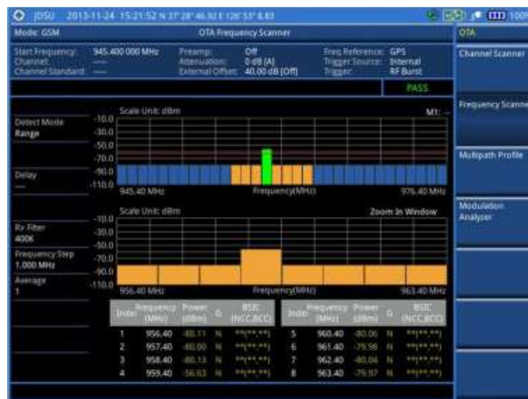
Figure 57 Frequency scanner measurement with GSM OTA signal analyzer
