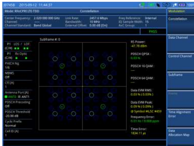
Figure 332 Constellation measurement with RFoCPRI LTE-TDD signal analyzer
