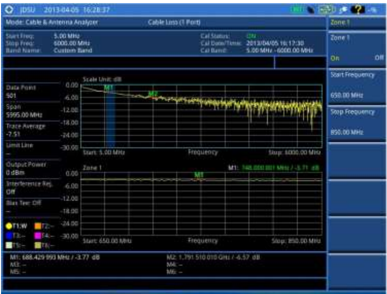
Figure 283 Cable loss (1 port) measurement with the zone enabled
