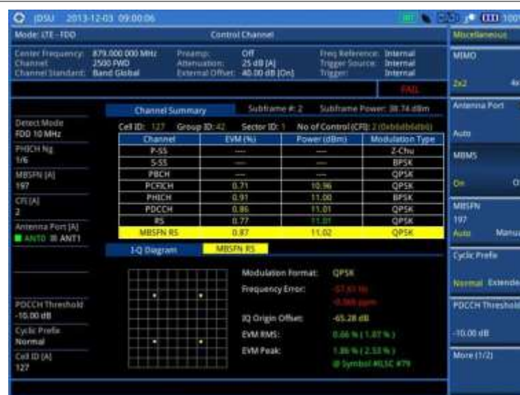
Figure 104 Control channel measurement with LTE-FDD signal analyzer (MBMS On)
