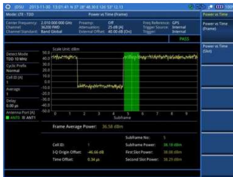
Figure 144 Power vs. time (frame) measurement with LTE – TDD signal analyzer
