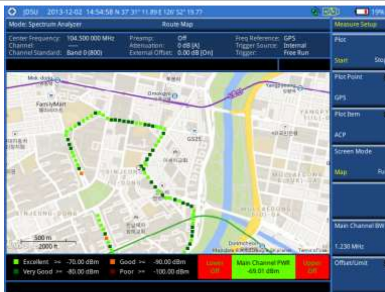
Figure 24 Route map measurement screen with GPS
