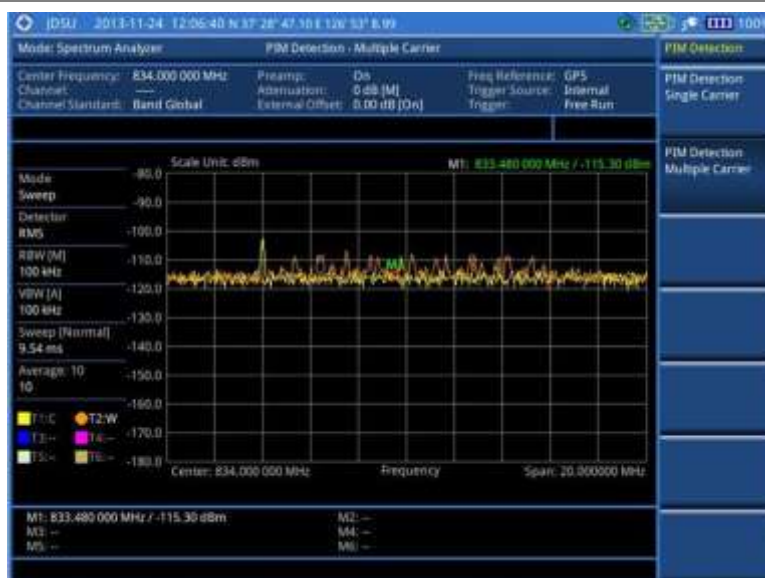
Figure 28 PIM detection for multiple carriers
