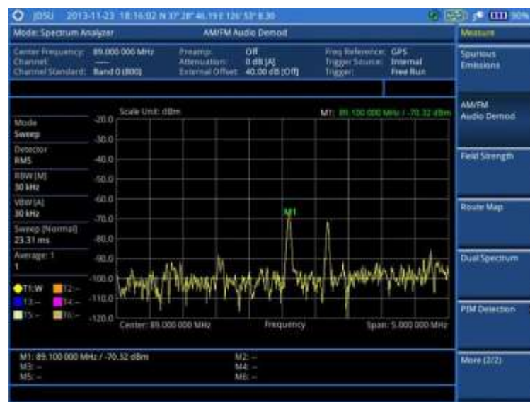
Figure 22 AM/FM audio demodulation with spectrum analyzer
