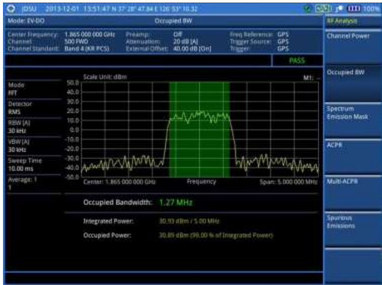
Figure 205 Occupied bandwidth measurement with EV-DO signal analyzer
