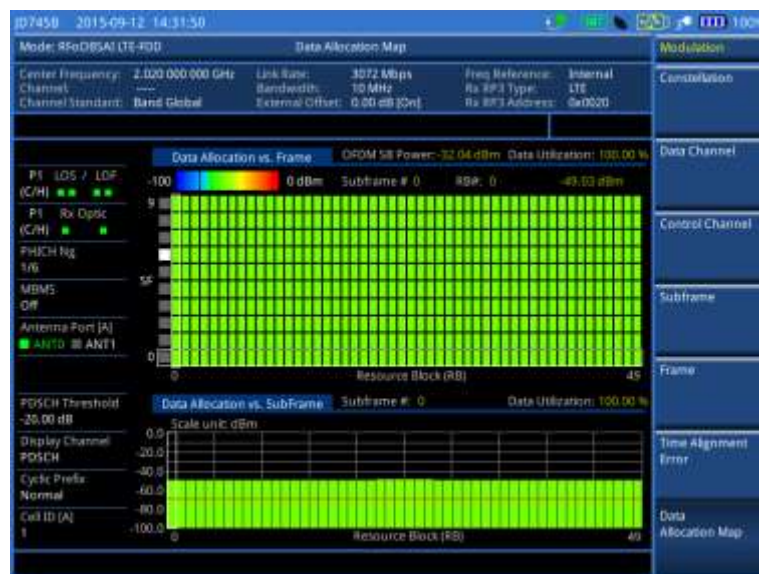
Figure 382 Data allocation map measurement with RFoBSAI LTE-FDD signal analyzer
