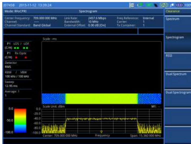
Figure 352 Example of spectrogram in BBU emulation
