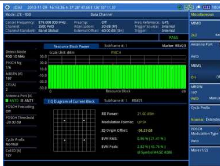
Figure 102 Data channel measurement with LTE-FDD signal analyzer (MBMS On)
