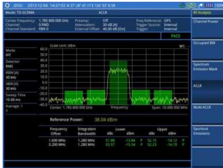
Figure 232 ACLR measurement with TD-SCDMA signal analyzer
