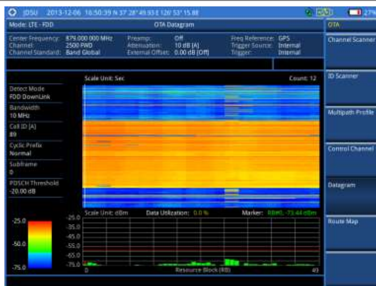
Figure 121 Datagram measurement with LTE-FDD signal analyzer
