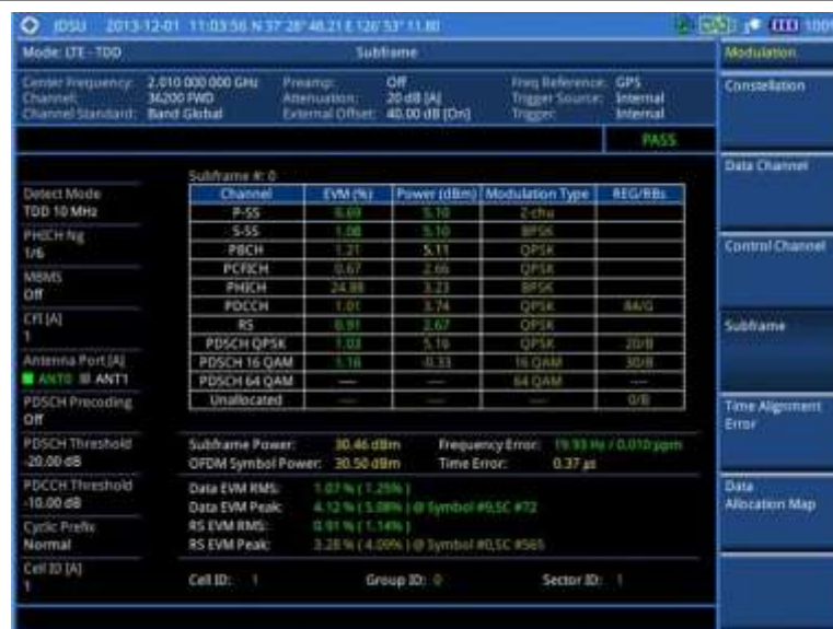
Figure 151 Subframe measurement with LTE-TDD signal analyzer
