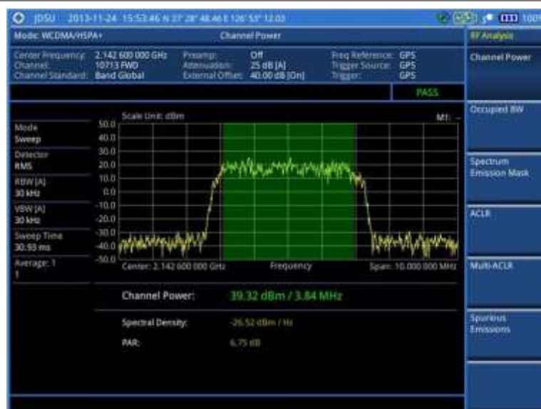
Figure 66 Channel power measurement with WCDMA/HSPA+ signal analyzer
