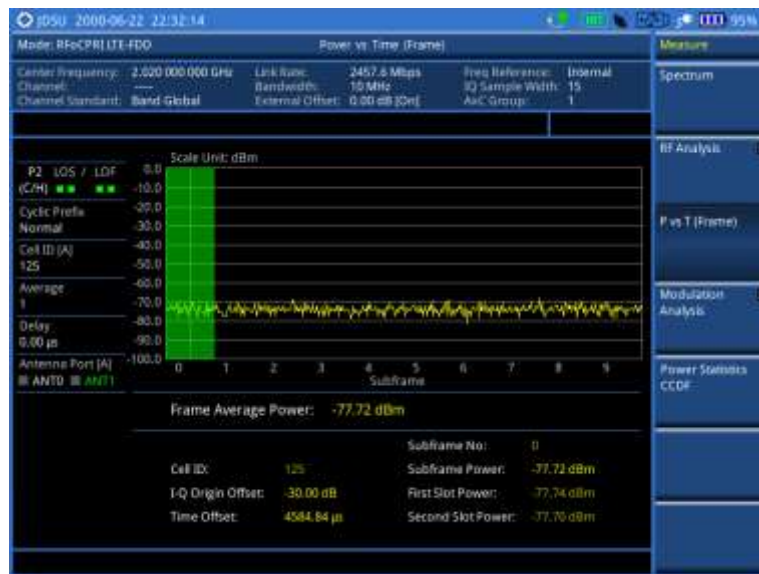
Figure 318 Power vs. time (frame) measurement with RFoCPRI LTE-FDD signal analyzer
