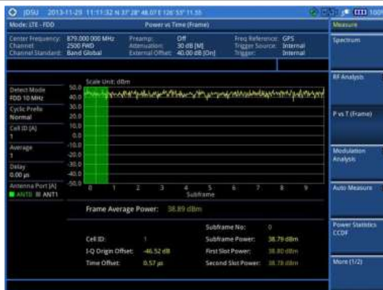
Figure 98 Power vs. time (frame) measurement with LTE – FDD signal analyzer
