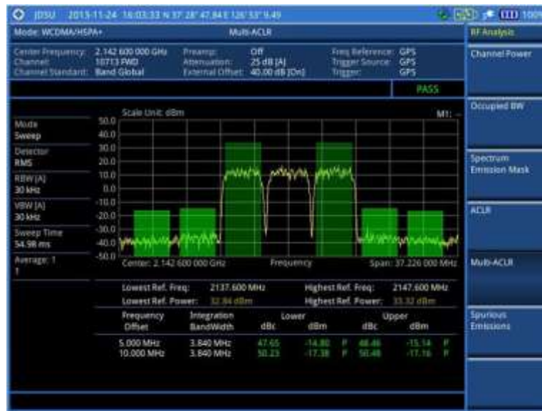
Figure 70 Multi-ACLR measurement with WCDMA/HSPA+ signal analyzer
