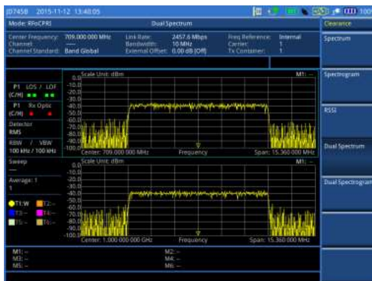
Figure 351 Example of dual spectrum analysis in BBU emulation
