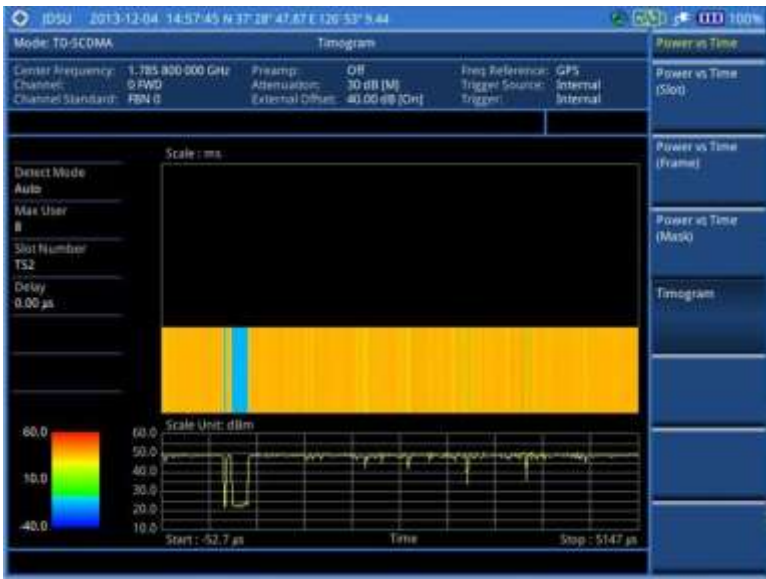
Figure 238 Timogram with TD-SCDMA signal analyzer
