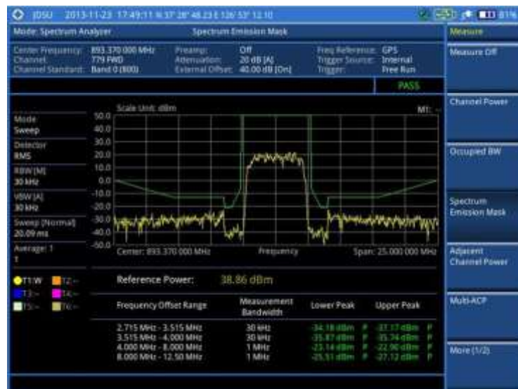
Figure 18 Spectrum emission mask measurement with spectrum analyzer
