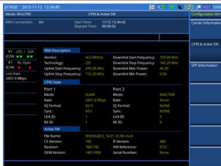
Figure 346 Example of verification of CPRI state and active software
