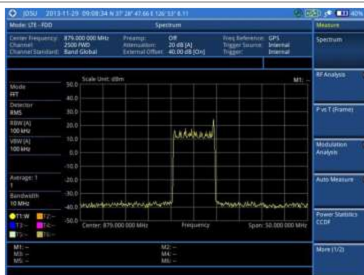
Figure 91 Spectrum measurement screen with LTE-FDD signal analyzer
