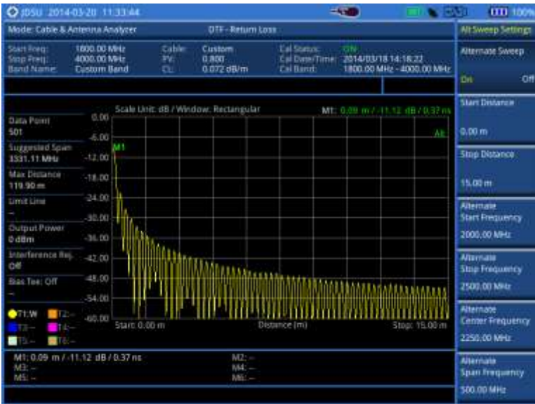
Figure 280 DTF measurement with the alternate sweep on
