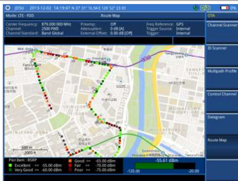
Figure 122 Route map measurement (RSRP) with LTE-FDD OTA signal analyzer
