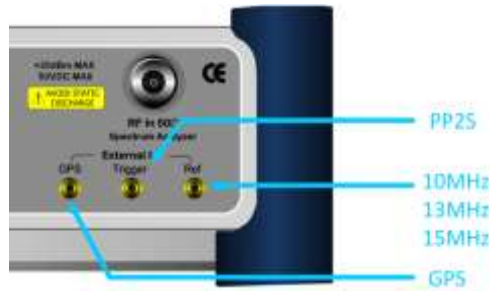
Figure 179 Connection ports for external reference clock
