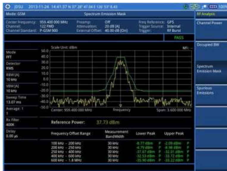
Figure 48 SEM measurement with GSM signal analyzer
