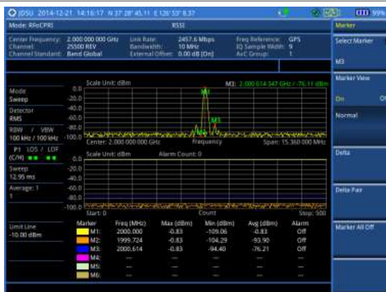
Figure 308 RFoCPRI interference measurement in RSSI
