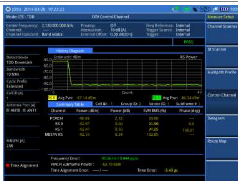
Figure 164 Control channel measurement with LTE-TDD OTA signal analyzer
