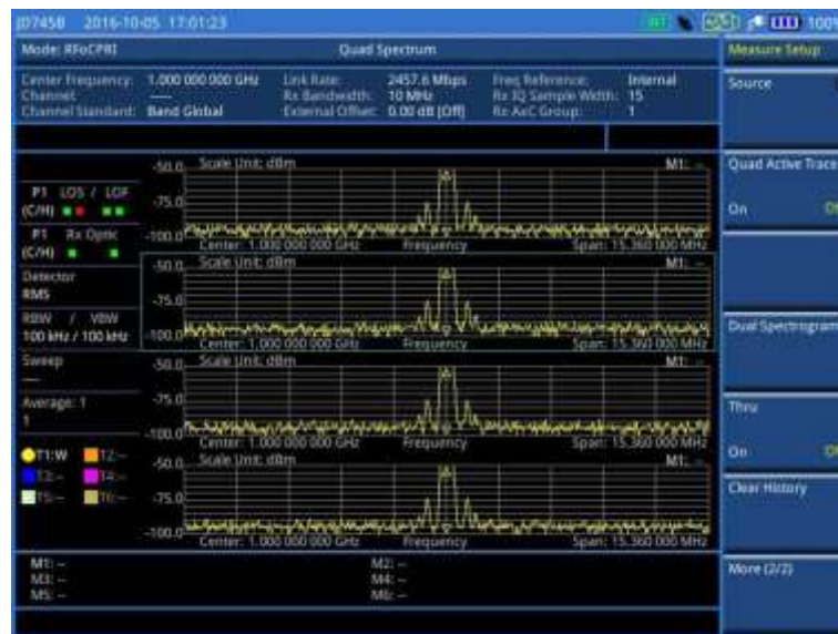
Figure 305 RFoCPRI quad spectrum with quad active trace on
