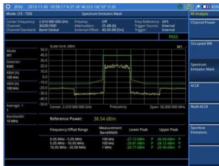
Figure 139 SEM measurement with LTE-TDD signal analyzer
