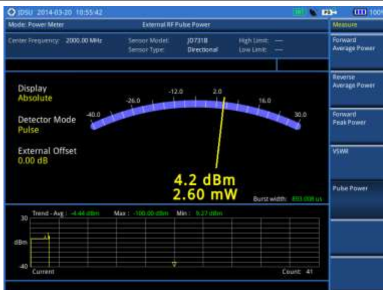
Figure 396 External power measurement of pulse power
