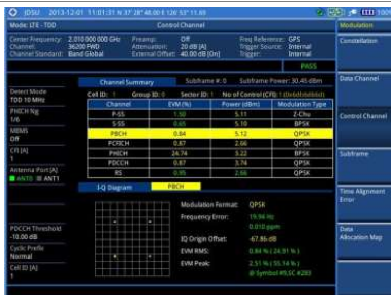
Figure 149 Control channel measurement with LTE-TDD signal analyzer
