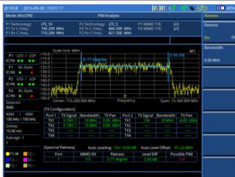
Figure 357 Example of Wideband Mode PIM analysis in BBU emulation
