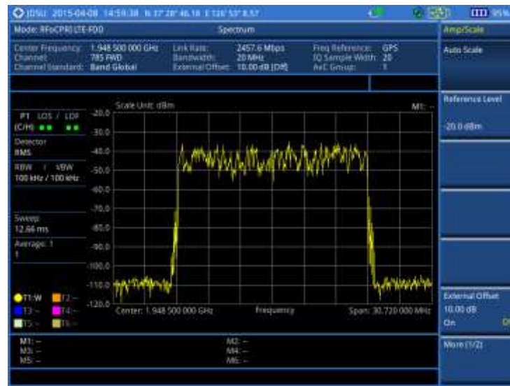
Figure 315 Spectrum measurement with RFoCPRI LTE-FDD signal analyzer
