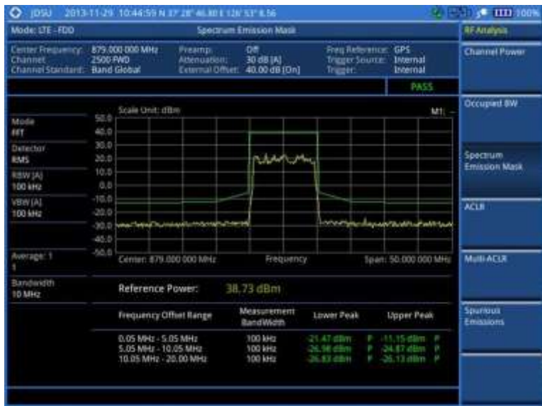
Figure 94 SEM measurement with LTE-FDD signal analyzer
