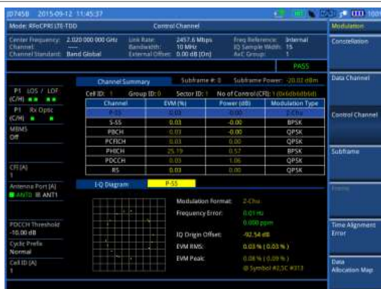
Figure 334 Control channel measurement with RFoCPRI LTE-TDD signal analyzer
