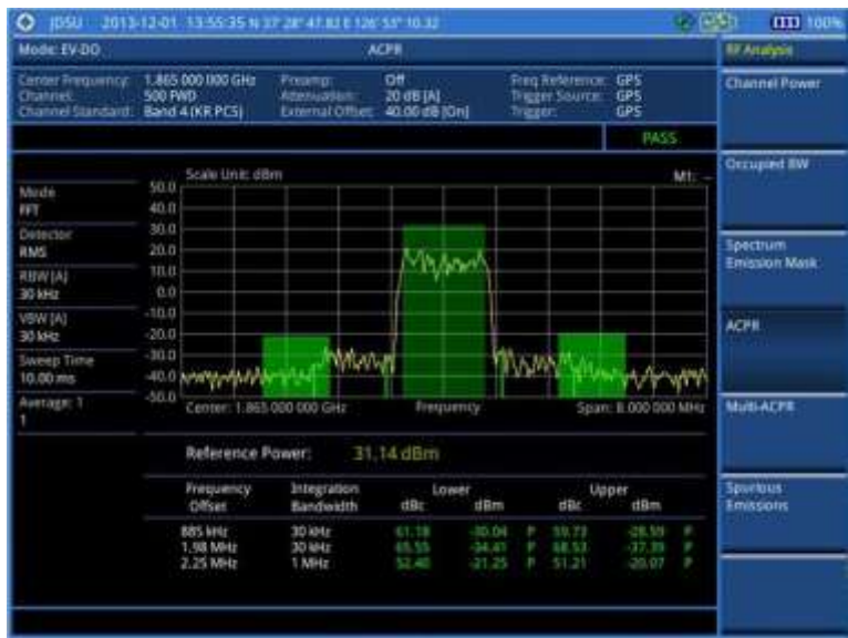
Figure 207 ACPR measurement with EV-DO signal analyzer
