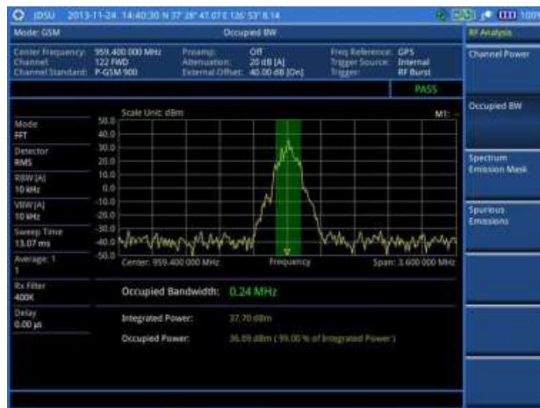
Figure 47 Occupied bandwidth measurement with GSM signal analyzer
