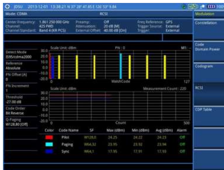
Figure 190 RCSI measurement with CDMA signal analyzer
