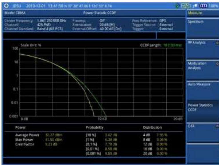
Figure 192 CCDF measurement with CDMA signal analyzer
