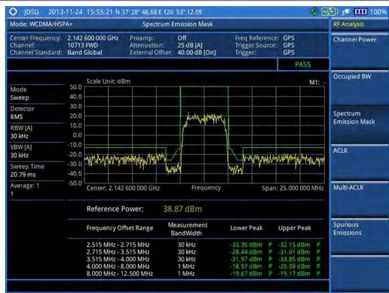
Figure 64 SEM measurement with WCDMA/HSPA+ signal analyzer
