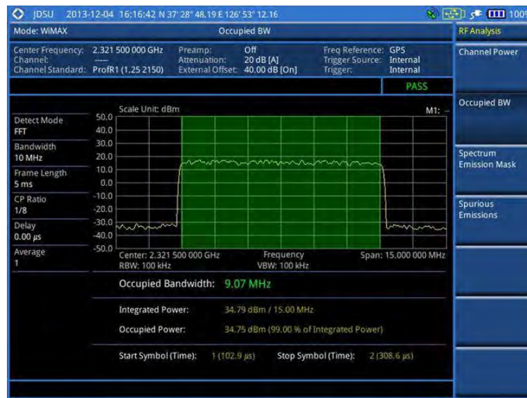
Figure 251 Occupied bandwidth measurement with Mobile WiMAX signal analyzer
