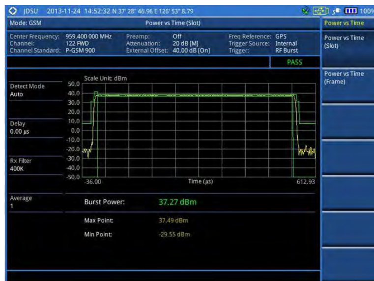
Figure 47 Power vs. time (slot) measurement with GSM signal analyzer
