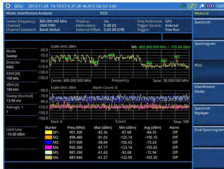
Figure 32 Interference measurement in RSSI
