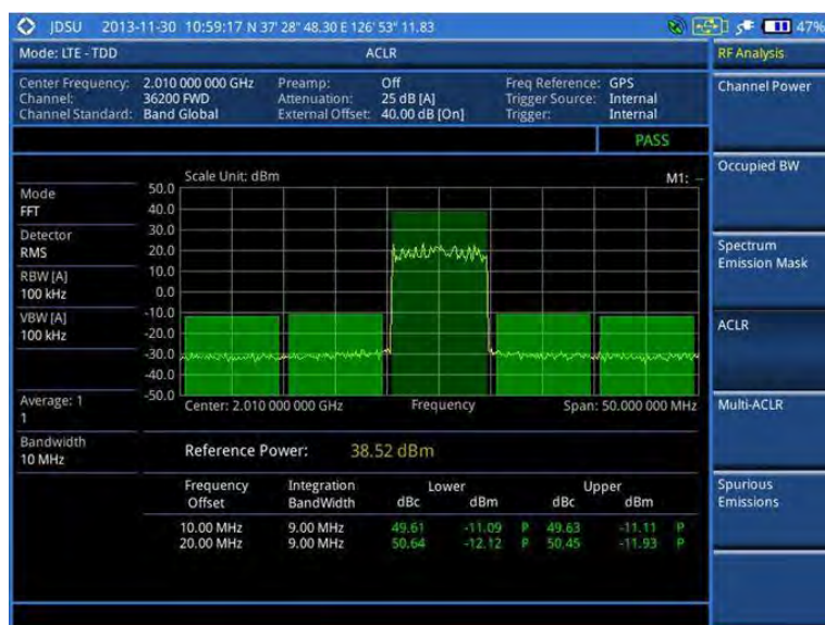
Figure 136 ACLR measurement with LTE-TDD signal analyzer
