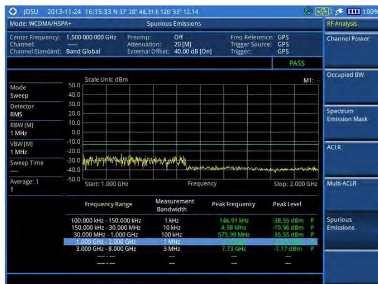
Figure 67 Spurious emissions measurement with WCDMA/HSPA+ signal analyzer
