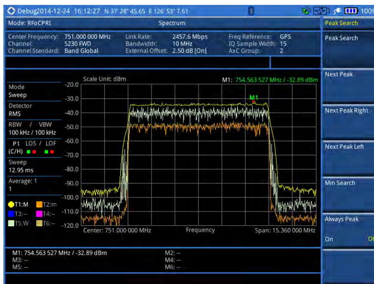
Figure 295 RFoCPRI spectrum analysis on LTE Uplink 10 MHz, antenna 2
