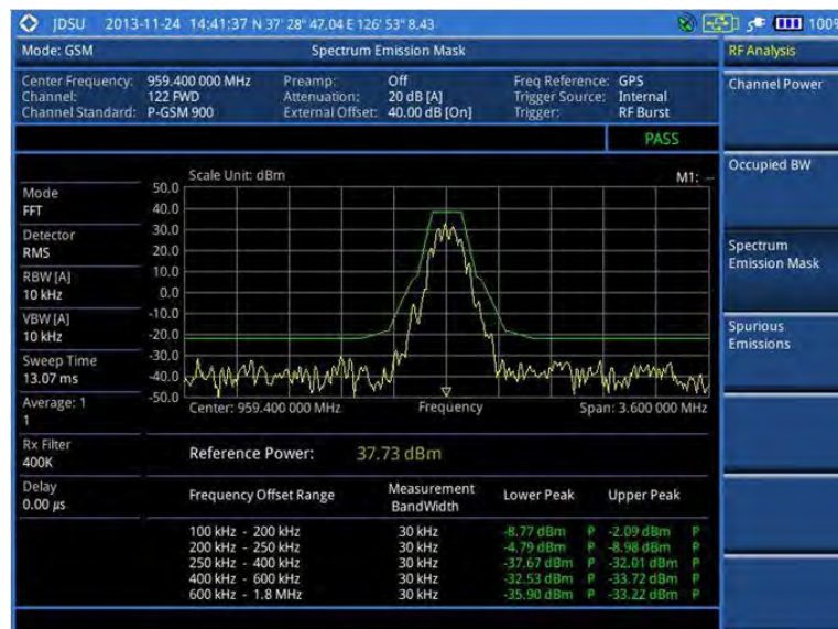
Figure 44 SEM measurement with GSM signal analyzer
