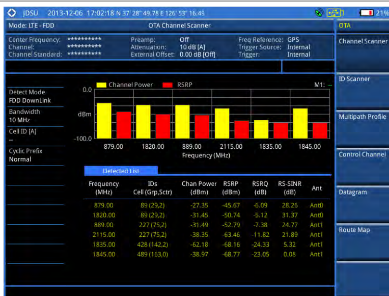
Figure 113 Channel scanner measurement with LTE-FDD OTA signal analyzer
