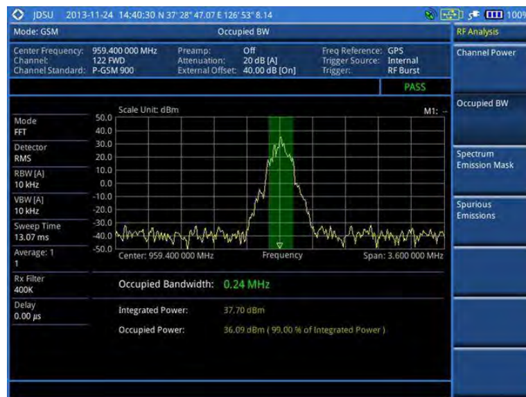
Figure 43 Occupied bandwidth measurement with GSM signal analyzer
