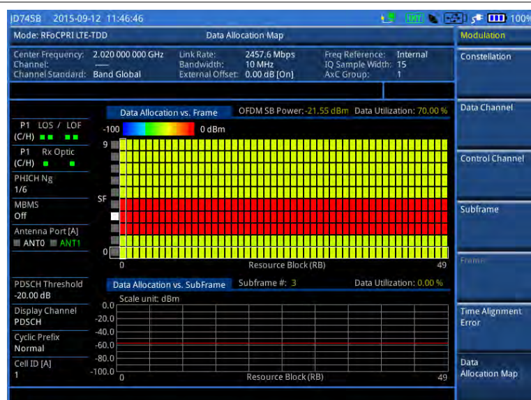
Figure 330 Data allocation map measurement with RFoCPRI LTE-TDD signal analyzer
