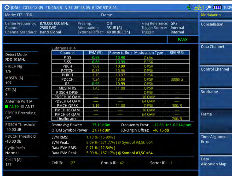
Figure 105 Frame measurement with LTE-FDD signal analyzer (MBMS On)
