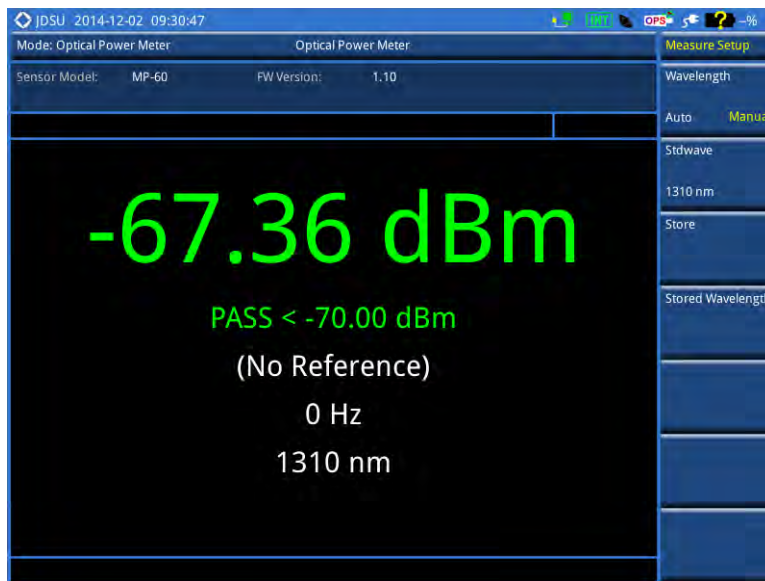
Figure 389 optical power measurement
