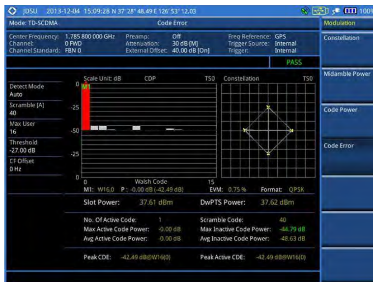
Figure 238 Code error measurement with TD-SCDMA signal analyzer
