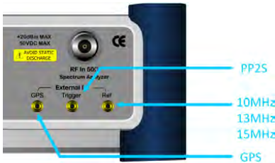
Figure 131 Connection ports for external reference clock
