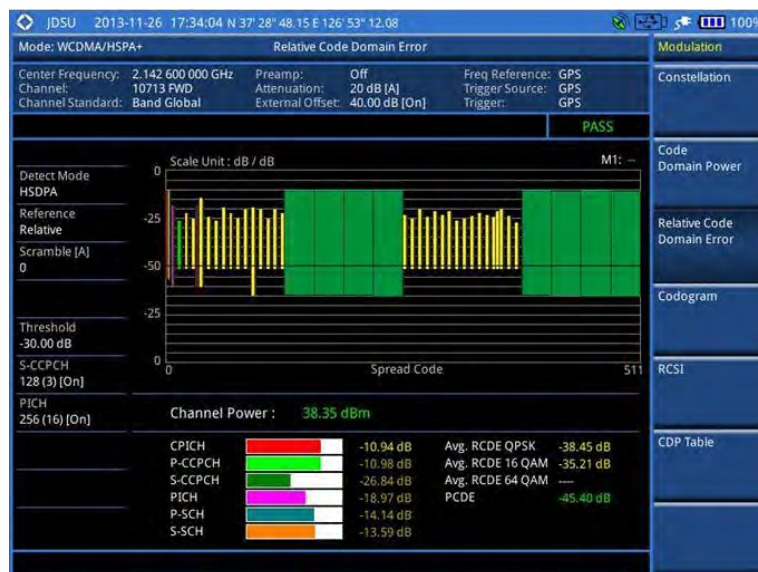
Figure 70 Relative code domain error with WCDMA/HSPA+ signal analyzer
