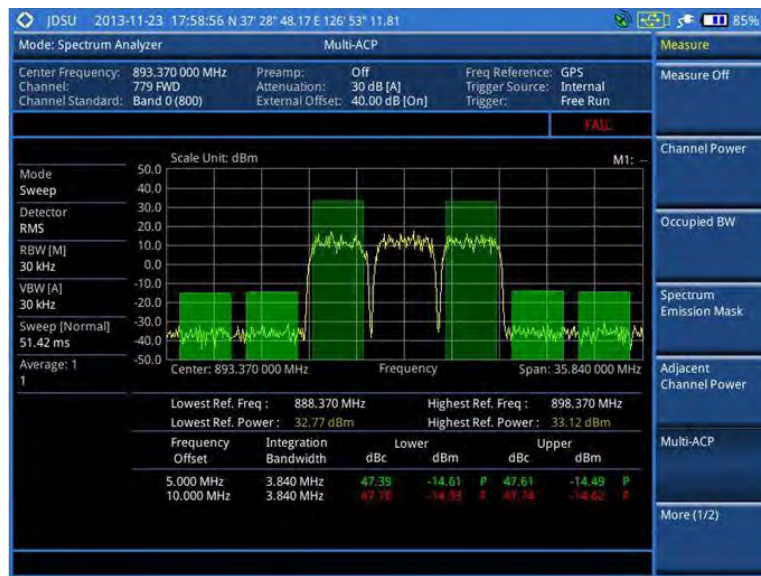
Figure 17 Multi-ACP measurement with spectrum analyzer
