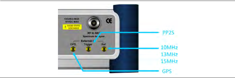
Figure 248 Connection ports for external reference clock
