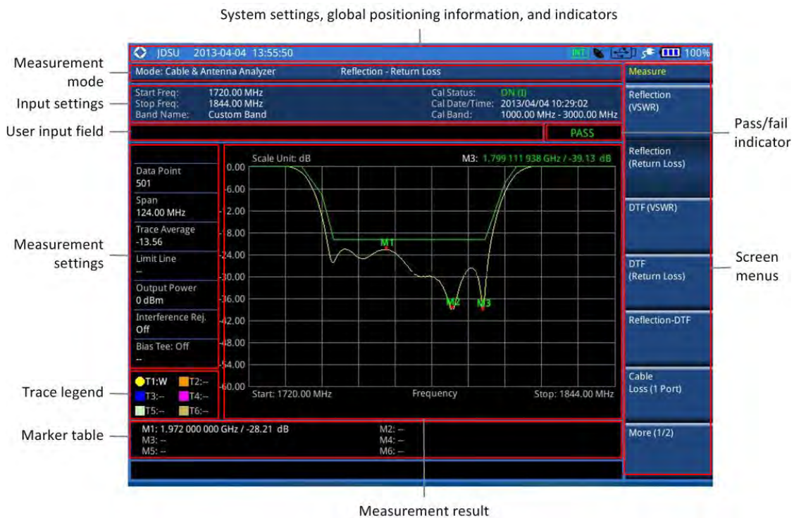
Figure 264 Reflection measurement screen
