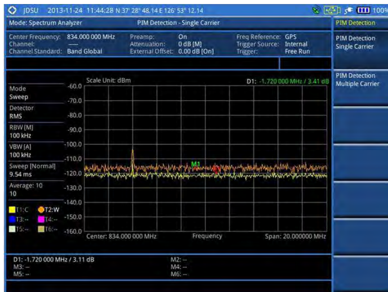
Figure 25 PIM detection for multiple carriers
