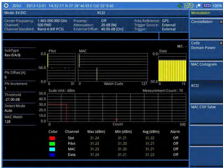
Figure 211 RCSI measurement with EV-DO signal analyzer
