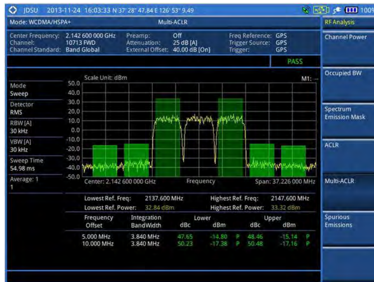
Figure 66 Multi-ACLR measurement with WCDMA/HSPA+ signal analyzer
