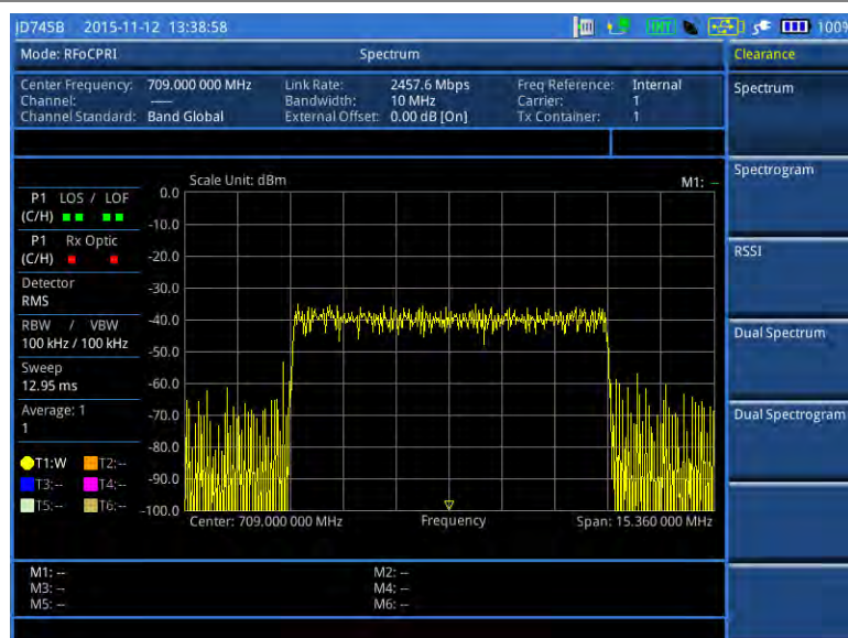
Figure 343 Example of spectrum measurement in BBU emulation
