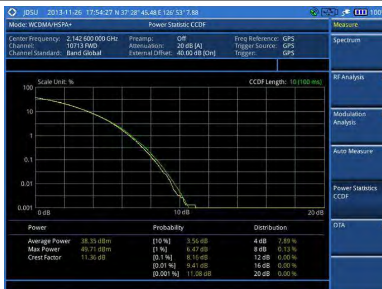
Figure 74 CCDF measurement with WCDMA/HSPA+ signal analyzer
