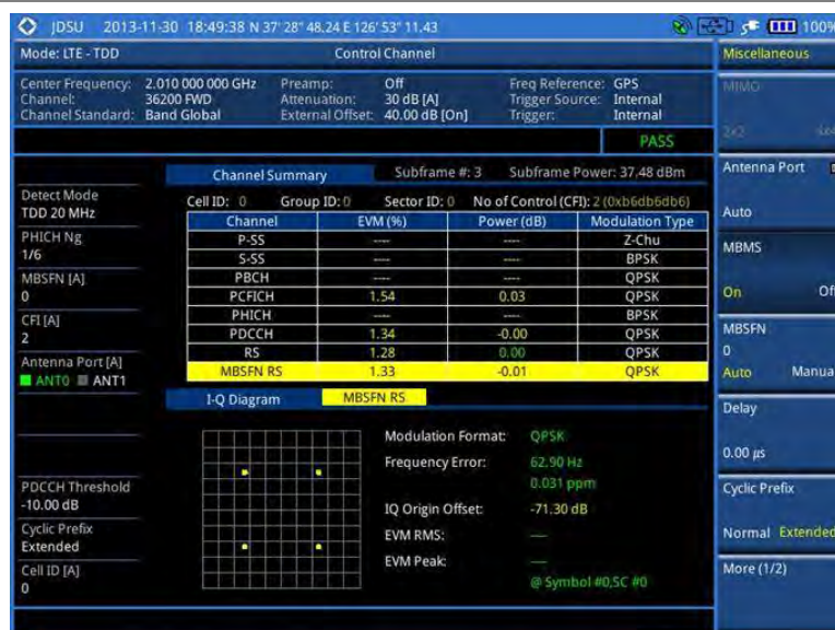
Figure 146 Control channel measurement with LTE-TDD signal analyzer (MBMS On)
