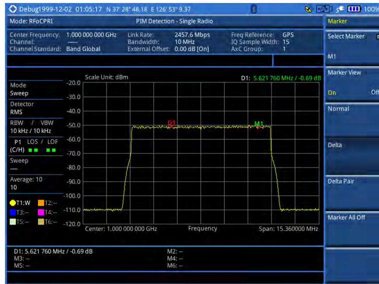
Figure 305 PIM detection of single radio
