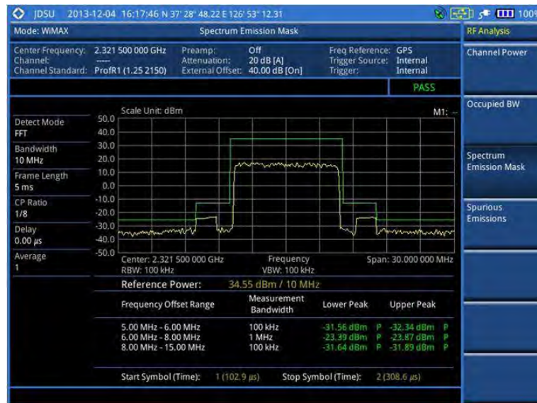
Figure 252 SEM measurement with Mobile WiMAX signal analyzer
