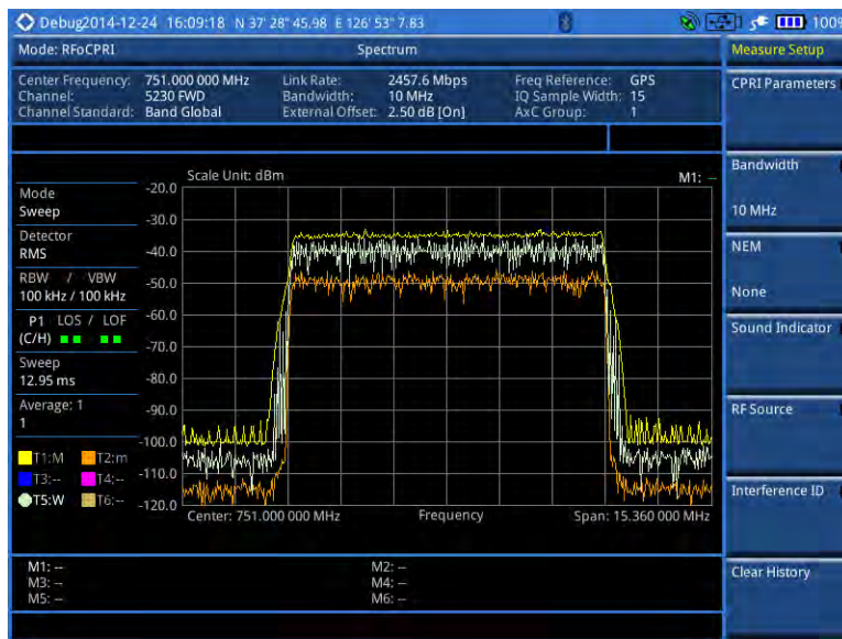
Figure 294 RFoCPRI spectrum analysis on LTE Uplink 10 MHz, antenna 1
