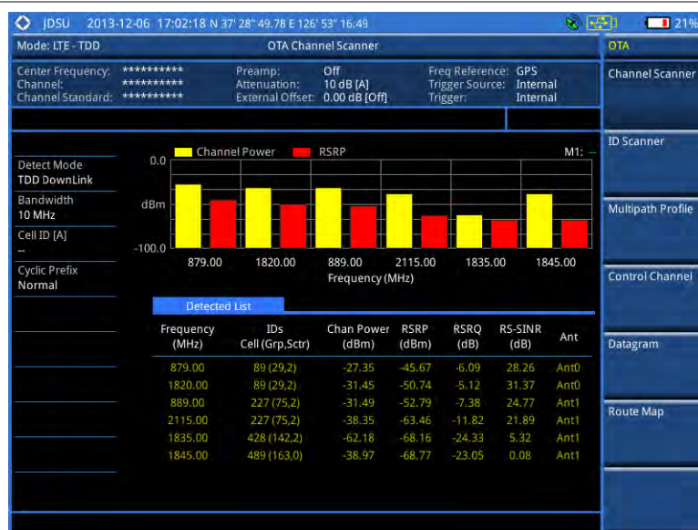
Figure 157 Channel scanner measurement with LTE-TDD OTA signal analyzer
