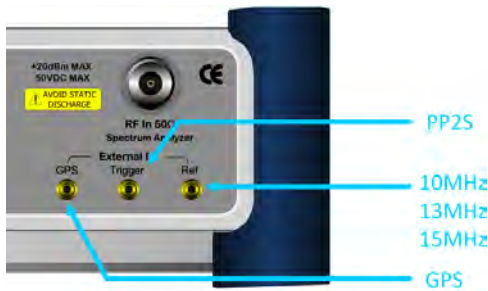
Figure 223 Connection ports for external reference clock
