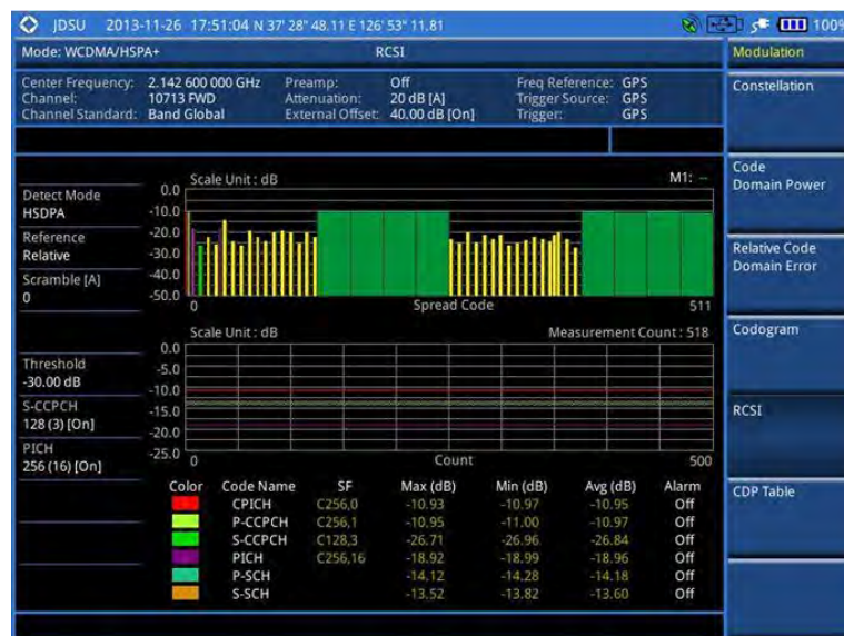
Figure 72 RCSI measurement with WCDMA/HSPA+ signal analyzer
