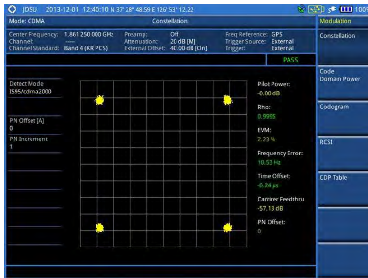
Figure 183 Constellation measurement with CDMA signal analyzer
