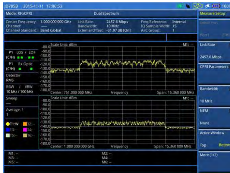
Figure 298 RFoCPRI dual spectrum with dual active trace on
