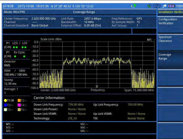
Figure 348 Example of coverage range in BBU emulation
