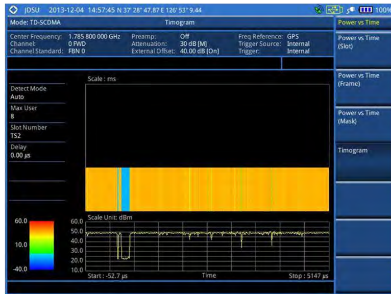
Figure 234 Timogram with TD-SCDMA signal analyzer
