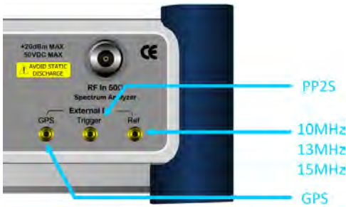
Figure 198 Connection ports for external reference clock
