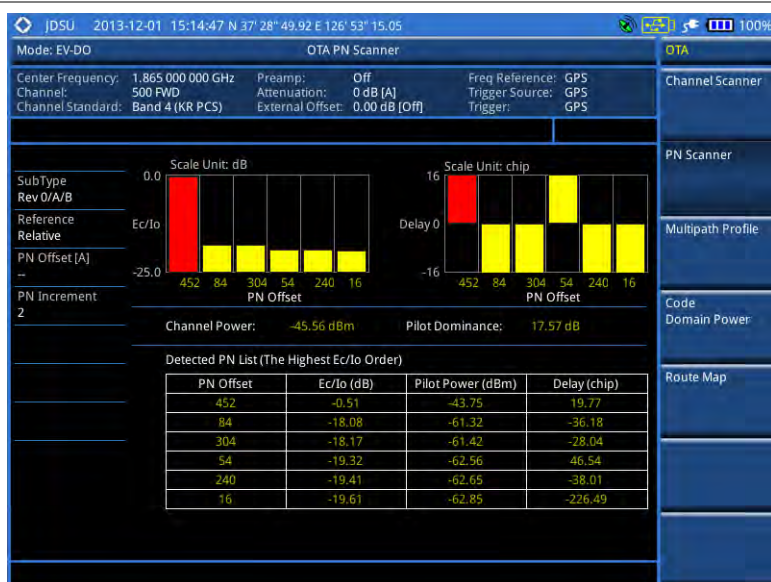
Figure 215 PN scanner measurement with EV-DO OTA signal analyzer
