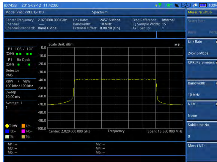
Figure 321 Spectrum measurement with RFoCPRI LTE-TDD signal analyzer
