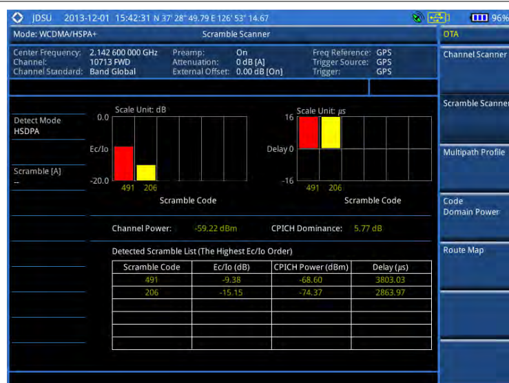
Figure 76 Scramble scanner measurement with WCDMA/HSPA+ OTA signal analyzer
