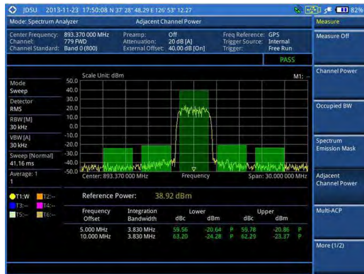
Figure 16 Adjacent channel power measurement with spectrum analyzer
