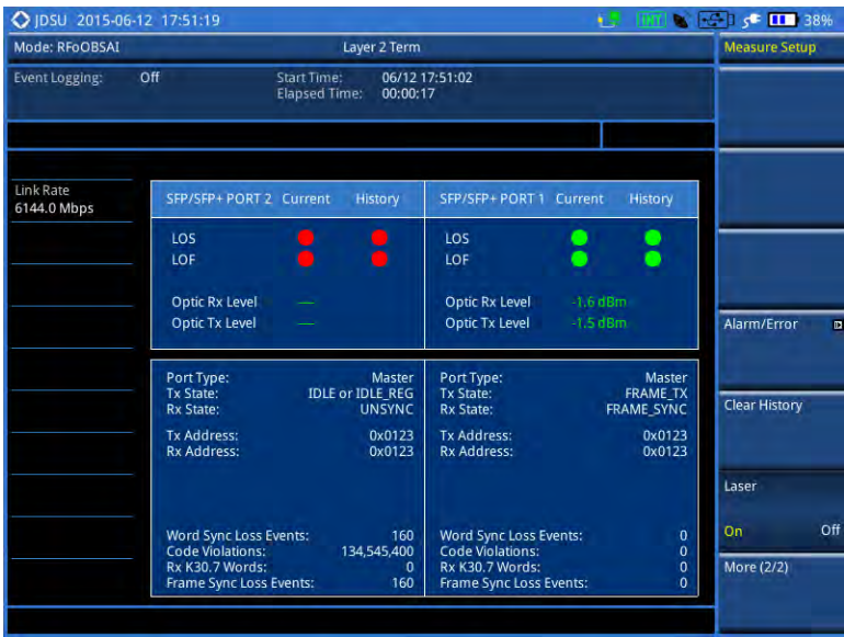
Figure 354 OBSAI layer 2 term test
