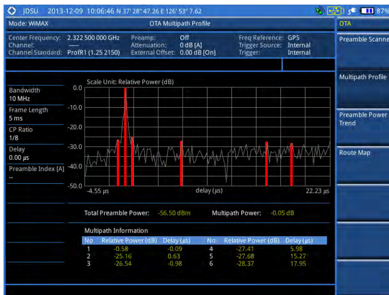
Figure 261 Multipath profile measurement with Mobile WiMAX OTA signal analyzer
