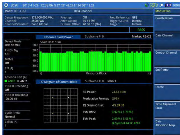
Figure 97 Data channel measurement with LTE-FDD signal analyzer
