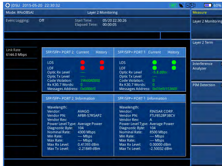
Figure 352 OBSAI RP3 layer 2 monitoring
