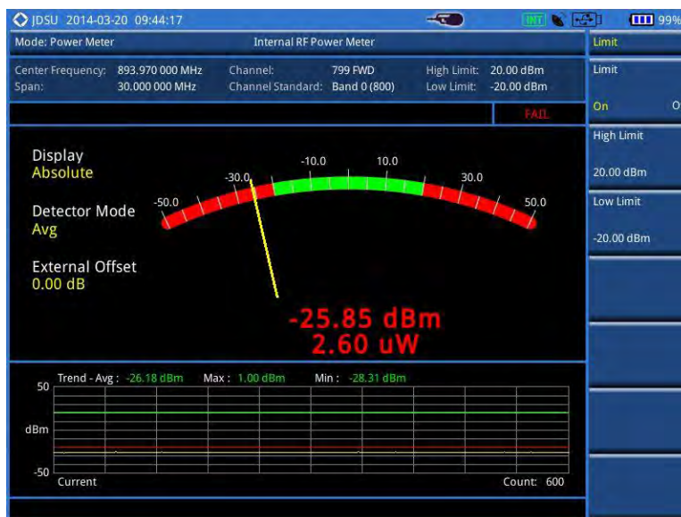
Figure 385 Internal power measurement
