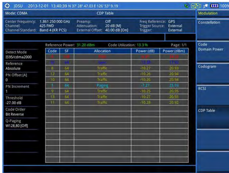
Figure 187 CDP Table measurement with CDMA signal analyzer
