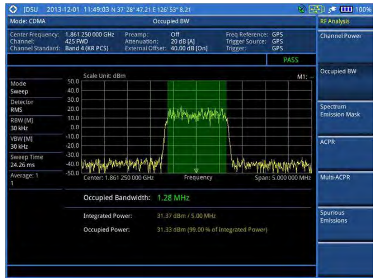
Figure 178 Occupied bandwidth measurement with CDMA signal analyzer
