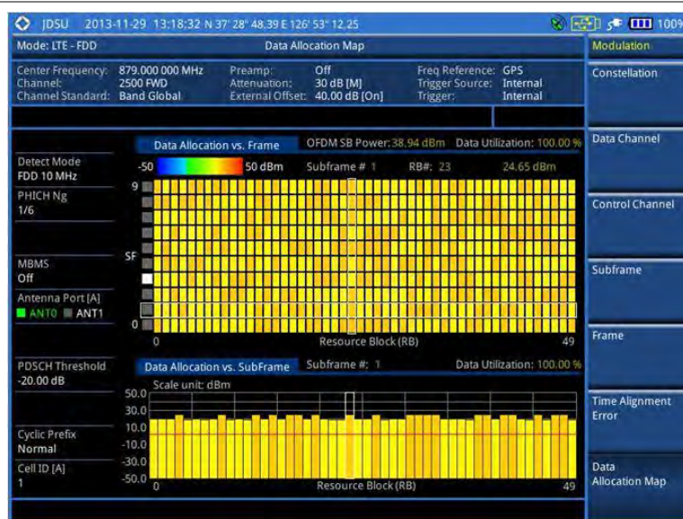
Figure 108 Data allocation map measurement with LTE-FDD signal analyzer (MBMS On)
