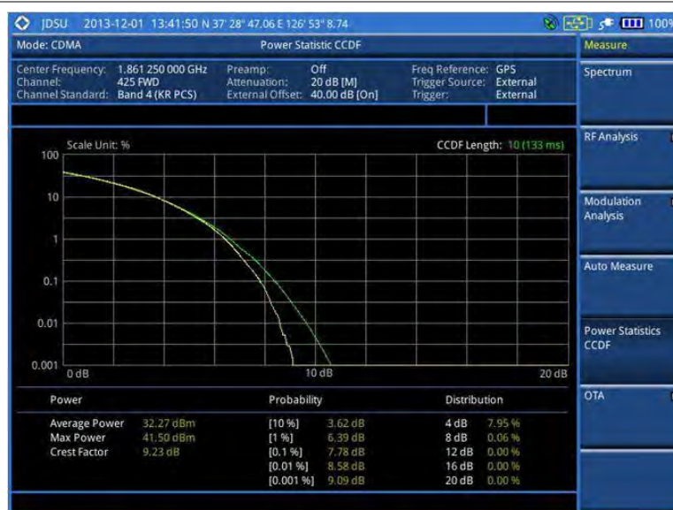
Figure 188 CCDF measurement with CDMA signal analyzer
