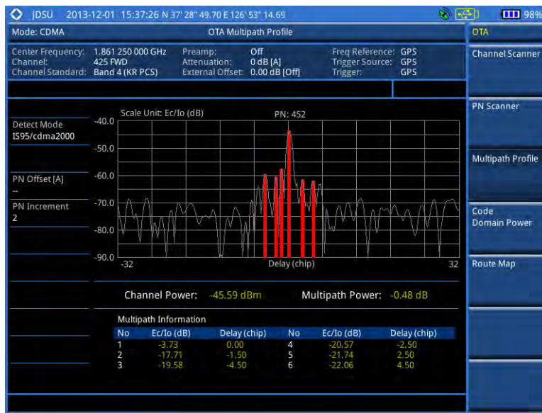
Figure 191 Multipath profile measurement with CDMA OTA signal analyzer
