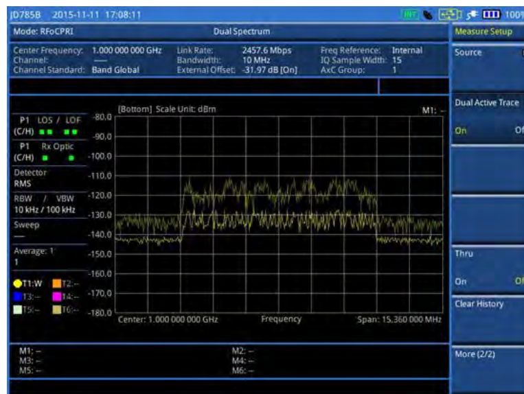
Figure 298 RFoCPRI dual spectrum with dual active trace on
