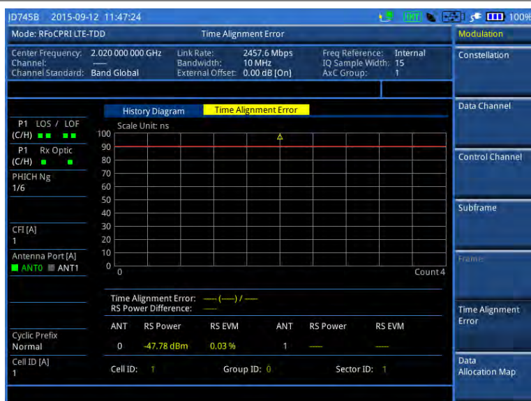
Figure 329 Time alignment error measurement with RFoCPRI LTE-TDD signal analyzer
