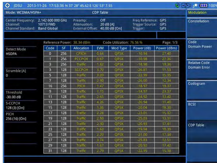
Figure 73 CDP Table measurement with WCDMA/HSPA+ signal analyzer
