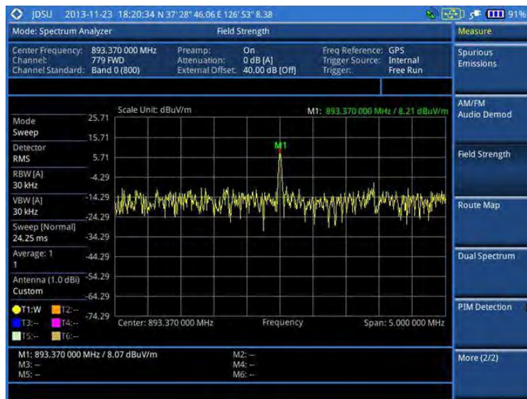
Figure 20 Field strength measurement with spectrum analyzer
