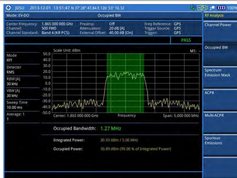
Figure 201 Occupied bandwidth measurement with EV-DO signal analyzer
