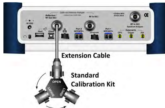
Figure 265 1-port calibration connection with mechanical Y-Cal kit
