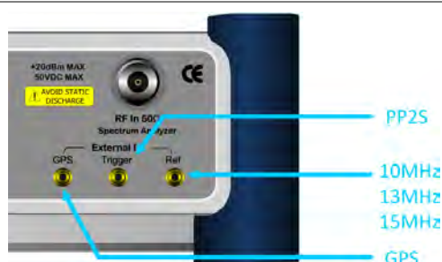
Figure 60 Connection ports for external reference clock
