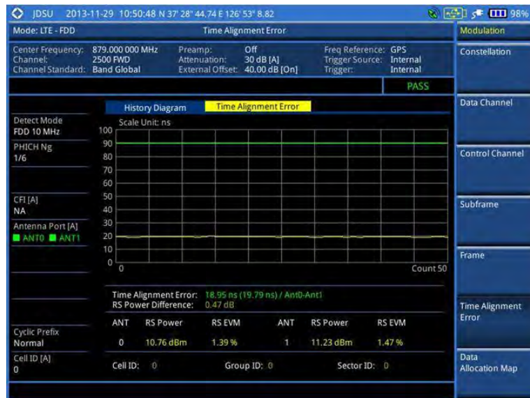
Figure 106 Time alignment error measurement with LTE-FDD signal analyzer
