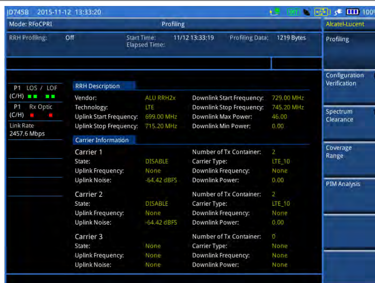
Figure 334 Example of RRH profiling results with carrier information
