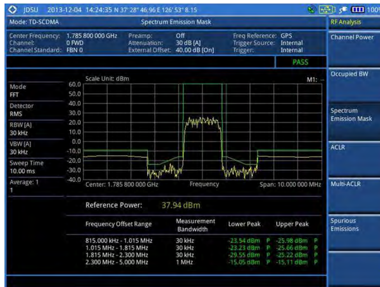
Figure 227 SEM measurement with TD-SCDMA signal analyzer
