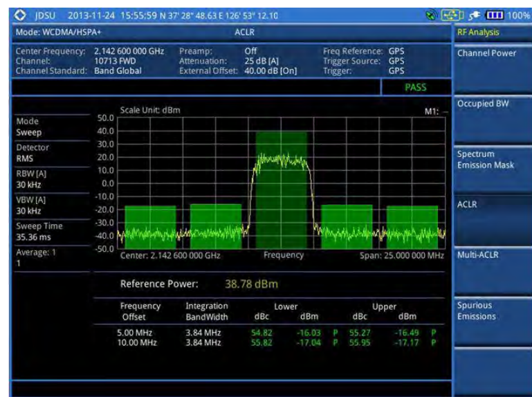
Figure 65 ACLR measurement with WCDMA/HSPA+ signal analyzer
