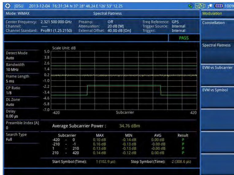
Figure 256 Spectral flatness measurement with Mobile WiMAX signal analyzer
