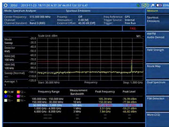
Figure 18 Spurious emissions measurement with spectrum analyzer
