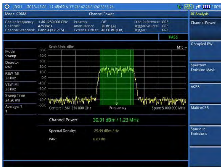
Figure 177 Channel power measurement with CDMA signal analyzer
