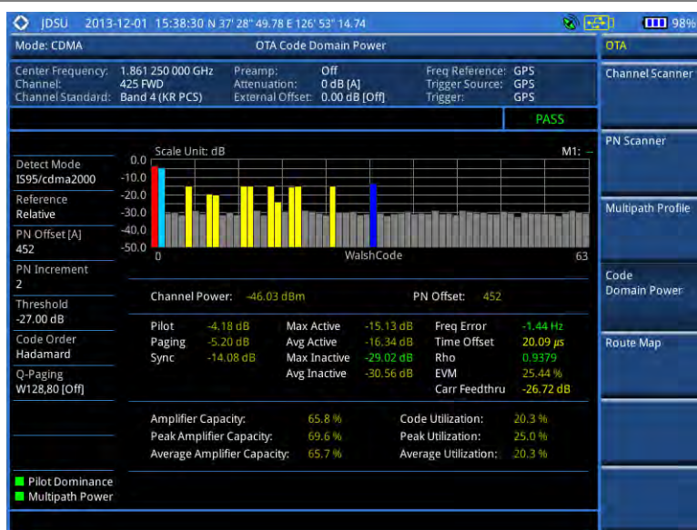
Figure 192 Code domain power measurement with CDMA OTA signal analyzer
