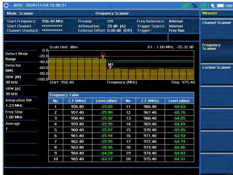
Figure 380 Frequency scanner measurement
