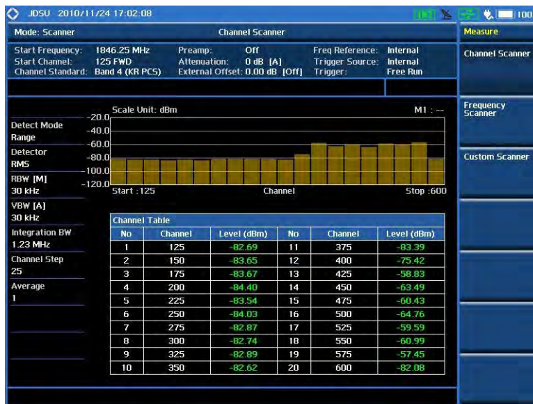
Figure 379 Channel scanner measurement
