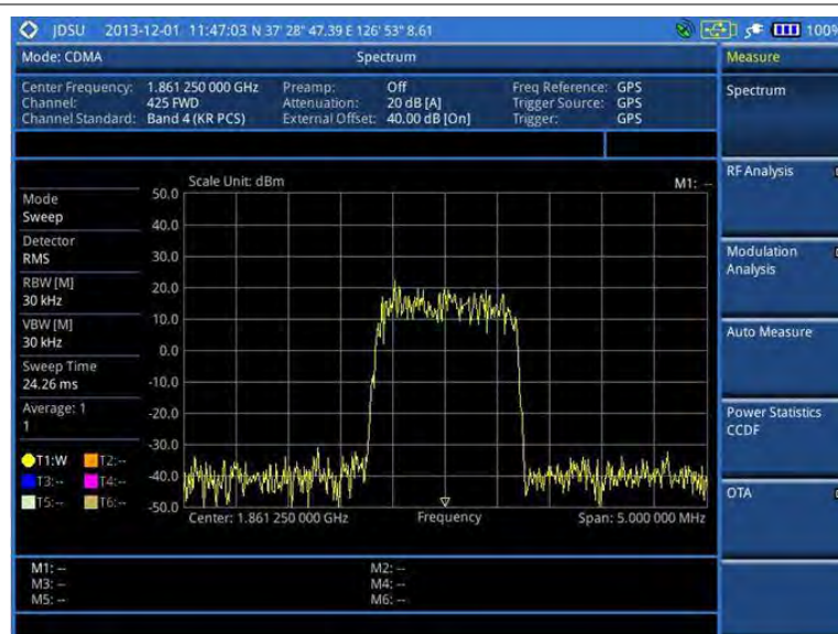
Figure 176 Spectrum measurement screen with CDMA signal analyzer
