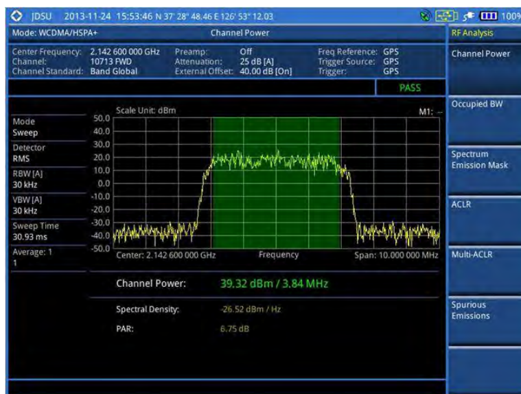
Figure 62 Channel power measurement with WCDMA/HSPA+ signal analyzer
