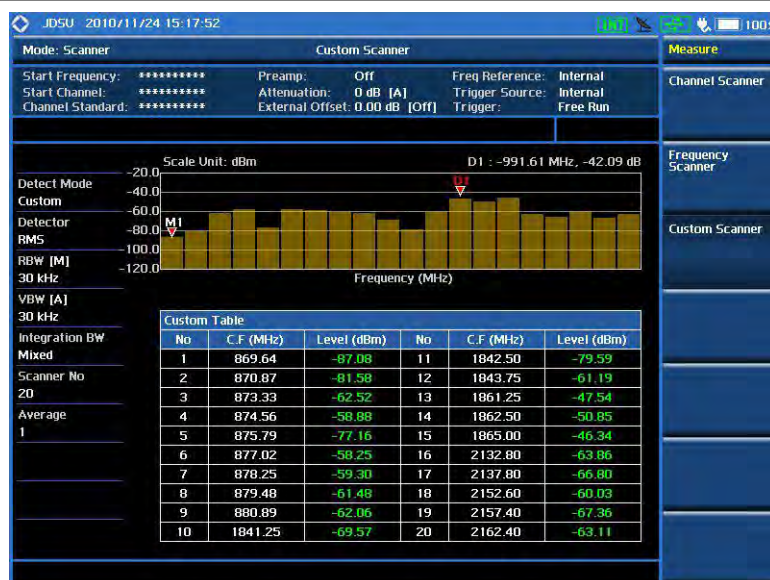
Figure 381 Custom scanner measurement
