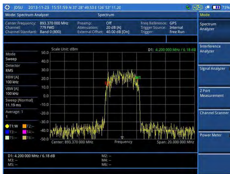
Figure 11 Spectrum measurement with spectrum analyzer
