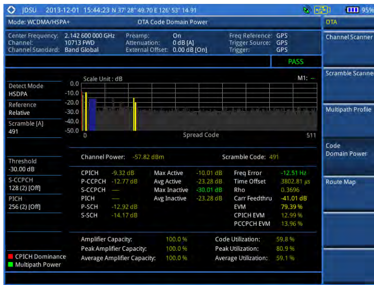
Figure 78 Code domain power measurement with WCDMA/HSPA+ OTA signal analyzer
