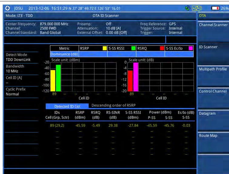
Figure 158 ID scanner measurement with LTE-TDD OTA signal analyzer
