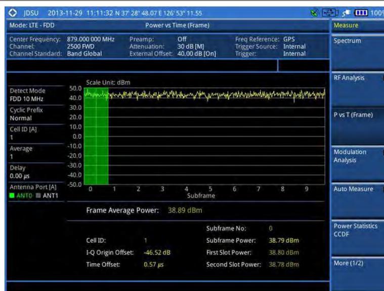
Figure 94 Power vs. time (frame) measurement with LTE – FDD signal analyzer
