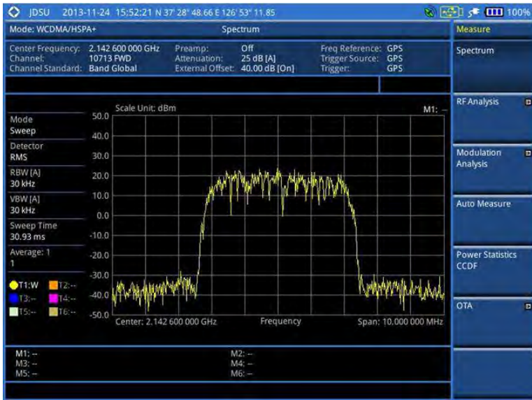
Figure 61 Spectrum measurement screen with WCDMA signal analyzer
