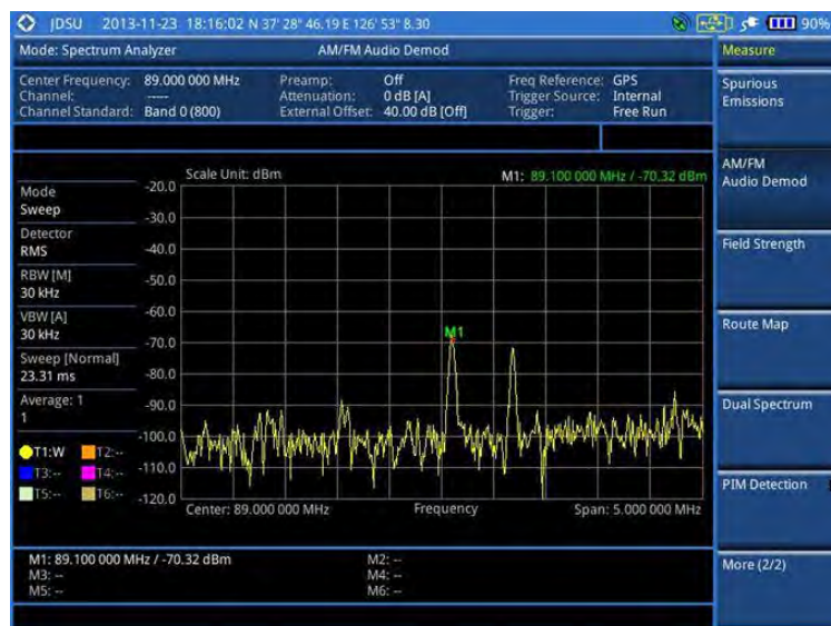
Figure 19 AM/FM audio demodulation with spectrum analyzer
