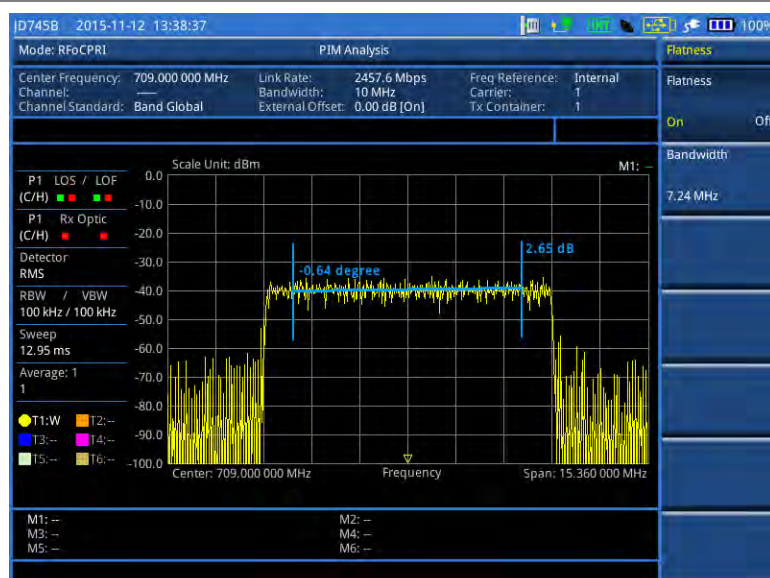
Figure 349 Example of PIM analysis in BBU emulation
