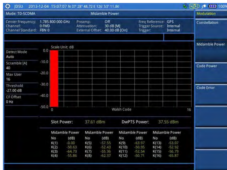
Figure 236 Midamble measurement with TD-SCDMA signal analyzer
