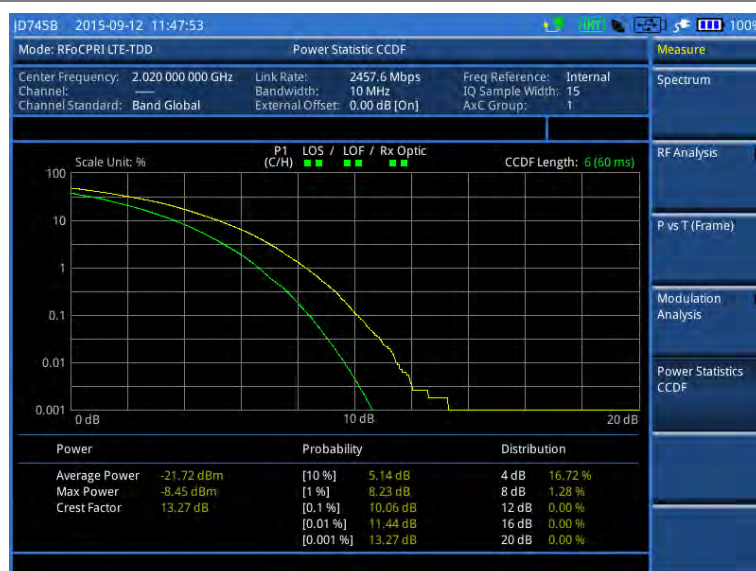
Figure 331 CCDF measurement with RFoCPRI LTE-TDD signal analyzer
