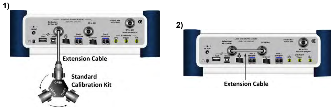
Figure 267 2-port calibration connection with Y-Cal in vector measurements
