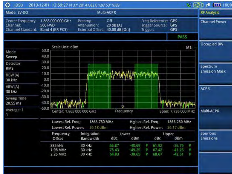
Figure 204 Multi-ACPR measurement with EV-DO signal analyzer
