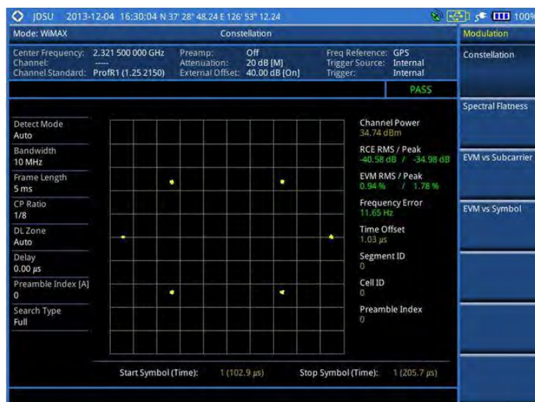
Figure 255 Constellation measurement with Mobile WiMAX signal analyzer
