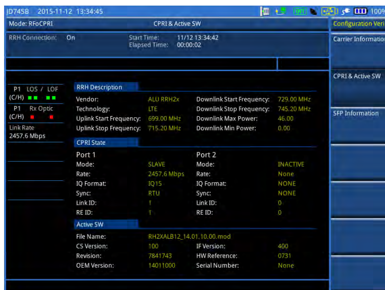
Figure 339 Example of verification of CPRI state and active software
