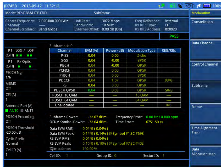
Figure 370 Subframe measurement with RFoBSAI LTE-FDD signal analyzer
