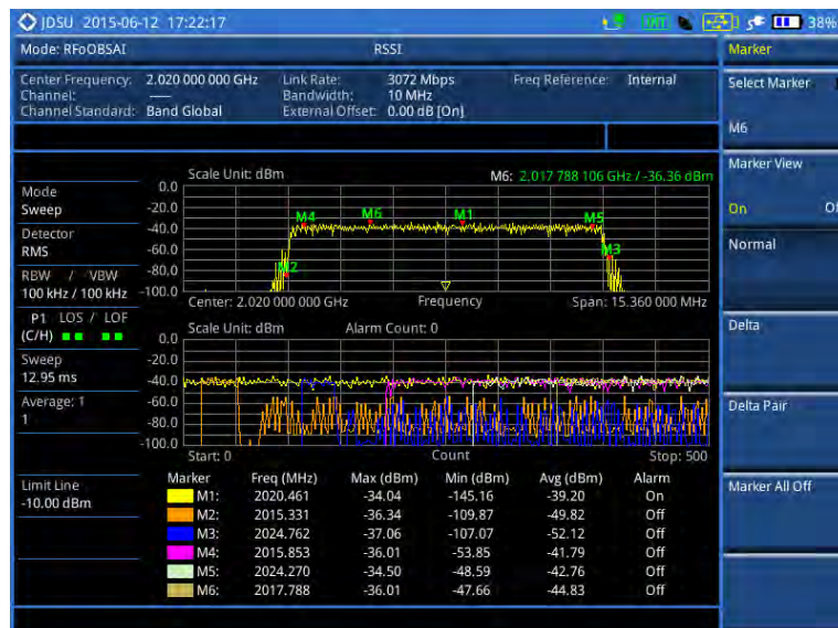
Figure 358 RFoBSAI interference measurement in RSSI
