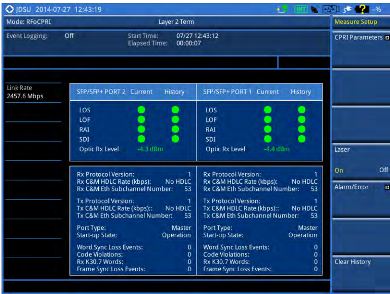
Figure 289 CPRI layer 2 term test
