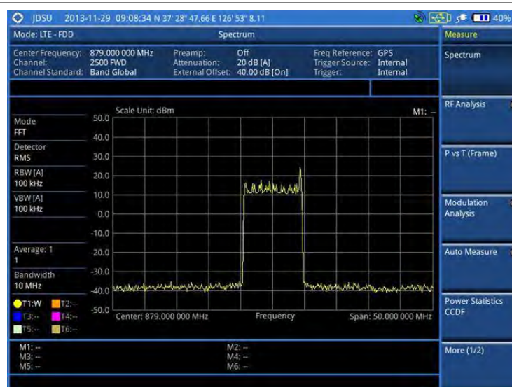
Figure 87 Spectrum measurement screen with LTE-FDD signal analyzer
