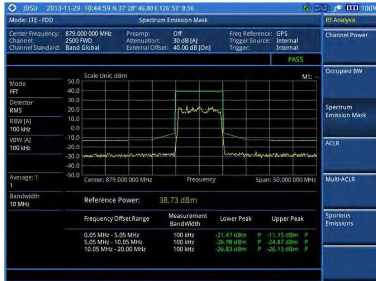
Figure 90 SEM measurement with LTE-FDD signal analyzer
