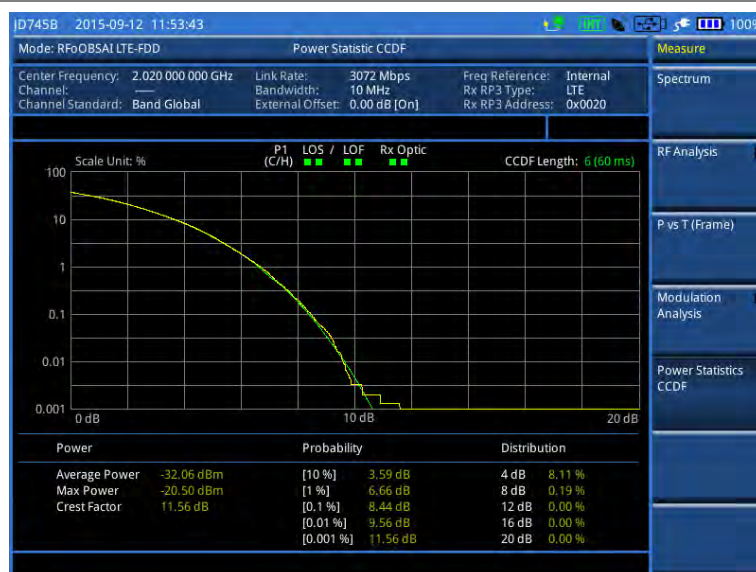
Figure 374 CCDF measurement with RFoBSAI LTE-FDD signal analyzer
