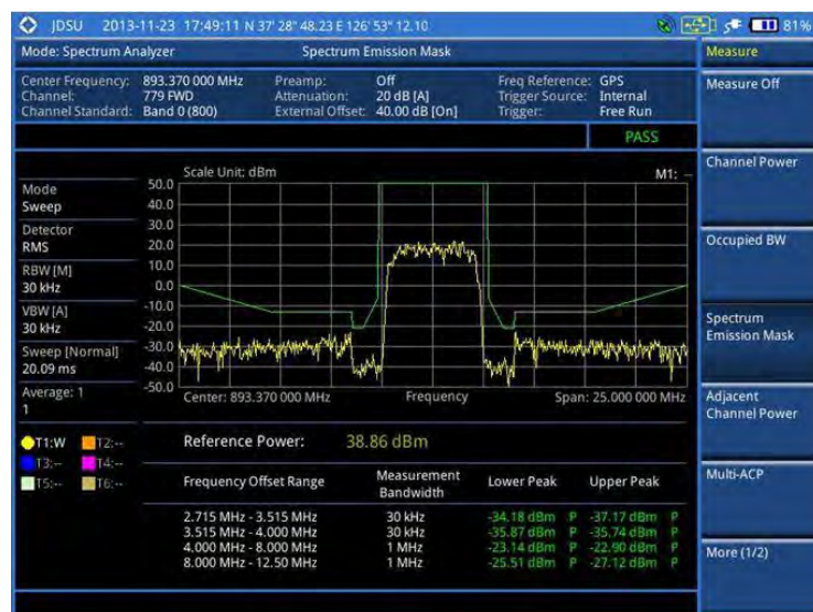
Figure 15 Spectrum emission mask measurement with spectrum analyzer
