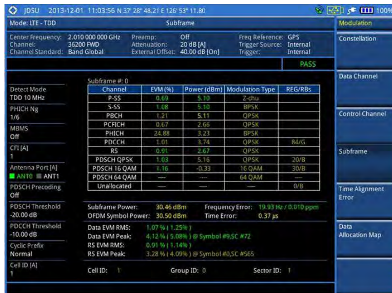
Figure 147 Subframe measurement with LTE-TDD signal analyzer
