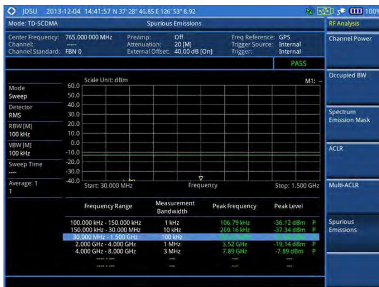
Figure 230 Spurious emissions measurement with TD-SCDMA signal analyzer
