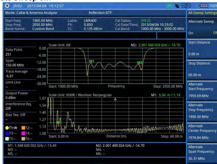
Figure 277 Reflection-DTF dual measurement
