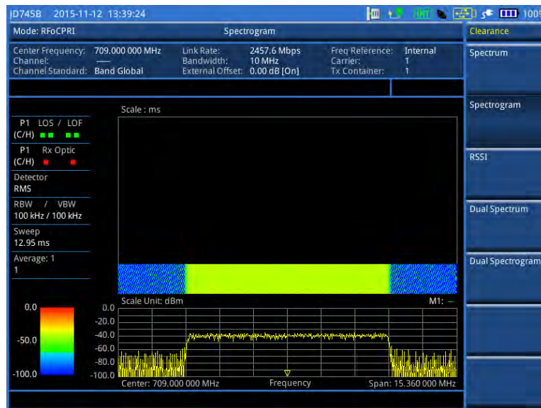
Figure 345 Example of spectrogram in BBU emulation
