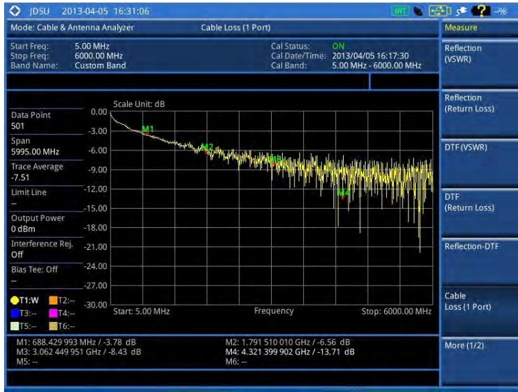
Figure 278 Cable loss (1 port) measurement
