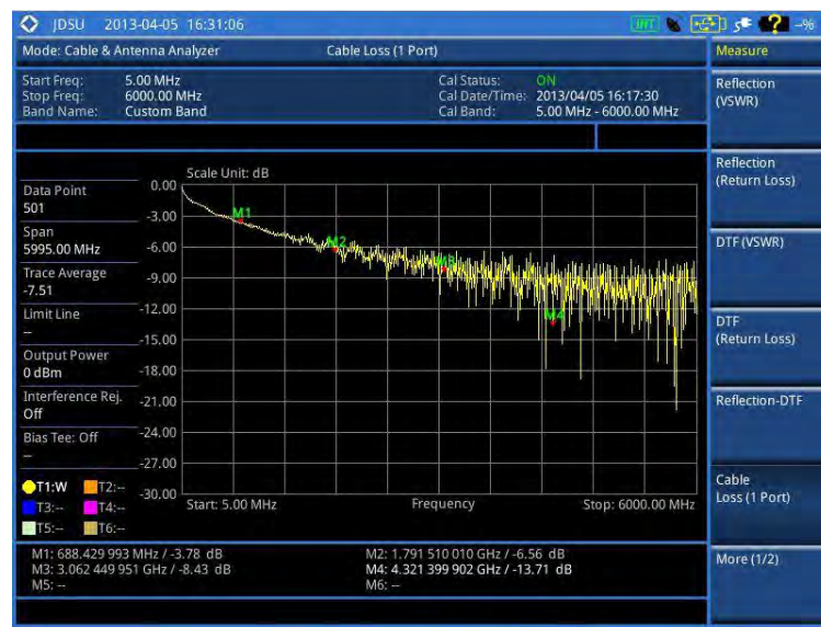
Figure 280 Cable loss (1 port) measurement
