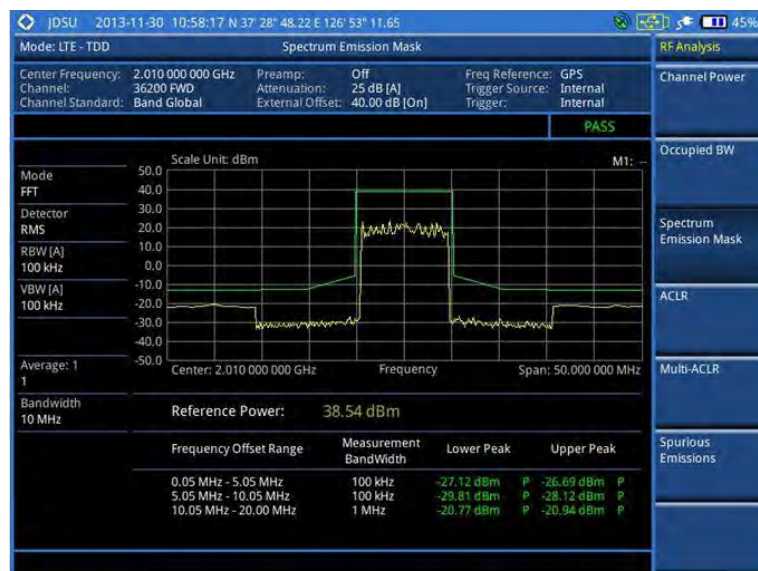
Figure 135 SEM measurement with LTE-TDD signal analyzer
