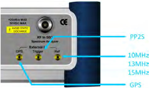
Figure 175 Connection ports for external reference clock
