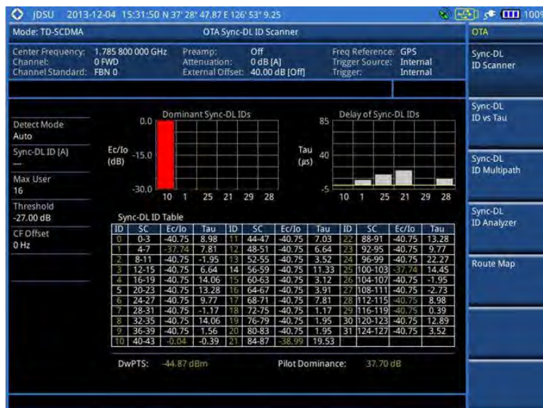
Figure 239 Sync-DL ID scanner measurement with TD-SCDMA OTA signal analyzer
