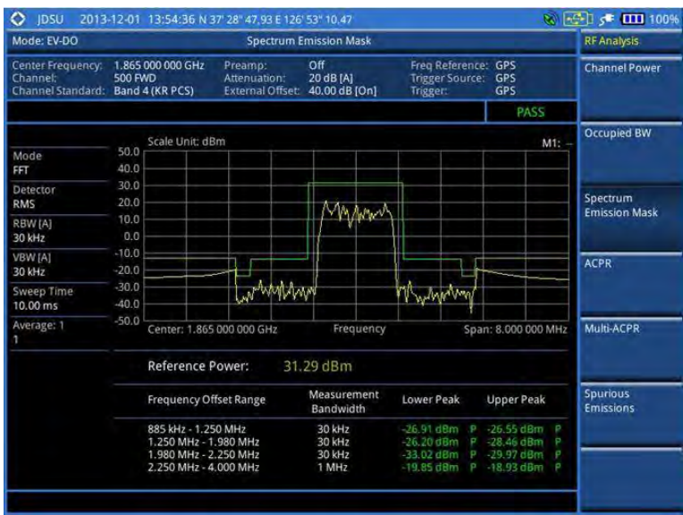
Figure 202 SEM measurement with EV-DO signal analyzer
