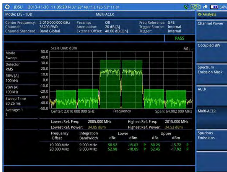
Figure 137 Multi-ACLR measurement with LTE-TDD signal analyzer
