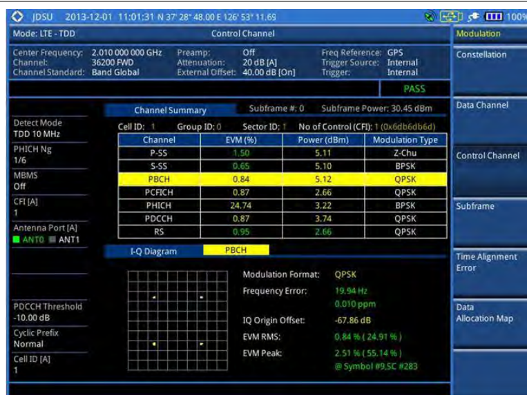
Figure 145 Control channel measurement with LTE-TDD signal analyzer
