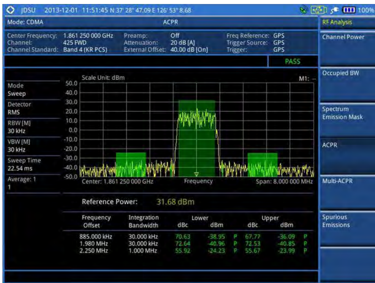
Figure 180 ACPR measurement with CDMA signal analyzer
