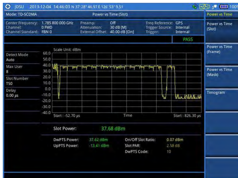
Figure 231 Power vs. time (slot) measurement with TD-SCDMA signal analyzer
