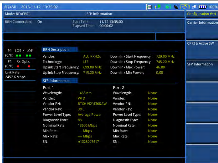
Figure 340 Example of verification of SFP information
