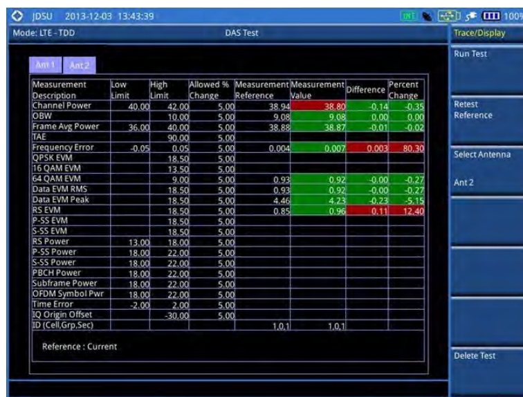
Figure 153 DAS measurement with LTE-TDD signal analyzer
