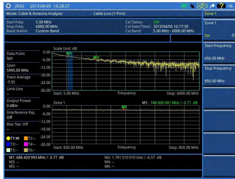
Figure 281 Cable loss (1 port) measurement with zoom
