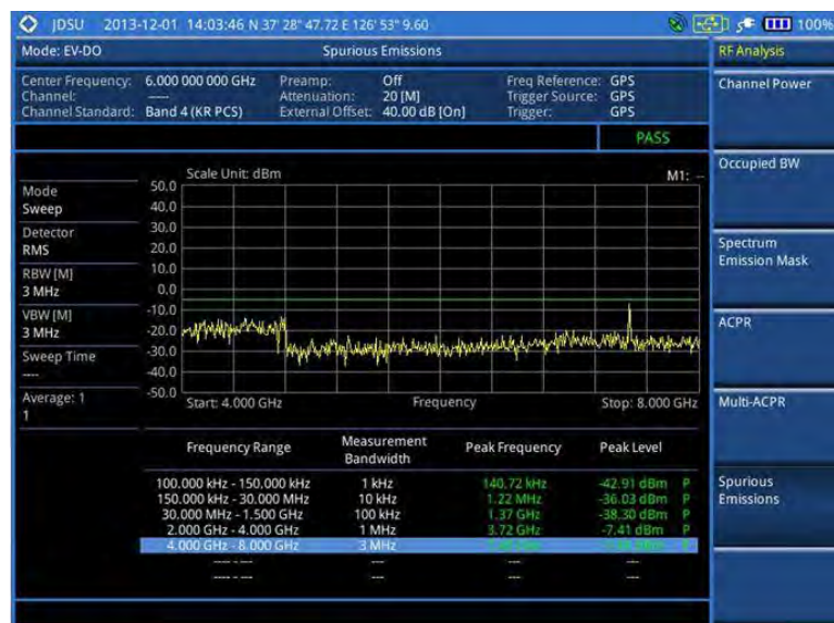
Figure 205 Spurious emissions measurement with EV-DO signal analyzer
