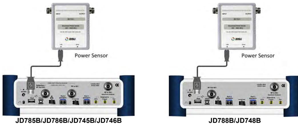
Figure 386 Directional power sensor connection
