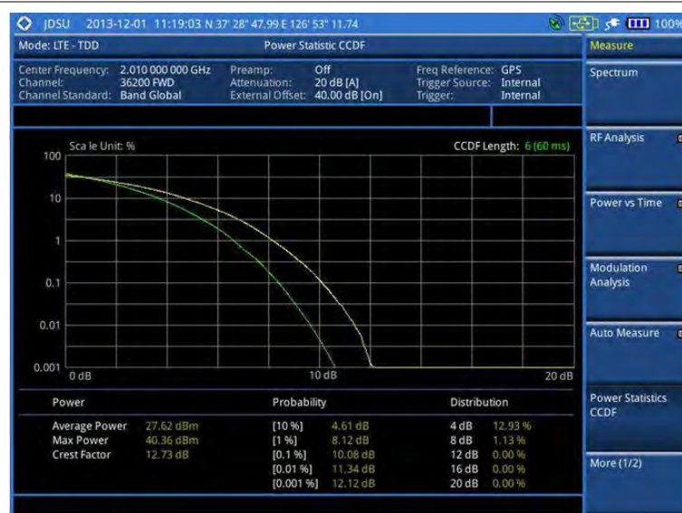
Figure 154 CCDF measurement with LTE-TDD signal analyzer
