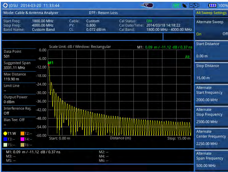
Figure 276 DTF measurement with the alternate sweep on
