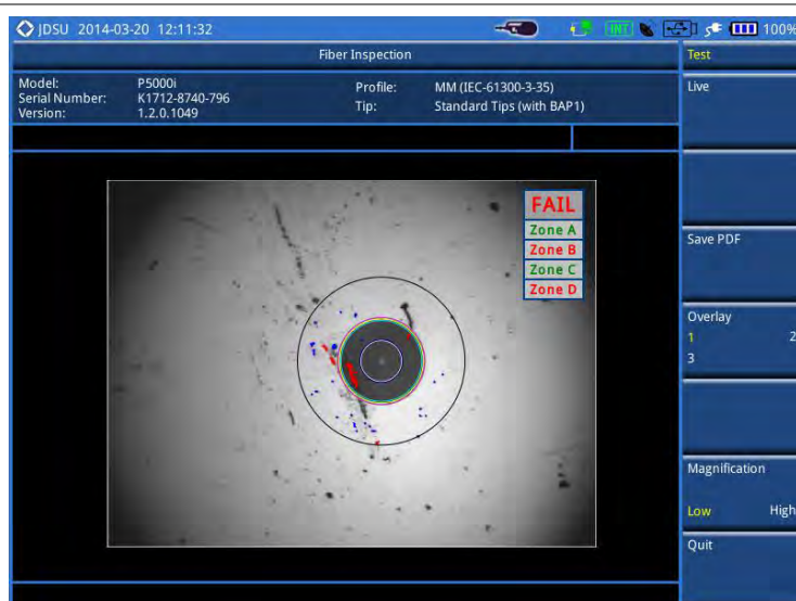
Figure 392 Analyzed fiber image and fiber inspection result
