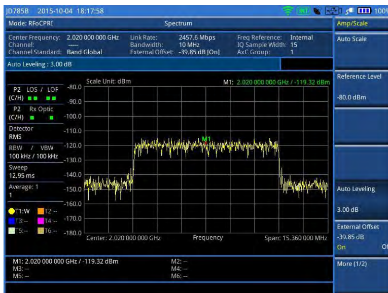
Figure 292 After enabling Auto Leveling
