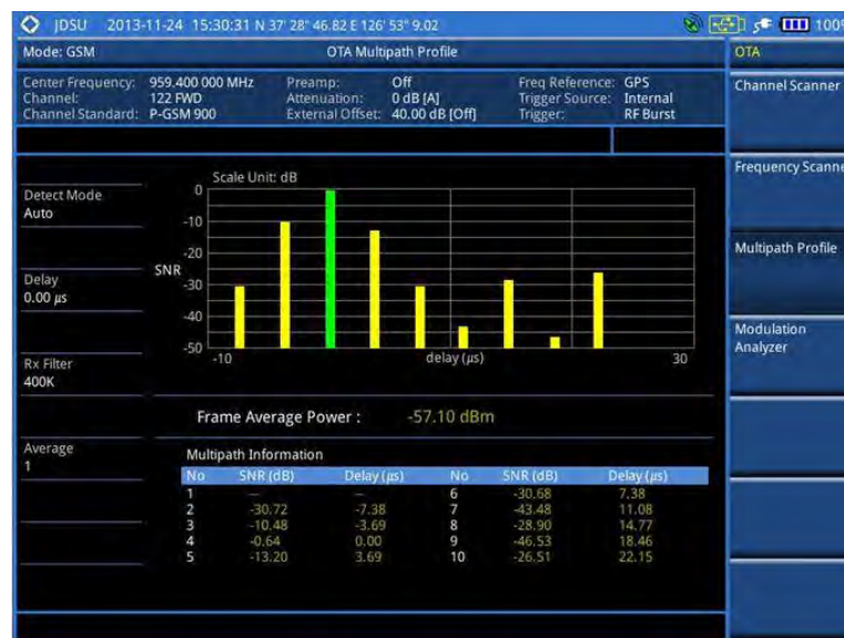
Figure 54 Multipath profile measurement with GSM OTA signal analyzer
