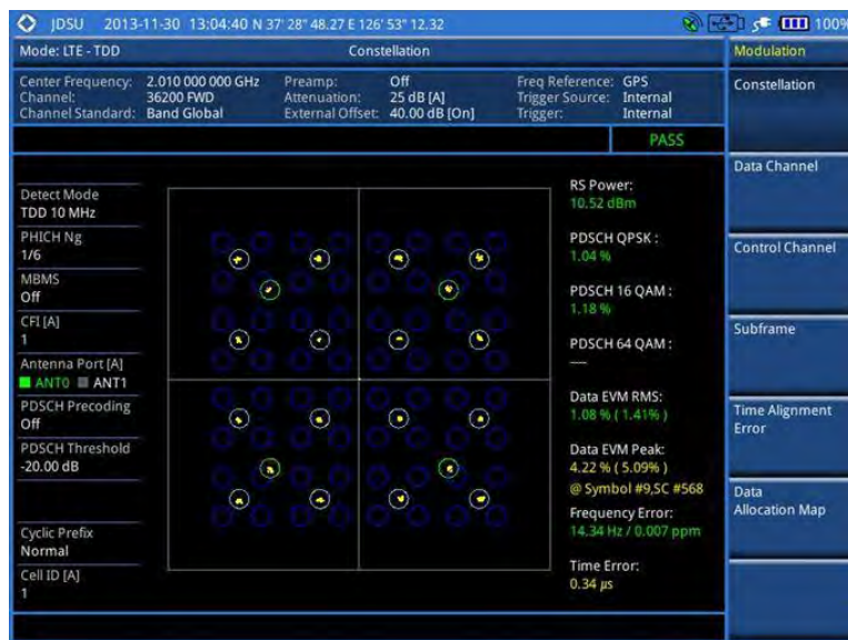
Figure 141 Constellation measurement with LTE-TDD signal analyzer
