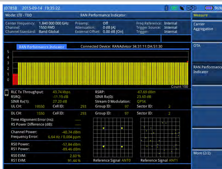
Figure 170 RAN performance indicator with LTE-TDD signal analyzer
