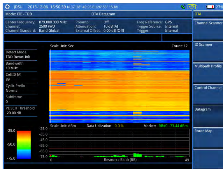
Figure 161 Datagram measurement with LTE-TDD signal analyzer
