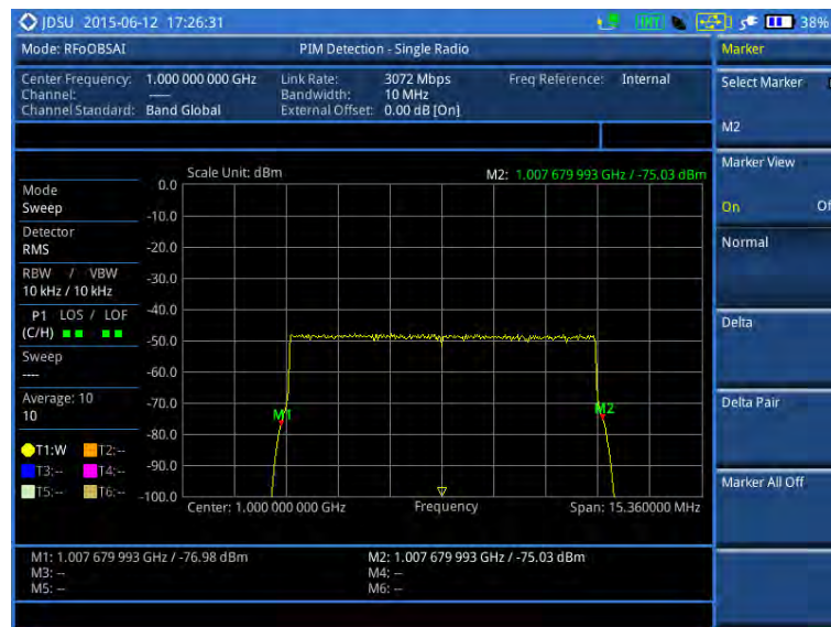
Figure 361 PIM detection of single radio
