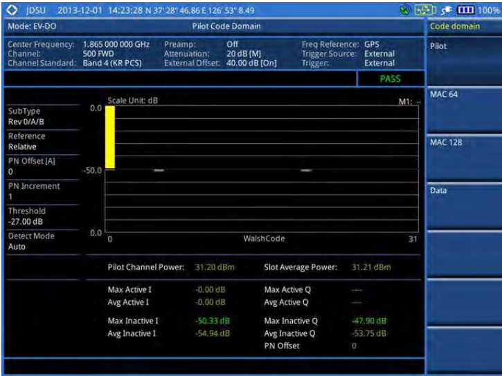
Figure 209 Code domain power measurement with EV-DO signal analyzer
