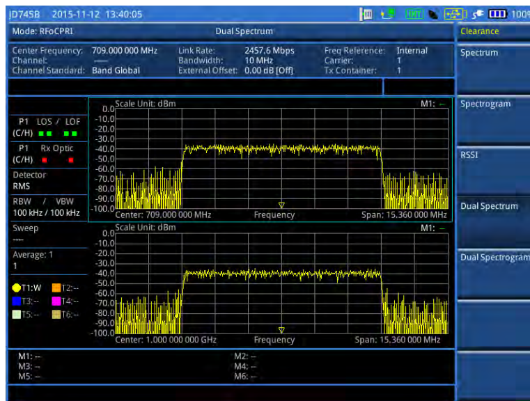
Figure 344 Example of dual spectrum analysis in BBU emulation
