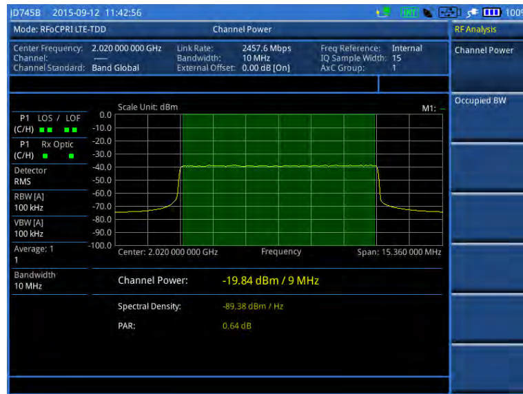
Figure 322 Channel power measurement with RFoCPRI LTE-TDD signal analyzer
