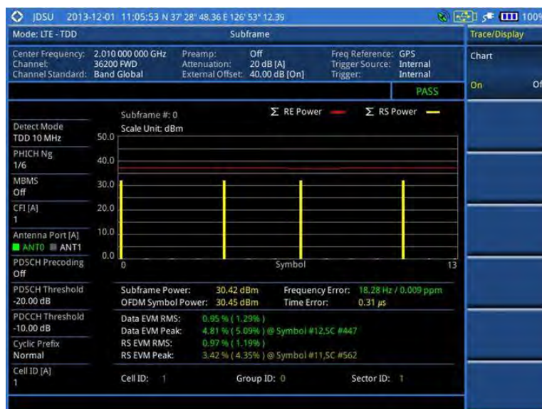
Figure 149 Subframe measurement with LTE-TDD signal analyzer (MBMS On)
