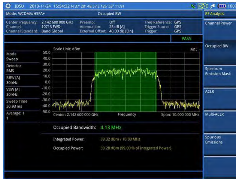
Figure 63 Occupied bandwidth measurement with WCDMA/HSPA+ signal analyzer
