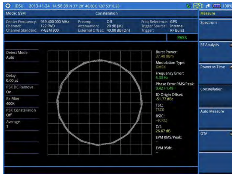
Figure 51 Constellation measurement (PSK on) with GSM signal analyzer
