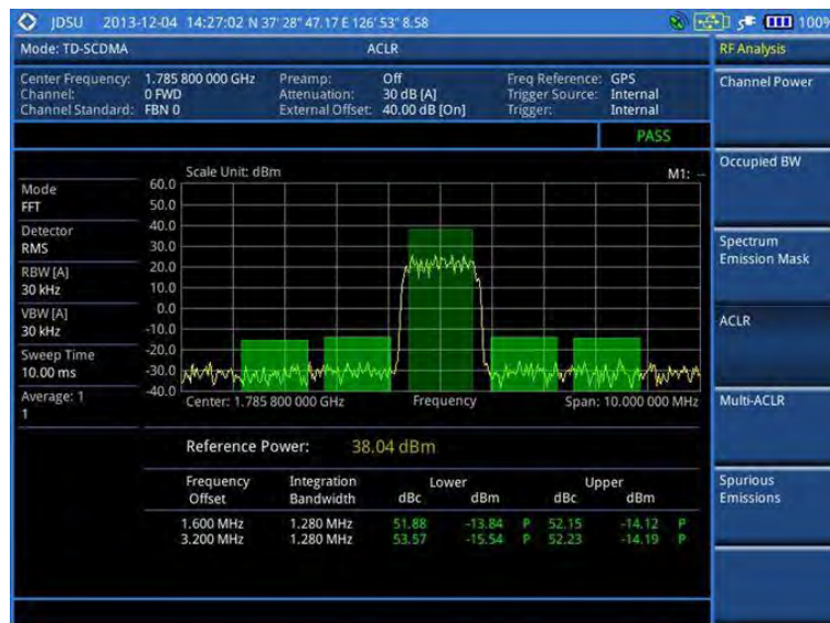
Figure 228 ACLR measurement with TD-SCDMA signal analyzer
