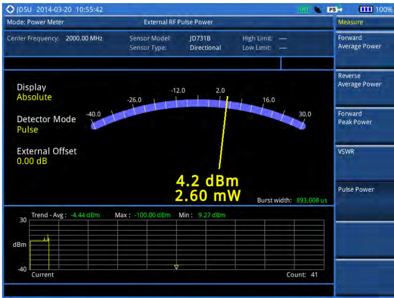
Figure 387 External power measurement of pulse power
