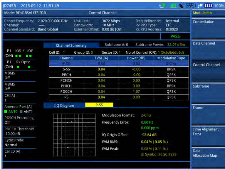
Figure 369 Control channel measurement with RFoBSAI LTE-FDD signal analyzer
