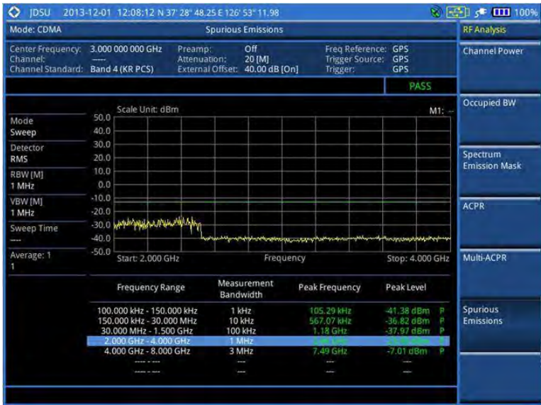
Figure 182 Spurious emissions measurement with CDMA signal analyzer
