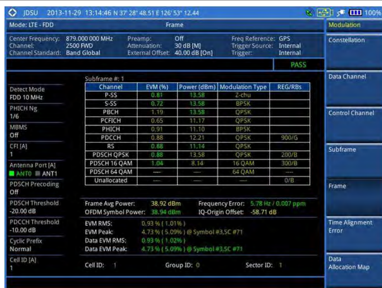
Figure 104 Frame measurement with LTE-FDD signal analyzer
