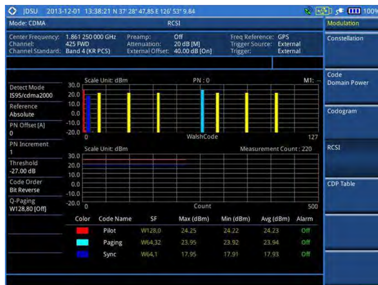
Figure 186 RCSI measurement with CDMA signal analyzer
