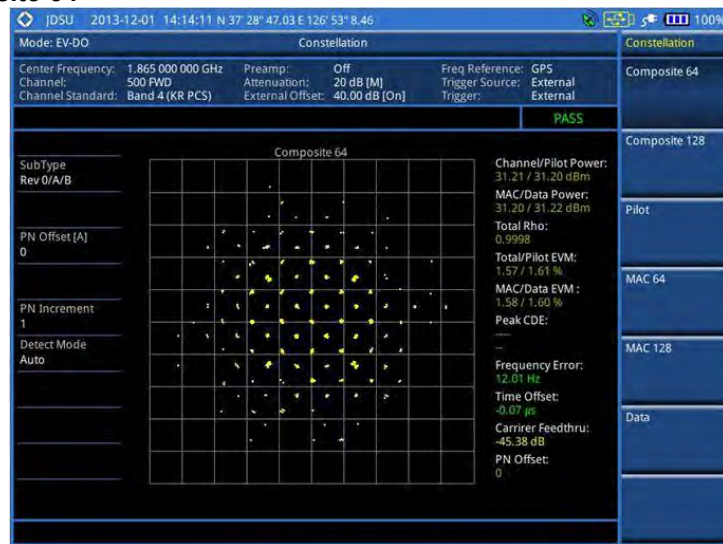
Figure 208 Constellation measurement with EV-DO signal analyzer
