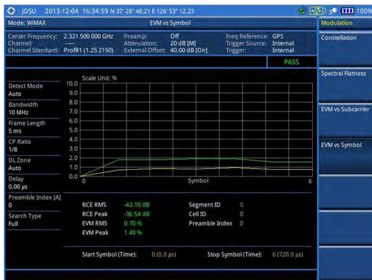
Figure 258 EVM vs. symbol measurement with Mobile WiMAX signal analyzer
