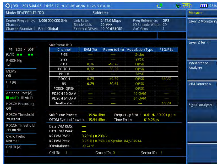
Figure 315 Subframe measurement (regular view) with RFoCPRI LTE-FDD signal analyzer
