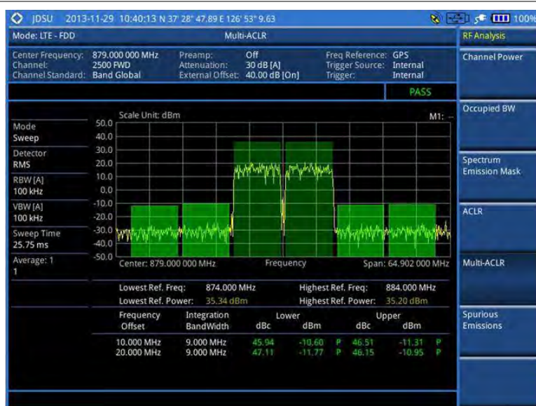
Figure 92 Multi-ACLR measurement with LTE-FDD signal analyzer
