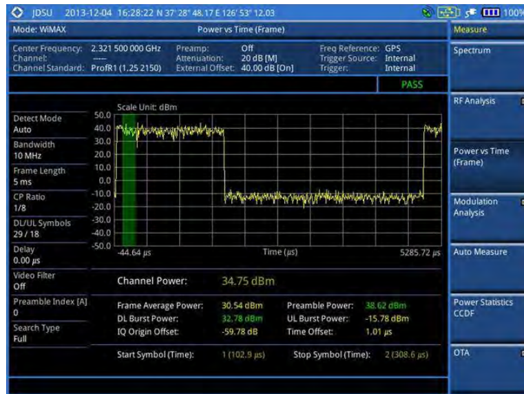
Figure 254 Power vs. time (frame) measurement with Mobile WiMAX signal analyzer
