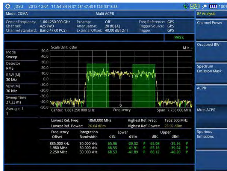
Figure 181 Multi-ACPR measurement with CDMA signal analyzer
