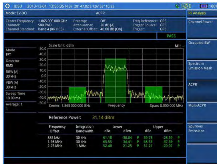
Figure 203 ACPR measurement with EV-DO signal analyzer
