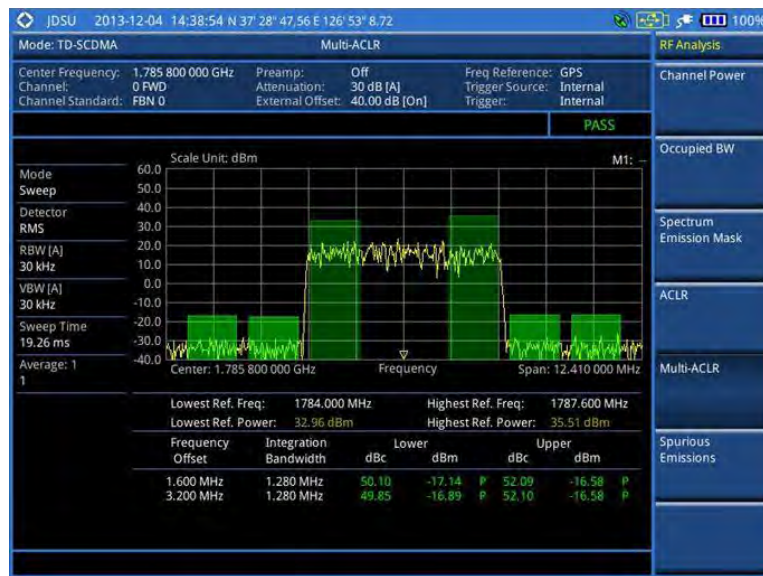
Figure 229 Multi-ACLR measurement with TD-SCDMA signal analyzer
