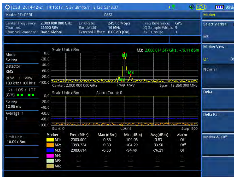
Figure 301 RFoCPRI interference measurement in RSSI
