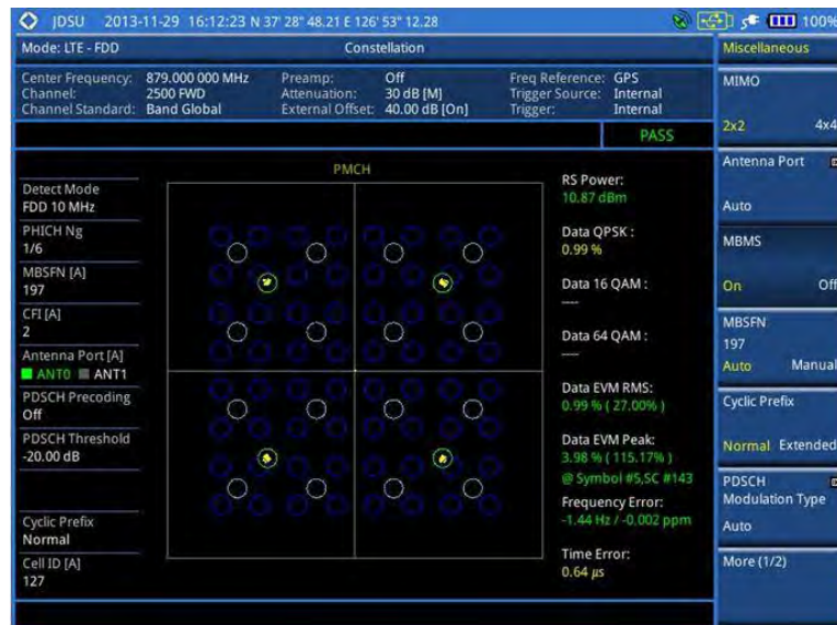
Figure 96 Constellation measurement with LTE-FDD signal analyzer (MBMS On)
