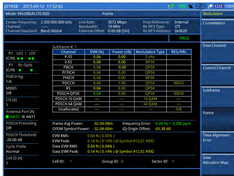
Figure 371 Frame measurement with RFoBSAI LTE-FDD signal analyzer
