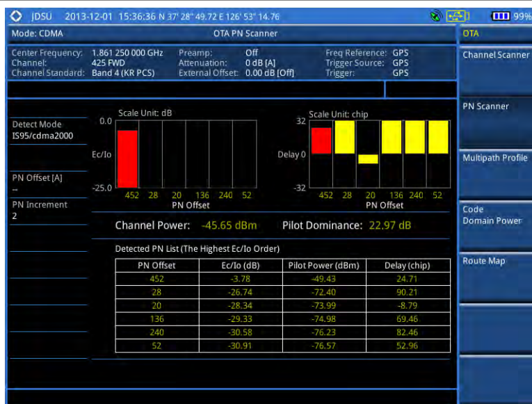
Figure 190 PN scanner measurement with CDMA OTA signal analyzer
