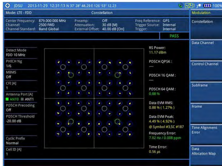
Figure 96 Constellation measurement with LTE-FDD signal analyzer (MBMS On)
