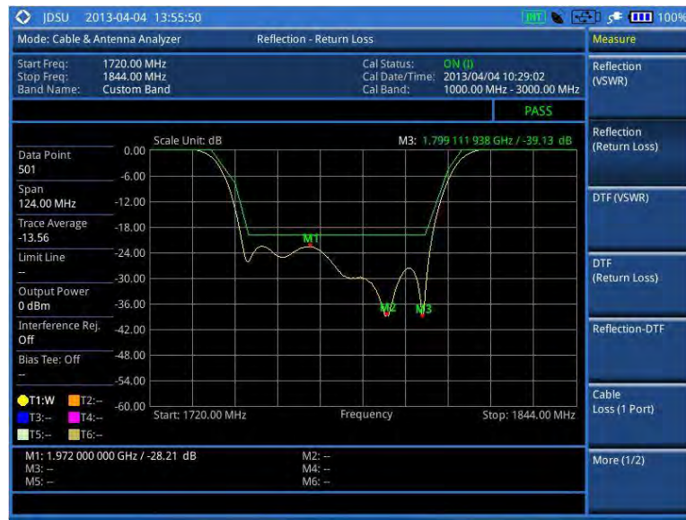
Figure 274 Reflection measurement in return loss scale
