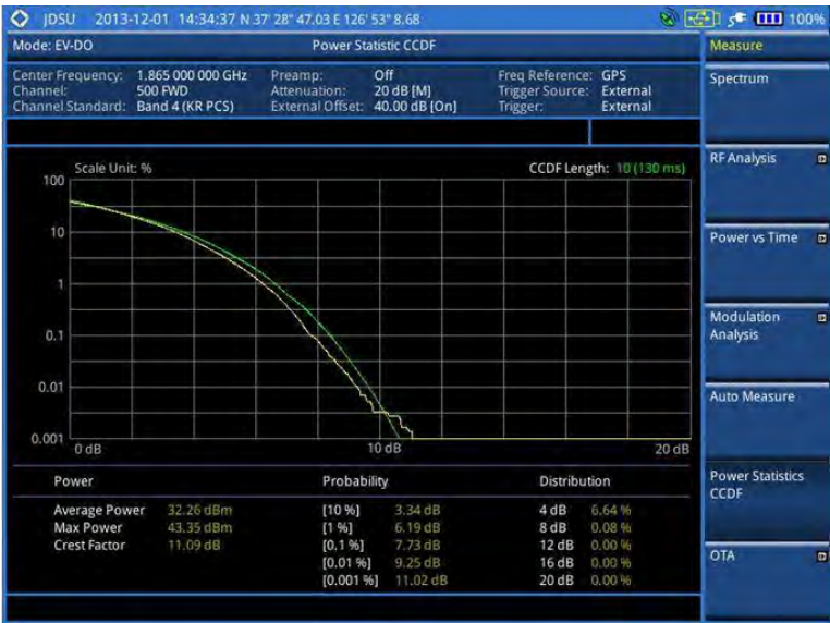
Figure 213 CCDF measurement with EV-DO signal analyzer
