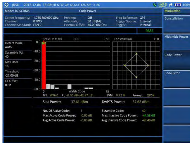
Figure 237 Code power measurement with TD-SCDMA signal analyzer
