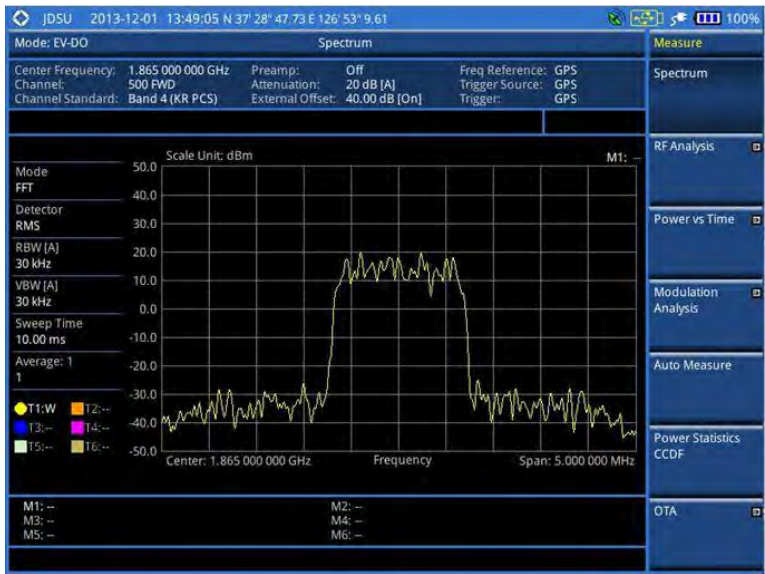
Figure 199 Spectrum measurement screen with EV-DO signal analyzer
