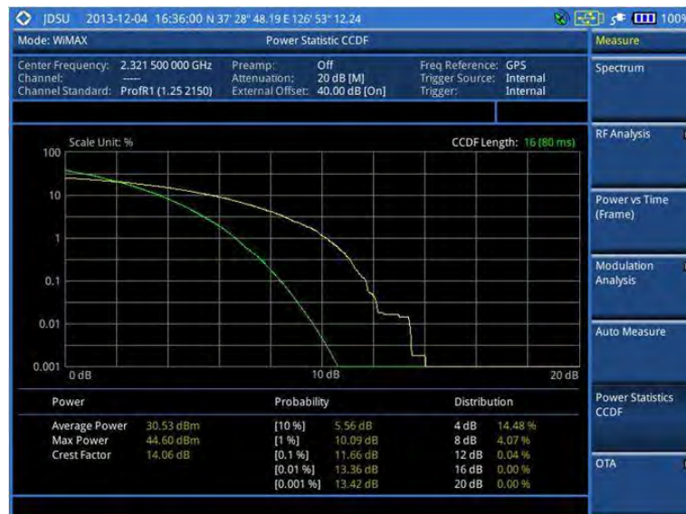
Figure 259 CCDF measurement with Mobile WiMAX signal analyzer
