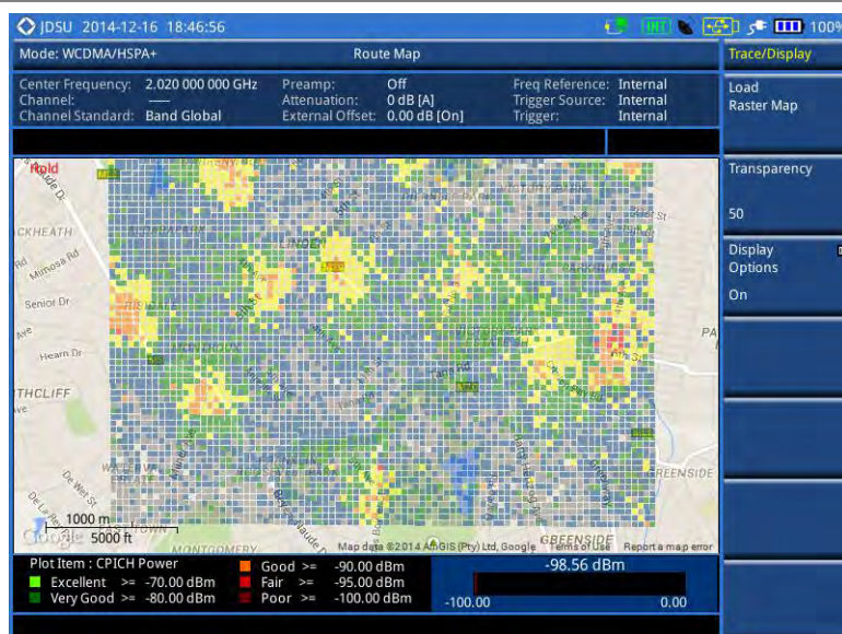
Figure 81 Raster image overlaid on the base map in WCDMA/HSPA+ OTA signal analyzer
