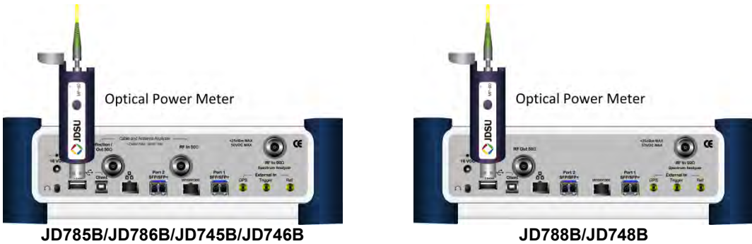
Figure 388 Optical power sensor connection
