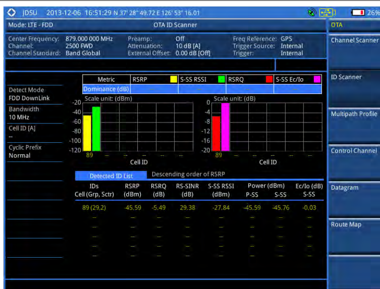
Figure 114 ID scanner measurement with LTE-FDD OTA signal analyzer
