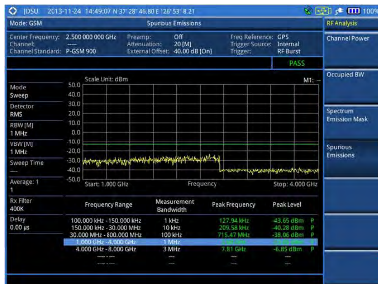
Figure 46 Spurious emissions measurement with GSM signal analyzer
