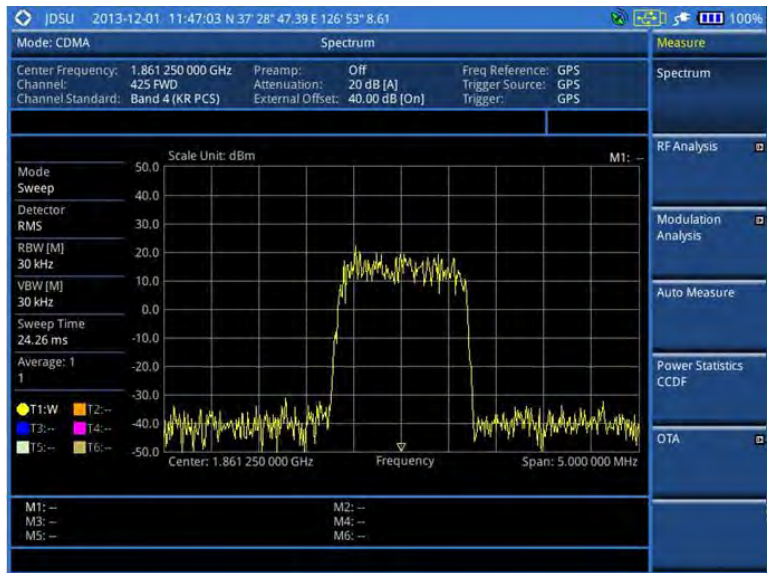
Figure 176 Spectrum measurement screen with CDMA signal analyzer
