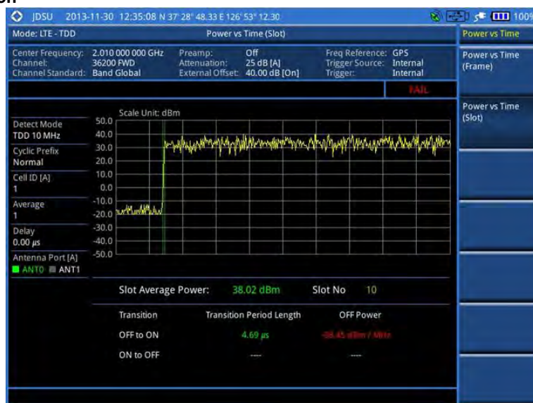
Figure 139 Power vs. time (slot) measurement with LTE – TDD signal analyzer
