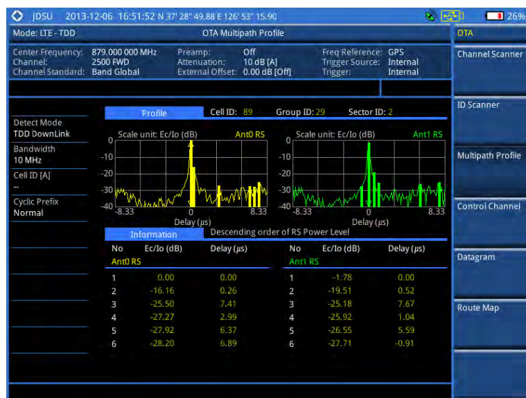
Figure 159 Multipath profile measurement with LTE-TDD OTA signal analyzer
