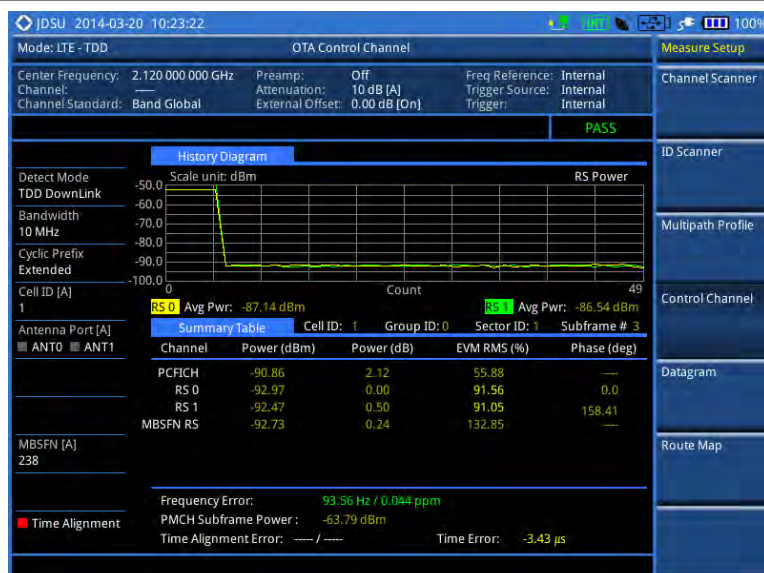
Figure 160 Control channel measurement with LTE-TDD OTA signal analyzer
