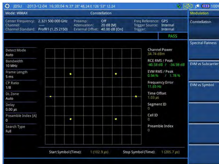
Figure 255 Constellation measurement with Mobile WiMAX signal analyzer
