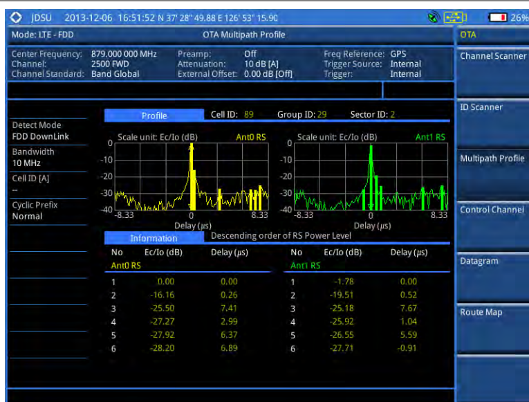
Figure 115 Multipath profile measurement with LTE-FDD OTA signal analyzer
