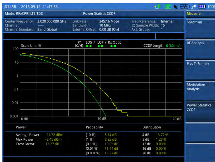
Figure 328 CCDF measurement with RFoCPRI LTE-TDD signal analyzer
