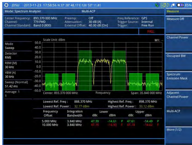
Figure 17 Multi-ACP measurement with spectrum analyzer
