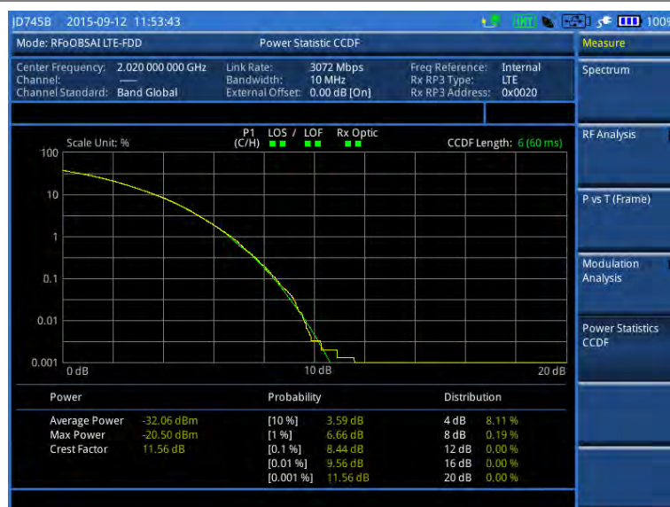
Figure 353 CCDF measurement with RFoBSAI LTE-FDD signal analyzer
