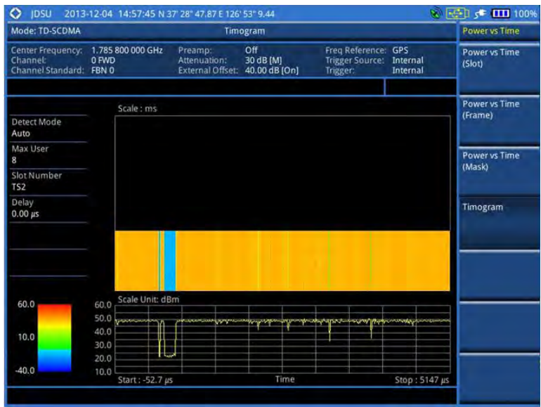
Figure 234 Timogram with TD-SCDMA signal analyzer
