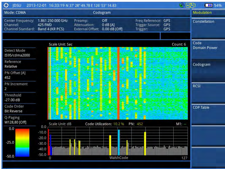
Figure 185 Codogram in full view with CDMA signal analyzer
