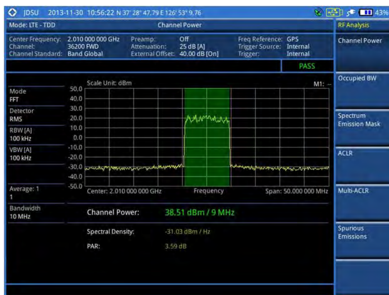
Figure 133 Channel power measurement with LTE-TDD signal analyzer
