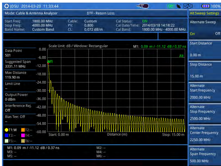
Figure 276 DTF measurement with the alternate sweep on
