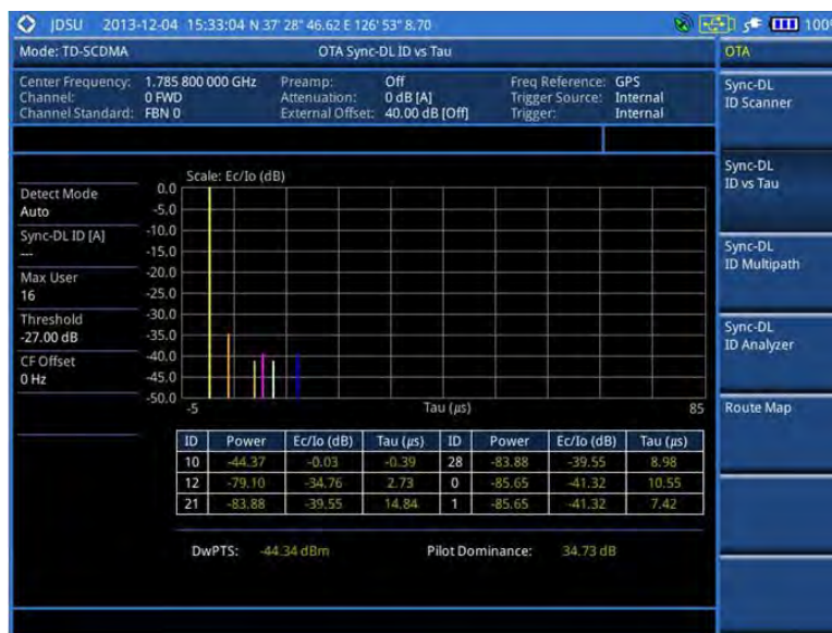
Figure 240 Sync-DL ID vs. Tau measurement with TD-SCDMA OTA signal analyzer
