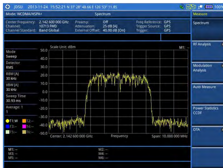
Figure 61 Spectrum measurement screen with WCDMA signal analyzer
