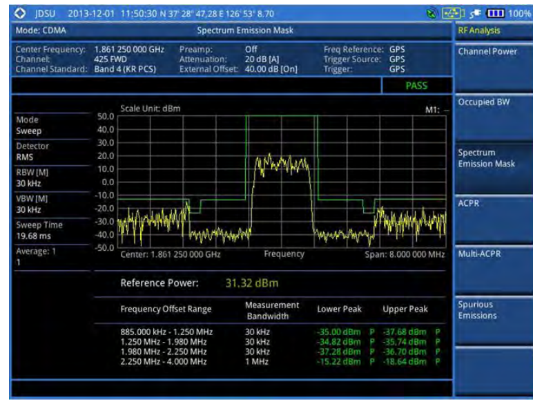
Figure 179 SEM measurement with CDMA signal analyzer
