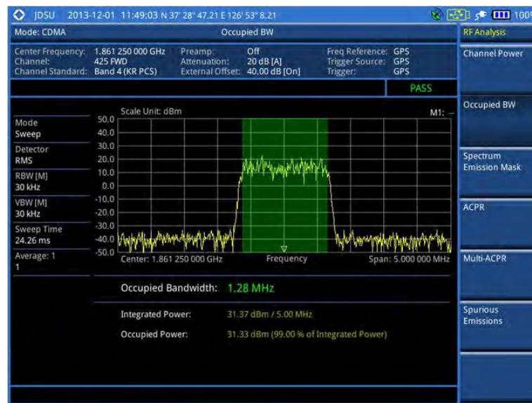
Figure 178 Occupied bandwidth measurement with CDMA signal analyzer
