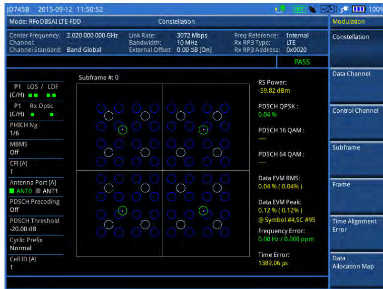
Figure 346 Constellation measurement with RFoBSAI LTE-FDD signal analyzer
