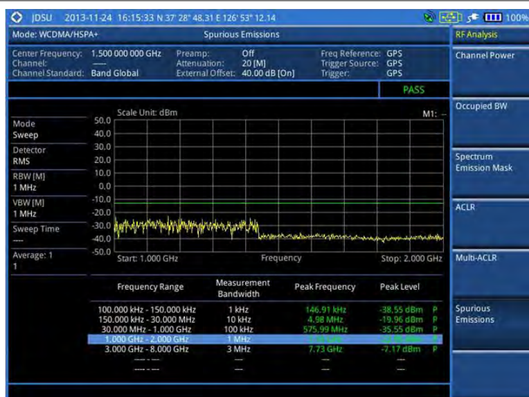
Figure 67 Spurious emissions measurement with WCDMA/HSPA+ signal analyzer
