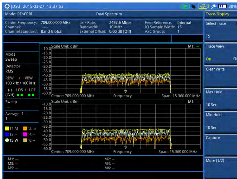
Figure 296 RFoCPRI dual spectrum analysis
