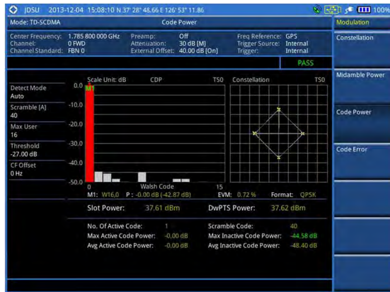
Figure 237 Code power measurement with TD-SCDMA signal analyzer
