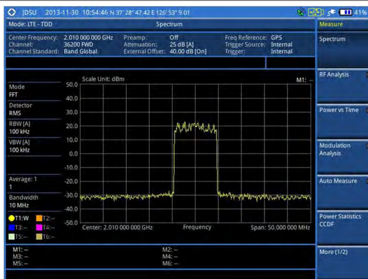
Figure 132 Spectrum measurement screen with LTE-TDD signal analyzer
