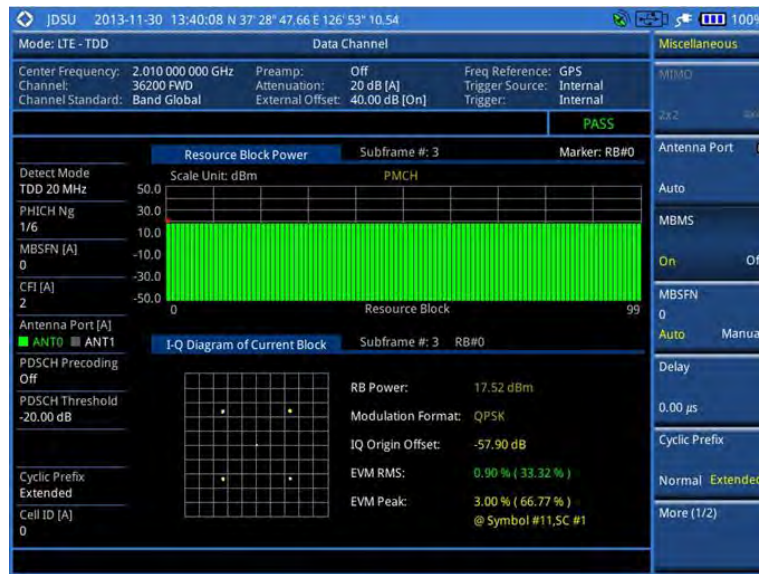
Figure 144 Data channel measurement with LTE-TDD signal analyzer (MBMS On)
