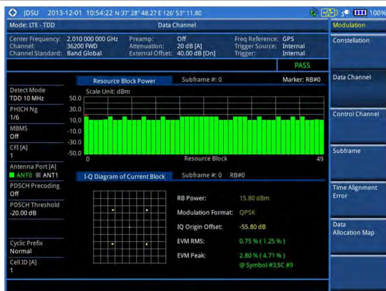
Figure 143 Data channel measurement with LTE-TDD signal analyzer
