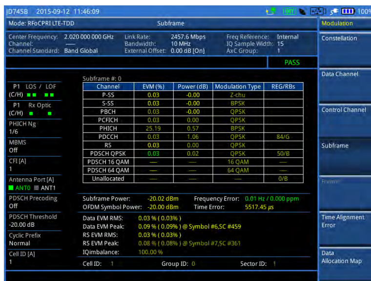
Figure 325 Subframe measurement (regular view) with RFoCPRI LTE-TDD signal analyzer
