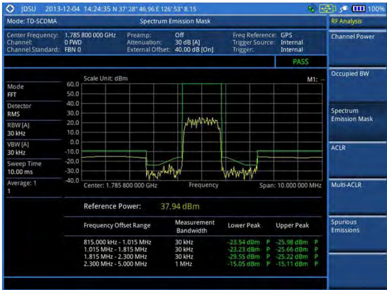
Figure 227 SEM measurement with TD-SCDMA signal analyzer
