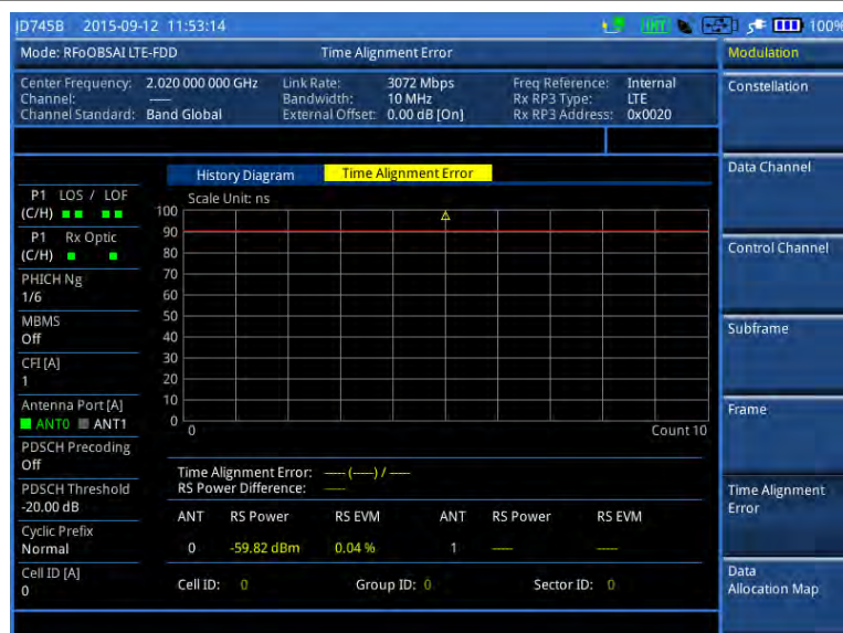
Figure 351 Time alignment error measurement with RFoBSAI LTE-FDD signal analyzer
