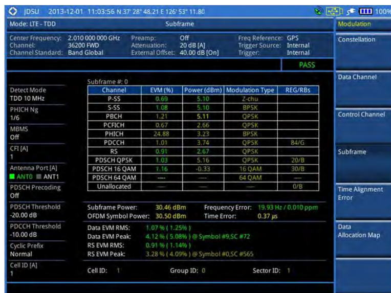
Figure 147 Subframe measurement with LTE-TDD signal analyzer
