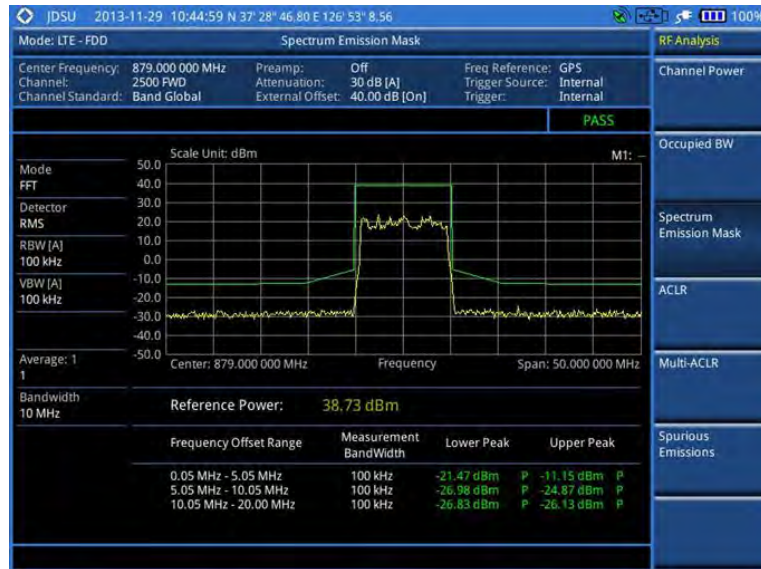
Figure 90 SEM measurement with LTE-FDD signal analyzer
