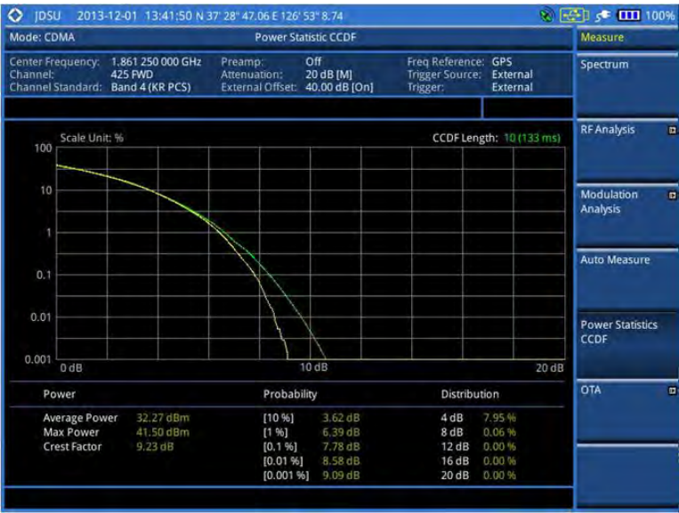
Figure 188 CCDF measurement with CDMA signal analyzer
