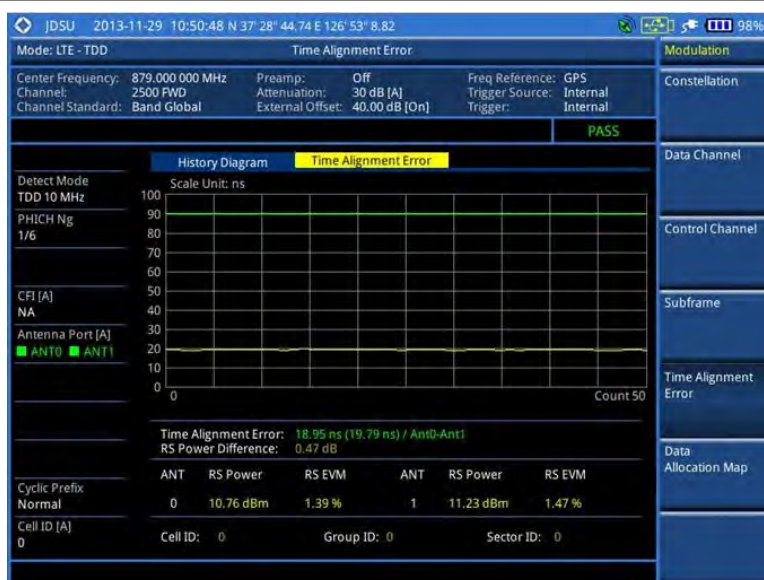
Figure 150 Time alignment error measurement with LTE-TDD signal analyzer
