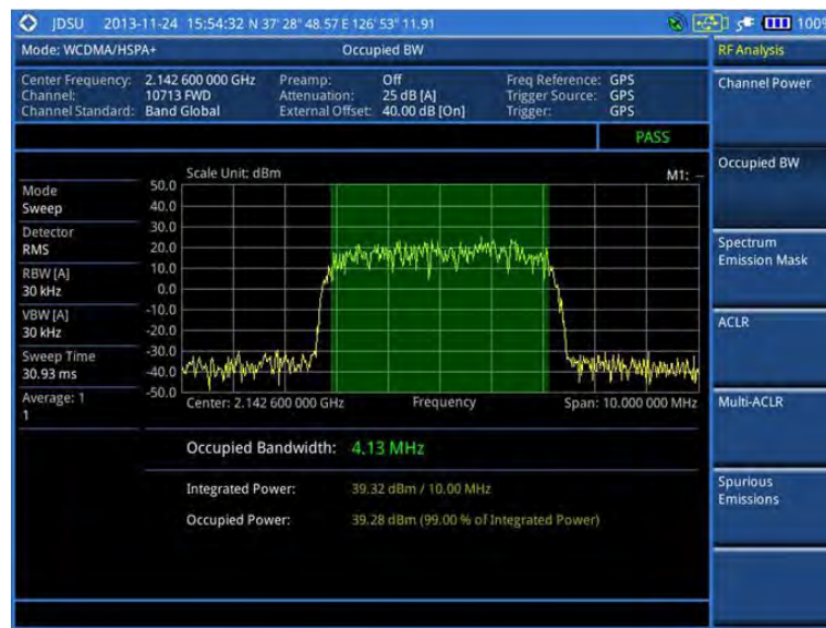
Figure 63 Occupied bandwidth measurement with WCDMA/HSPA+ signal analyzer
