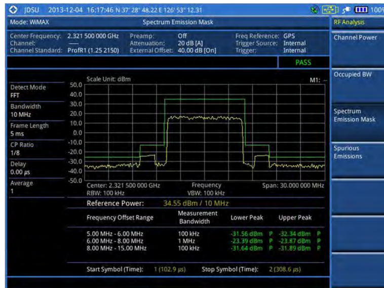
Figure 252 SEM measurement with Mobile WiMAX signal analyzer
