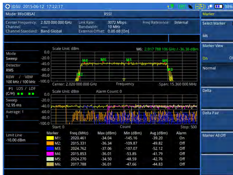
Figure 337 RFoOBSAI interference measurement in RSSI
