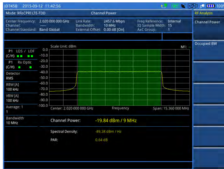
Figure 319 Channel power measurement with RFoCPRI LTE-TDD signal analyzer
