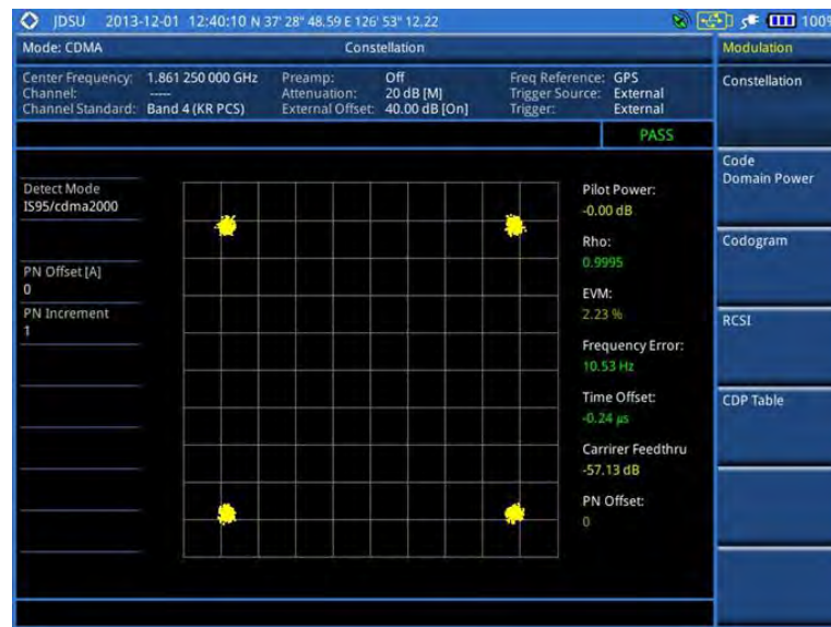
Figure 183 Constellation measurement with CDMA signal analyzer
