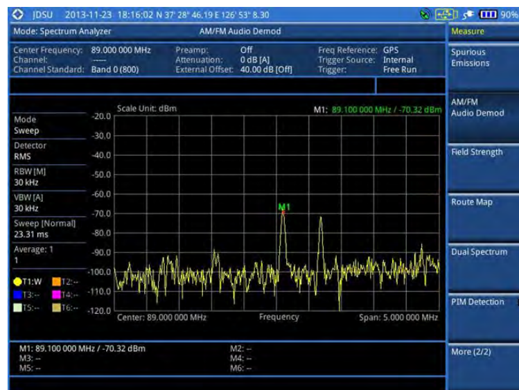
Figure 19 AM/FM audio demodulation with spectrum analyzer
