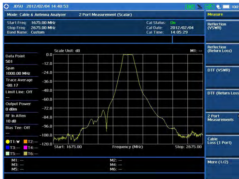
Figure 284 2-port scalar measurement
