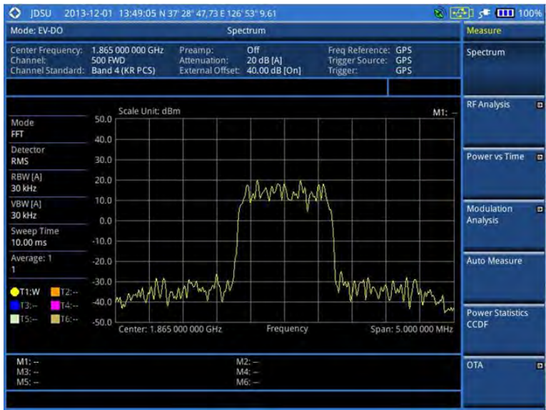
Figure 199 Spectrum measurement screen with EV-DO signal analyzer
