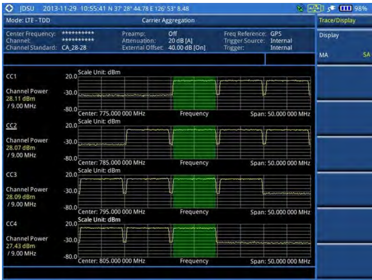
Figure 156 Carrier aggregation measurement with LTE-TDD signal analyzer (SA)
