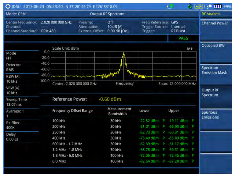
Figure 45 Output RF spectrum measurement with GSM signal analyzer
