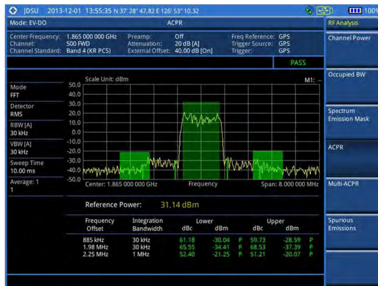
Figure 203 ACPR measurement with EV-DO signal analyzer
