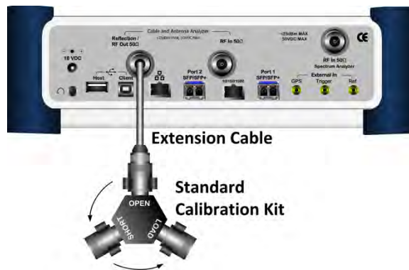
Figure 265 1-port calibration connection with mechanical Y-Cal kit
