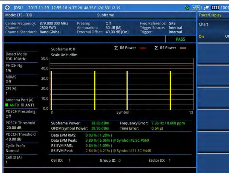
Figure 103 Subframe measurement with LTE-FDD signal analyzer (MBMS On)
