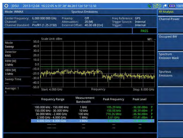
Figure 253 Spurious emissions measurement with Mobile WiMAX signal analyzer
