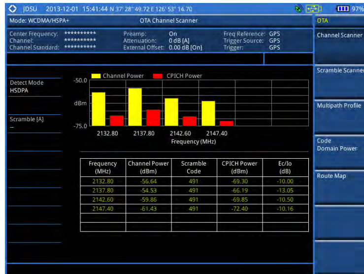
Figure 75 Channel scanner measurement with WCDMA/HSPA+ OTA signal analyzer
