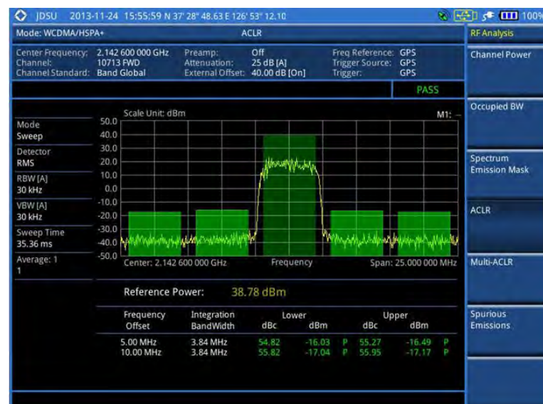
Figure 65 ACLR measurement with WCDMA/HSPA+ signal analyzer
