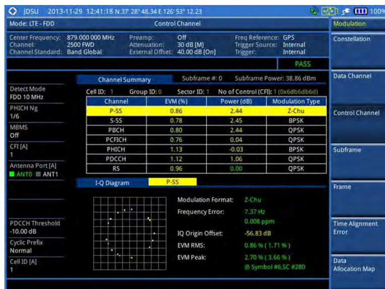
Figure 100 Control channel measurement with LTE-FDD signal analyzer (MBMS On)
