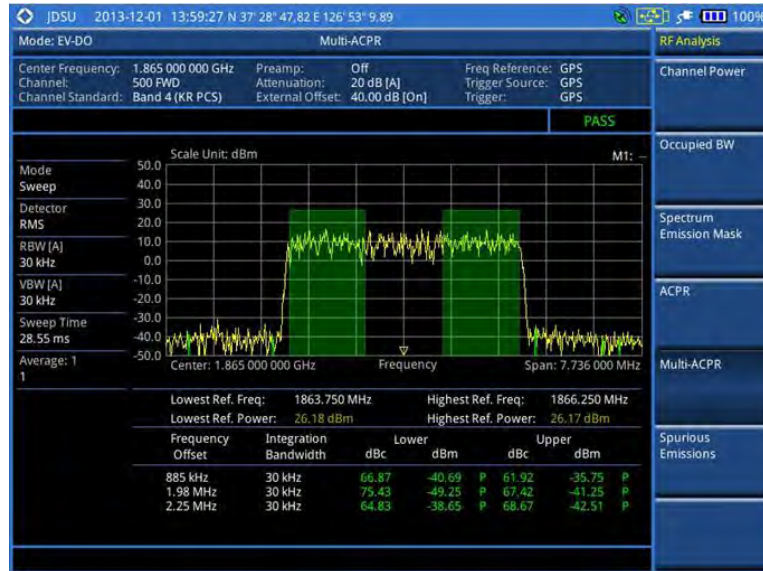
Figure 204 Multi-ACPR measurement with EV-DO signal analyzer
