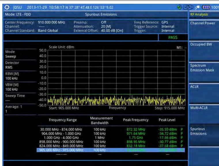
Figure 93 Spurious emissions measurement with LTE-FDD signal analyzer
