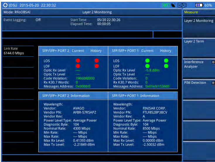
Figure 331 OBSAI RP3 layer 2 monitoring
