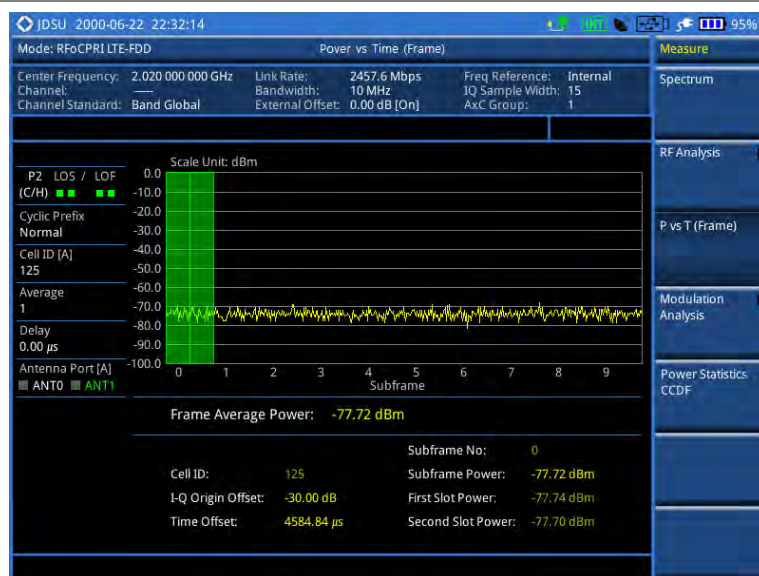
Figure 308 Power vs. time (frame) measurement with RFoCPRI LTE-FDD signal analyzer
