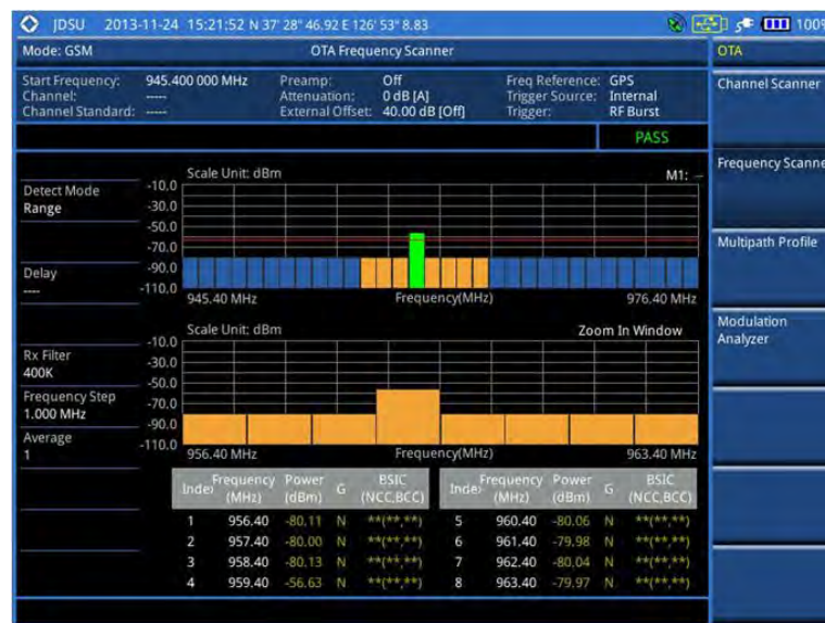
Figure 53 Frequency scanner measurement with GSM OTA signal analyzer
