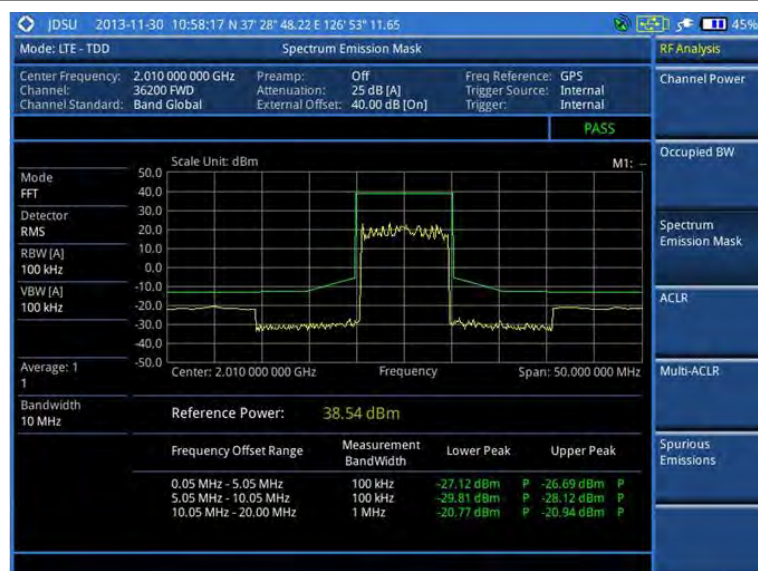
Figure 135 SEM measurement with LTE-TDD signal analyzer
