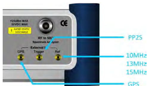
Figure 175 Connection ports for external reference clock
