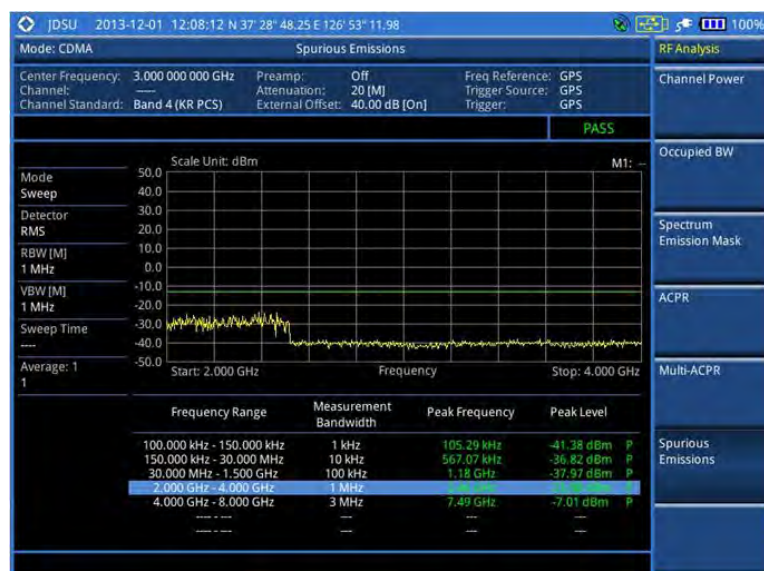
Figure 182 Spurious emissions measurement with CDMA signal analyzer
