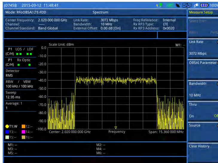
Figure 342 Spectrum measurement with RFoBSAI LTE-FDD signal analyzer
