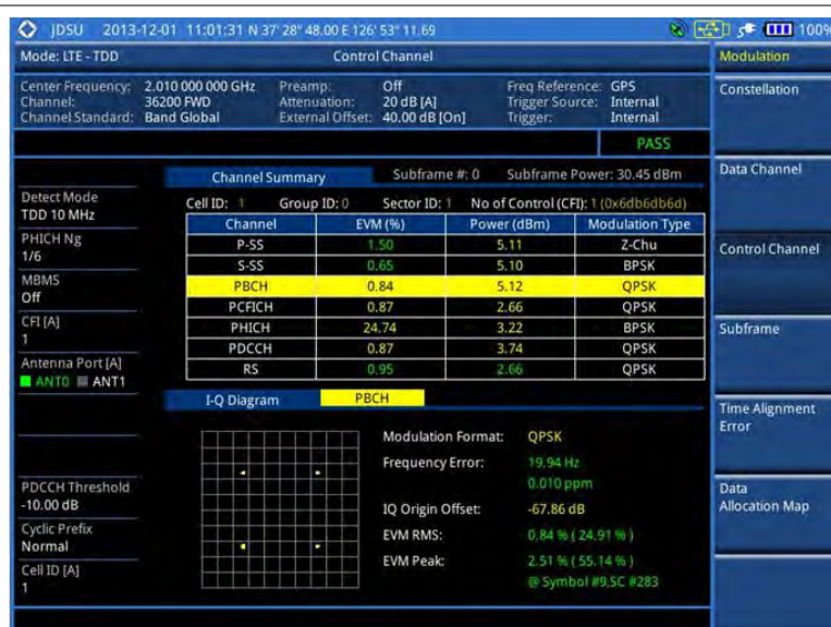
Figure 145 Control channel measurement with LTE-TDD signal analyzer
