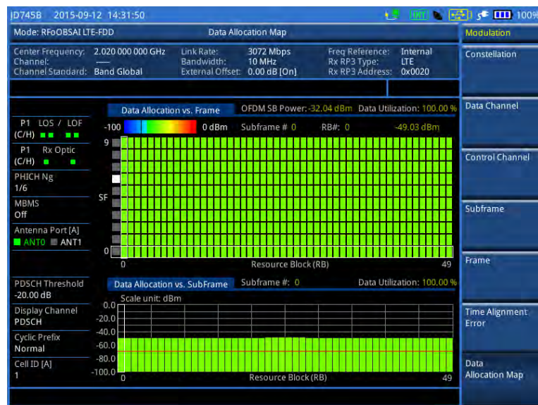
Figure 352 Data allocation map measurement with RFoBSAI LTE-FDD signal analyzer
