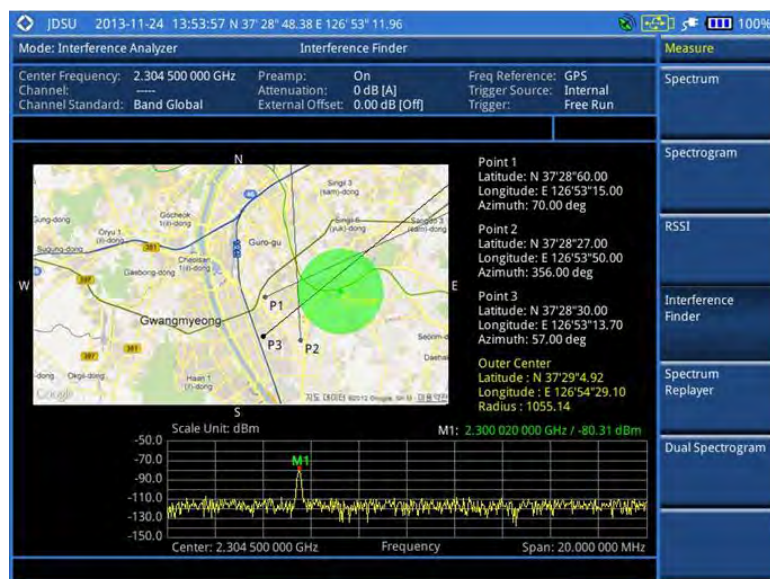
Figure 33 Interference finder measurement in map view
