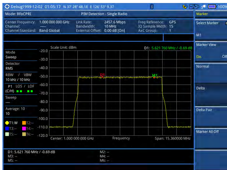
Figure 302 PIM detection of single radio
