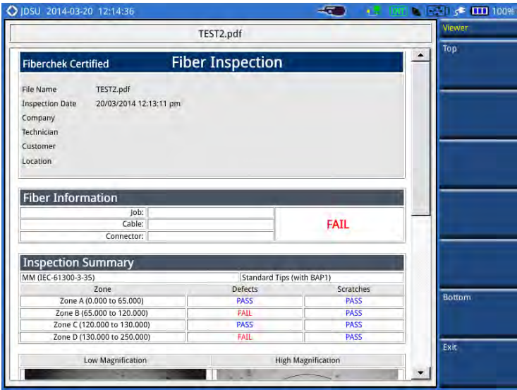
Figure 372 Fiber inspection report
