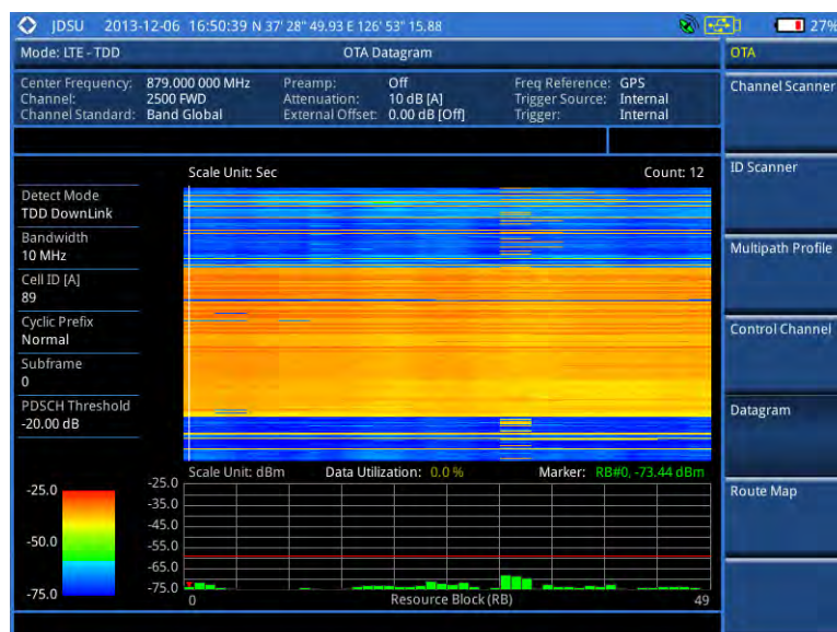
Figure 161 Datagram measurement with LTE-TDD signal analyzer
