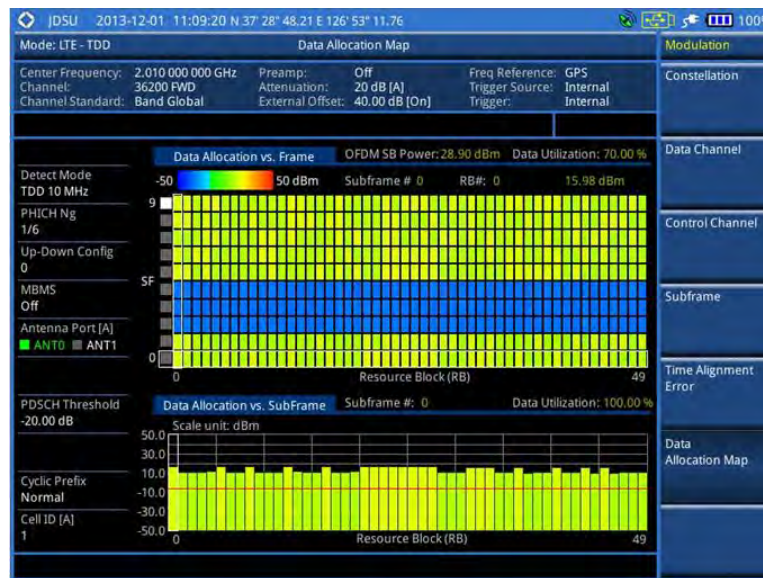
Figure 152 Data allocation map measurement with LTE-TDD signal analyzer (MBMS On)
