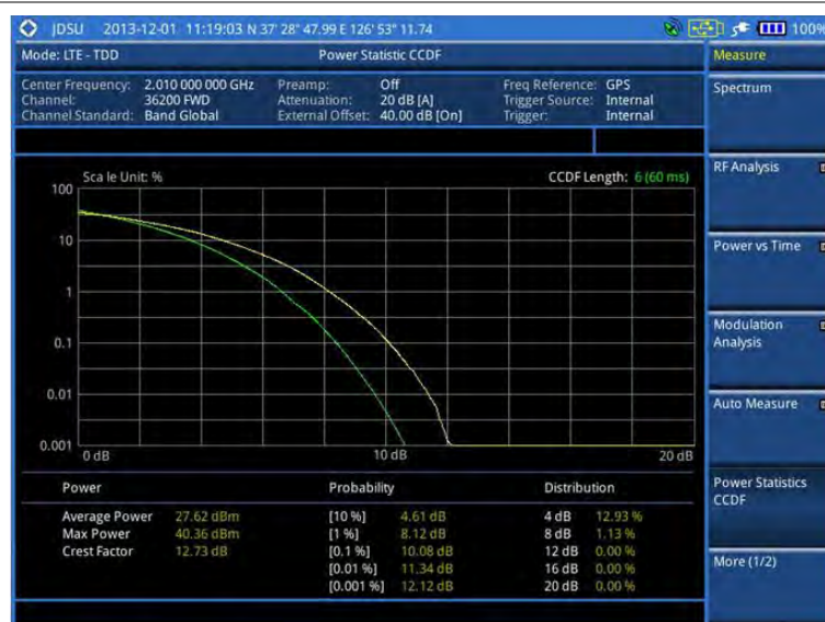
Figure 154 CCDF measurement with LTE-TDD signal analyzer
