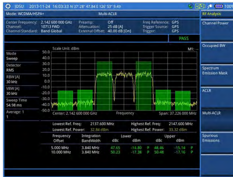
Figure 66 Multi-ACLR measurement with WCDMA/HSPA+ signal analyzer
