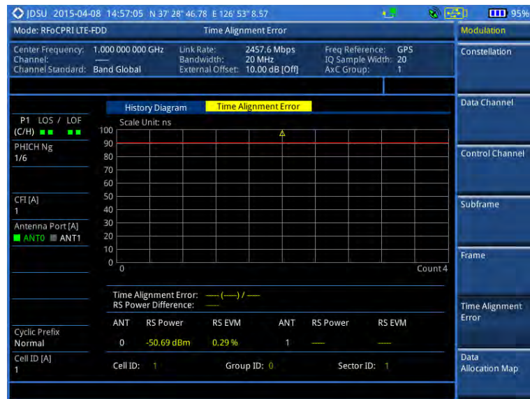
Figure 314 Time alignment error measurement with RFoCPRI LTE-FDD signal analyzer
