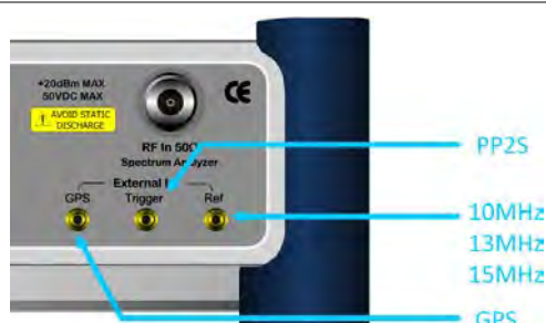
Figure 60 Connection ports for external reference clock
