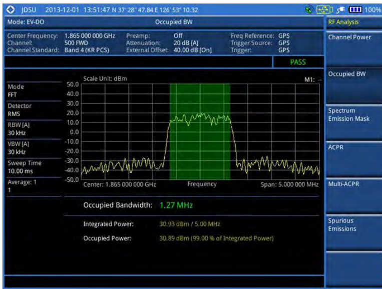
Figure 201 Occupied bandwidth measurement with EV-DO signal analyzer
