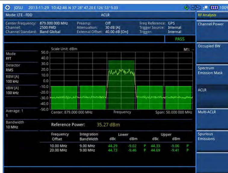
Figure 91 ACLR measurement with LTE-FDD signal analyzer
