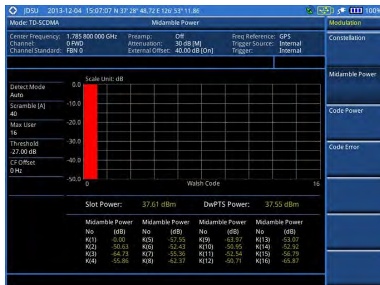
Figure 236 Midamble measurement with TD-SCDMA signal analyzer
