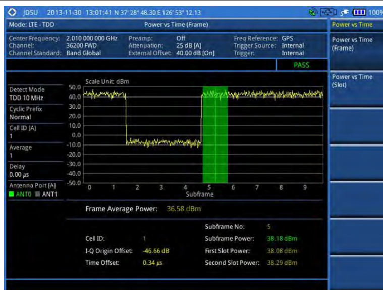
Figure 140 Power vs. time (frame) measurement with LTE – TDD signal analyzer
