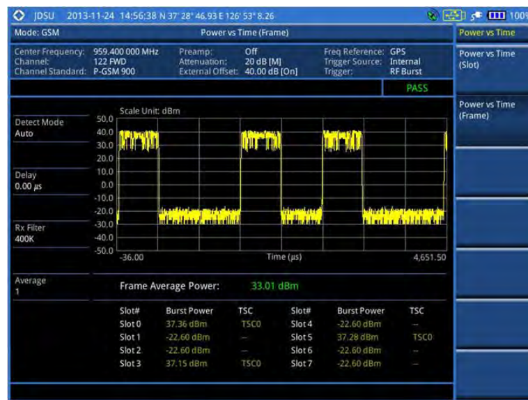
Figure 49 Power vs. time (frame) measurement with GSM signal analyzer
