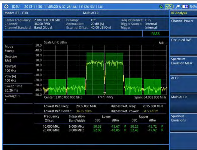
Figure 137 Multi-ACLR measurement with LTE-TDD signal analyzer
