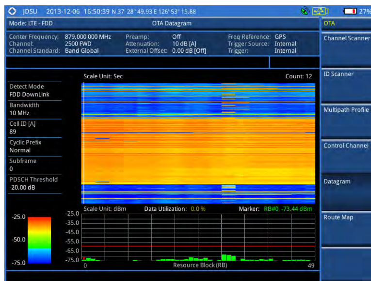
Figure 117 Datagram measurement with LTE-FDD signal analyzer
