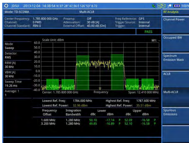
Figure 229 Multi-ACLR measurement with TD-SCDMA signal analyzer
