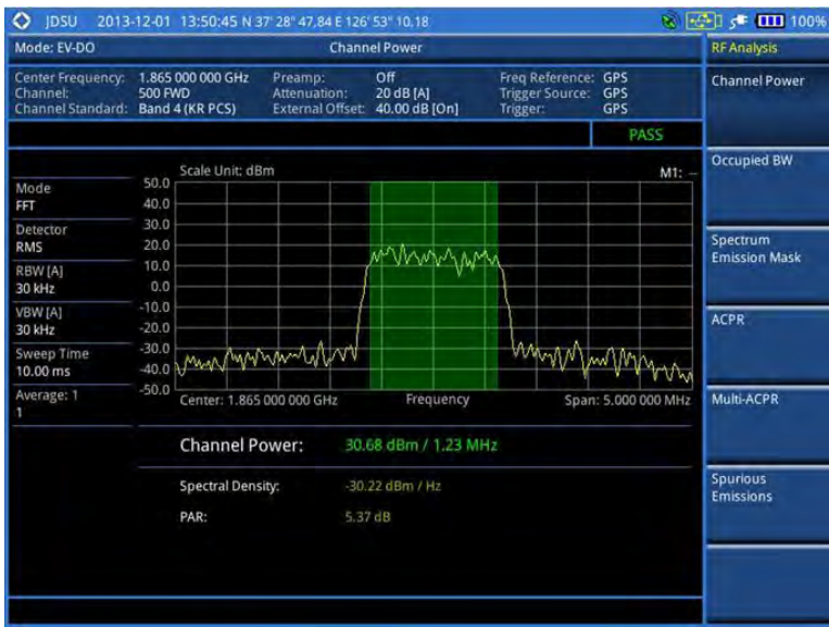
Figure 200 Channel power measurement with EV-DO signal analyzer
