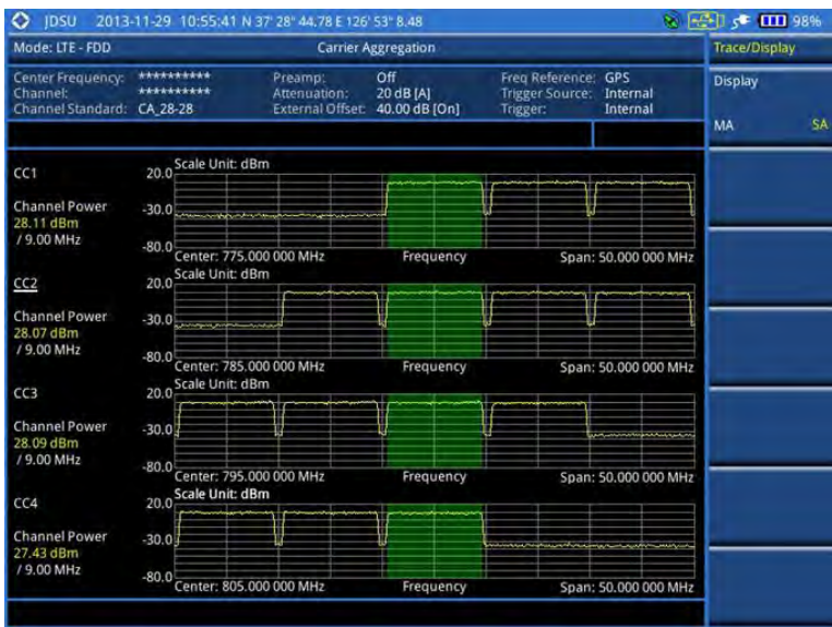
Figure 112 Carrier aggregation measurement with LTE-FDD signal analyzer (SA)
