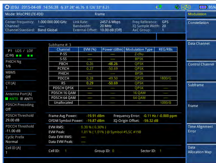
Figure 313 Frame measurement with RFoCPRI LTE-FDD signal analyzer
