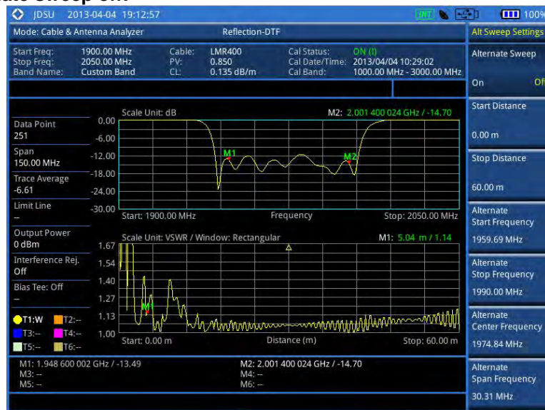
Figure 277 Reflection-DTF dual measurement
