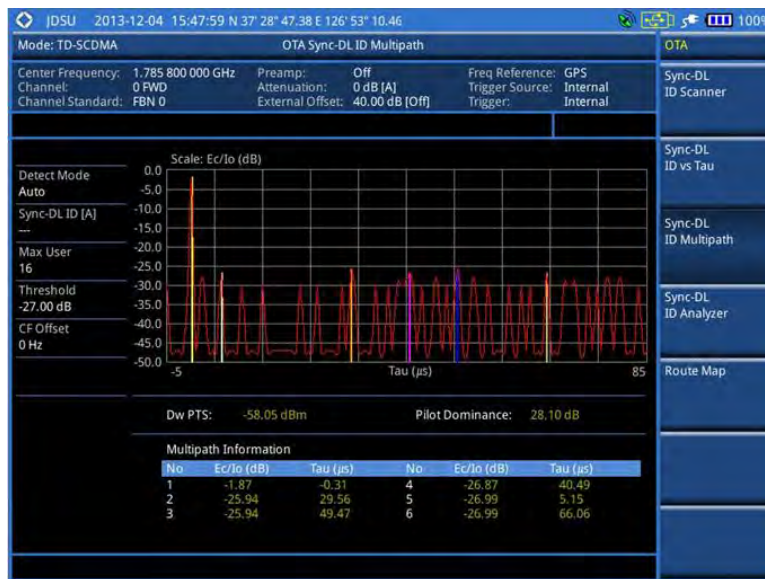
Figure 241 Sync-DL ID multipath measurement with TD-SCDMA OTA signal analyzer
