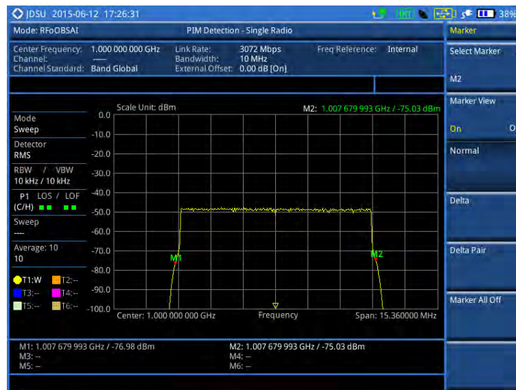
Figure 340 PIM detection of single radio
