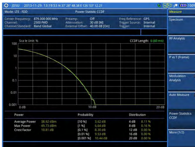
Figure 110 CCDF measurement with LTE-FDD signal analyzer
