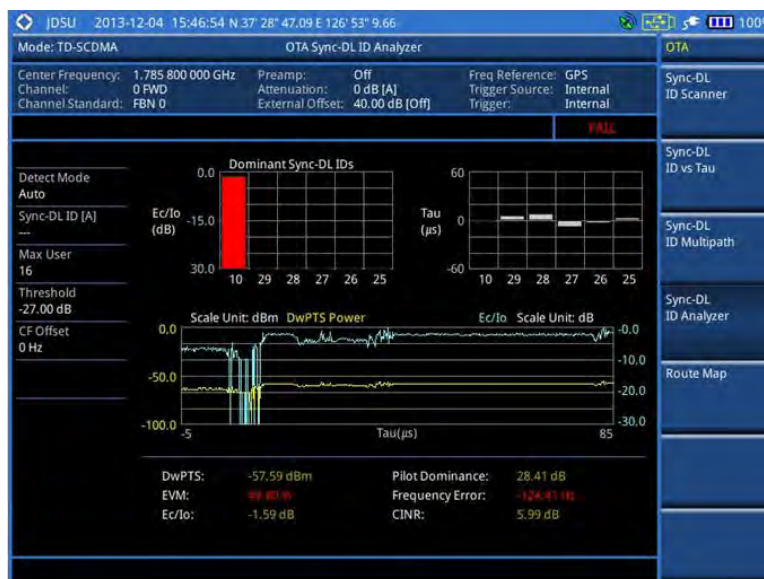
Figure 242 Sync-DL ID analyzer measurement with TD-SCDMA OTA signal analyzer
