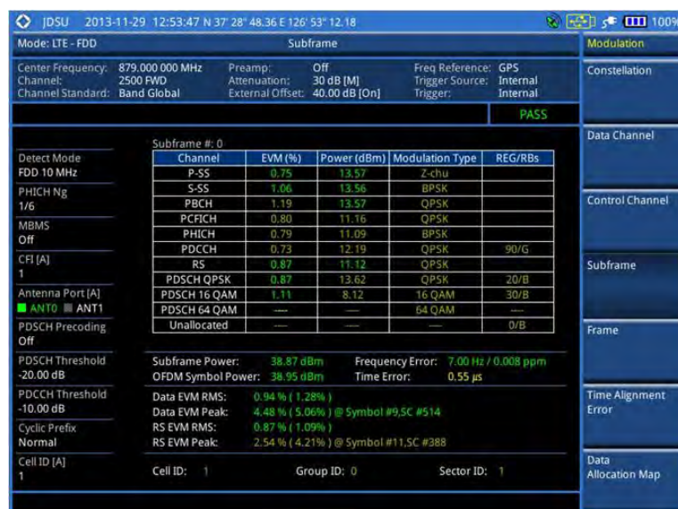
Figure 101 Subframe measurement with LTE-FDD signal analyzer
