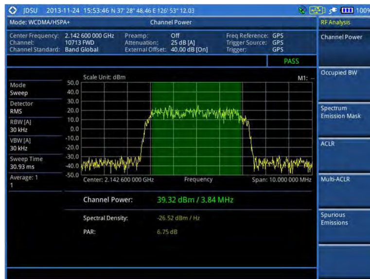
Figure 62 Channel power measurement with WCDMA/HSPA+ signal analyzer
