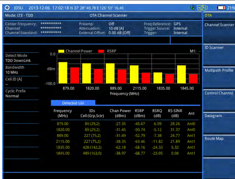
Figure 157 Channel scanner measurement with LTE-TDD OTA signal analyzer
