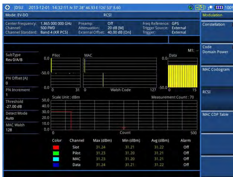
Figure 211 RCSI measurement with EV-DO signal analyzer
