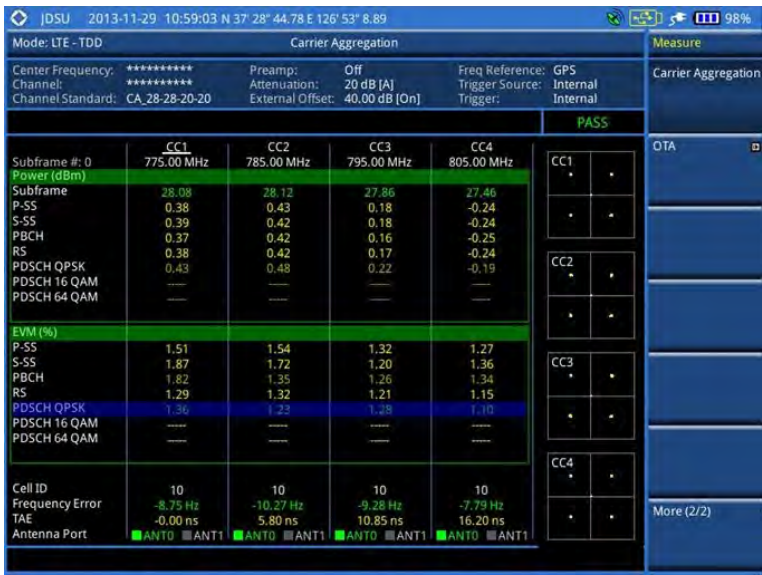
Figure 156 Carrier aggregation measurement with LTE-TDD signal analyzer (SA)
