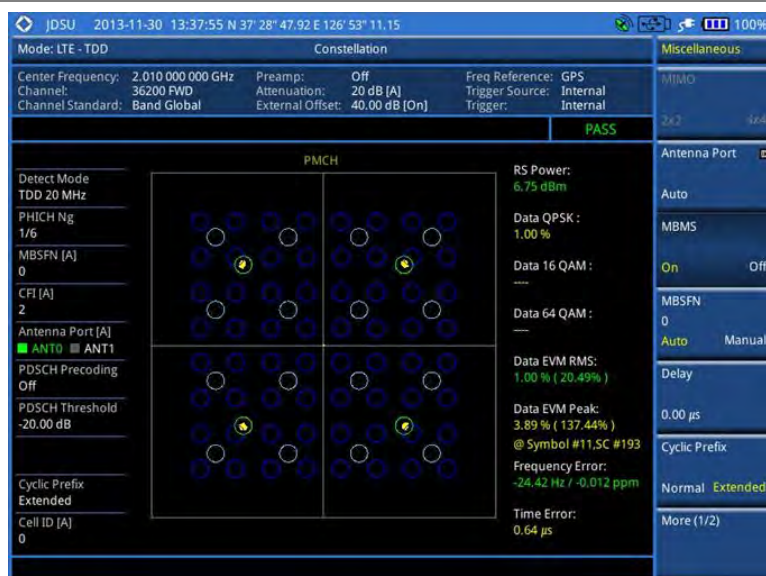
Figure 142 Constellation measurement with LTE-TDD signal analyzer (MBMS On)
