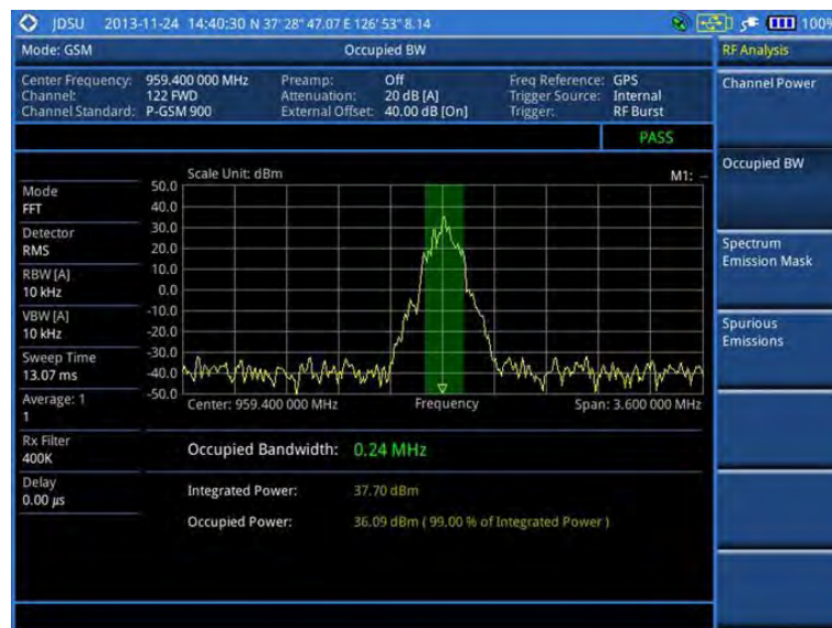
Figure 43 Occupied bandwidth measurement with GSM signal analyzer
