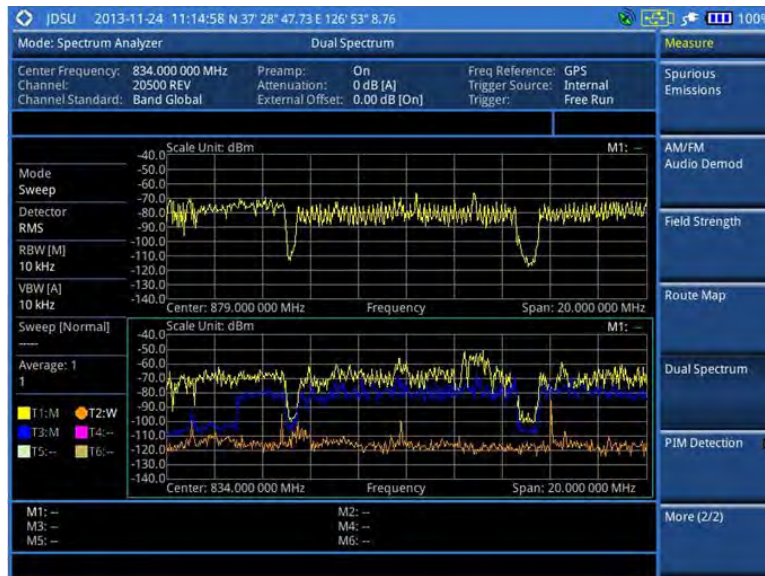
Figure 23 Dual spectrum measurement with spectrum analyzer
