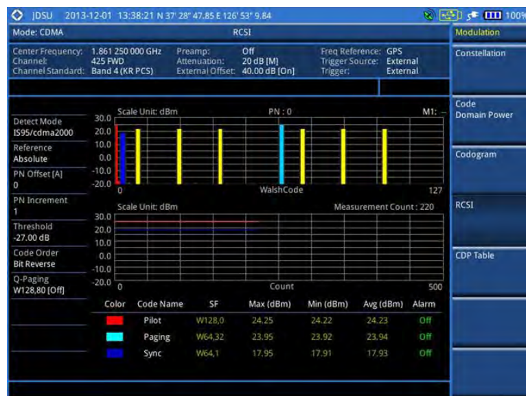
Figure 186 RCSI measurement with CDMA signal analyzer
