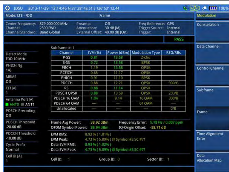
Figure 104 Frame measurement with LTE-FDD signal analyzer
