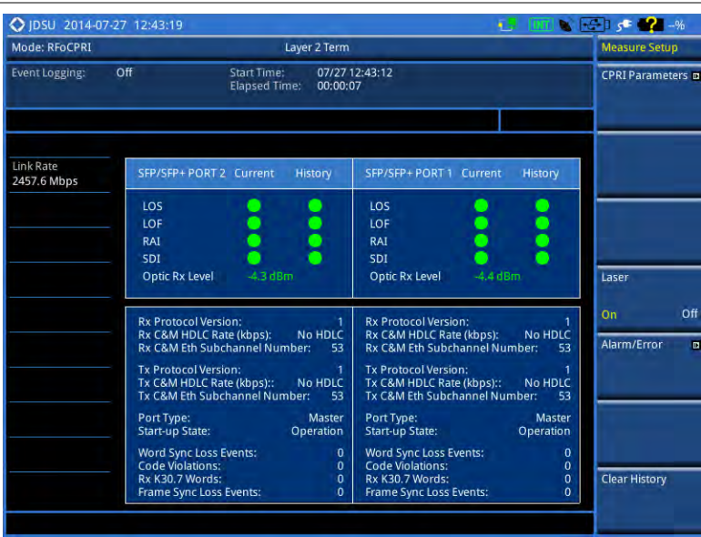
Figure 289 CPRI layer 2 term test
