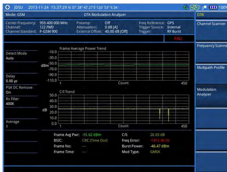
Figure 55 Modulation analyzer measurement with GSM OTA signal analyzer
