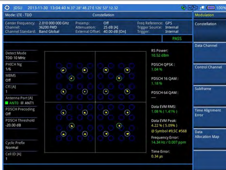
Figure 141 Constellation measurement with LTE-TDD signal analyzer
