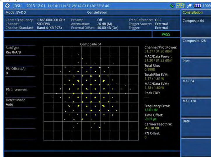
Figure 208 Constellation measurement with EV-DO signal analyzer
