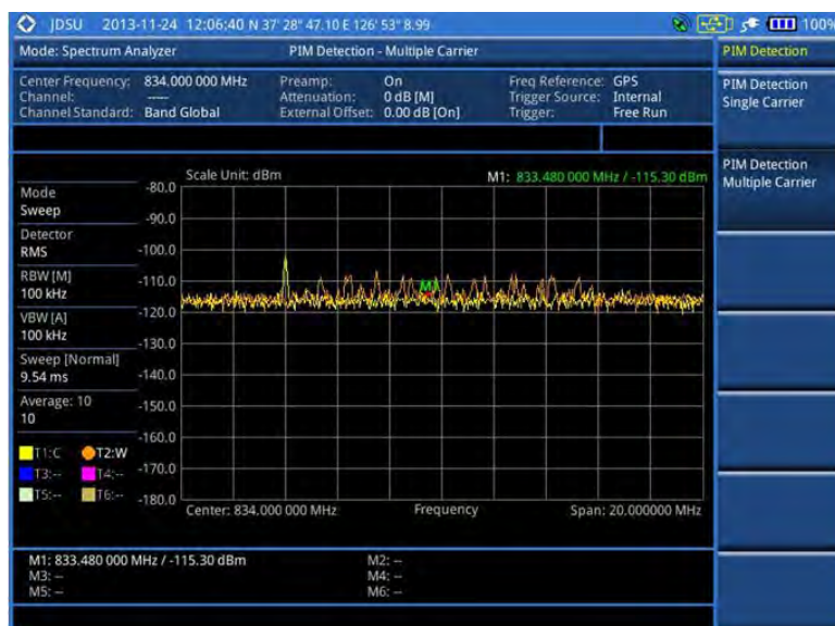
Figure 25 PIM detection for multiple carriers
