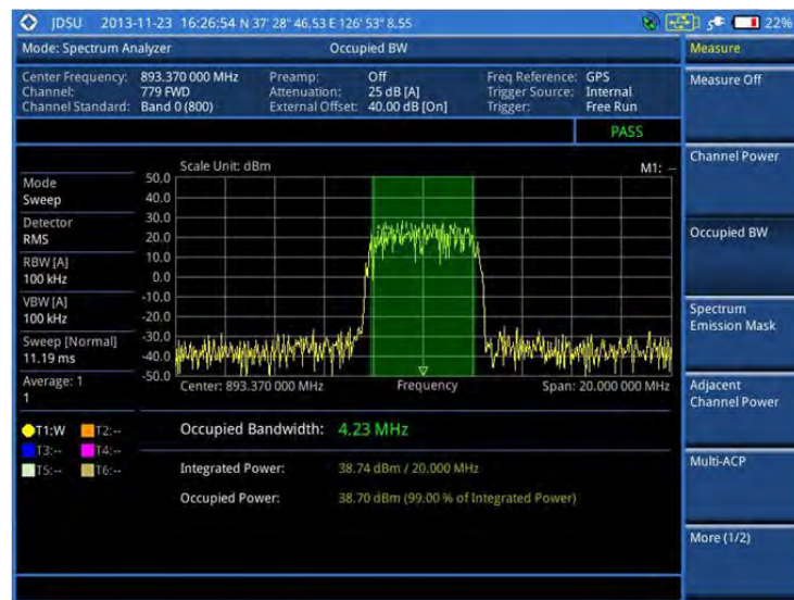
Figure 14 Occupied bandwidth measurement with spectrum analyzer
