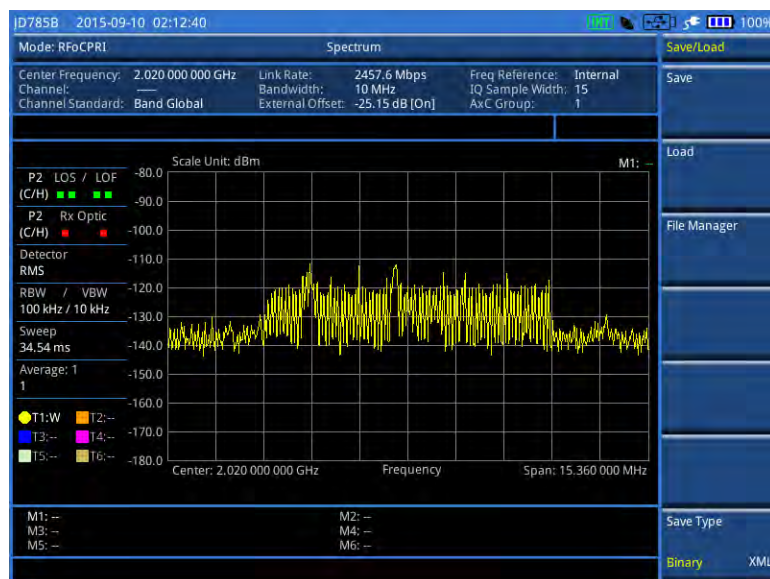
Figure 293 RFoCPRI spectrum measurement
