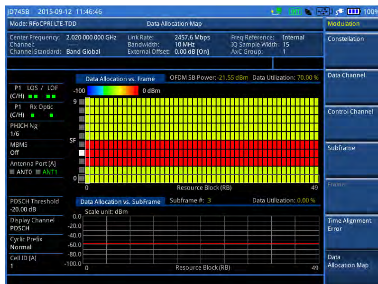
Figure 327 Data allocation map measurement with RFoCPRI LTE-TDD signal analyzer
