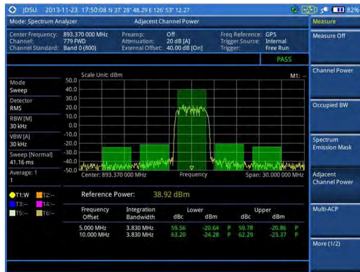
Figure 16 Adjacent channel power measurement with spectrum analyzer
