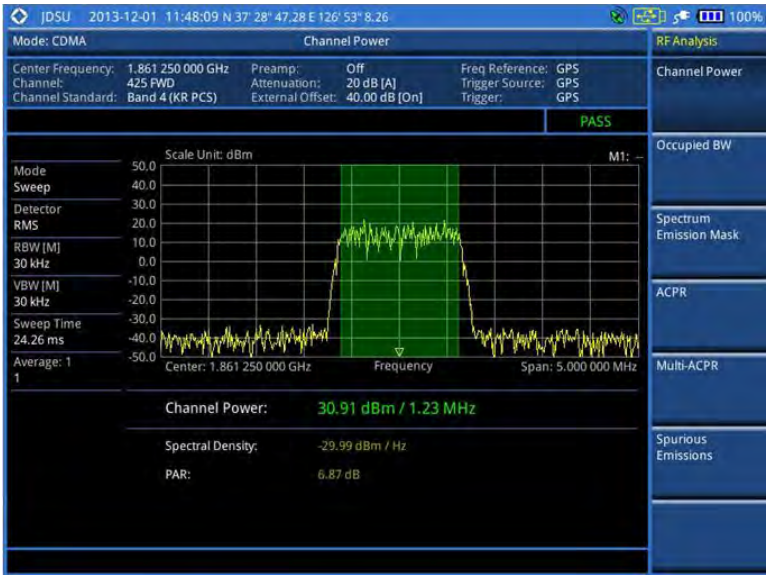
Figure 177 Channel power measurement with CDMA signal analyzer
