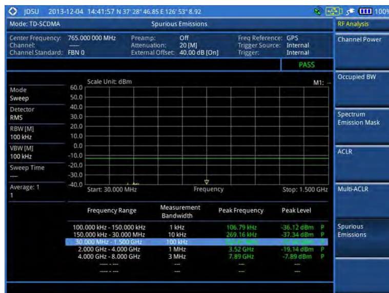
Figure 230 Spurious emissions measurement with TD-SCDMA signal analyzer
