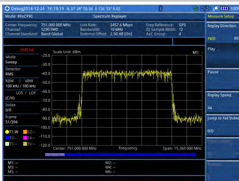
Figure 300 RFoCPRI spectrum replay
