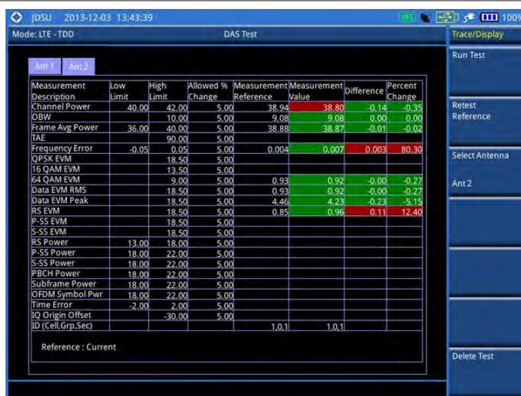
Figure 153 DAS measurement with LTE-TDD signal analyzer
