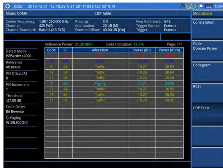
Figure 187 CDP Table measurement with CDMA signal analyzer
