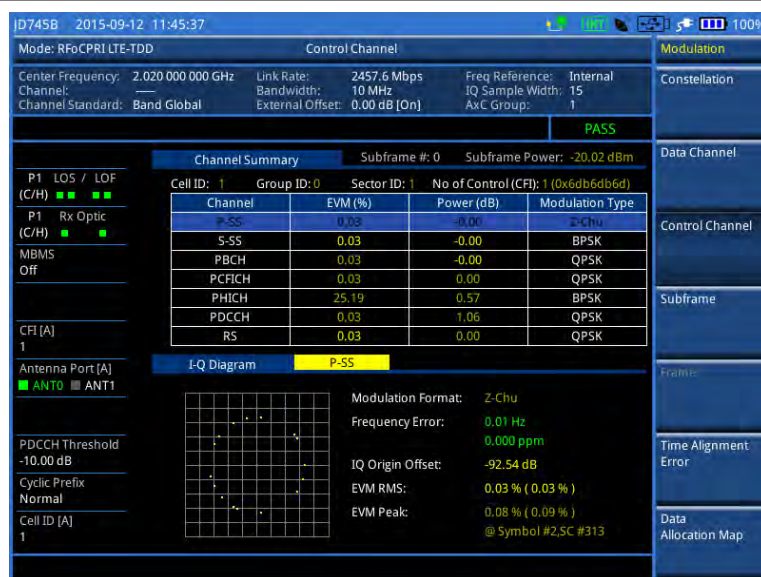
Figure 324 Control channel measurement with RFoCPRI LTE-TDD signal analyzer
