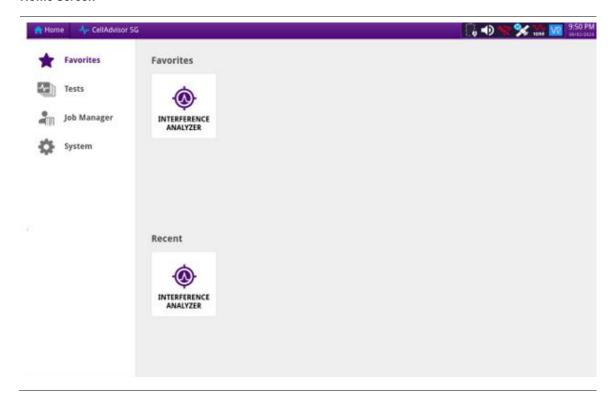
The Home screen provides access to the **Tests**, **Job Manager**, and **System** pages. You can return to the **Home** screen at any time by clicking the **Home** button in the top left corner of the screen.
