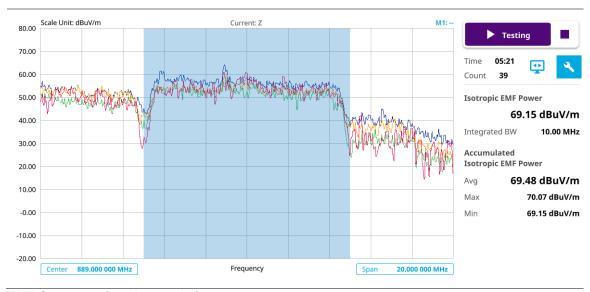
EMF Spectrum (level recorder) measurement
