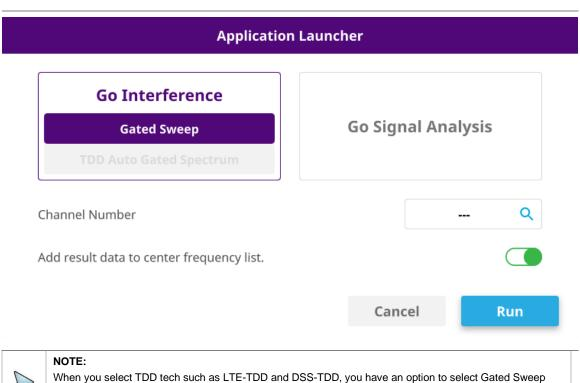
(only when you have Gated Sweep license) and the instrument moves to Gated Sweep Spectrum in Spectrum Analyzer.
