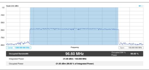
The Occupied Bandwidth measurement shows both of power across the band and power bandwidth in a user specified percentage to determine the amount of spectrum used by a modulated signal. Occupied bandwidth is typically calculated as the bandwidth containing 99% of the transmitted power.
