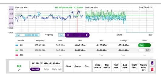
You can go to Menu > Limit to analyze your measurements with the display line, multi-segment line, and channel limit. See "Setting limit" for more details. Once you tap the vertical move bar and move it up and down, the reference line value changes.
