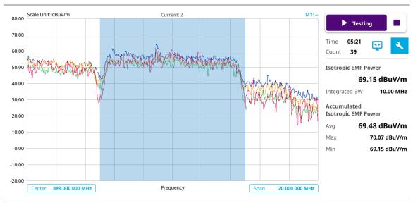
EMF Spectrum (level recorder) measurement
