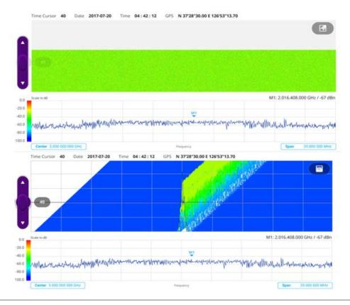
The Spectrogram shows a vertical line on the chart when the marker is enabled on the screen. The first figure shows Normal chart view, and the second figure below shows Waterfall (3D display) chart view.
