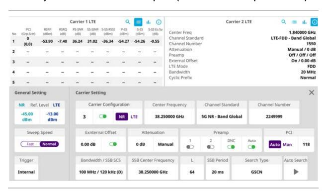
NSA analyzer measurement with sweep normal (chart view)
