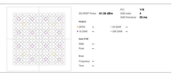
Constellation measurement with time offset histograrm with 5G NR Signal Analyzer
